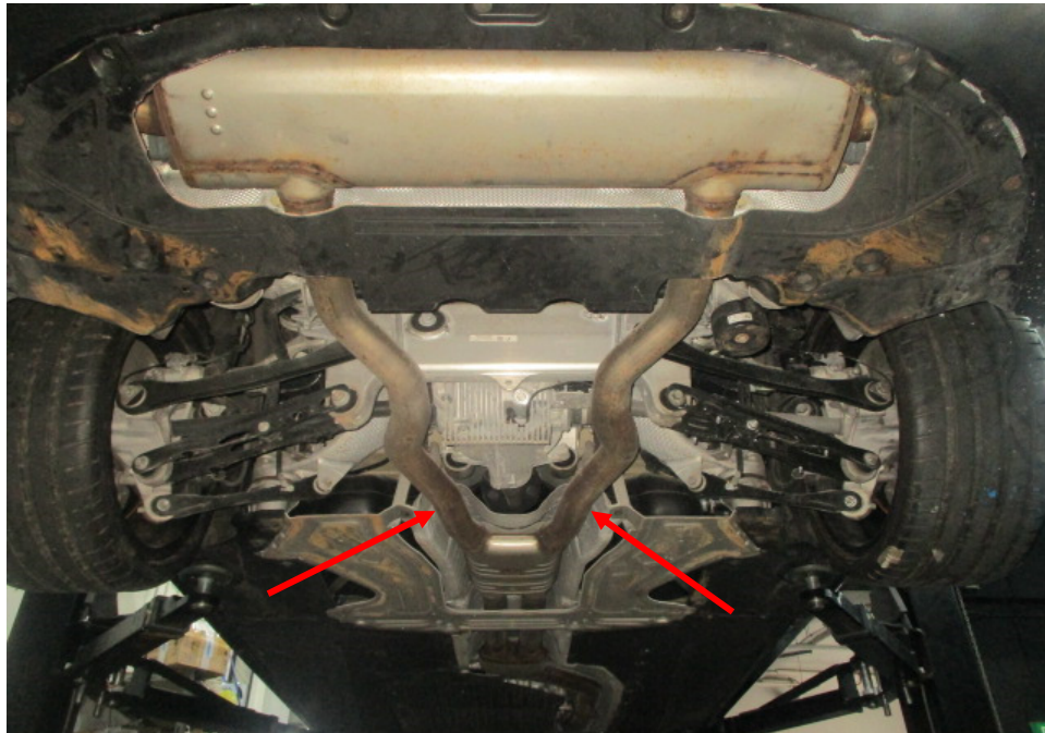
Photo 27 shows the rear section of the Motor Car's exhaust system. My examination of the Motor Car's exhaust system revealed no sign(s) or indication(s) of any cut or weld marks along its exhaust pipes (arrowed), on its rear muffler, on its centre resonator boxes and on its catalytic converter.
