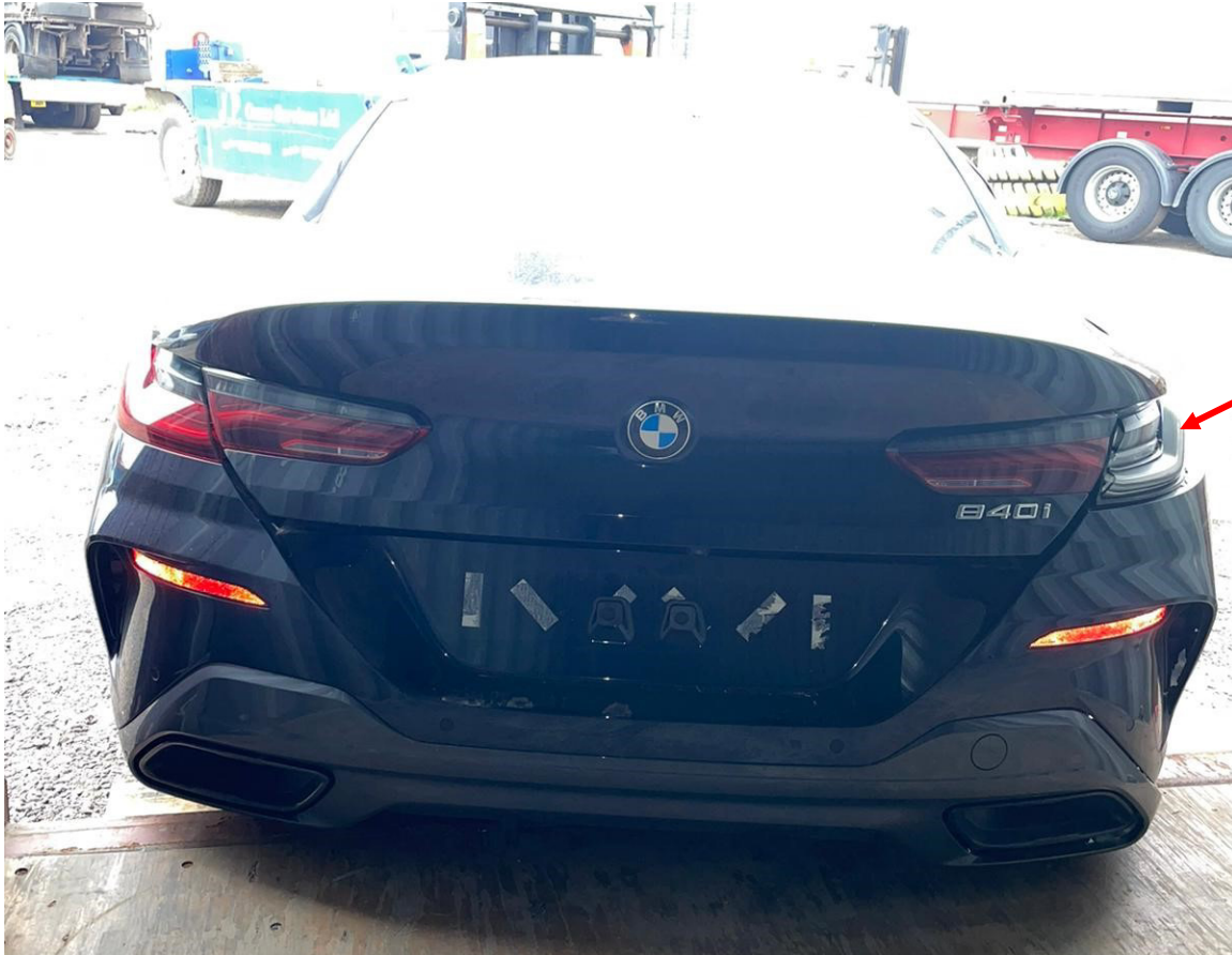
Photo 5 shows the rear body of the Motor Car (photograph provided to me). The rear right taillamp (arrowed) was observed to be broken. Apart for this, the rear body of the Motor Car was undamaged.
