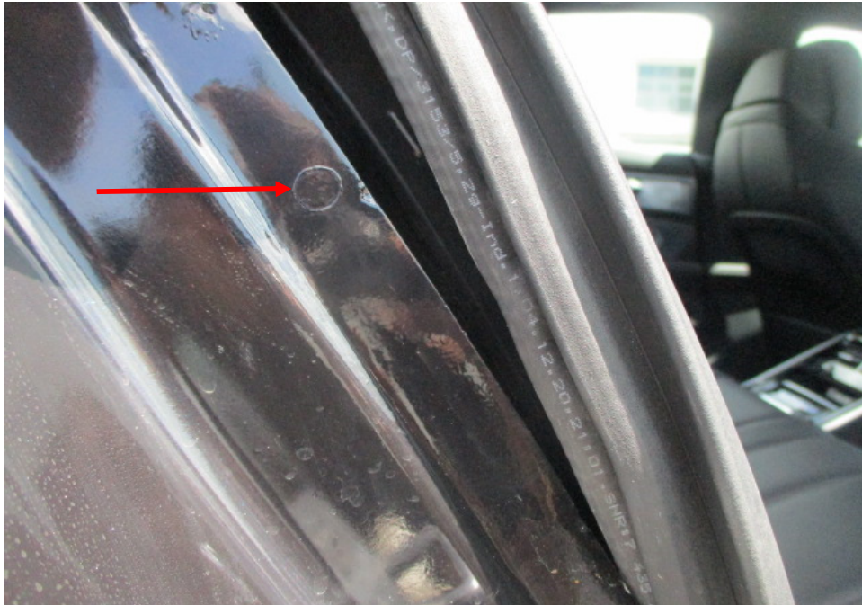
Photo 36 shows the right side "C" pillar of the Motor Car. I did not find any weld marks other than original spot weld marks (arrowed) on the right side "C" pillar of the Motor Car, which indicates that there was no re-welding works carried out. In general, I had found all the non-detachable body panels of the Motor Car to be originally fitted at the time of my inspection.
