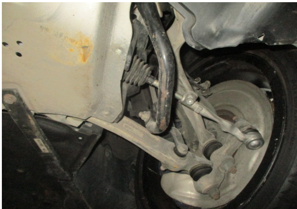
Photo 25 shows the various undercarriage components at the front left wheel of the Motor Car. The mechanical components, control arms and linkages were all found to be intact and secured in an appropriate manner.
