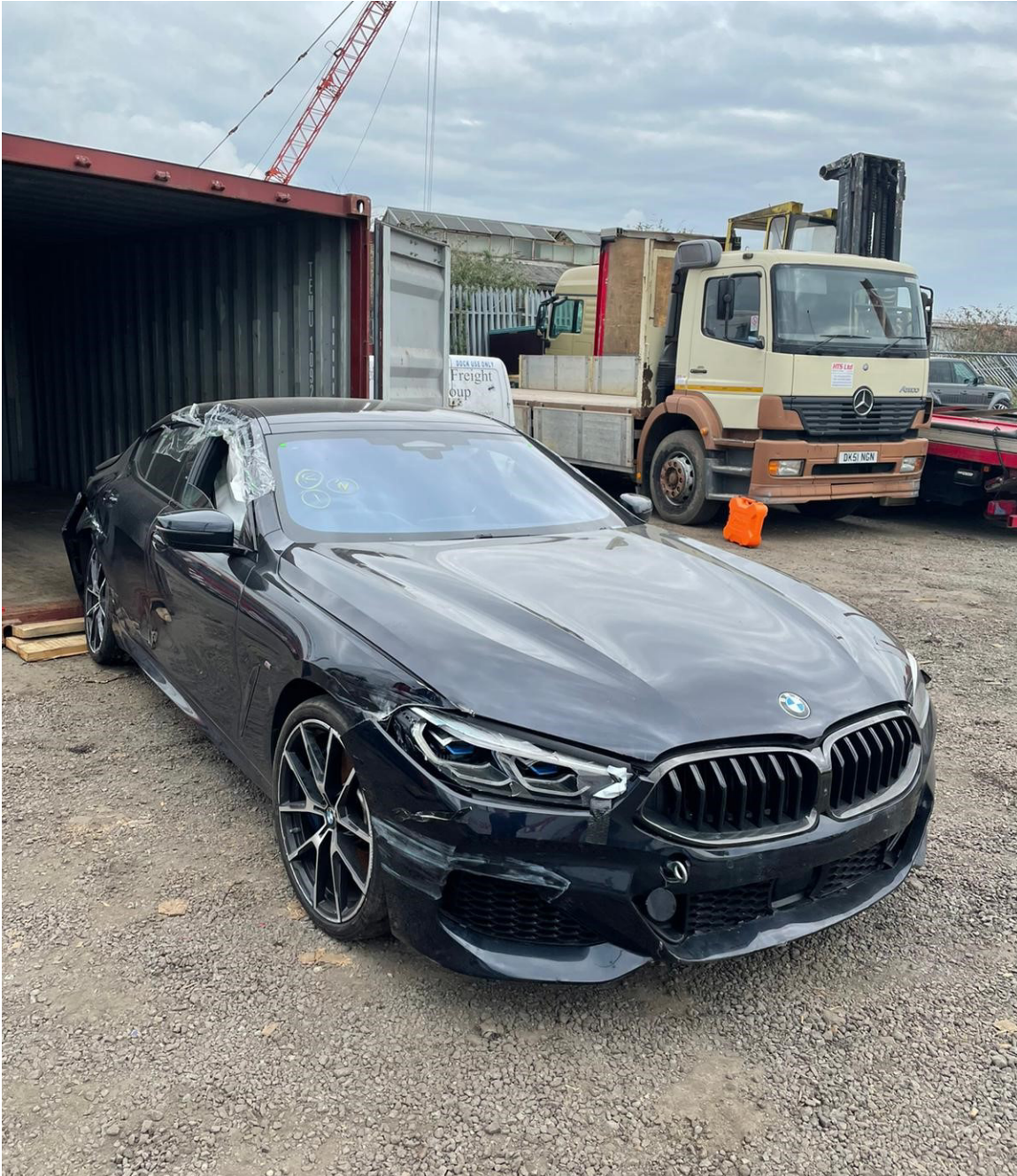
Photo 1 shows a general view of the front right body of the Motor Car (photograph provided to me). The Motor Car was observed to have sustained damage at its right side portion. The front bumper, front bonnet, front right headlamp, front right fender and front right wheel rim were amongst the body parts that were observed to have been damaged.
