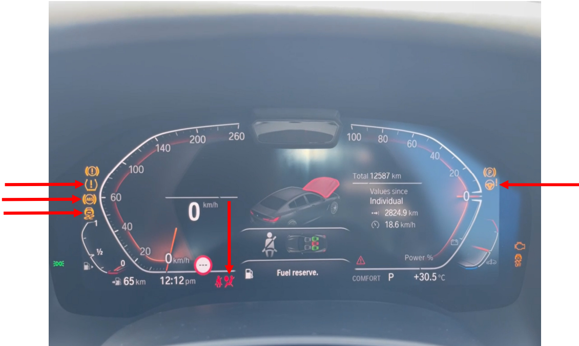
Photo 20 shows the warning lights for the various electronic safety features appearing on the instrument panel of the Motor Car during its self-test when the engine is cranked, in particular the ABS, SRS, IAS, TPM and DSC lights (arrowed).
