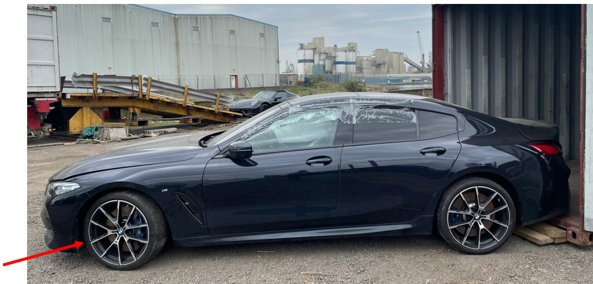
Photo 6 shows the left side body of the Motor Car (photograph provided to me). The left side portion of the Motor Car was observed to be undamaged. The Motor Car's front left wheel (arrowed) and front right wheel (refer to photograph 2 & 3 above) were both orientated inwards. This would suggest damage to the undercarriage parts at the front right wheel of the Motor Car.
