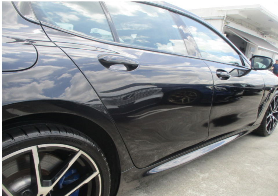
Photo 13 shows a closer view of the Motor Car's rear right fender, rear right door and right side rocker panel garnish. The body parts at the right side rear portion of the Motor Car were visually examined and it was observed that the repair/restoration works carried out to the damaged area of the Motor Car (refer to photograph 3 & 4 above) were reasonably adequate and in order.
