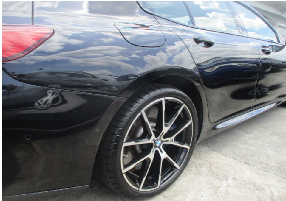
Photo 12 shows a closer view of the Motor Car's rear bumper, rear right taillamp, rear right fender and rear right wheel rim. The body parts at the right side rear portion of the Motor Car were visually examined and it was observed that the repair/restoration works carried out to the damaged area of the Motor Car (refer to photograph 4 & 5 above) were reasonably adequate and in order.
