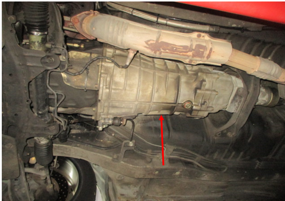
Photo 3 shows another view of the transmission assembly (arrowed) that was fitted on the Motor Car, as viewed from the left to right. The front (input) side of the transmission assembly is bolted to the crankshaft side of the engine block while the rear (output) side of the transmission assembly, connects to the propeller shaft, which links to the differential at the rear axle of the Motor Car.
