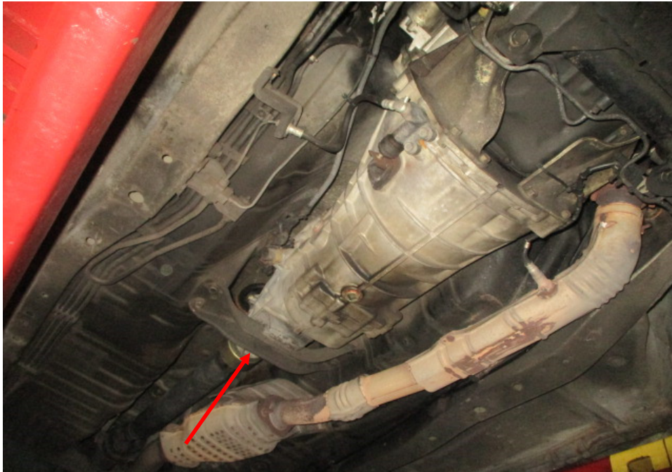
Photo 4 shows a general view of the bracket (arrowed) that was mounted to the underside of the Motor Car's floorboard, via bolts and nuts. The bracket supports the rear (output) side of the transmission assembly.
