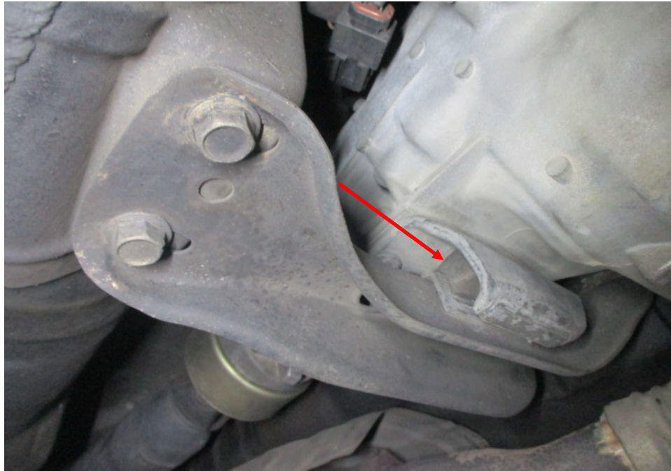
Photo 6 shows the rubber bushing (arrowed), sitting between the transmission assembly and the bracket. The rubber bushing absorbs any vibrations arising from the rotation of the transmission gears, minimising any stress to the bracket.
