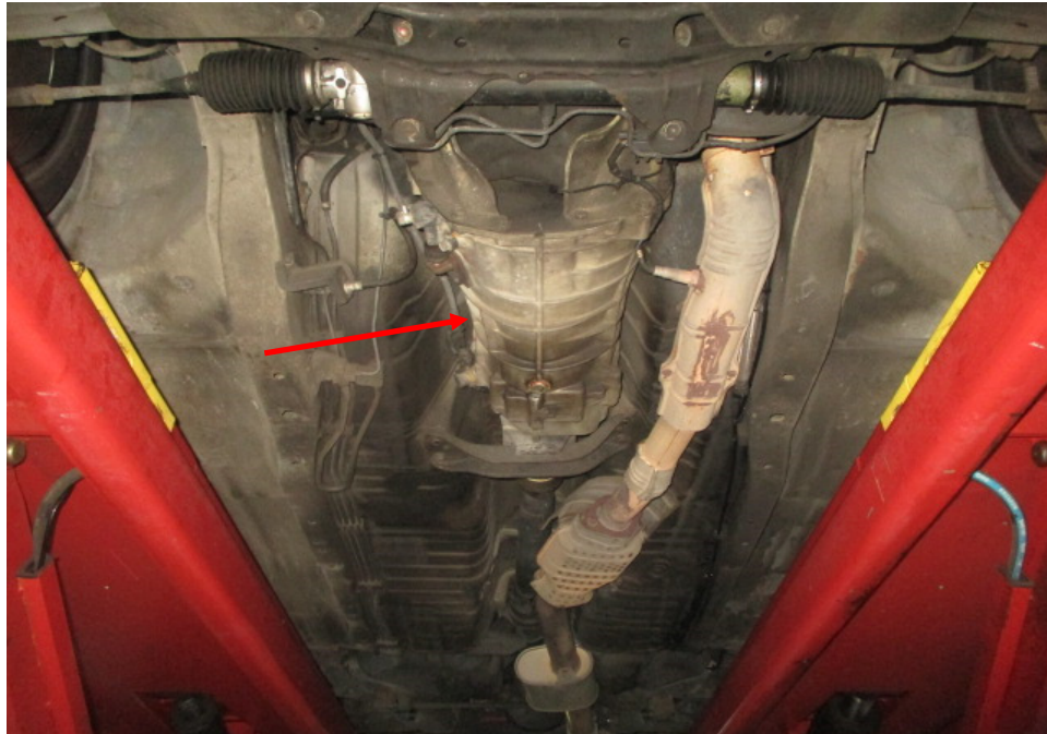
Photo 2 shows a general view of the transmission assembly (arrowed) that was fitted on the Motor Car, as viewed from the front to rear. The front (input) side of the transmission assembly is bolted to the crankshaft side of the engine block while the rear (output) side of the transmission assembly, connects to the propeller shaft, which links to the differential at the rear axle of the Motor Car.
