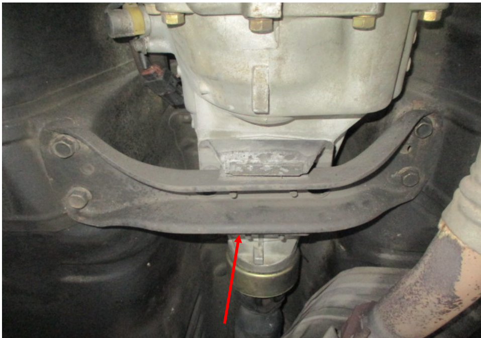
Photo 5 shows a closer view of the bracket (arrowed) that was mounted to the underside of the Motor Car's floorboard, via bolts and nuts. The bracket supports the rear (output) side of the transmission assembly. The bracket was also with rubber bushings that absorb any vibrations arising from the rotation of the transmission gears, minimising any stress to the bracket.
