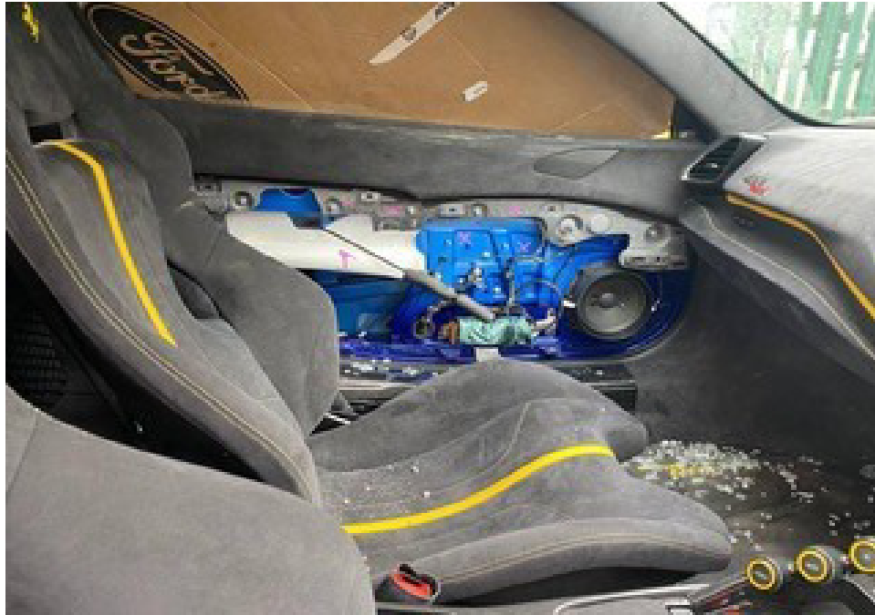
Photo 6 shows the interior compartment of the Motor Car (photograph provided to me). The Motor Car's front left door window was observed to be shattered. Its front left door inner trimboard was also missing/dislodged/damaged. The Motor Car's airbag(s) was not deployed.
