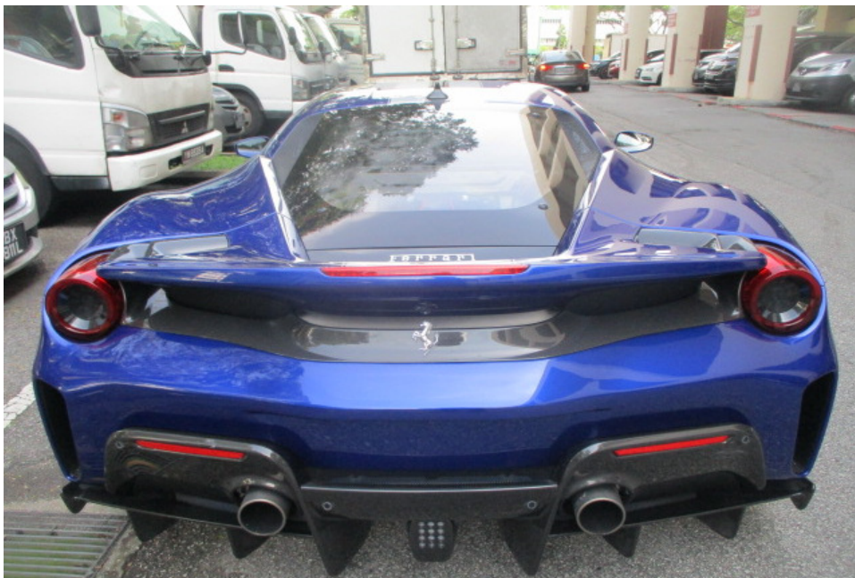
Photo 9 shows a closer view of the Motor Car's rear left taillamp, rear right taillamp, rear centre top garnish, rear bumper, rear bumper lower cover, rear bumper left reflector and rear bumper right reflector. The body parts at the rear portion of the Motor Car were visually examined and it was observed that the repair/restoration works carried out to the damaged area of the Motor Car (refer to photograph 4 & 5 above) were reasonably adequate and in order.
