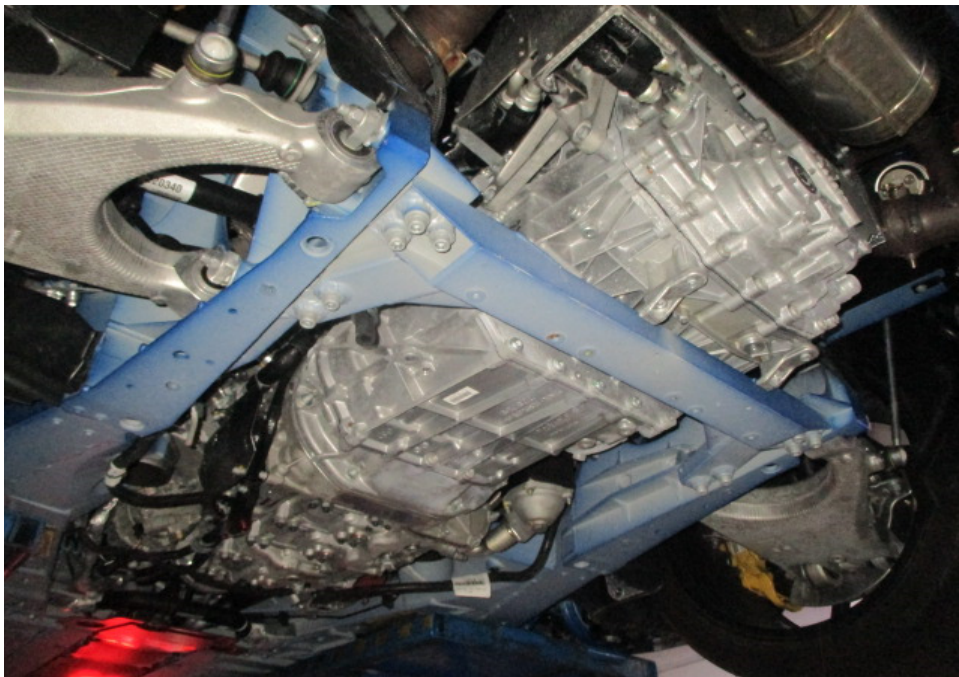
Photo 33 shows the Motor Car's engine compartment as viewed from the rear underside of the Motor Car. The various parts and components inside the engine compartment were all observed to be intact and properly fitted. There was also no sign(s) or indication(s) of fluid leak and/or fluid stain found inside the engine compartment.
