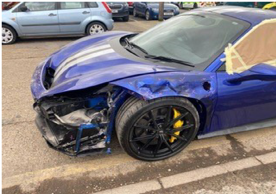
Photo 3 shows the left side front body of the Motor Car (photograph provided to me). The Motor Car's front left fender was observed to be dented. The front left fender emblem, front left fender inner shield and front left signal lamp amongst others were missing/dislodged/damaged.
