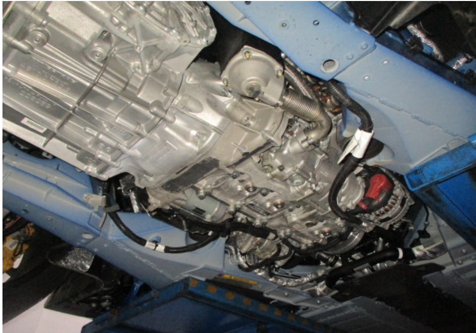
Photo 34 shows another view of the Motor Car's engine compartment as viewed from the rear underside of the Motor Car. The various parts and components inside the engine compartment were all observed to be intact and properly fitted. There was also no sign(s) or indication(s) of fluid leak and/or fluid stain found inside the engine compartment.
