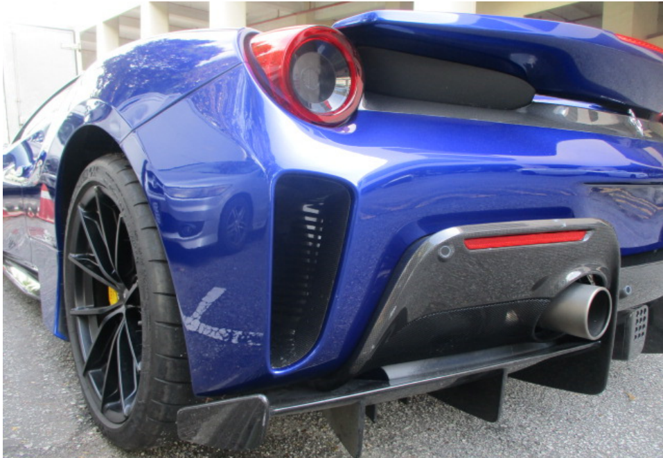
Photo 8 shows a closer view of the Motor Car's rear left taillamp, rear left exhaust tip, rear bumper, rear bumper lower cover, rear bumper left reflector, rear bumper left side garnish and rear bumper sensors. The body parts at the rear portion of the Motor Car were visually examined and it was observed that the repair/restoration works carried out to the damaged area of the Motor Car (refer to photograph 4 & 5 above) were reasonably adequate and in order.
