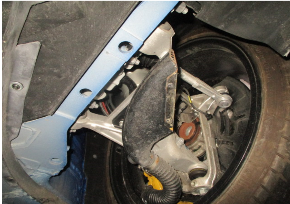
Photo 30 shows the various undercarriage components at the front left wheel of the Motor Car. The mechanical components, control arms and linkages were all found to be intact and secured in an appropriate manner.
