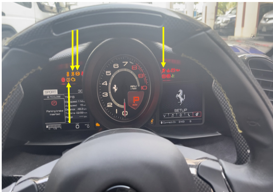
Photo 25 shows the warning lights for the various electronic safety features appearing on the instrument panel of the Motor Car during its self-test when the engine is cranked, in particular the ABS, SRS, TPM and TCS lights (arrowed).
