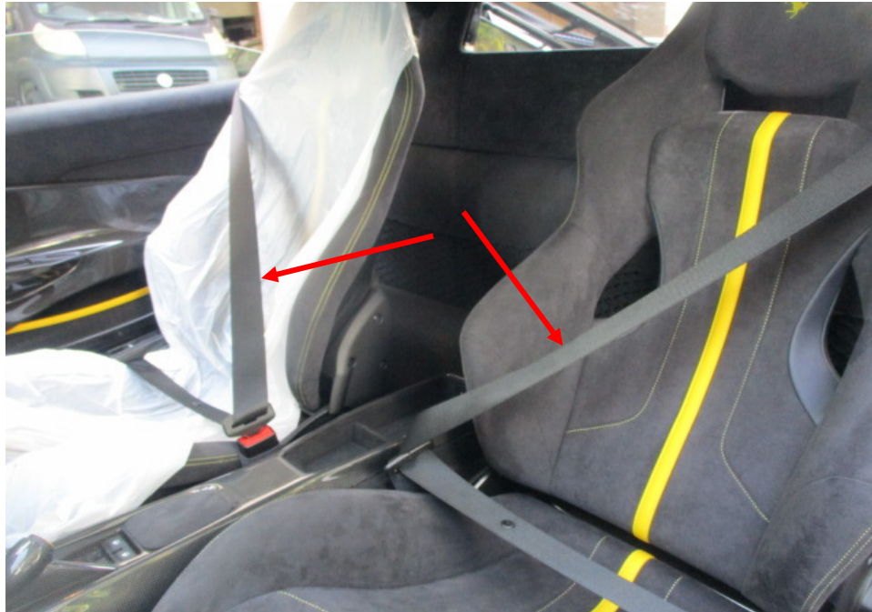
Photo 24 shows the seats of the Motor Car. All the seats of the Motor Car were secured via seat rails to the floorboard. They were also fitted with a retractable seat belt reel and a pre-tensioner. The seat belts (arrowed) were tested and were able to be fastened into the respective pre-tensions that were fitted on the side of each individual seat.
