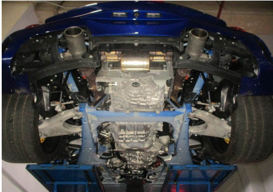
Photo 32 shows the Motor Car's exhaust system after removal of the rear bumper lower cover and rear under cover. In general, my examination of the Motor Car's exhaust system revealed no sign(s) or indication(s) of any cut or weld marks along its exhaust pipes, on its catalytic converters and on its rear muffler.
