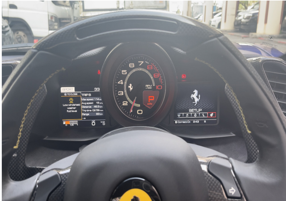
Photo 26 shows the respective warning lights no longer illuminated, indicating that there is no fault detected to the ABS, SRS TPM and TCS systems of the Motor Car during the self-test. These electronic systems were hence in working condition at the time of my inspection.
