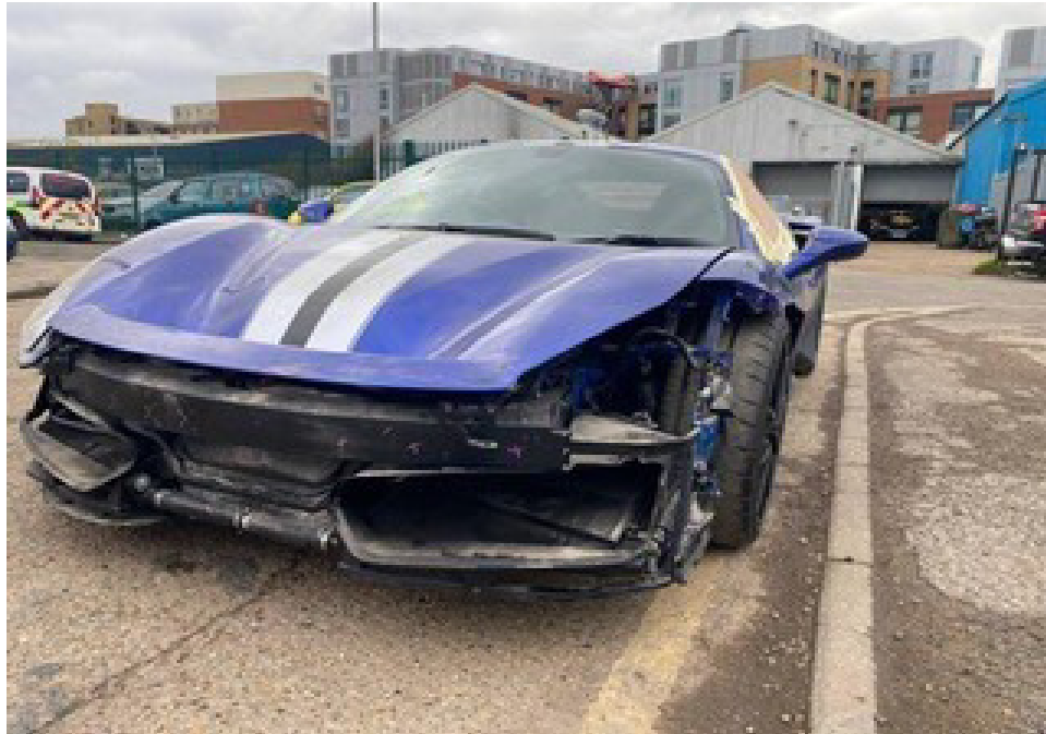
Photo 2 shows the front left body of the Motor Car (photograph provided to me). The photographs provided to me had showed the front left headlamp, front bumper and all its related parts and attachments like the front bumper left lower lip, front bumper left side bracket, front bumper left lower grille, front bumper centre lower carbon garnish and front bumper sensors amongst others, missing/dislodged/damaged.
