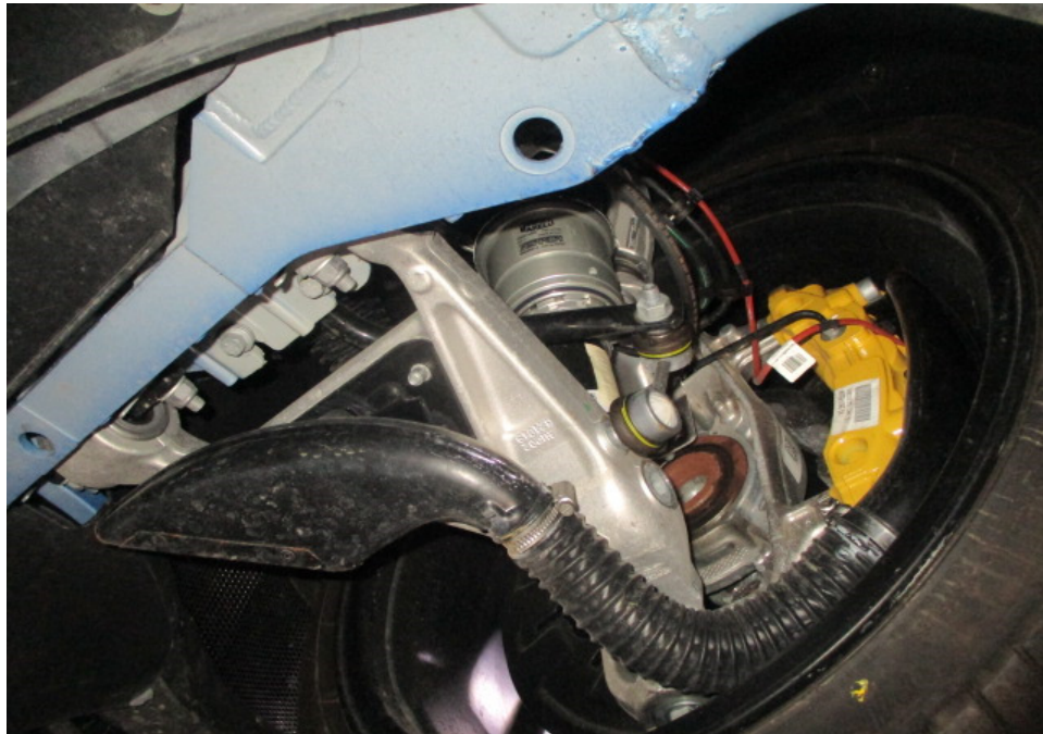
Photo 31 shows the various undercarriage components at the front right wheel of the Motor Car. The mechanical components, control arms and linkages were all found to be intact and secured in an appropriate manner. I also did not observe any fluid leak and/or fluid stain on the underside of the Motor Car.
