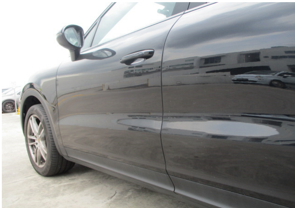
Photo 9 shows a closer view of the Motor Car's rear left door, rear left door lower moulding, front left door and front left door lower moulding. The body parts at the left side centre portion of the Motor Car were visually examined and it was observed that the repair/restoration works carried out to the damaged area of the Motor Car (refer to photograph 1 & 2 above) were reasonably adequate and in order.
