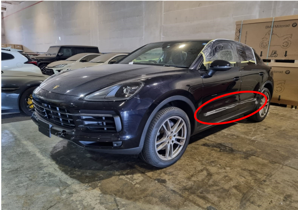
Photo 1 shows the front left body of the Motor Car (photograph provided to me). The Motor Car was observed to have sustained damage at its left side centre portion (circled). Its front left door and rear left door were damaged. The Motor Car's airbag (s) was not deployed as seen from the photographs that were provided to me.
