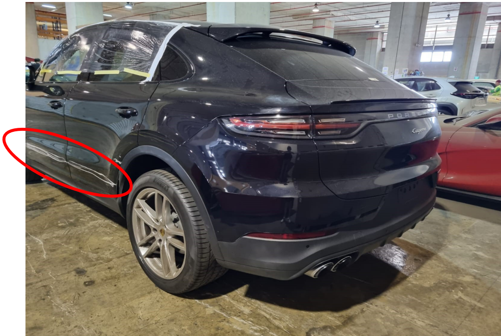
Photo 2 shows the rear left body of the Motor Car (photograph provided to me). The Motor Car was observed to have sustained damage at its left side centre portion (circled). Its front left door and rear left door were damaged.
