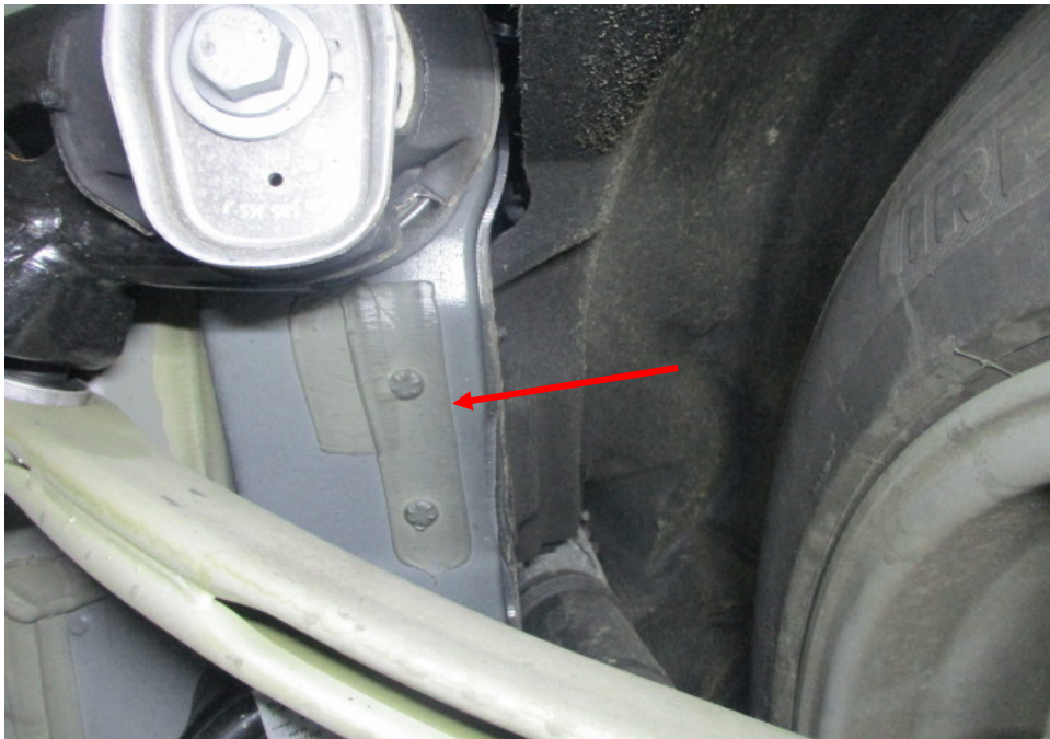
Photo 25 shows the chassis/structural body at the underside rear right of the Motor Car. I did not find any weld marks other than original spot weld marks on the chassis/structural body of the Motor Car. The original factory sealant (arrowed) at the joints along the chassis/structural body was untouched, indicating no work was done on the chassis/structural body of the Motor Car and that the chassis/structural body was originally fitted.
