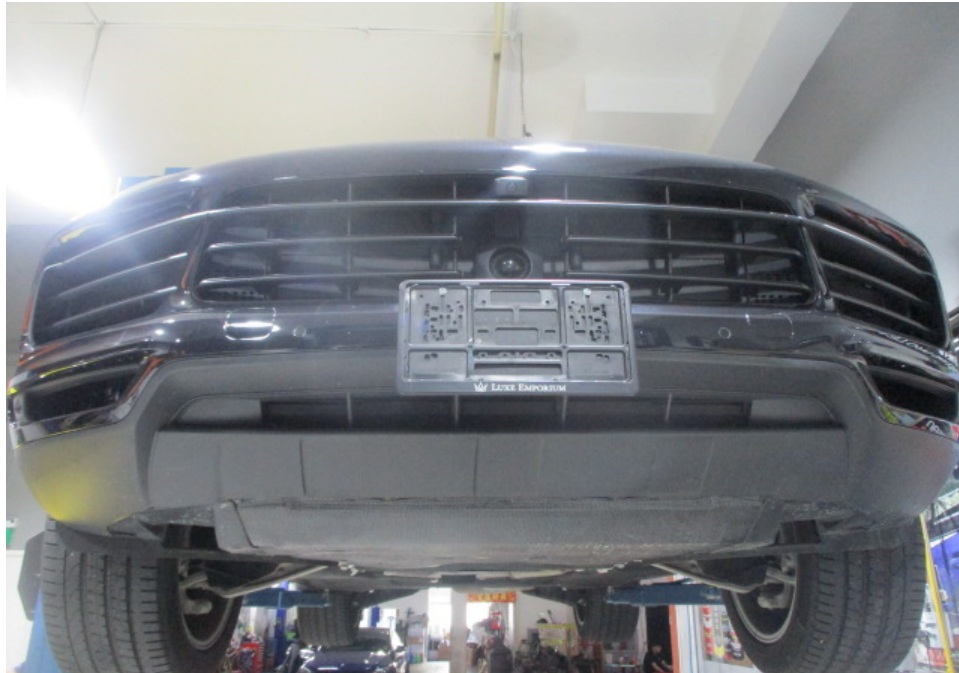
Photo 18 shows the Motor Car hoisted up for checks on its undercarriage. There was no sign(s) or indication(s) of fluid leakage and/or fluid stain(s) on the underside of the Motor Car. The undercarriage components of the Motor Car were also all observed to be intact and secured in an appropriate manner.
