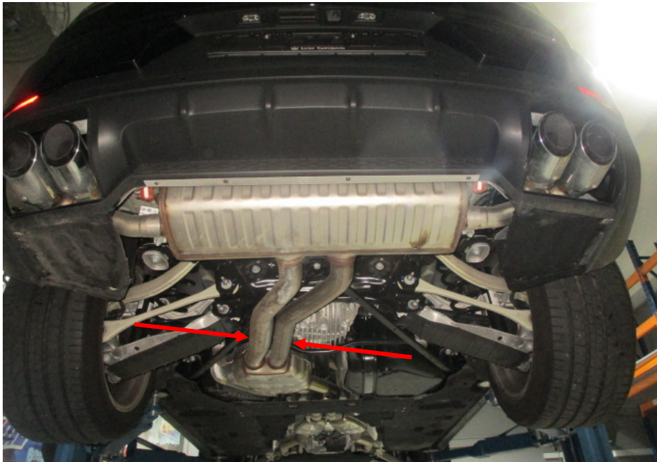
Photo 23 shows the rear section of the Motor Car's exhaust system. My examination of the Motor Car's exhaust system revealed no sign(s) or indication(s) of any cut or weld marks along its exhaust pipes (arrowed), on its rear muffler, on its centre resonator boxes and on its catalytic converters.
