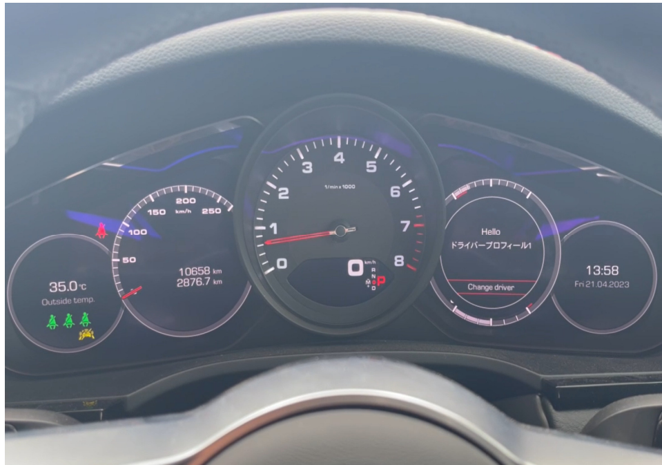
Photo 17 shows the respective warning lights no longer illuminated, indicating that there is no fault detected to the ABS, SRS, TPM, EPS and TCS systems of the Motor Car during the self-test. These electronic systems were hence in working condition at the time of my inspection.
