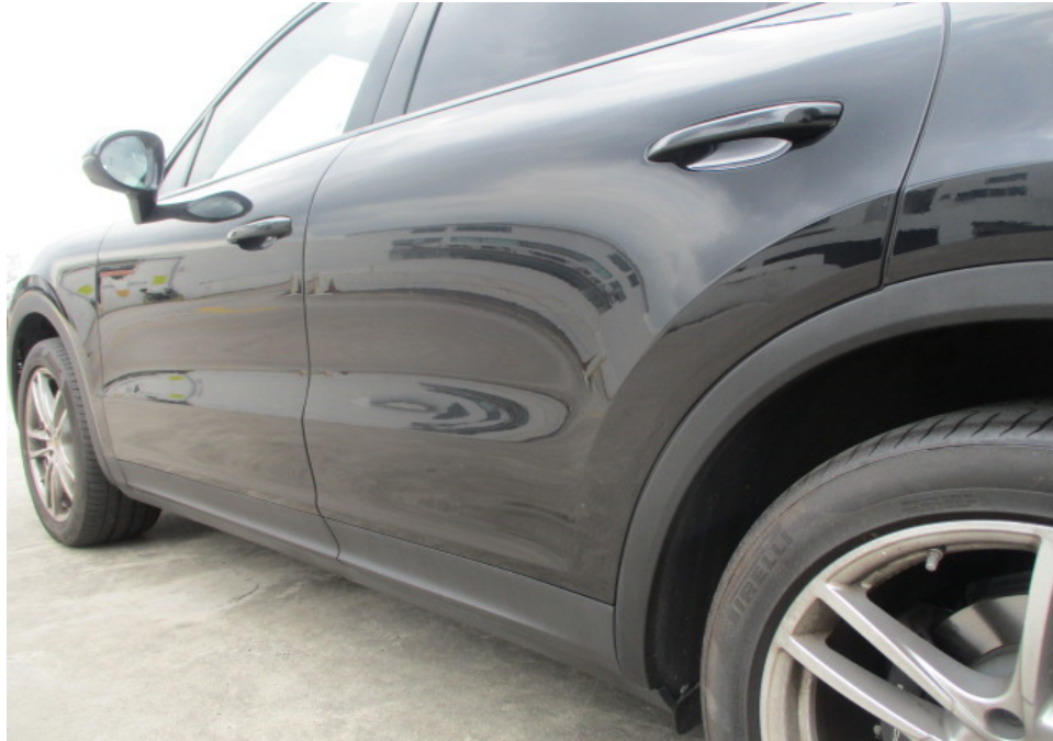
Photo 8 shows a closer view of the Motor Car's rear left fender, rear left fender wheel arc garnish and rear left door. The body parts at the left side centre portion of the Motor Car were visually examined and it was observed that the repair/restoration works carried out to the damaged area of the Motor Car (refer to photograph 1 & 2 above) were reasonably adequate and in order.
