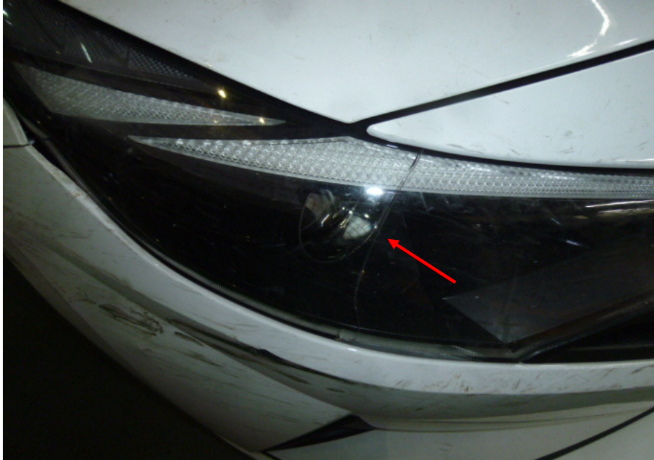
Photo 5 shows the cracked right front headlamp of the Insured Vehicle as a result of the accident (arrowed).
