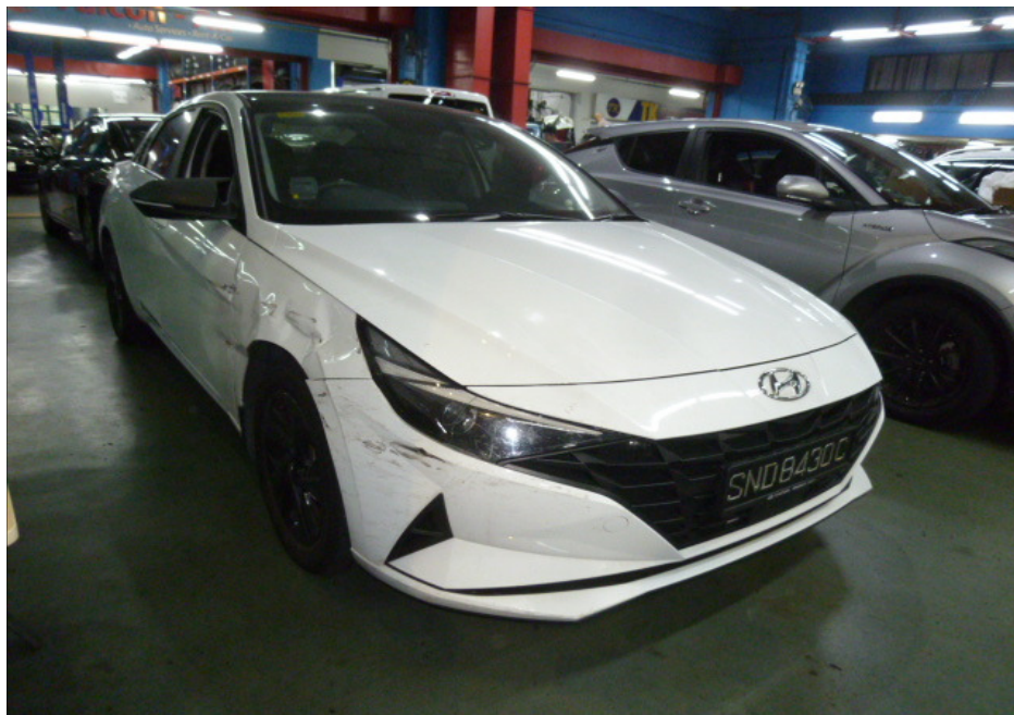
Photo 4 shows the general frontal right portion of the Insured Vehicle during the physical inspection at Falcon. The Insured Vehicle had sustained significant damages to its right body, particularly to its right front headlamp, front bumper, right front fender, driver door, right rear door, rear bumper and right wheel rims as a result of the incident.
