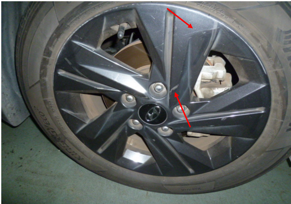
Photo 10 shows a closer view of the relatively minor marks of grazing nature observed around the right front wheel rim (arrowed) of the Insured Vehicle during the physical inspection at Falcon.
