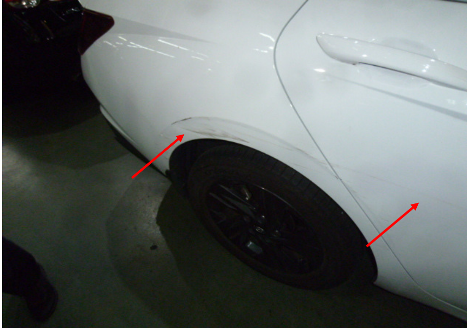
Photo 9 shows the grazed right rear door and rear bumper of the Insured Vehicle as a result of the accident (arrowed).
