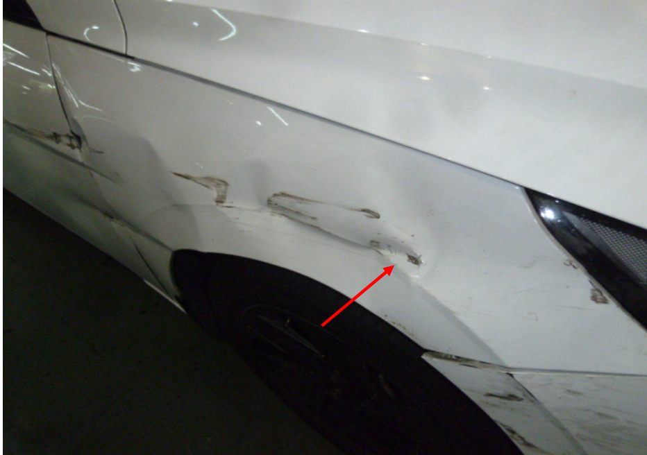
Photo 7 shows the dented right front fender of the Insured Vehicle as a result of the accident (arrowed).
