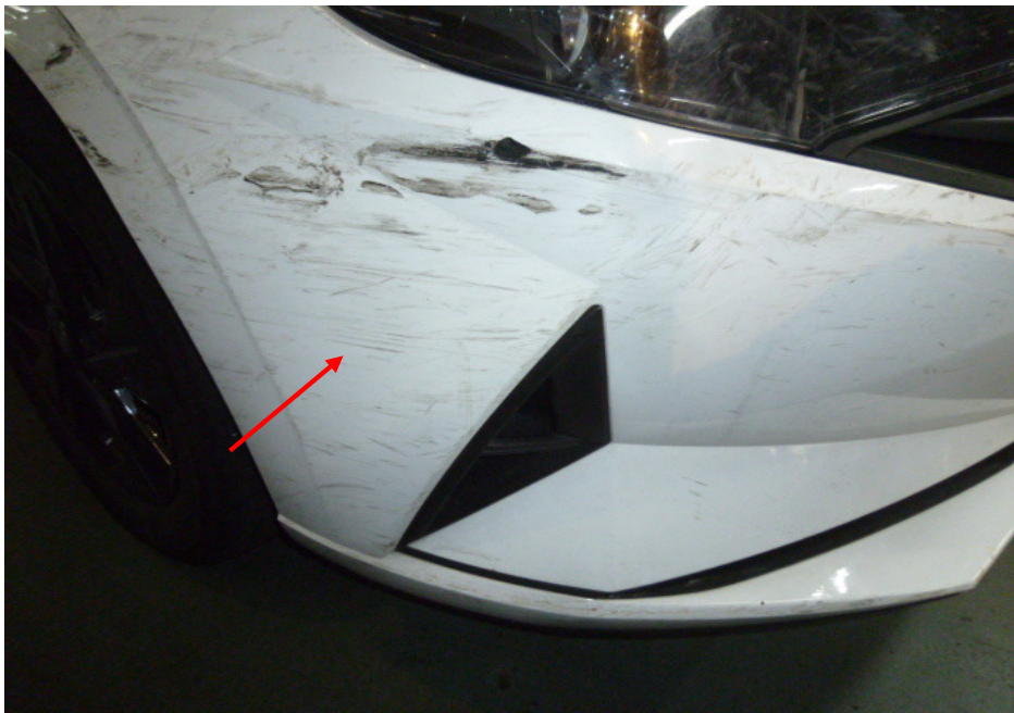
Photo 6 shows upon closer inspection, the graze marks and scuff marks sustained to the front bumper of the Insured Vehicle (arrowed) did not corroborate with Mr Kee's statement of a hit-and-run accident.
