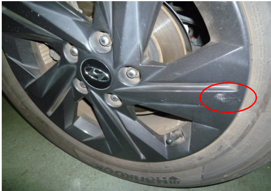
Photo 11 shows a closer view of the relatively minor marks of grazing nature observed around the right rear wheel rim (circled) of the Insured Vehicle during the physical inspection at Falcon.
