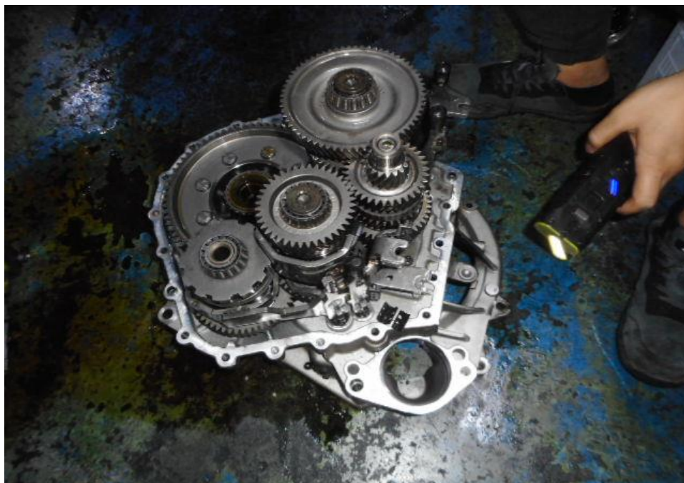
Photo 5 shows the general view of gearbox unit of the Insured Vehicle at the time of our inspection. The gearbox component in the gearbox unit is observed to be damaged and fallen out of place. These damaged components is likely the cause of the failure to the gearbox system.
