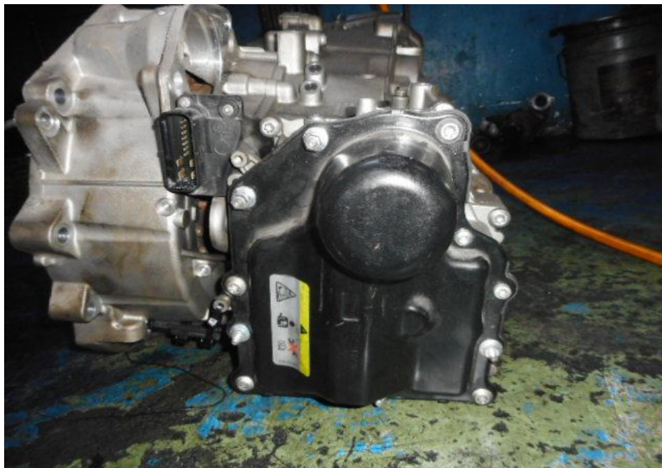
Photo 3 shows the general view of the gearbox and mechatronic unit portion of the Insured Vehicle at the time of our inspection. These undercarriage components is observed to be unaffected by any signs of accident.
