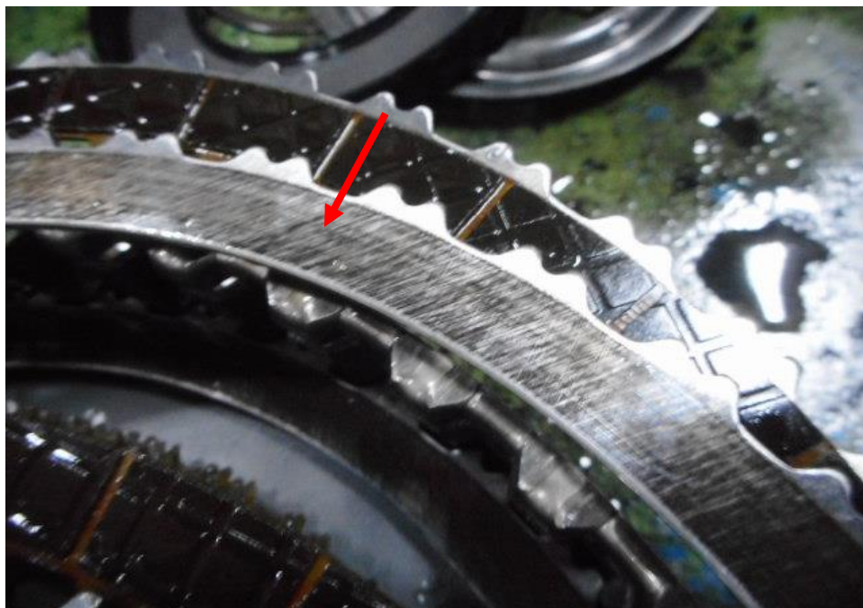
Photo 7 shows the close up view of inside the gearbox unit of the Insured Vehicle at the time of our inspection. The clutch pack (arrowed) component in the gearbox unit is observed to be damaged with scratches on the surface on the clutch packs linings, this is the cause for the complained problems of difficulty in changing gears and the sound coming for the gearbox of the Insured Vehicle.
