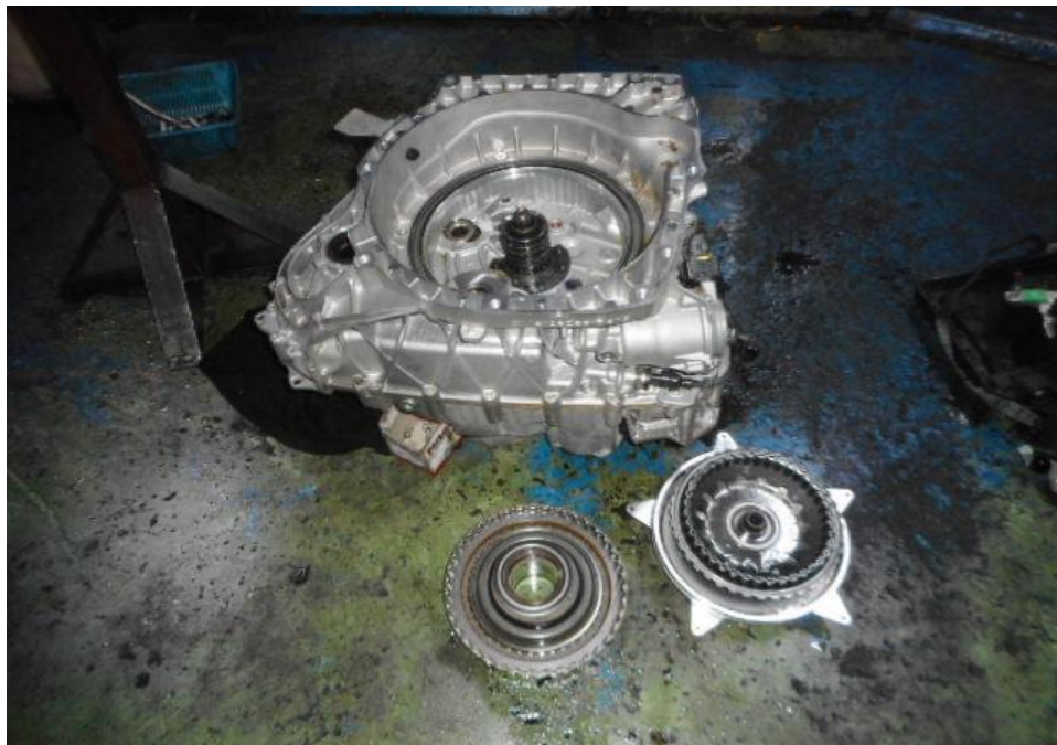
Photo 6 shows the general view of inside the gearbox unit of the Insured Vehicle at the time of our inspection. The components in the gearbox unit is observed to be unaffected and by any signs of accident.
