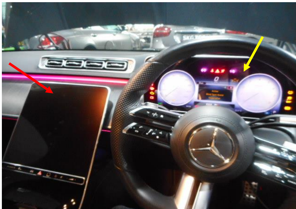
Photo 6 shows the close up view of the vehicle instrument portion of the Insured Vehicle at the time of our inspection. The infotainment instrument display (red arrowed) did not turn on even when the vehicle's engine is turned on as compared to the driver's display panel (yellow arrow).
