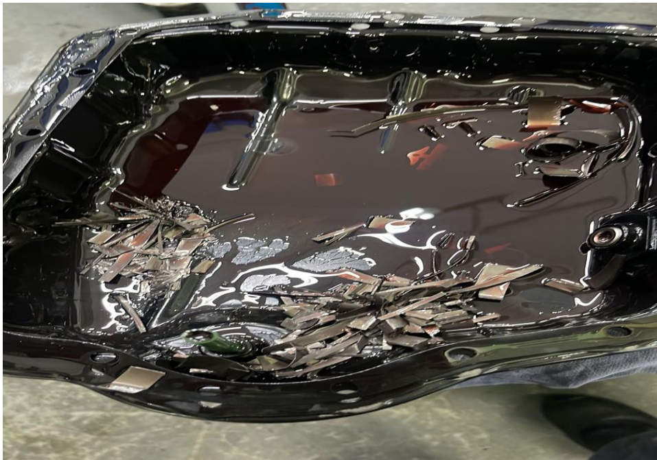
Photo 6 shows the close up view of the CVT transmission unit underside portion of the Insured Vehicle at the time of our inspection. We observed broken CVT transmission drive belt and transmission components that had fallen down to the oil sump.
