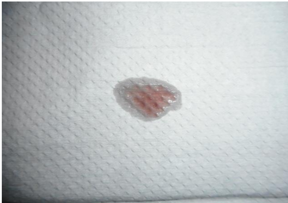
Photo 7 shows the close up view of the CVT transmission fluid of the Insured Vehicle at the time of our inspection. We observed that CVT transmission fluid was observed to be without any visible contamination.
