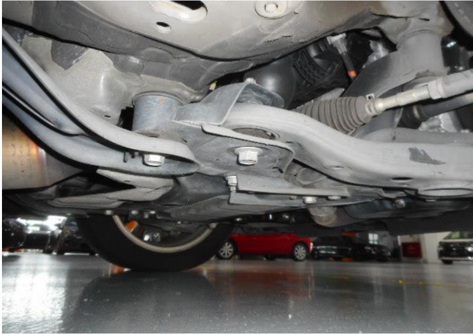
Photo 5 shows the general view of the engine and transmission underside portion of the Insured Vehicle at the time of our inspection. The engine and transmission underside compartment is observed to be unaffected and by any signs of accident.
