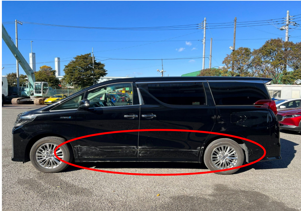
Photo 1 shows the left side body of the Motor Car (photograph provided to me). The Motor Car was observed to have sustained damage at its left side portion (circled). The front left fender, front left door, front left door lower moulding, rear left door, rear left door lower moulding, rear left fender and rear bumper were observed to be damaged. The airbag(s) of the Motor Car was not deployed.
