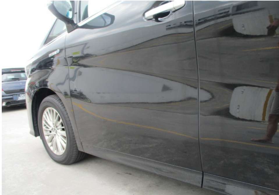
Photo 8 shows a closer view of the Motor Car's front left door, front left door lower moulding and front left fender. The body parts at the left side portion of the Motor Car were visually examined and it was observed that the repair/restoration works carried out to the damaged area of the Motor Car (refer to photograph 1 above) were reasonably adequate and in order.
