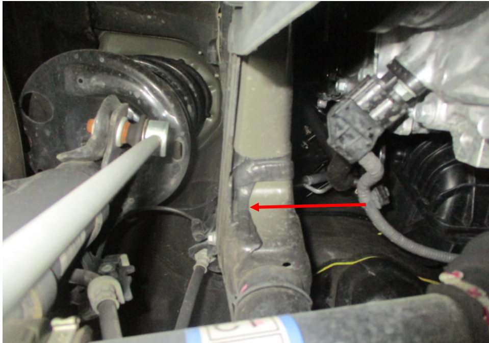
Photo 30 shows the chassis/structural body at the underside front right of the Motor Car. I did not find any weld marks other than original spot weld marks on the chassis/structural body of the Motor Car. The original factory sealant (arrowed) at the joints along the chassis/structural body was untouched, indicating no work was done on the chassis/structural body of the Motor Car and that the chassis/structural body was originally fitted.
