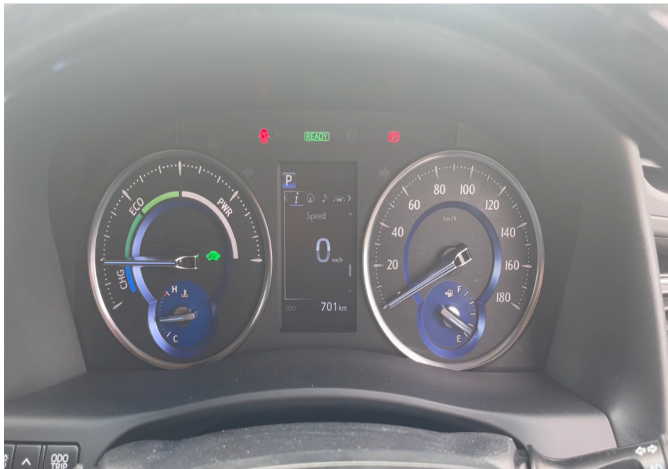
Photo 19 shows the respective warning lights no longer illuminated, indicating that there is no fault detected to the ABS, SRS, EPS, VSC and the various collision prevention systems of the Motor Car during the self-test. These electronic systems were hence in working condition at the time of my inspection.
