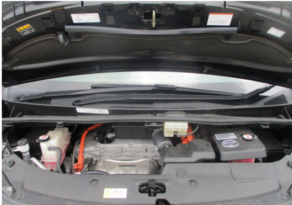
Photo 13 shows a general view of the engine compartment of the Motor Car at the time of my inspection. The various parts and components inside the engine compartment were all observed to be intact and properly fitted. There was no sign(s) or indication(s) of fluid leak and/or fluid stain found inside the engine compartment.
