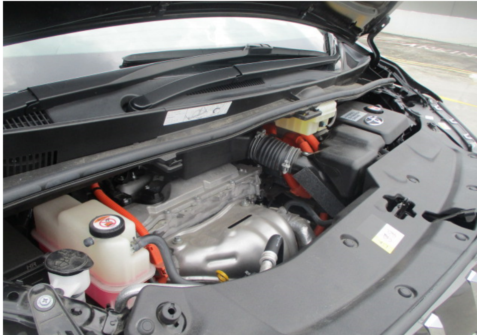
Photo 14 shows another view of the engine compartment of the Motor Car at the time of my inspection. The various parts and components inside the engine compartment were all observed to be intact and properly fitted. There was no sign(s) or indication(s) of fluid leak and/or fluid stain found inside the engine compartment.
