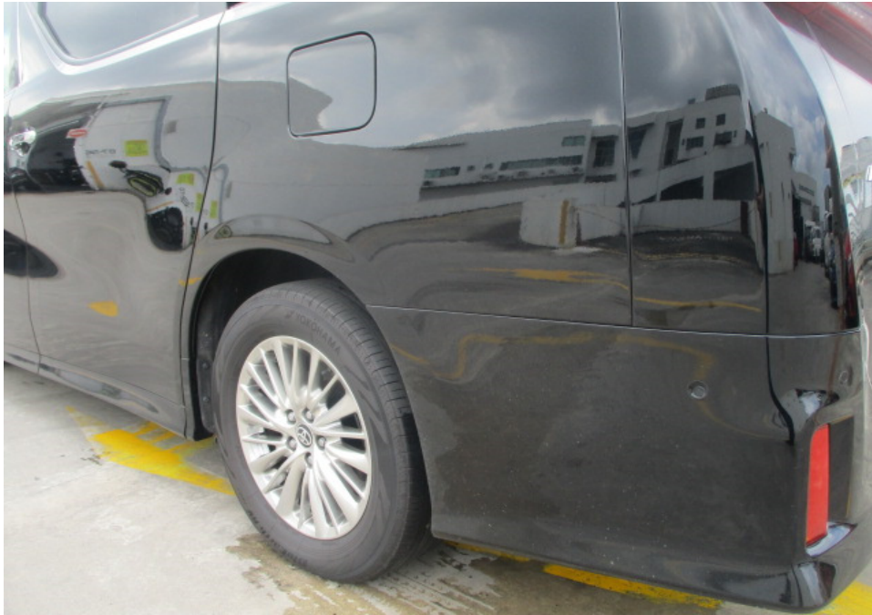
Photo 6 shows a closer view of the Motor Car's rear bumper, rear left wheel rim and rear left fender. The body parts at the left side portion of the Motor Car were visually examined and it was observed that the repair/restoration works carried out to the damaged area of the Motor Car (refer to photograph 1 above) were reasonably adequate and in order.
