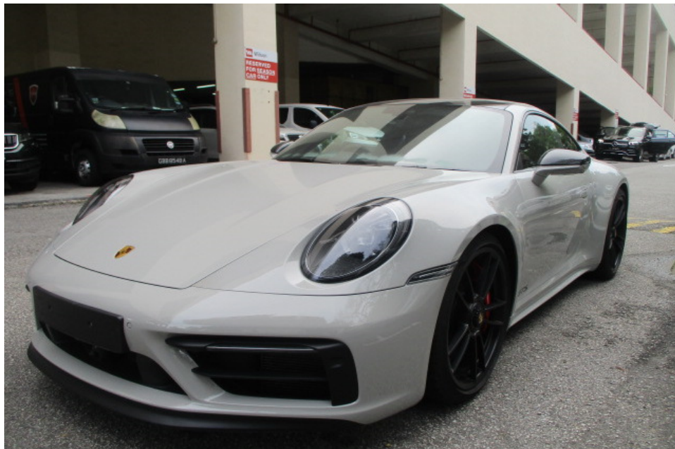
Photo 8 shows a general view of the front left body of the Motor Car at the time of my inspection. The Motor Car was observed to be in a relatively good general condition with no loose exterior fittings observed. The body parts at the frontal portion and left side front portion of the Motor Car were visually examined and it was observed that the repair/restoration works carried out to the damaged area of the Motor Car (refer to photograph 1 - 3 above) were reasonably adequate and in order.
