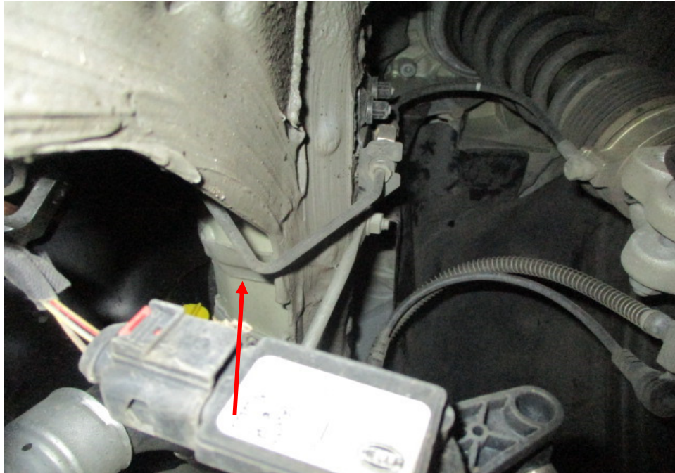
Photo 39 shows the chassis/structural body at the underside front right of the Motor Car. The original factory sealant (arrowed) at the joints along the chassis/structural body was observed to be untouched. In general, I had found no work was carried out on the chassis/structural body of the Motor Car. The chassis/structural body of the Motor Car was originally fitted.
