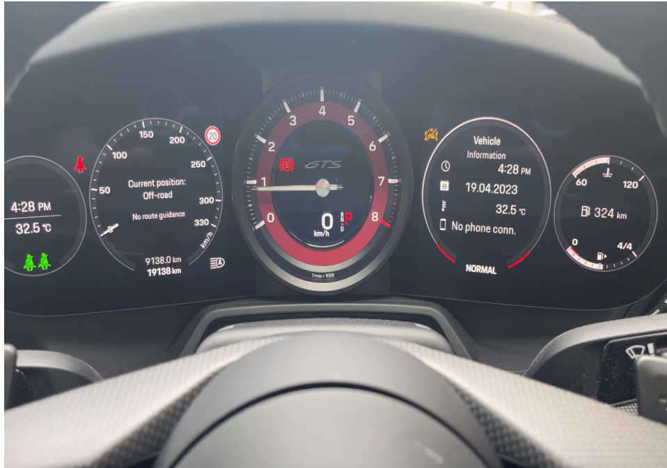
Photo 27 shows the respective warning lights no longer illuminated, indicating that there is no fault detected to the ABS, SRS, EPS, TPM and TCS systems of the Motor Car during the self-test. These electronic systems were hence in working condition at the time of my inspection.
