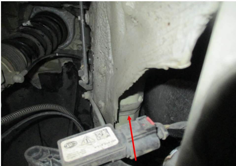
Photo 38 shows the chassis/structural body at the underside front left of the Motor Car. I did not find any weld marks other than original spot weld marks on the chassis/structural body of the Motor Car. The original factory sealant (arrowed) at the joints along the chassis/structural body was untouched, indicating no work was done on the chassis/structural body of the Motor Car and that the chassis/structural body was originally fitted.
