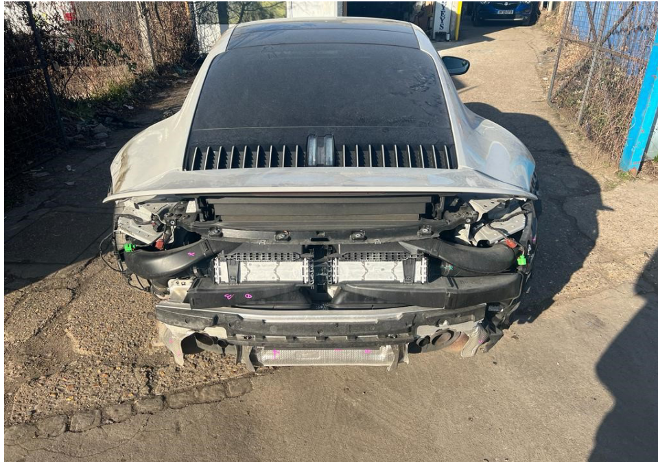
Photo 5 shows the rear body of the Motor Car (photograph provided to me). The Motor Car's rear left taillamp, rear right taillamp, rear centre lamp, rear bumper and all its related parts and attachments like the rear bumper lower cover, rear bumper left reflector, rear bumper right reflector, rear bumper sensors, rear bumper tow cover, rear left exhaust garnish and rear right exhaust garnish amongst others, were missing/dislodged/damaged.
