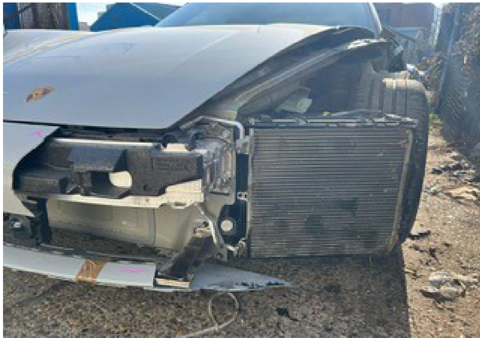
Photo 2 shows a closer view of the front left body of the Motor Car (photograph provided to me). The Motor Car's front left headlamp, front left fender, front left fender inner shield, front bumper lower lip, front bumper sensors, front bumper left lower grille, front bumper centre air guide, front left day light and front left signal lamp amongst others, were missing/dislodged/damaged.
