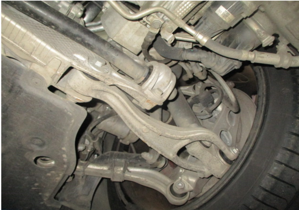
Photo 29 shows a general view of the control arms and linkages at the rear right wheel of the Motor Car. I did not observe any fluid leak and/or fluid stain on the underside of the Motor Car. All of the Motor Car's undercarriage components were observed to be intact and secured in an appropriate manner.
