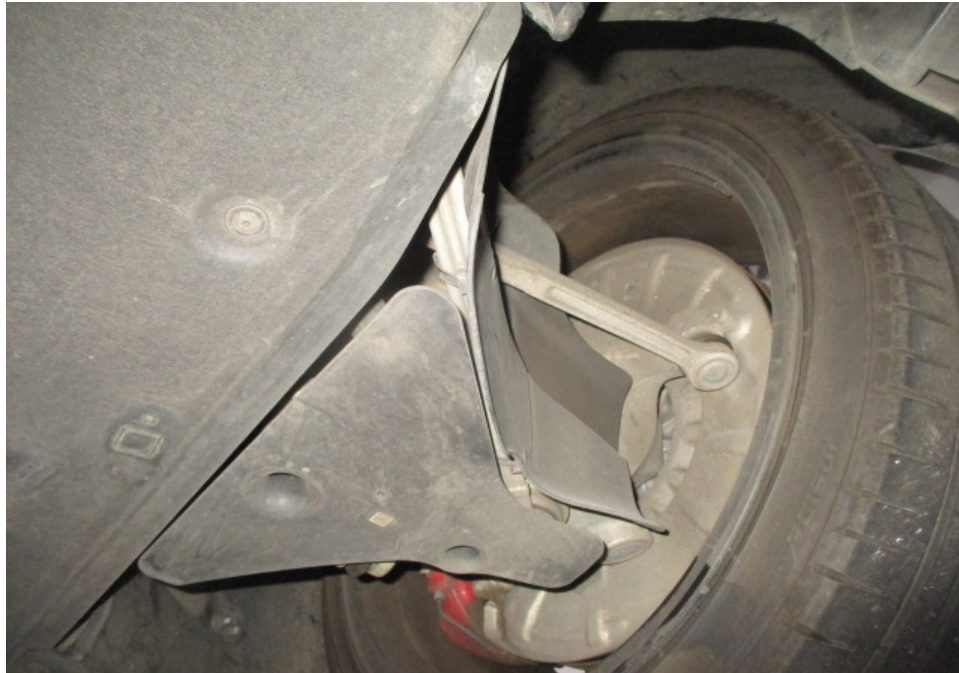
Photo 31 shows the various undercarriage components at the front left wheel of the Motor Car. The mechanical components, control arms and linkages were all found to be intact and secured in an appropriate manner.
