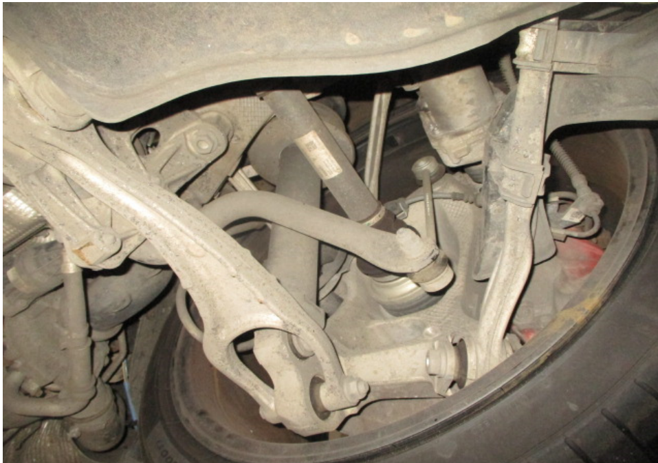
Photo 30 shows a general view of the control arms and linkages at the rear left wheel of the Motor Car. I did not observe any fluid leak and/or fluid stain on the underside of the Motor Car. All of the Motor Car's undercarriage components were observed to be intact and secured in an appropriate manner.
