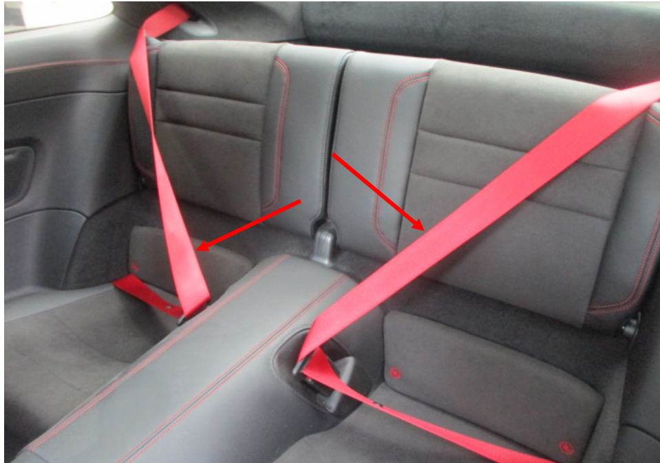
Photo 25 shows the rear seats of the Motor Car. All the seats of the Motor Car were secured via seat rails to the floorboard. They were also fitted with a retractable seat belt reel and a pre-tensioner. The seat belts (arrowed) were tested and were able to be fastened into the respective pre-tensions that were fitted on the side of each individual seat.
