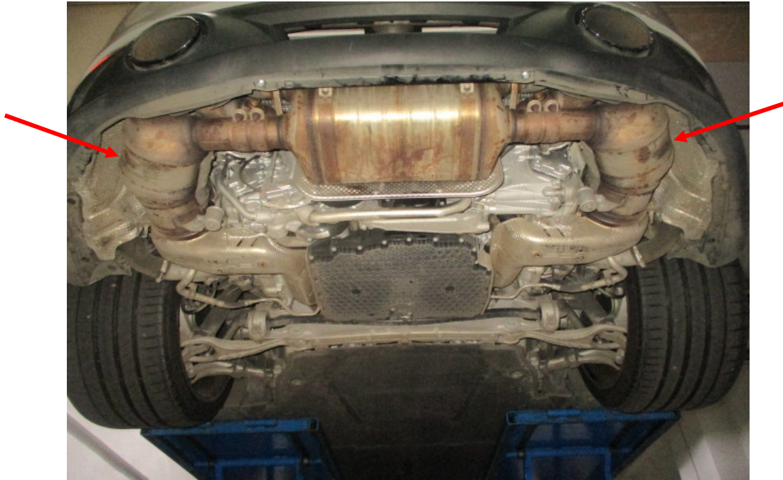
Photo 33 shows the Motor Car's exhaust system. My examination of the Motor Car's exhaust system revealed no sign(s) or indication(s) of any cut or weld marks along its exhaust pipes, on its catalytic converters (arrowed) and on its rear muffler.
