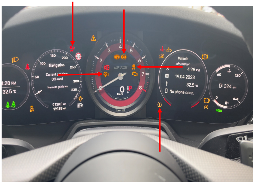
Photo 26 shows the warning lights for the various electronic safety features appearing on the instrument panel of the Motor Car during its self-test when the engine is cranked, in particular the ABS, SRS, EPS, TPM and TCS lights (arrowed).
