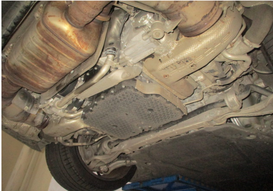
Photo 35 shows another view of the Motor Car's engine compartment. The engine compartment was at the rear underside of the Motor Car. The various parts and components within the engine compartment were all observed to be intact and properly fitted. There was also no sign(s) or indication(s) of fluid leak and/or fluid stain found inside the engine compartment.
