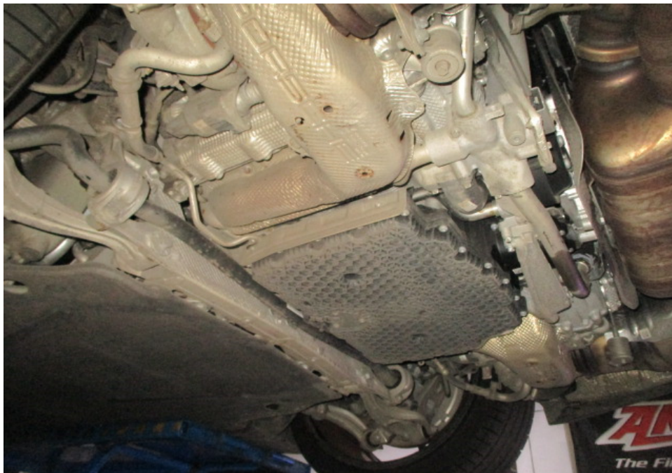
Photo 34 shows a general view of the Motor Car's engine compartment. The engine compartment was at the rear underside of the Motor Car. The various parts and components within the engine compartment were all observed to be intact and properly fitted. There was also no sign(s) or indication(s) of fluid leak and/or fluid stain found inside the engine compartment.
