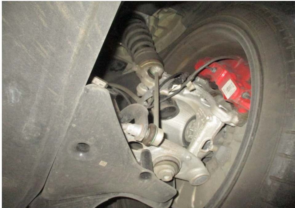
Photo 32 shows the various undercarriage components at the front right wheel of the Motor Car. The mechanical components, control arms and linkages were all found to be intact and secured in an appropriate manner. I also did not observe any fluid leak and/or fluid stain on the underside of the Motor Car.
