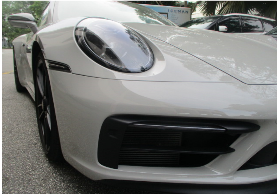
Photo 13 shows a closer view of the Motor Car's front bumper, front bumper right lower grille, front right day light, front right signal lamp and front right headlamp. The body parts at the frontal portion of the Motor Car were visually examined and it was observed that the repair/restoration works carried out to the damaged area of the Motor Car (refer to photograph 3 above) were reasonably adequate and in order.
