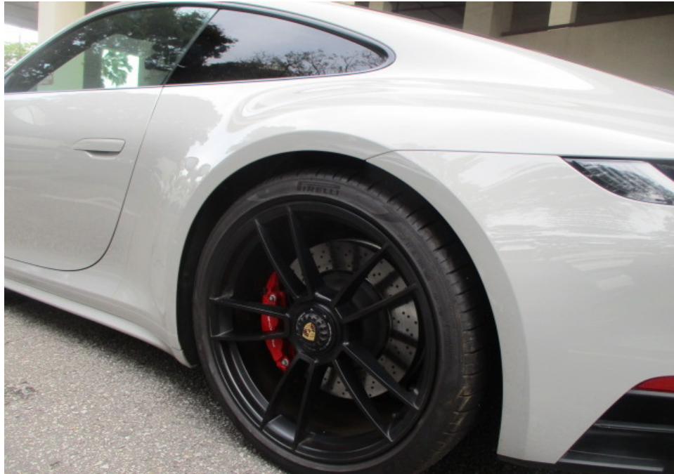
Photo 17 shows a closer view of the Motor Car's rear bumper, rear left wheel rim and rear left body panel. The body parts at the left rear portion of the Motor Car were visually examined and it was observed that the repair/restoration works carried out to the damaged area of the Motor Car (refer to photograph 1 & 4 above) were reasonably adequate and in order.
