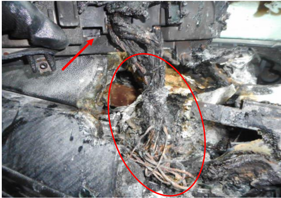
Photo 11 shows a close up view of the aftermarket infotainment unit and display panel (arrowed) and its wiring harness connected to the battery (circled) as there was greenish residue on the surface. The presence of greenish residue indicates internal heating of copper wires, a sign of an electrical short circuit occurring. The greenish residue is normally left behind from oxidation as a result of chemical reaction involving the copper wires. The fire damage had also melted the electrical components that it was connected to. These wirings and aftermarket infotainment unit and display panel components are not original wirings fitted from manufacturer and are additionally fitted.
