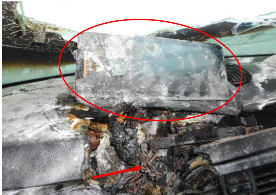
Photo 8 shows the interior dashboard of the Insured Vehicle an aftermarket infotainment unit and display panel (circled) and its wirings (arrowed) on the Insured Vehicle, which was observed to be affected by the fire.
