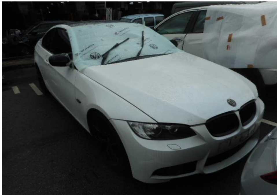
Photo 1 shows the general view of the front portion of the Insured Vehicle at the time of our inspection. The fire damage to the Insured Vehicle was confined to its interior portion. Its exterior is observed to be unaffected by the fire.
