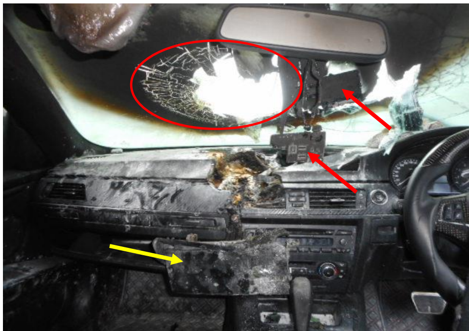
Photo 7 shows the close up view of the interior compartment of the Insured Vehicle at the time of our inspection. The front dash camera (red arrow), front windscreen (circled) and its infotainment unit and display panel (yellow arrow) had suffered heat and smoke damages as a result of the fire.
