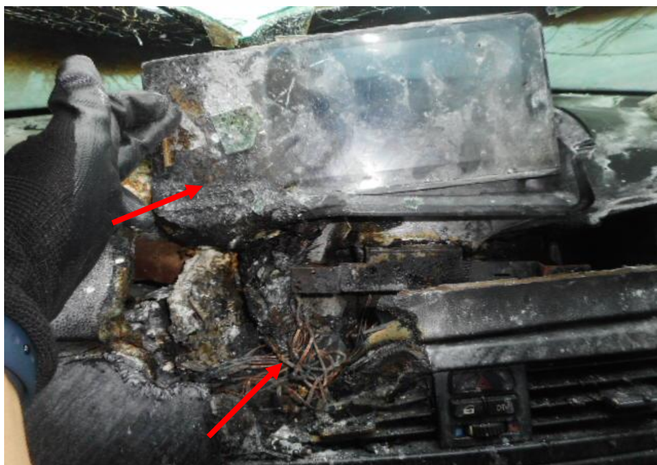
Photo 10 shows the general view of the wirings in the front centre dashboard of the Insured Vehicle at the time of our inspection. Observed where the fire had likely started from the wirings of the aftermarket infotainment unit and display panel and its wirings connecting to the battery of the Insured Vehicle (arrowed) as there was greenish residue on the surface. The presence of greenish residue indicates internal heating of copper wires, a sign of an electrical short circuit occurring. The greenish residue is normally left behind from oxidation as a result of chemical reaction involving the copper wires. The fire damage had also melted the electrical components that it was connected to. These wirings and aftermarket infotainment unit and display panel components are not original wirings fitted from manufacturer and are additionally fitted.
