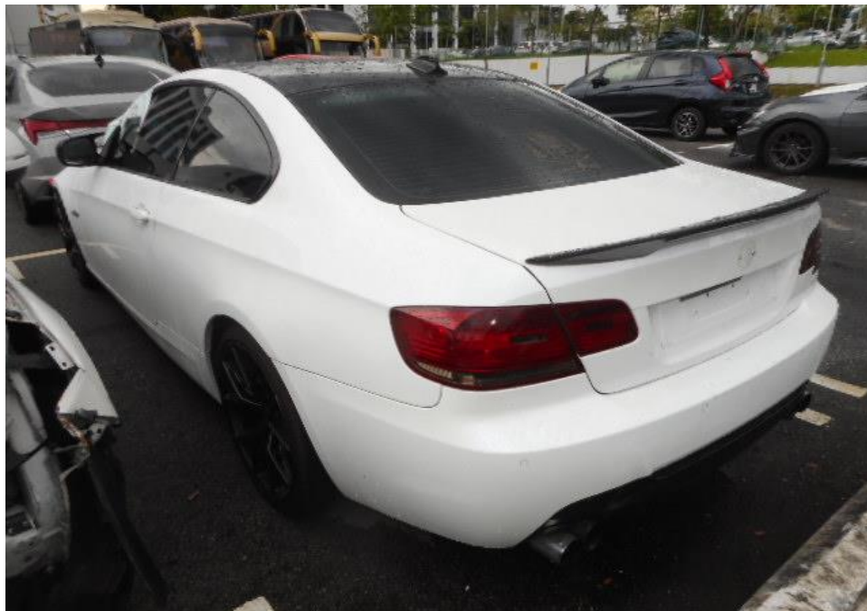
Photo 3 shows the general view of the left portion of the Insured Vehicle at the time of our inspection. The fire damage to the Insured Vehicle was confined to its interior portion. Its exterior is observed to be unaffected by the fire.
