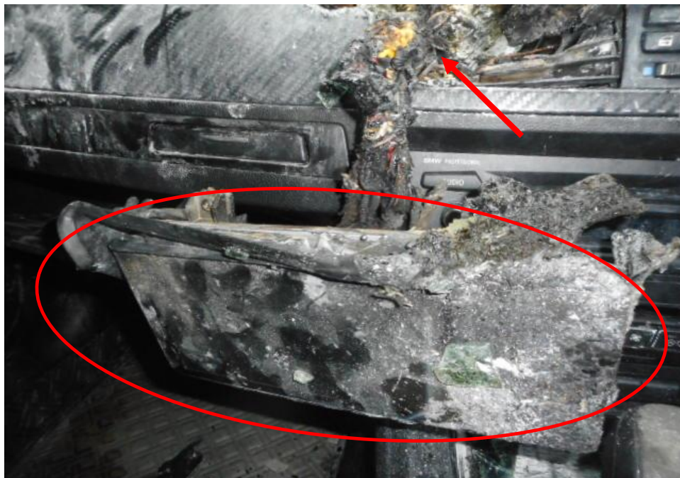
Photo 9 shows the interior dashboard of the Insured Vehicle an aftermarket infotainment unit and display panel (circled) and its wirings (arrowed) on the Insured Vehicle, which was observed to be affected by the fire.
