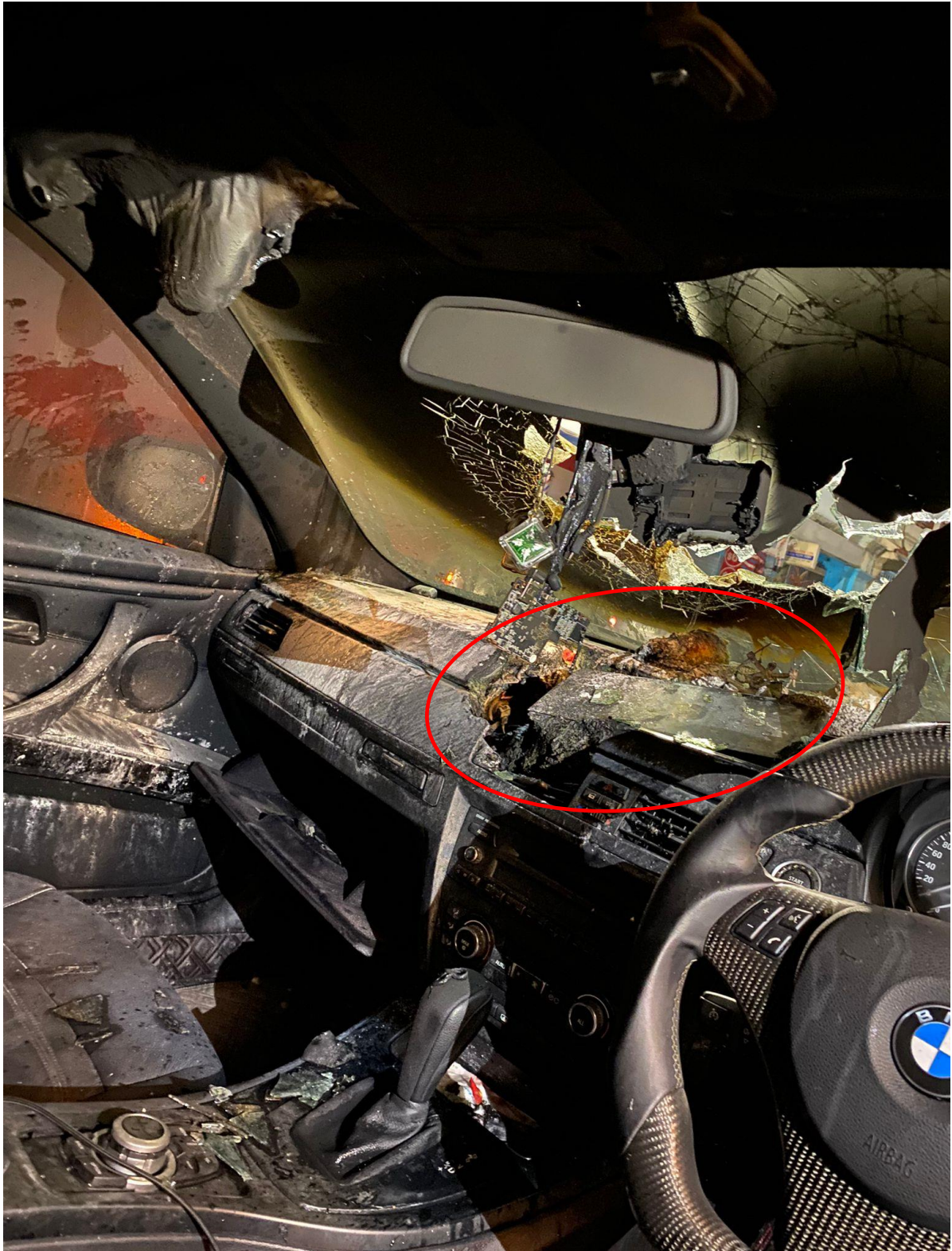
Photo 16 shows the interior front centre dashboard portion (circled) that was damaged on the Insured Vehicle at a result of the fire. In general, the information that could be gathered from this photograph had corresponded to the events that were related to us by Mr Lim, location when the fire broke out.
