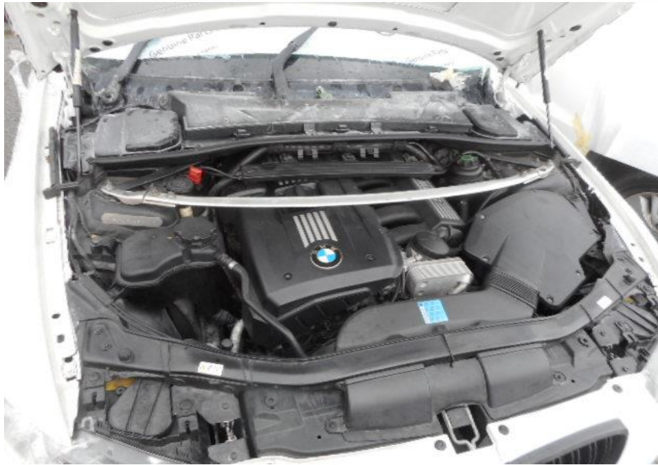
Photo 5 shows the general view of the engine portion of the Insured Vehicle at the time of our inspection. The fire damage to the Insured Vehicle was confined to its interior portion. Its engine compartment is observed to be unaffected by the fire.
