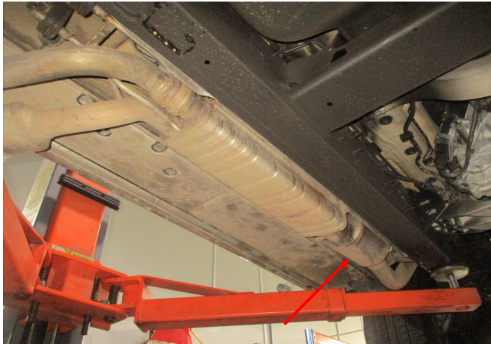
Photo 27 shows a general view of the Motor Car's left exhaust system. My examination of the Motor Car's left exhaust system revealed no sign(s) or indication(s) of any cut or weld marks along its exhaust pipe, on its catalytic converter, on its centre resonator box (arrowed) and on its rear muffler.
