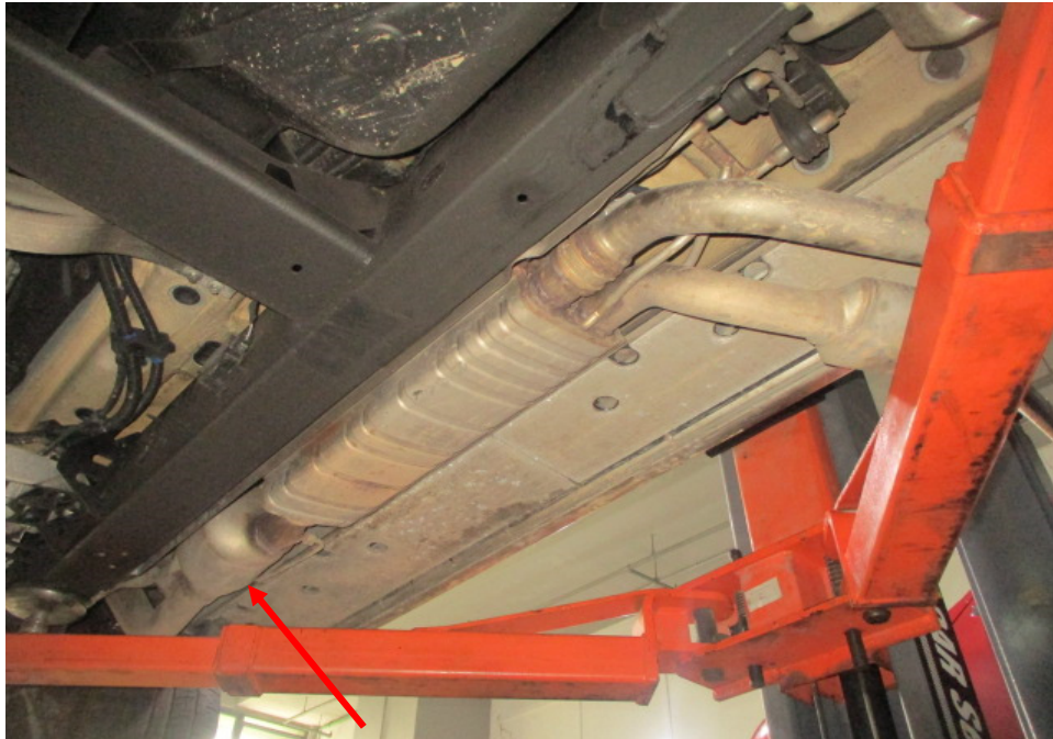
Photo 28 shows a general view of the Motor Car's right exhaust system. My examination of the Motor Car's left exhaust system revealed no sign(s) or indication(s) of any cut or weld marks along its exhaust pipe, on its catalytic converter, on its centre resonator box (arrowed) and on its rear muffler.
