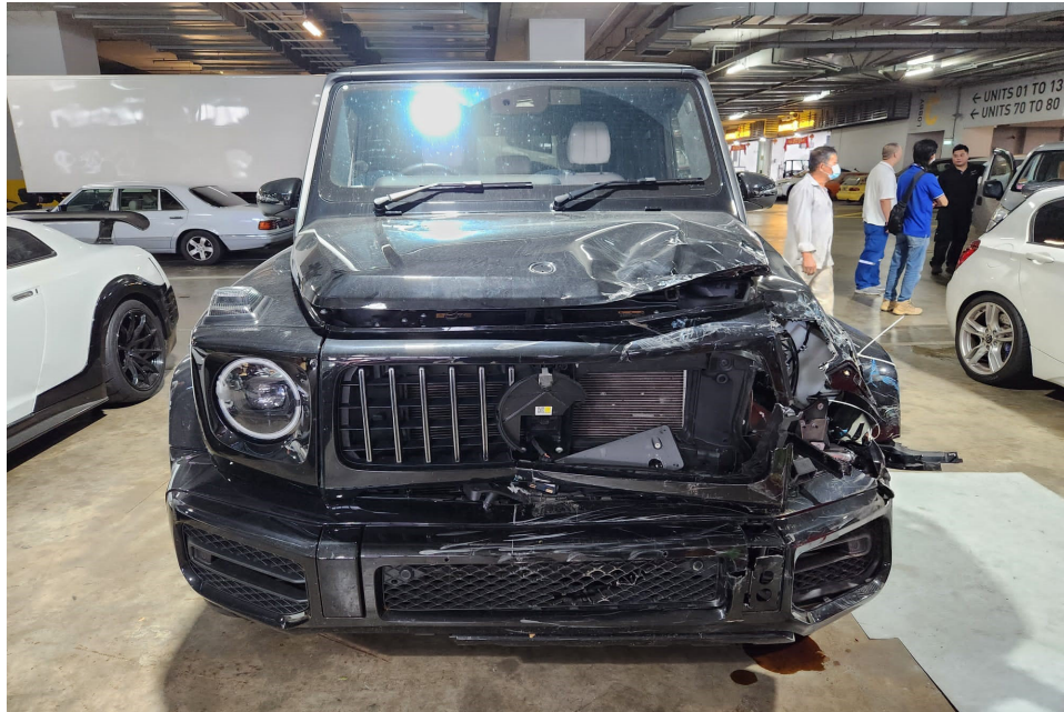
Photo 1 shows the frontal body of the Motor Car (photograph provided to me). The Motor Car was observed to have sustained damage at its front left portion. The front bumper, front bumper centre lower grille, front bumper left lower grille, front bumper sensors, radiator grille, front emblem, front number plate garnish, front bonnet, front support panel, air con condenser and radiator were amongst the body parts that were observed to have been damaged.
