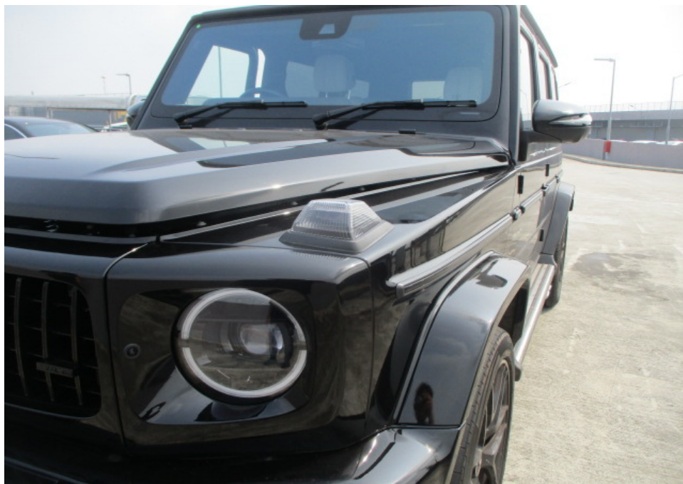
Photo 9 shows a closer view of the Motor Car's front bonnet, front left fender, front left fender wheel arc, front left signal lamp, front left headlamp and front left headlamp outer cover. The body parts at the front left portion of the Motor Car were visually examined and it was observed that the repair/restoration works carried out to the damaged area of the Motor Car (refer to photograph 1, 2 and 6 above) were reasonably adequate and in order.
