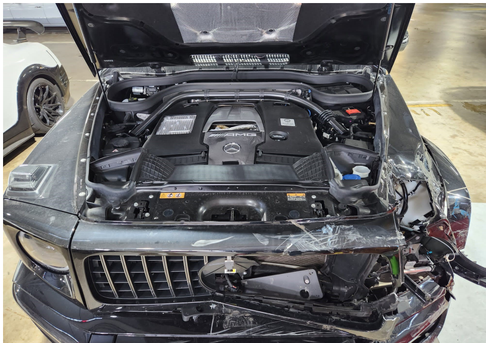
Photo 6 shows the engine compartment of the Motor Car (photograph provided to me). The Motor Car's front bumper, radiator grille, front emblem, front support panel, air con condenser and radiator were amongst the body parts that were observed to have been damaged. The various parts and components within the engine compartment were intact and unaffected.
