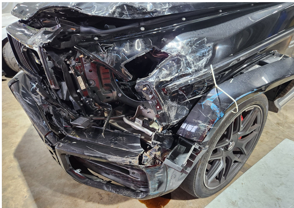
Photo 2 shows another view of the damage at the front left portion of the Motor Car (photograph provided to me). The front bumper, front bumper left bracket, front bumper sensors, front bonnet, front left signal lamp, front left headlamp, front left headlamp bracket, front left headlamp outer cover, front left fender, front left fender wheel arc and front left oil cooler were amongst the body parts that were observed to have been damaged.
