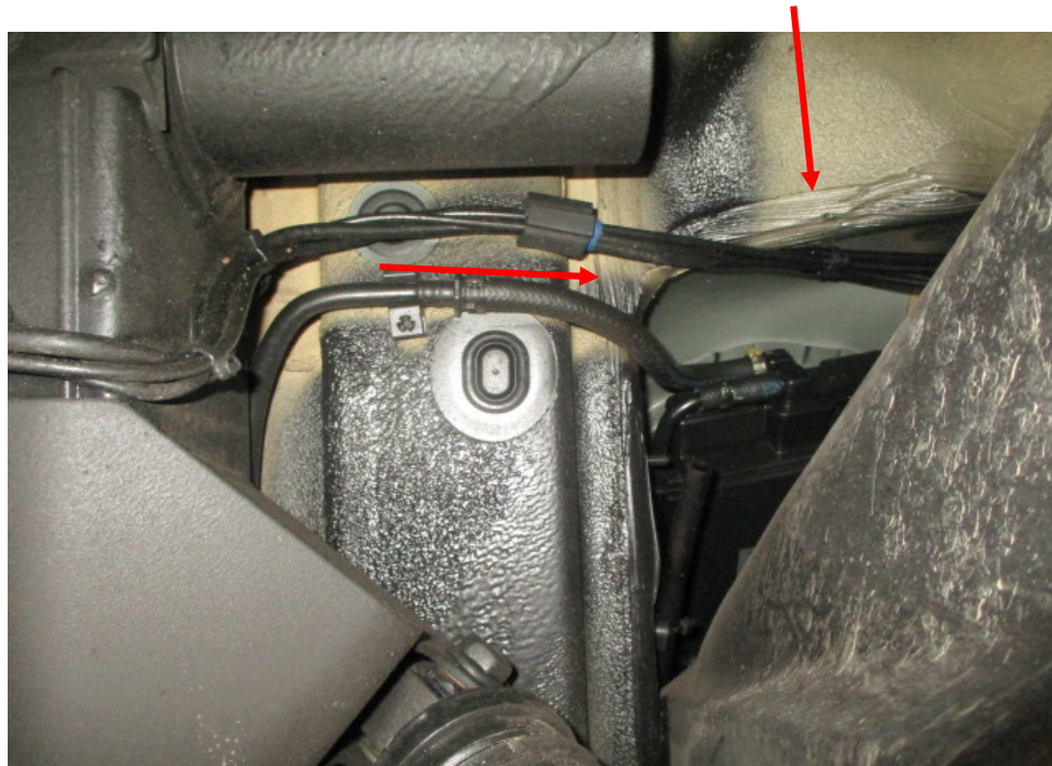
Photo 29 shows the chassis/structural body at the underside rear right of the Motor Car. I did not find any weld marks other than original spot weld marks on the chassis/structural body of the Motor Car. The original factory sealant (arrowed) at the joints along the chassis/structural body was untouched, indicating no work was done on the chassis/structural body of the Motor Car and that the chassis/structural body was originally fitted.
