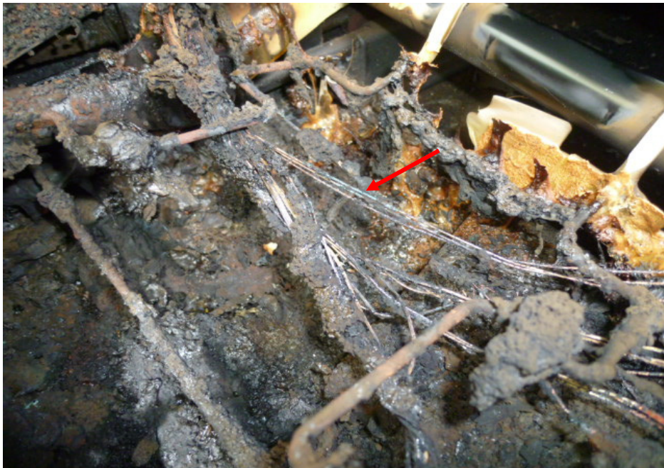
Photo 11 shows a closer view of some of the wirings with greenish residue (arrowed). The presence of such greenish residue suggest occurrence of an electrical short circuit.
