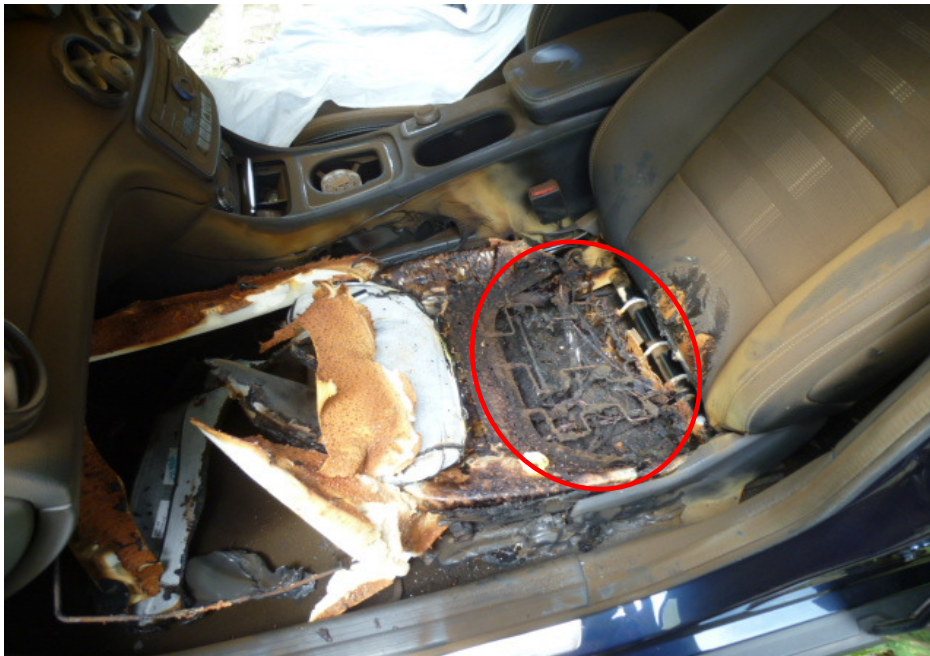
Photo 9 shows the front left passenger seat with its cushion removed. Upon closer examination, the fire appears to have started from one of the motors located at the centre portion of the front left passenger seat (circled).
