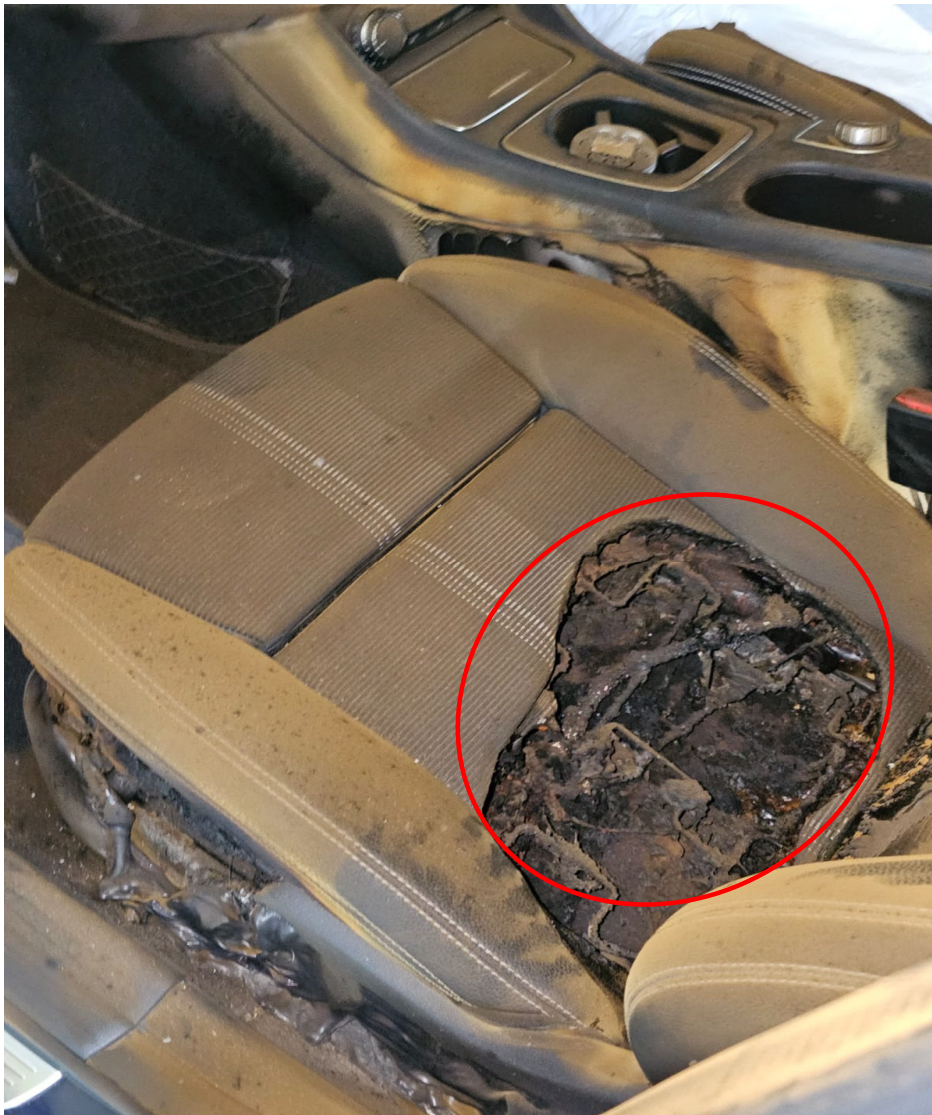
Photo 13 shows a close up view of the front left passenger seat of the Insured Vehicle post- incident. In general, the information that could be gathered from this photograph had corresponded to the events that were related to us by Mr Cheng, which is the fire had started from the front left passenger seat of the Insured Vehicle (circled).
