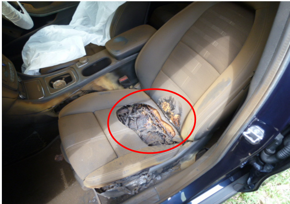
Photo 8 shows the front left passenger seat of the Insured Vehicle. The fire appears to have originated from the centre portion of the front left passenger seat of the Insured Vehicle. This can be observed from the burnt components of the front left passenger seat (circled).
