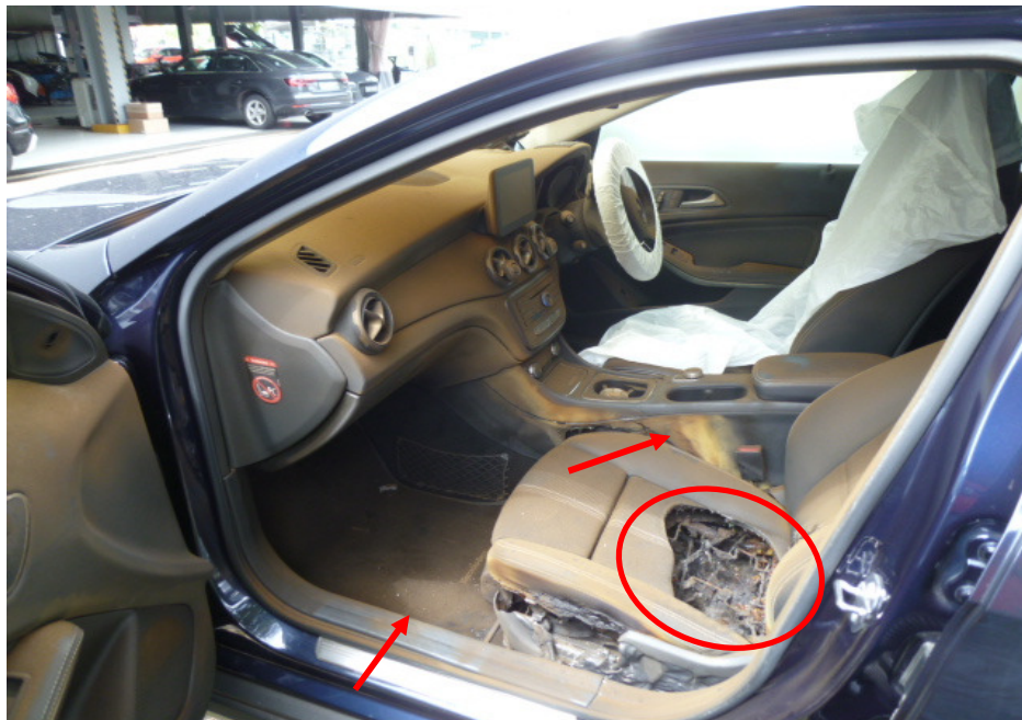
Photo 6 shows the interior compartment of the Insured Vehicle at the time of our inspection. The fire had resulted in several components in the interior compartment to be slightly burnt and/or damaged. This had included its front left passenger seat (circled), floor carpet, insulating material covering the floor panel (red arrows) amongst others.
