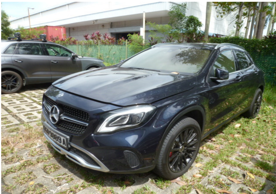
Photo 3 shows the general view of the left frontal portion of the Insured Vehicle at the time of our inspection. The fire damage was confined to its interior compartment. The exterior portion of the Insured Vehicle was observed to be relatively unaffected by the fire with the exception of the front windscreen and left front passenger door window.
