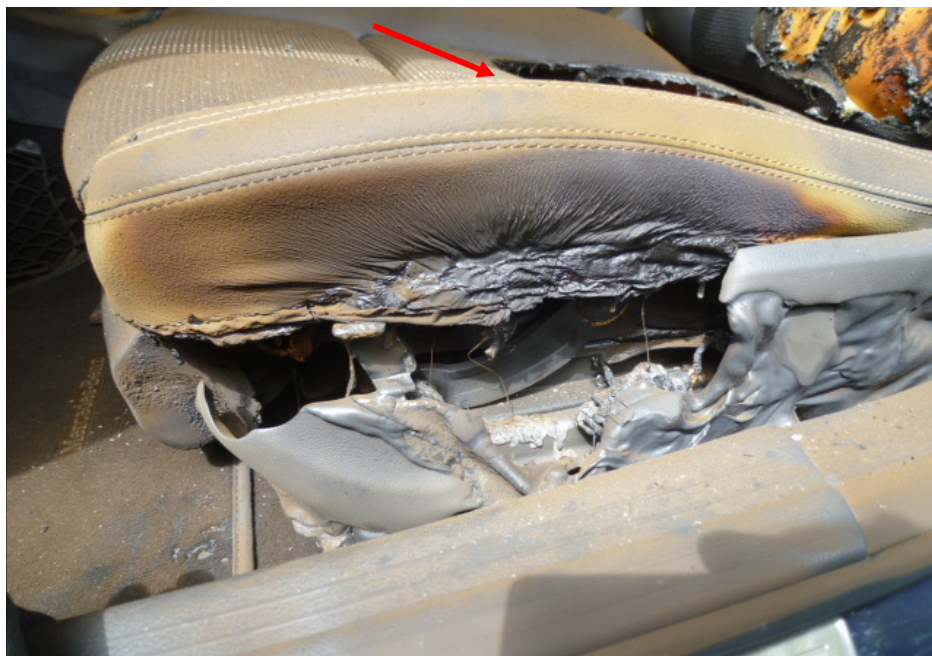
Photo 7 shows the front left passenger seat of the Insured Vehicle at the time of our inspection. The fire damage was confined to its front left passenger side. The front left passenger seat was observed to be partially burnt and/or melted (arrowed).
