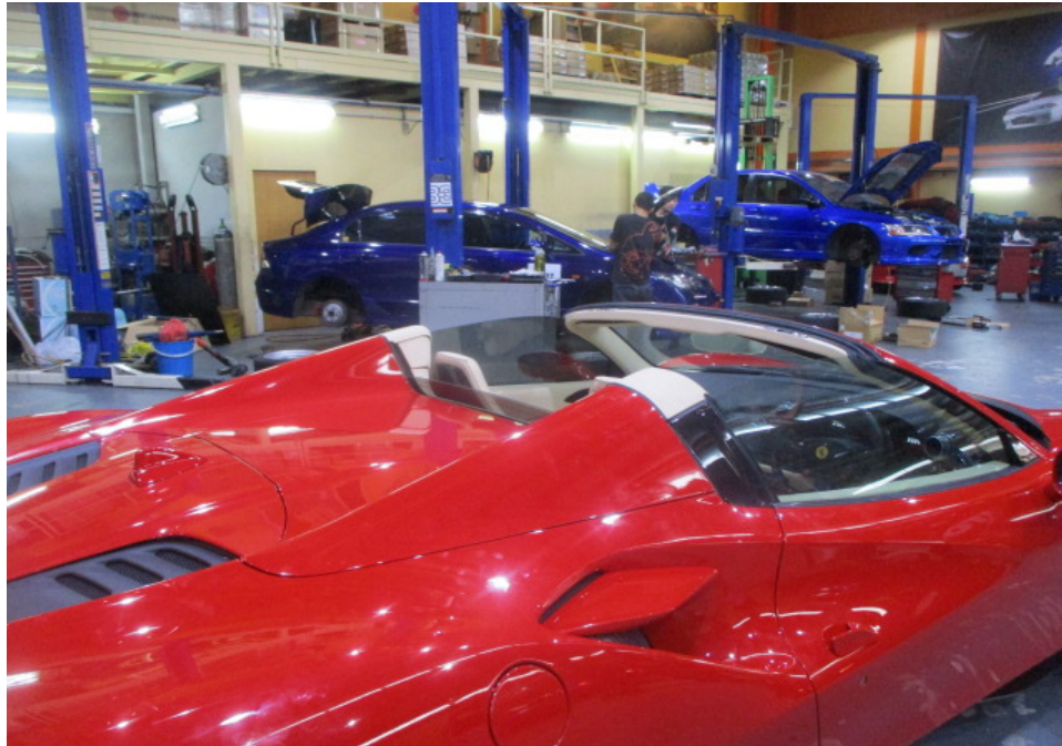
Photo 19 shows the Motor Car with its hard top roof completely folded. It was observed that as a safety feature, the hard top roof could only open and close when the Motor Car was in a stationary position or at low travelling speed. When opened, the hard top roof is completely folded into the rear compartment with no parts protruding out of the Motor Car's body. The hard top roof was also found adequately secured to the "A" pillar after closing.
