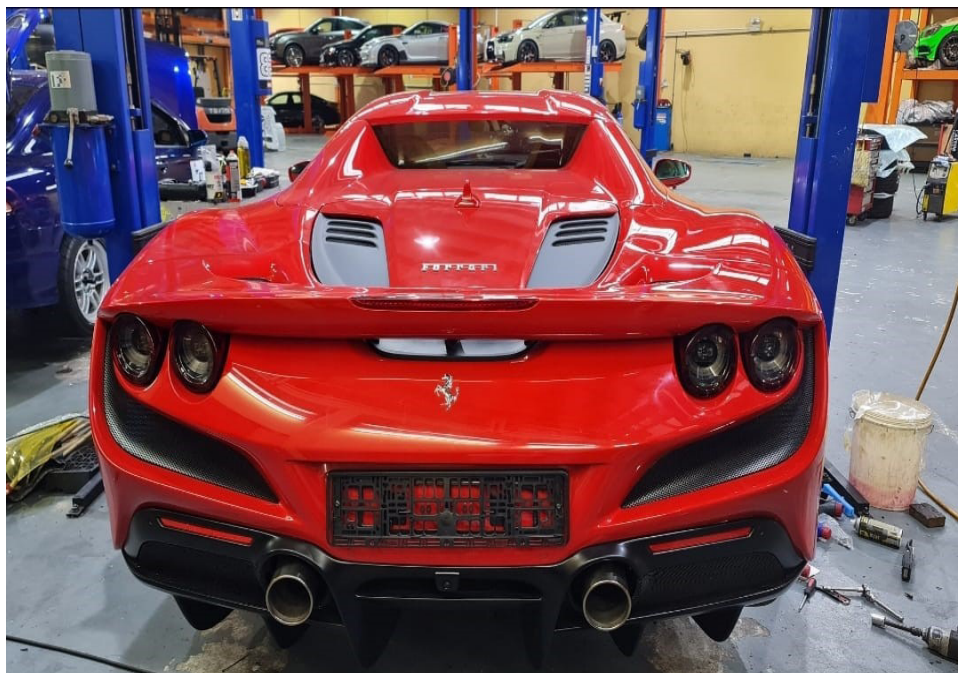
Photo 10 shows a general view of the rear body of the Motor Car with its rear bumper lower diffuser re-fitted. The Motor Car was observed to be in a relatively good general condition with no loose exterior fittings observed.
