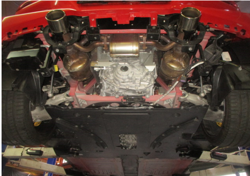
Photo 27 shows the Motor Car's exhaust system after removal of the rear bumper diffuser. In general, my examination of the Motor Car's exhaust system revealed no sign(s) or indication(s) of any cut or weld marks along its exhaust pipes, on its catalytic converters and on its rear mufflers.
