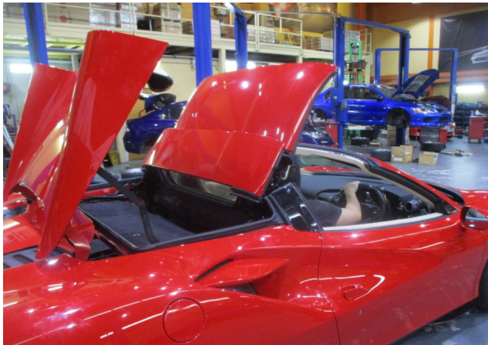
Photo 18 shows the Motor Car's hard top roof being tested. It was observed that as a safety feature, the hard top roof could only open and close when the Motor Car was in a stationary position or at low travelling speed. When opened, the hard top roof is completely folded into the rear compartment with no parts protruding out of the Motor Car's body. The hard top roof was also found adequately secured to the "A" pillar after closing.
