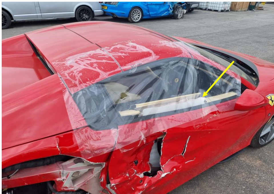
Photo 2 shows a closer view of the damage at the right side portion of the Motor Car (photograph provided to me). The front right door, front right door outer handle, front right door lock, front right door inner trimboard and right side rear body panel were amongst the body parts that were observed to have been damaged. The front right door airbag (arrowed) was activated.
