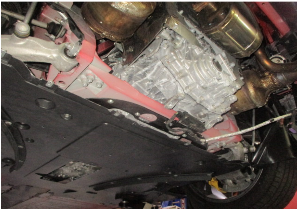
Photo 28 shows the Motor Car's engine compartment as viewed from the rear underside of the Motor Car. The various parts and components inside the engine compartment were all observed to be intact and properly fitted. There was also no sign(s) or indication(s) of fluid leak and/or fluid stain found inside the engine compartment.
