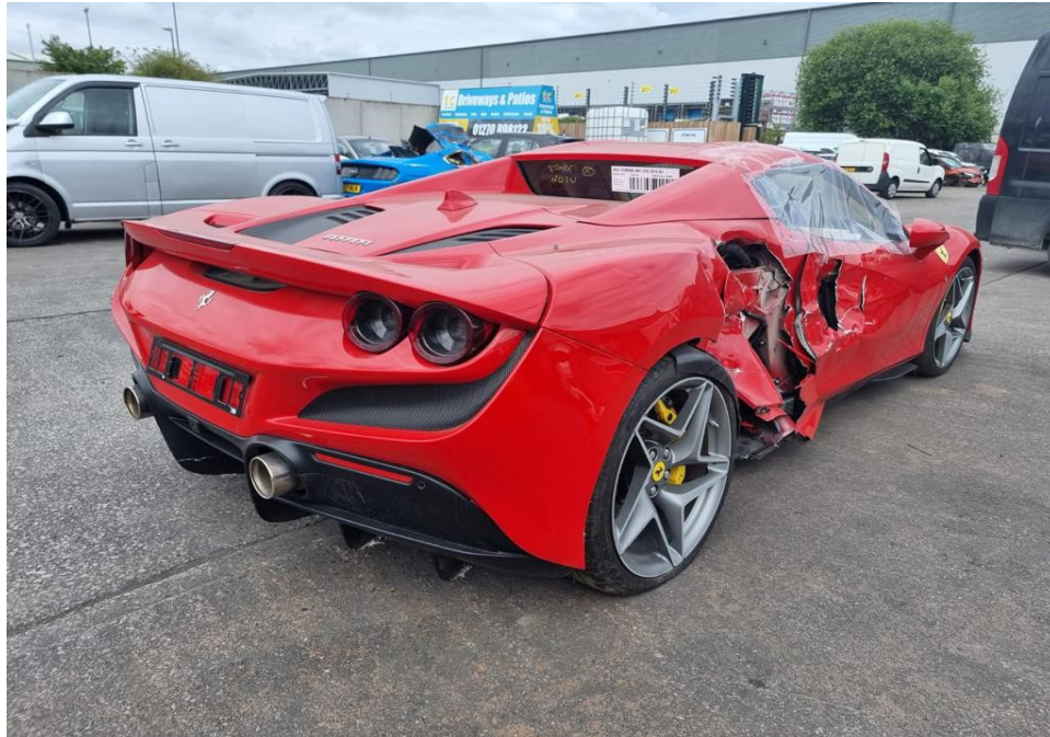
Photo 1 shows the rear right body of the Motor Car (photograph provided to me). The photographs provided to me had showed damage to the right side portion of the Motor Car. The front right door, front right door outer handle, front right door lock, right side rear body panel, rear right tyre and right side rocker panel garnish were amongst the body parts that were observed to have been damaged.
