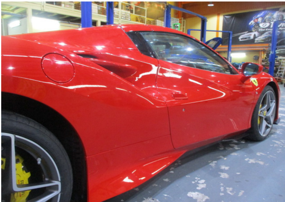
Photo 8 shows a closer view of the Motor Car's right side rear body panel, fuel filler cover, front right door, front right door outer handle and right side rocker panel garnish. The body parts at the right side portion of the Motor Car were visually examined and it was observed that the repair/restoration works carried out to the damaged area of the Motor Car (refer to photograph 1 & 2 above) were reasonably adequate and in order.
