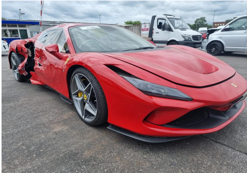
Photo 3 shows the front right body of the Motor Car (photograph provided to me). Apart for the right side portion, there was no physical damage observed to other areas of the Motor Car.
