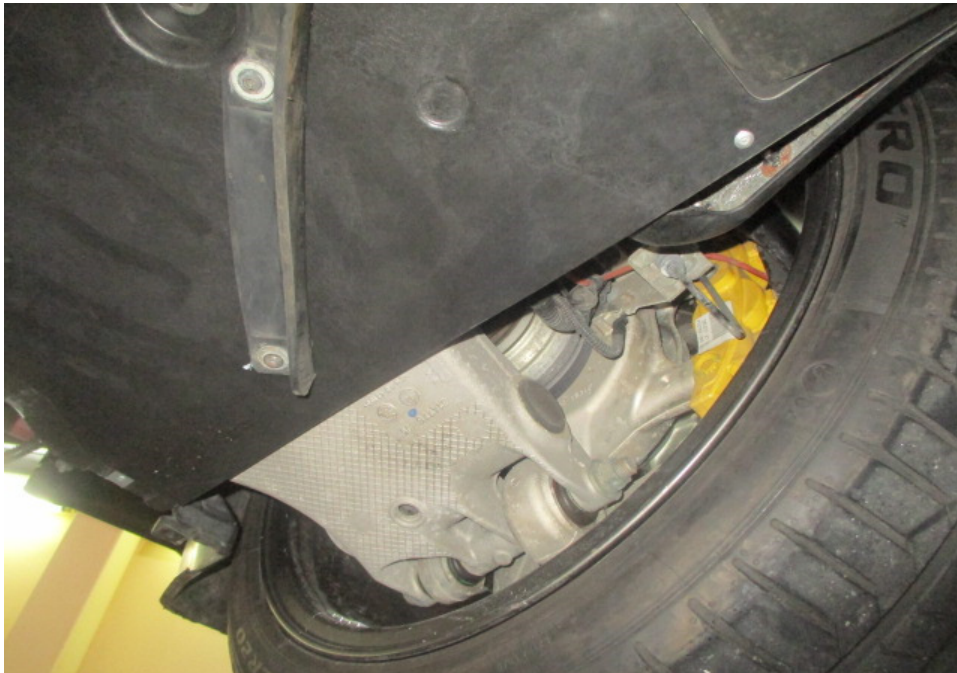
Photo 24 shows a general view of the control arms and linkages at the rear left wheel of the Motor Car. I did not observe any fluid leak and/or fluid stain on the underside of the Motor Car. All of the Motor Car's undercarriage components were observed to be intact and secured in an appropriate manner.
