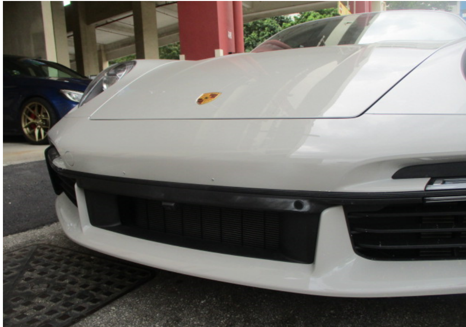
Photo 9 shows a closer view of the Motor Car's front bumper, front bumper sensors, front bumper centre lower air guide and front bonnet. The body parts at the frontal portion of the Motor Car were visually examined and it was observed that the repair/restoration works carried out to the damaged area of the Motor Car (refer to photograph 1 & 2 above) were reasonably adequate and in order.
