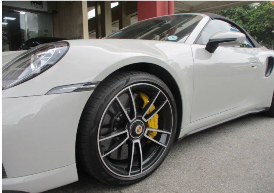
Photo 7 shows a closer view of the Motor Car's front left headlamp, front left signal lamp, front left fender and front left wheel rim. The body parts at the frontal portion of the Motor Car were visually examined and it was observed that the repair/restoration works carried out to the damaged area of the Motor Car (refer to photograph 1 & 2 above) were reasonably adequate and in order.
