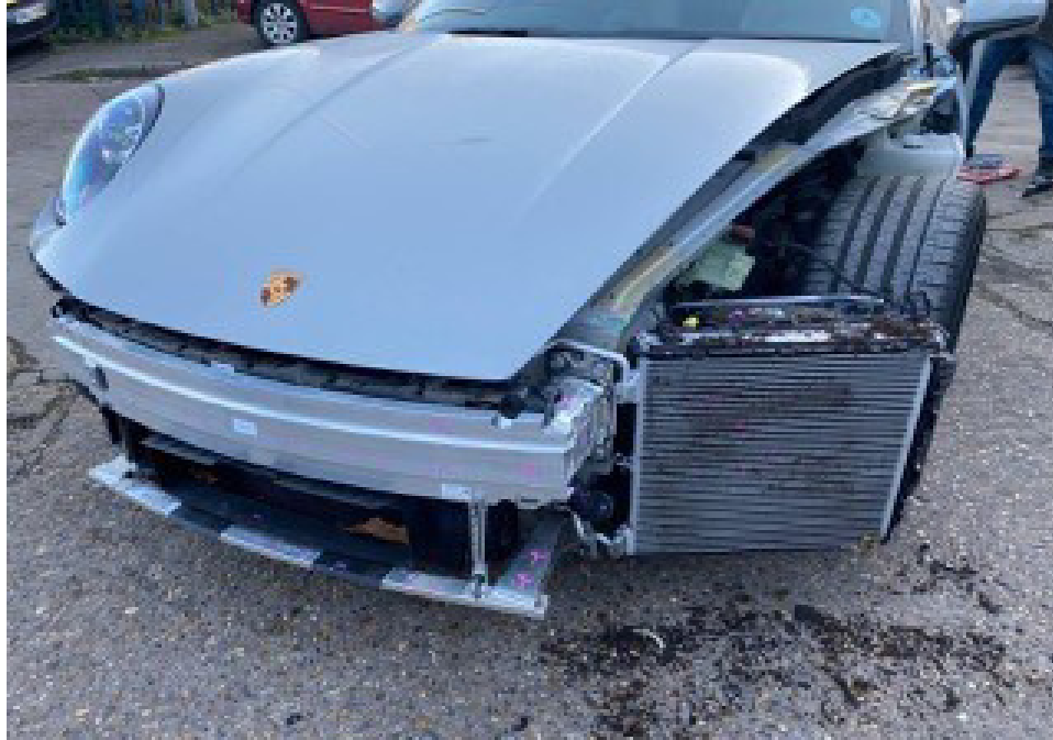
Photo 1 shows the front left body of the Motor Car (photograph provided to me). The front left fender, front left fender inner shield, front left headlamp, front bumper and all its related parts and attachments like the front bumper lower lip, front bumper sensors, front bumper tow cover, front bumper centre lower air guide, front bumper left lower grille, front bumper right lower grille, front left day light, front right day light, front left signal lamp and front right signal lamp amongst others were observed to be missing/dislodged/damaged.
