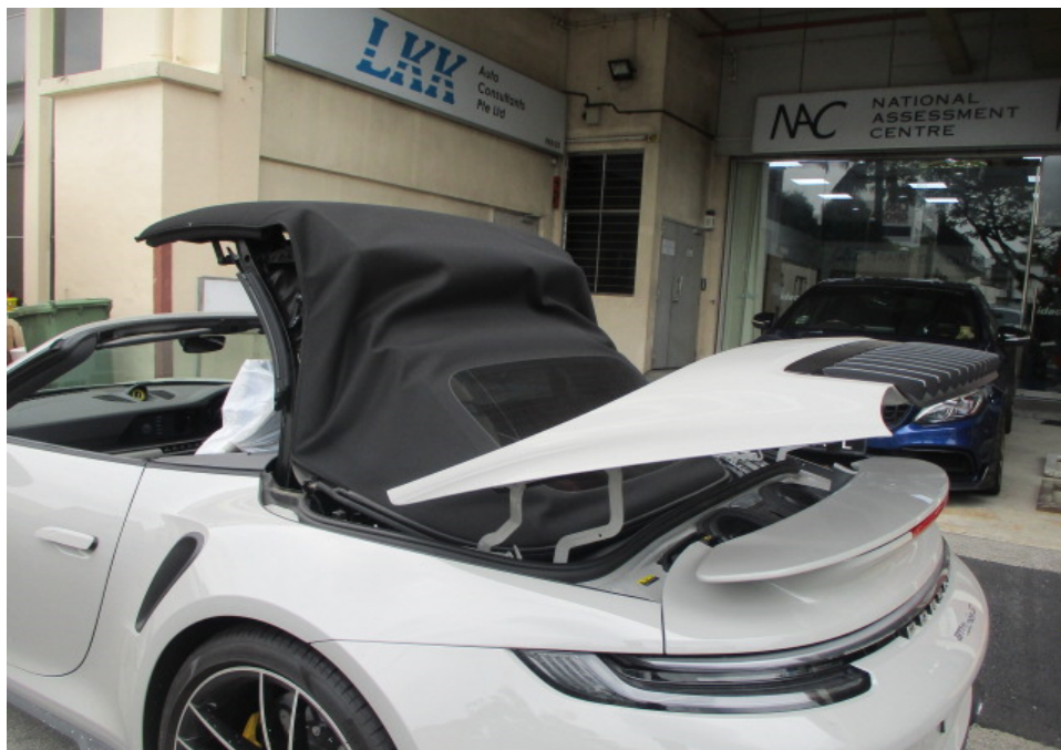
Photo 22 shows the Motor Car's soft top roof being tested. It was observed that as a safety feature, the soft top roof could only open and close when the Motor Car was in a stationary position or at low travelling speed. When opened, the soft top roof is completely folded into the rear compartment with no parts protruding out of the Motor Car's body. The soft top roof was also found adequately secured to the "A" pillar after closing.
