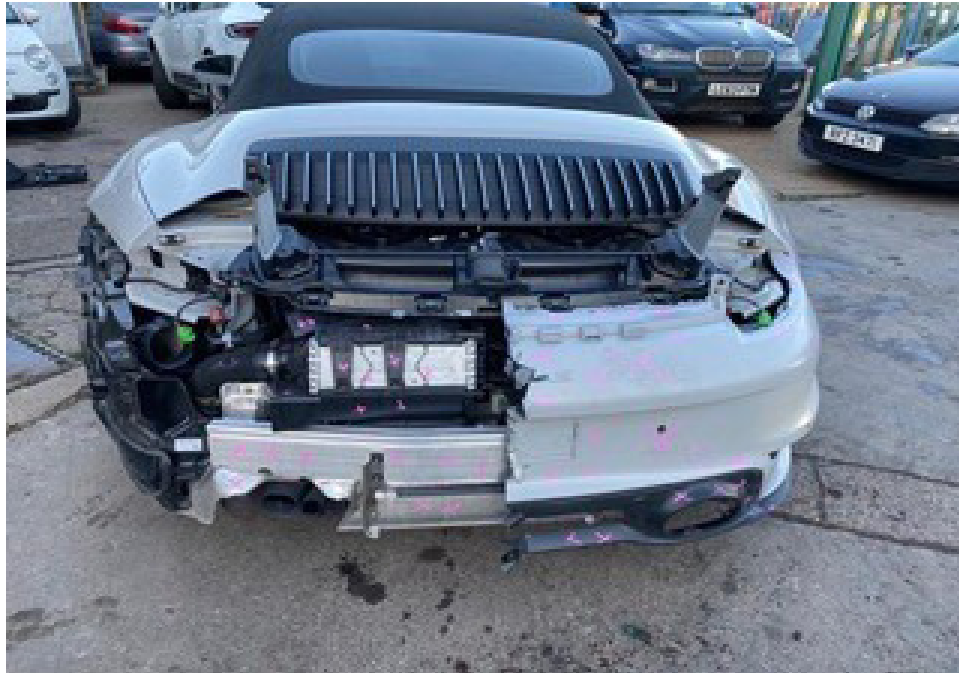
Photo 3 shows the rear body of the Motor Car (photograph provided to me). The photographs provided to me had showed damage to the rear portion of the Motor Car. Body parts that were either damaged, missing or dislodged include the rear bumper, rear bumper lower cover, rear bumper sensors, rear bumper left reflector, rear bumper left air duct, rear left exhaust garnish, rear right exhaust garnish, rear left taillamp, rear right taillamp, rear centre top reflector, rear centre top panel, rear top spoiler and third brake light amongst others.
