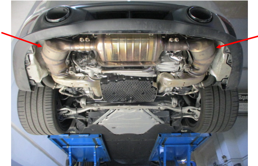
Photo 31 shows the Motor Car's exhaust system. My examination of the Motor Car's exhaust system revealed no sign(s) or indication(s) of any cut or weld marks along its exhaust pipes, on its catalytic converters (arrowed) and on its rear muffler.
