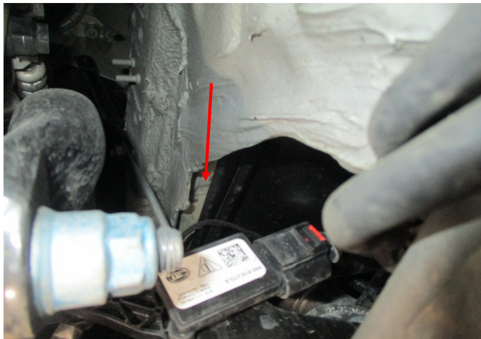
Photo 36 shows the chassis/structural body at the underside front left of the Motor Car. The original factory sealant (arrowed) at the joints along the chassis/structural body was observed to be untouched. In general, I had found no work was carried out on the chassis/structural body of the Motor Car. The chassis/structural body of the Motor Car was originally fitted.
