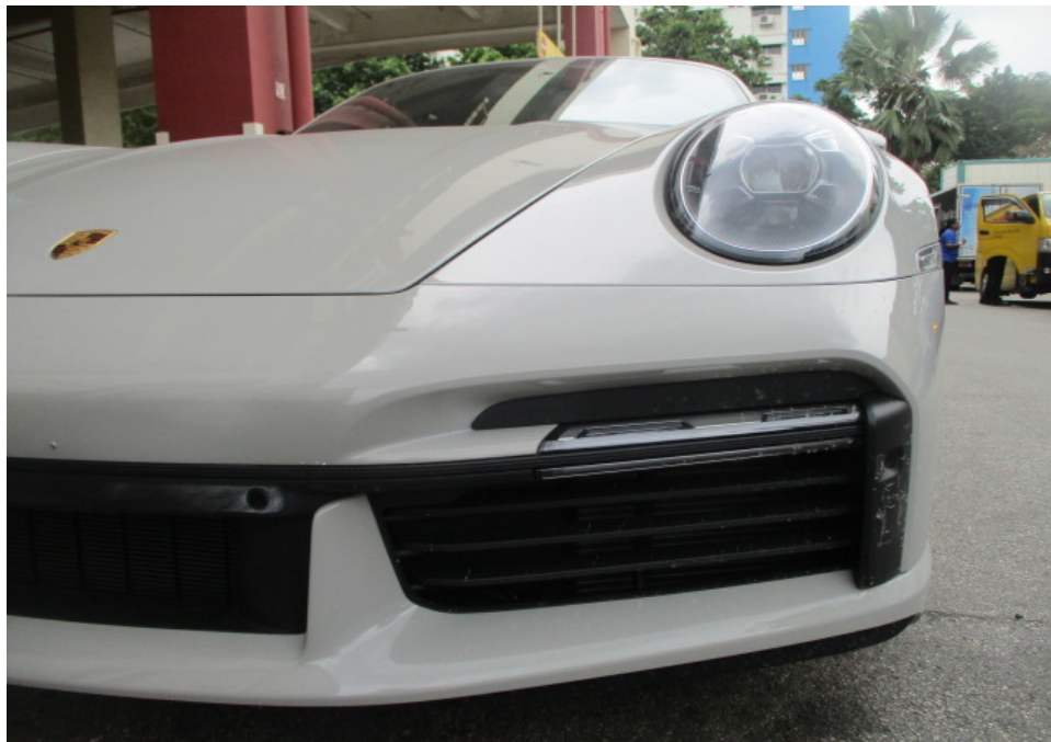
Photo 8 shows a closer view of the Motor Car's front bumper, front bumper left lower grille, front left day light and front left headlamp. The body parts at the frontal portion of the Motor Car were visually examined and it was observed that the repair/restoration works carried out to the damaged area of the Motor Car (refer to photograph 1 & 2 above) were reasonably adequate and in order.
