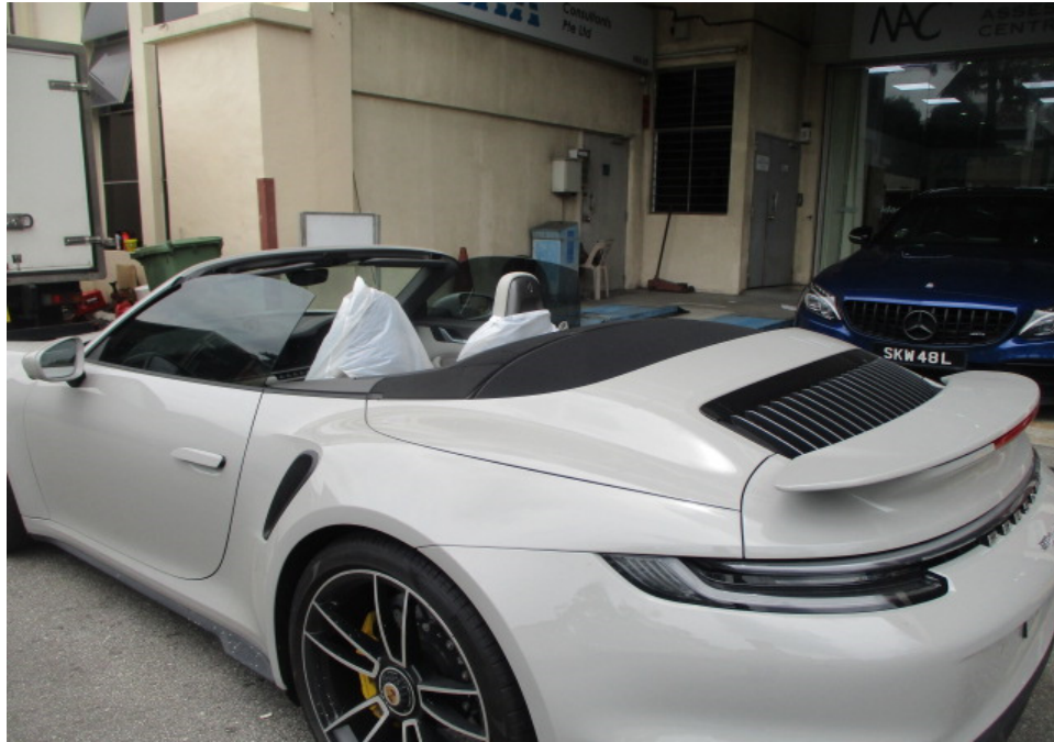
Photo 23 shows the Motor Car with its soft top roof completely folded. It was observed that as a safety feature, the soft top roof could only open and close when the Motor Car was in a stationary position or at low travelling speed. When opened, the soft top roof is completely folded into the rear compartment with no parts protruding out of the Motor Car's body. The soft top roof was also found adequately secured to the "A" pillar after closing.
