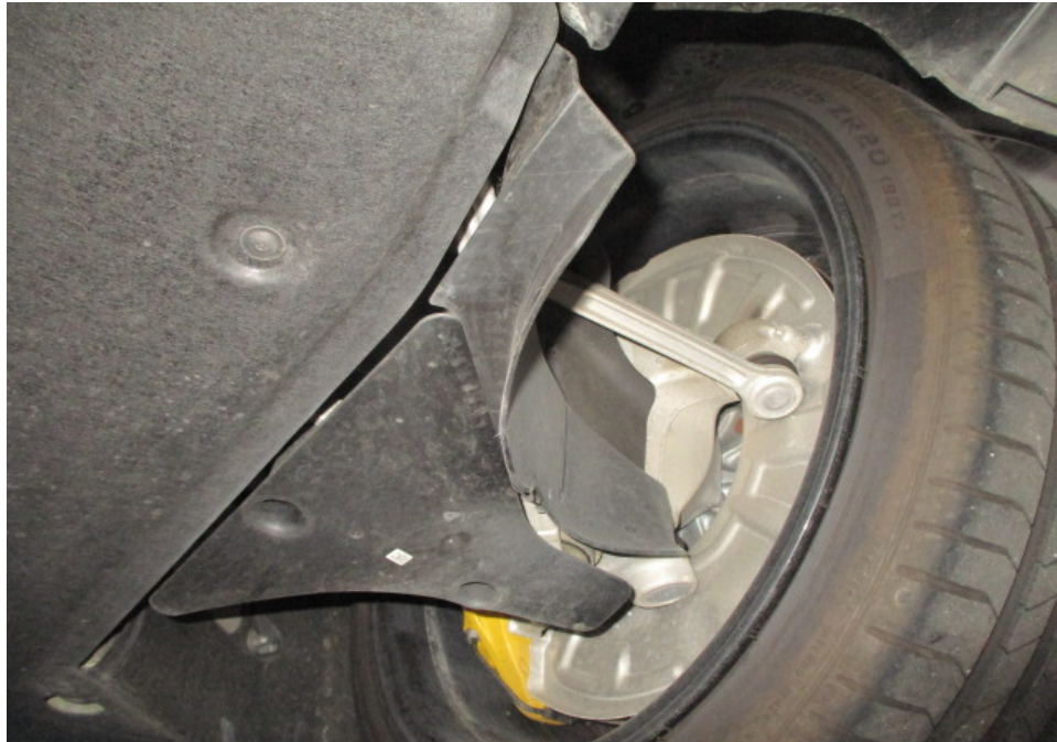
Photo 29 shows a general view of the control arms and linkages at the front left wheel of the Motor Car. I did not observe any fluid leak and/or fluid stain on the underside of the Motor Car. All of the Motor Car's undercarriage components were observed to be intact and secured in an appropriate manner.
