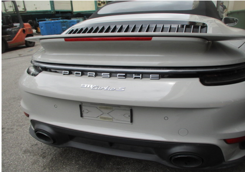
Photo 15 shows a closer view of the Motor Car's rear bumper, rear centre top reflector, rear centre top panel, rear top spoiler and third brake light. The body parts at the rear portion of the Motor Car were visually examined and it was observed that the repair/restoration works carried out to the damaged area of the Motor Car (refer to photograph 3 & 4 above) were reasonably adequate and in order.
