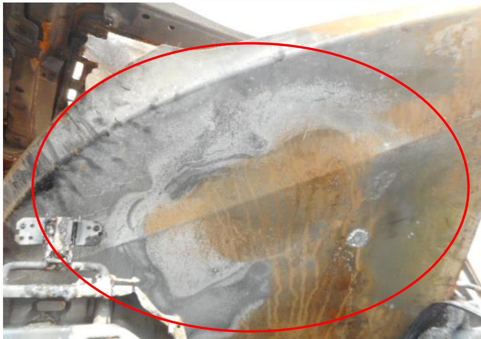
Photo 8 shows the exterior of the front bonnet of the Insured Vehicle at the time of our inspection. The high heat intensity burn marks (whitish burn marks) (circled) and rust that had development found on the exterior surface of the bonnet indicates that the fire had originated from the front portion of the Insured Vehicle.
