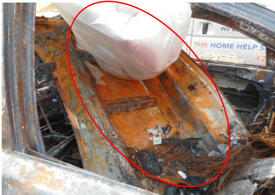
Photo 9 shows the underside of the front bonnet cover of the Insured Vehicle at the time of our inspection. The High heat intensity burn marks (whitish burn marks) and rust that had development found on the interior surface of the bonnet indicates that the fire had originated from the front portion of the Insured Vehicle.
