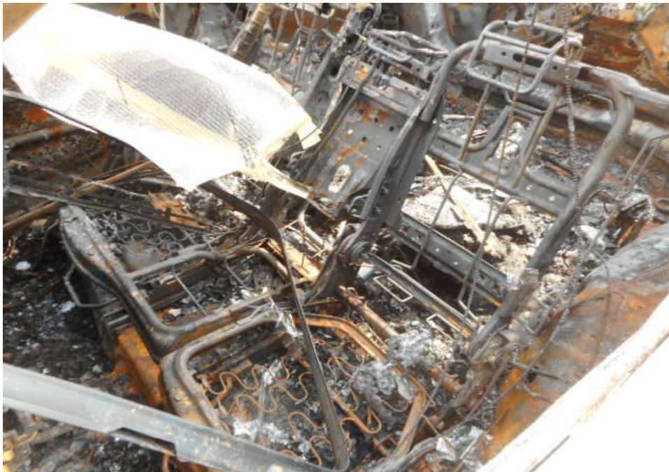
Photo 6 shows the general view of the interior compartment of the Insured Vehicle at the time of our inspection. Its interior compartment completely burnt as a result of the fire.
