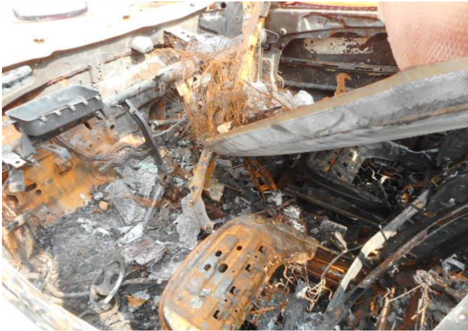
Photo 5 shows the general view of the interior compartment of the Insured Vehicle at the time of our inspection. Its interior compartment completely burnt as a result of the fire.
