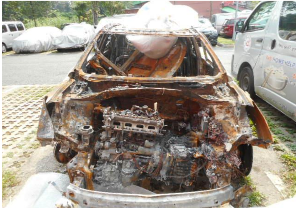
Photo 1 shows the general view of the front portion of the Insured Vehicle at the time of our inspection. The Insured Vehicle was observed to have sustained extensive fire damage all around. Its engine compartment and interior compartment was completely burnt. Rust had accumulated all over the front engine portion of the Insured Vehicle as a result of exposure to environmental condition for a period of time.
