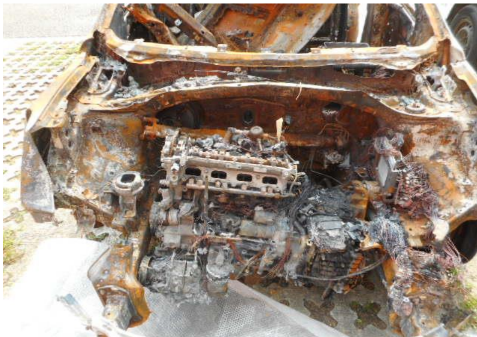
Photo 7 shows the engine compartment of the Insured Vehicle at the time of our inspection. The entire engine compartment of the Insured Vehicle was observed to be severely burnt. Most of the parts inside the engine compartment were found to be burnt and/or melted as a result of the fire.
