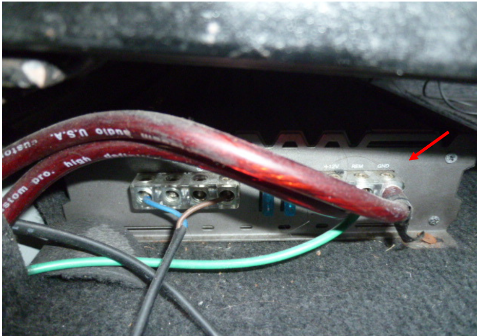
Photo 14 shows the aftermarket amplifier additionally fitted onto the Insured Vehicle upon our inspection (arrowed).
