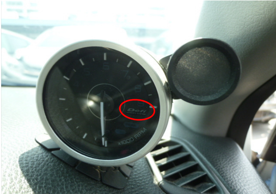
Photo 12 shows the aftermarket tachometer gauge additionally fitted onto the Insured Vehicle upon our inspection. The brand of the tachometer gauge was 'DEFI' (circled).
