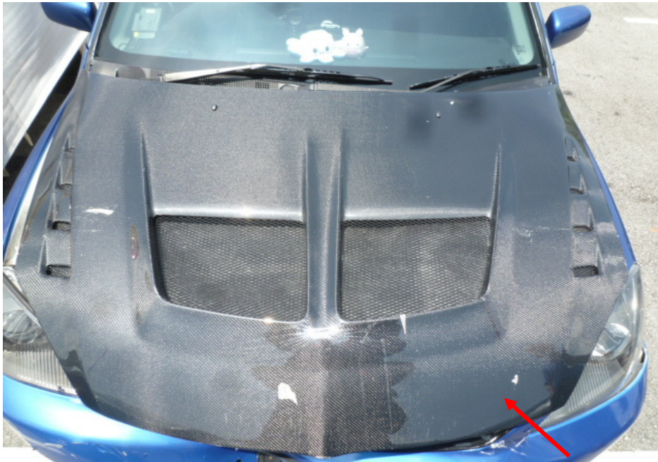
Photo 28 shows a general view of the aftermarket carbon fibre front bonnet found fitted onto the Insured Vehicle at the time of our inspection (arrowed).
