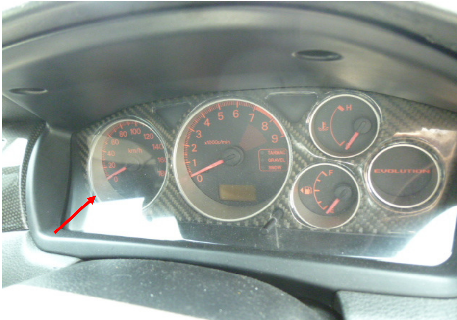
Photo 13 shows the aftermarket speedometer gauge display fitted onto the Insured Vehicle upon our inspection (arrowed).
