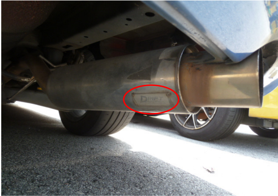
Photo 22 shows a close up left side view of the non-standard rear exhaust muffler which is part of the full exhaust system that was found to be fitted on the Insured Vehicle at the time of our inspection. The brand of the rear exhaust muffler was 'DRIFT RACING' (circled).
