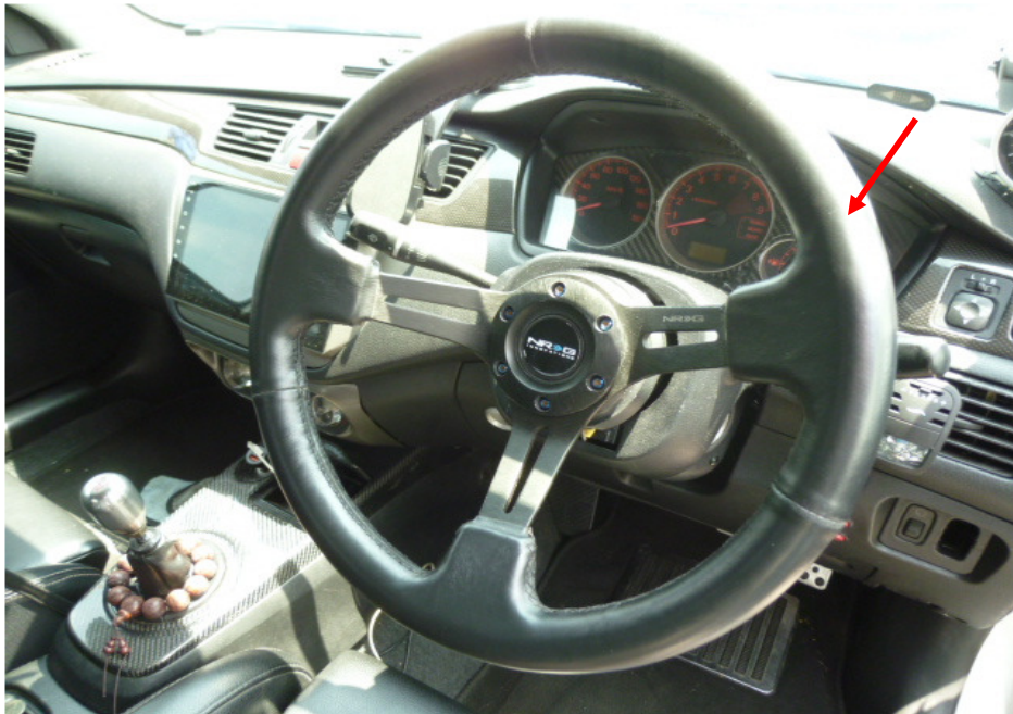
Photo 10 shows a closer view of the aftermarket steering wheel found to be fitted on the Insured Vehicle at the time of our inspection (arrowed). The steering wheel found fitted on the Insured Vehicle was not the standard type for the Insured Vehicle.
