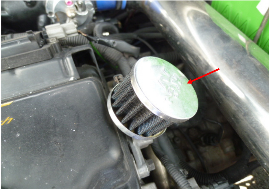
Photo 8 shows a close up view of the non- standard crank case engine breather air filter (arrowed) fitted onto the Insured Vehicle upon our inspection.
