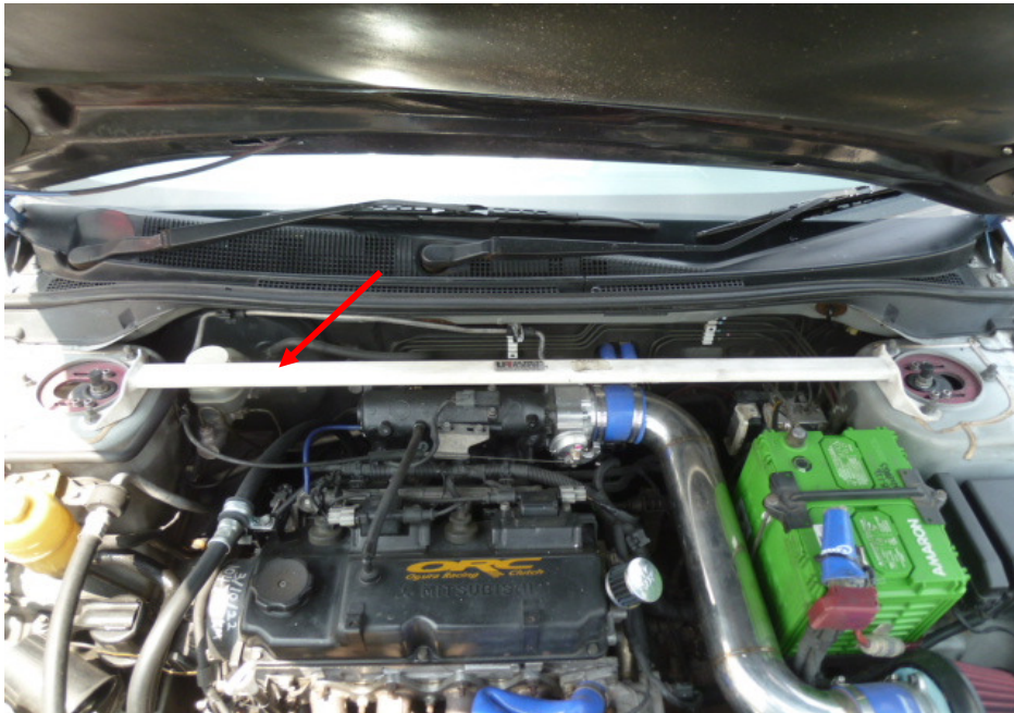
Photo 4 shows a closer view of the non- standard front strut bar fitted onto the Insured Vehicle upon our inspection (arrowed).
