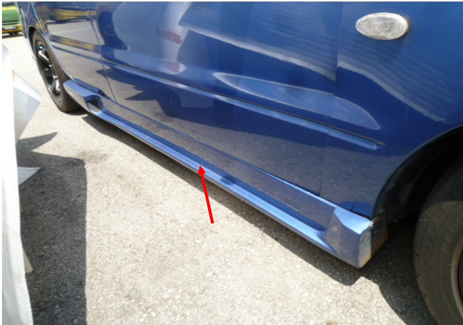
Photo 29 shows a general view of the aftermarket right side skirting found fitted onto the Insured Vehicle at the time of our inspection (arrowed).
