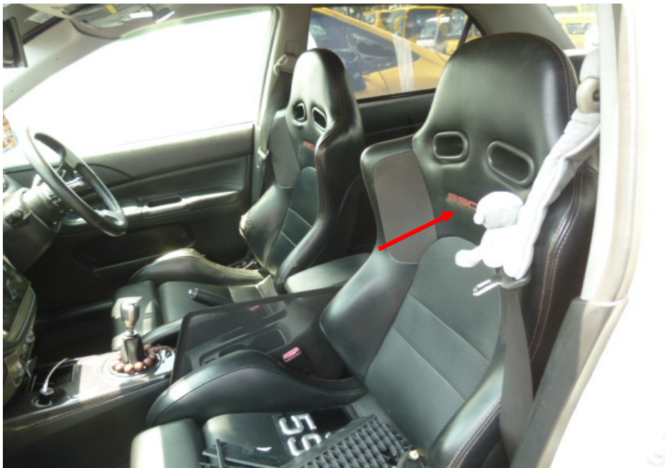
Photo 11 shows a closer view of the aftermarket bucket seats found to be fitted on the Insured Vehicle at the time of our inspection. The brand of the bucket seats was 'SSCUS' (arrowed).
