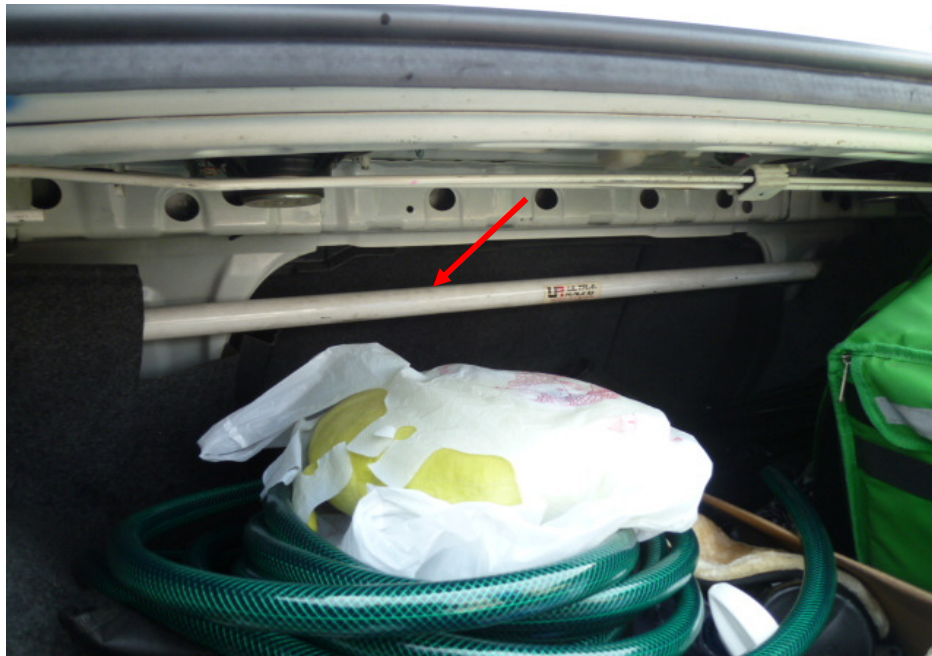
Photo 17 shows a closer view of the non- standard rear strut bar fitted onto the Insured Vehicle upon our inspection (arrowed).
