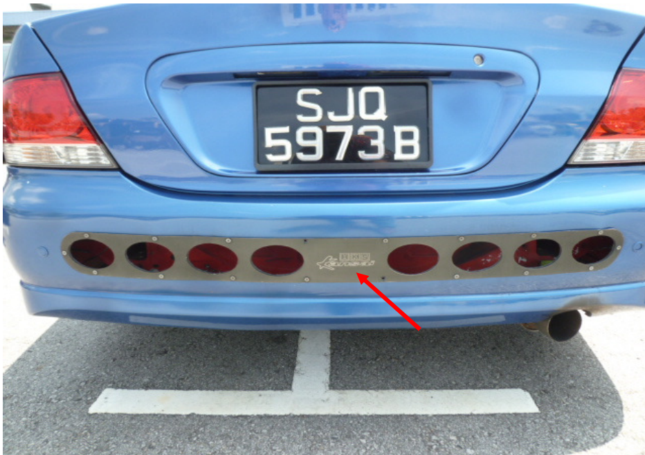
Photo 30 shows a general view of the aftermarket rear bumper found fitted onto the Insured Vehicle at the time of our inspection (arrowed).
