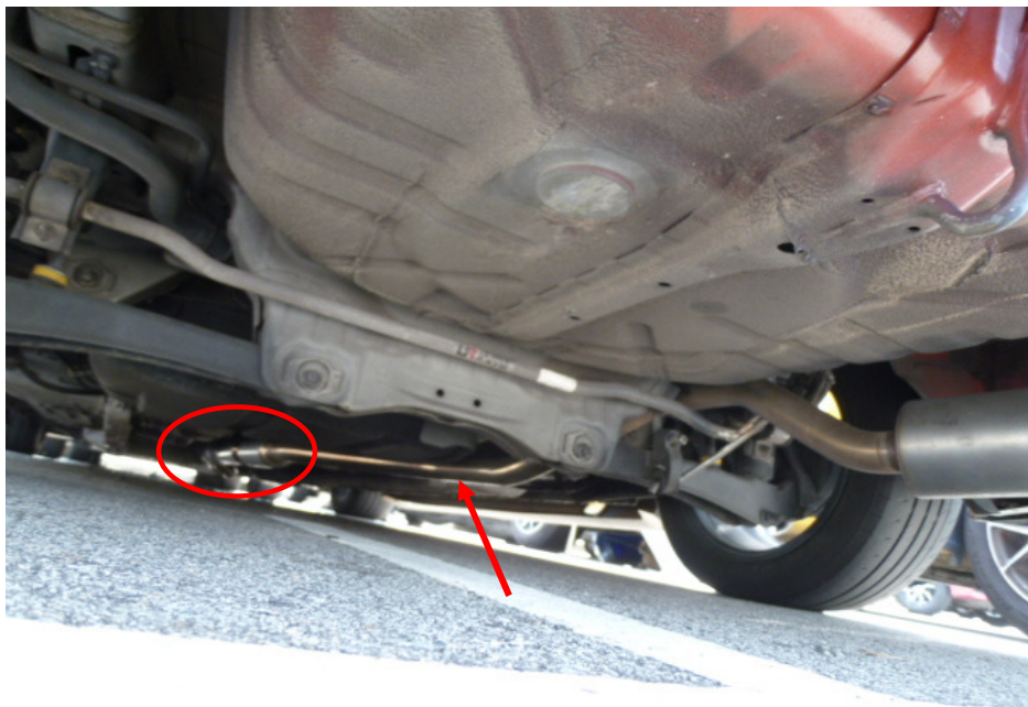
Photo 23 shows a closer view of the mid- pipe (arrowed) and catalytic converter (circled) of the non-standard full exhaust system that was found to be fitted on the Insured Vehicle at the time of our inspection. The brand of the full exhaust system was 'DRIFT RACING'.
