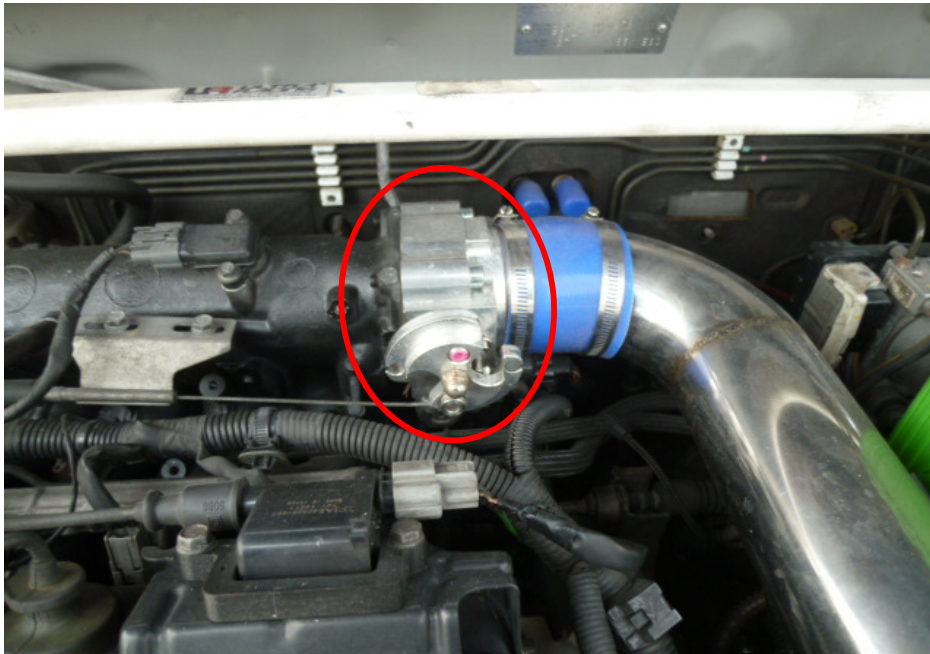
Photo 9 shows a close up view of the non- standard throttle body fitted onto the Insured Vehicle upon our inspection (circled).
