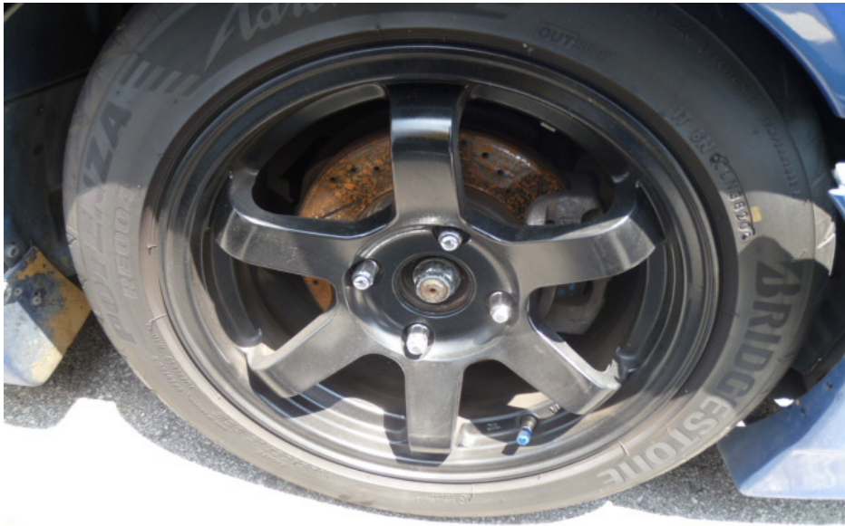
Photo 16 shows the non-standard rim found to be fitted on the Insured Vehicle at the time of our inspection. The 15- inch alloy rims fitted on the Insured Vehicle were not the standard type for the Insured Vehicle.
