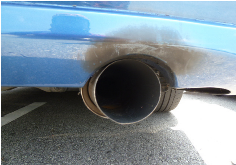
Photo 21 shows a front view of the non-standard rear exhaust muffler which is part of the full exhaust system that was found to be fitted on the Insured Vehicle at the time of our inspection. The brand of the rear exhaust muffler was 'DRIFT RACING'.
