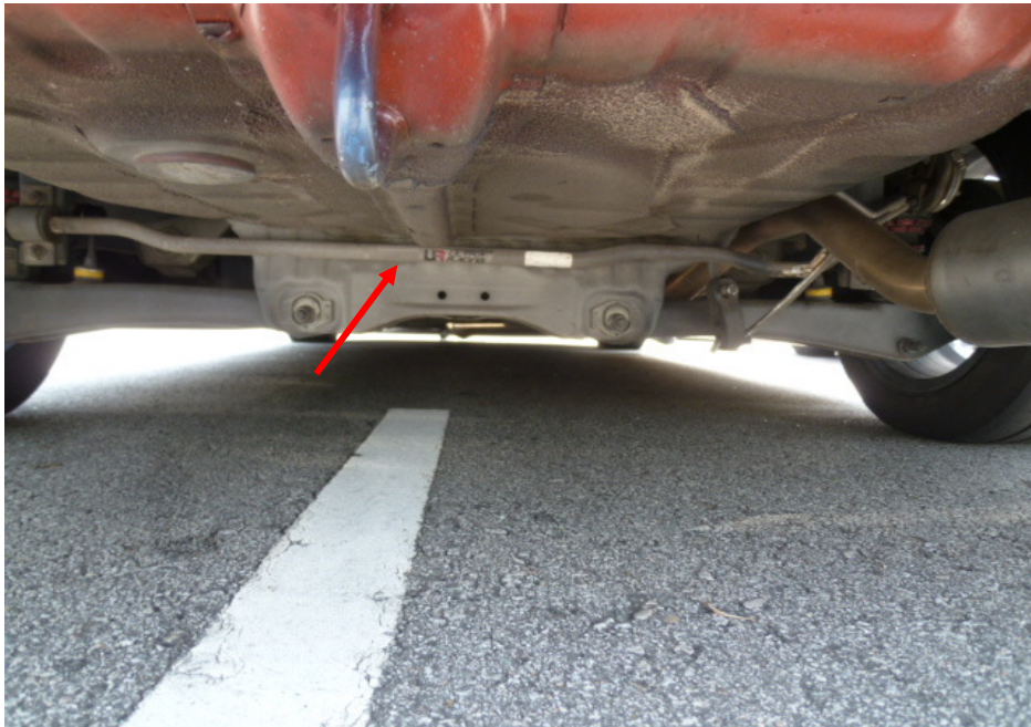
Photo 18 shows a closer view of the non- standard lower rear strut bar fitted onto the Insured Vehicle upon our inspection (arrowed).
