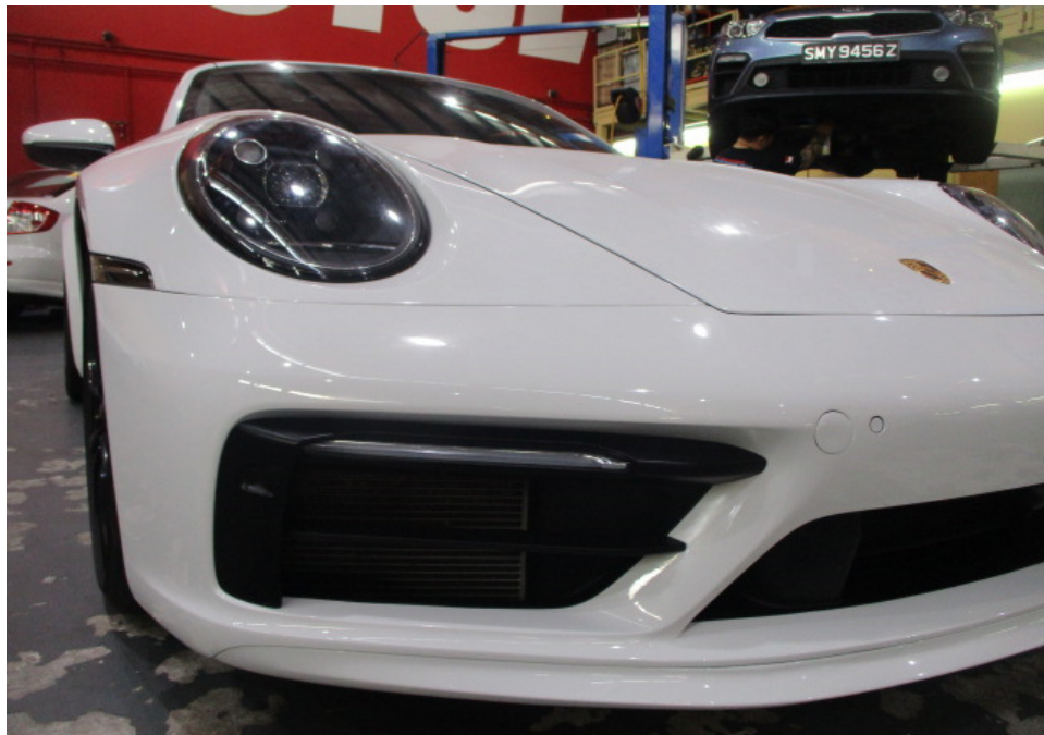
Photo 10 shows a closer view of the Motor Car's front bumper, front bumper right grille, front right day light, front right headlamp and front bonnet. The body parts at the front right portion of the Motor Car were visually examined and it was observed that the repair/restoration works carried out to the damaged area of the Motor Car (refer to photograph 2 above) were reasonably adequate and in order.
