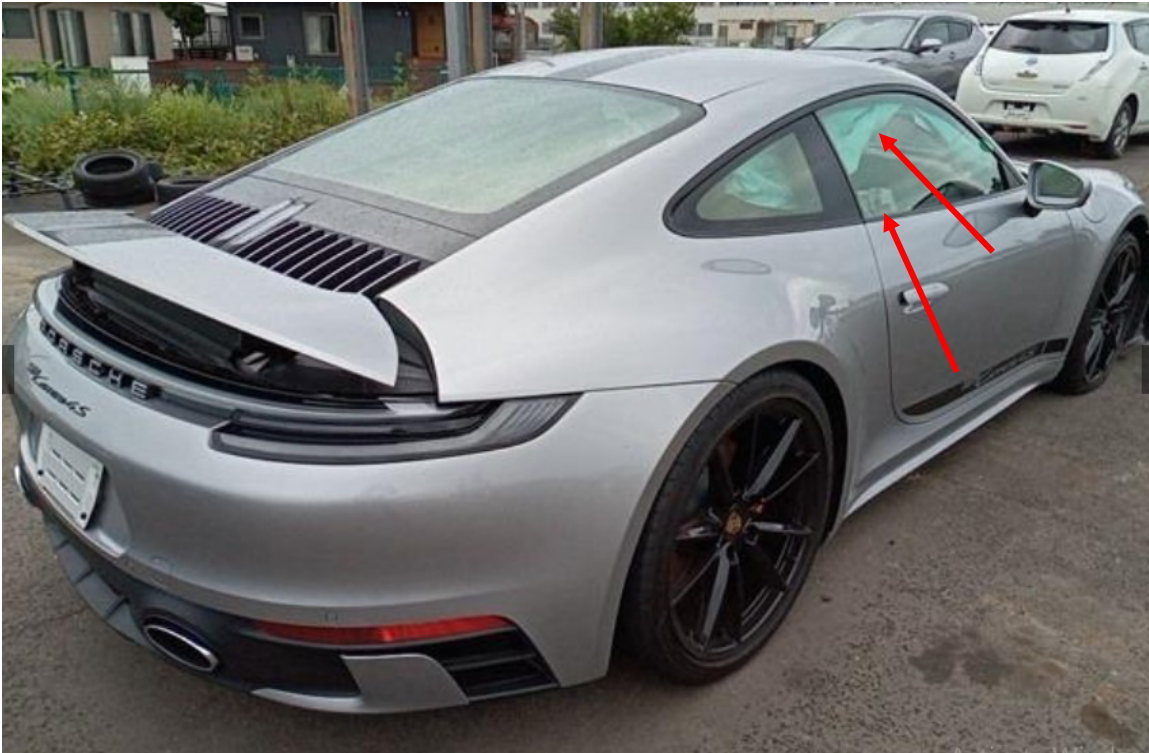
Photo 3 shows the rear right body of the Motor Car (photograph provided to me). There was no physical damage observed to other areas of the Motor Car apart for its front left portion. The driver's airbag and right curtain airbag were deployed (arrowed).
