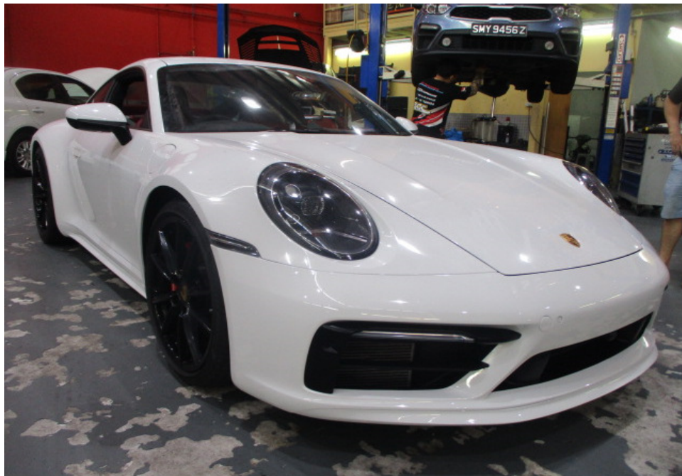
Photo 8 shows a general view of the front right body of the Motor Car at the time of my inspection. The Motor Car was observed to be in a relatively good general condition with no loose exterior fittings observed. The body parts at the front right portion of the Motor Car were visually examined and it was observed that the repair/restoration works carried out to the damaged area of the Motor Car (refer to photograph 2 above) were reasonably adequate and in order.
