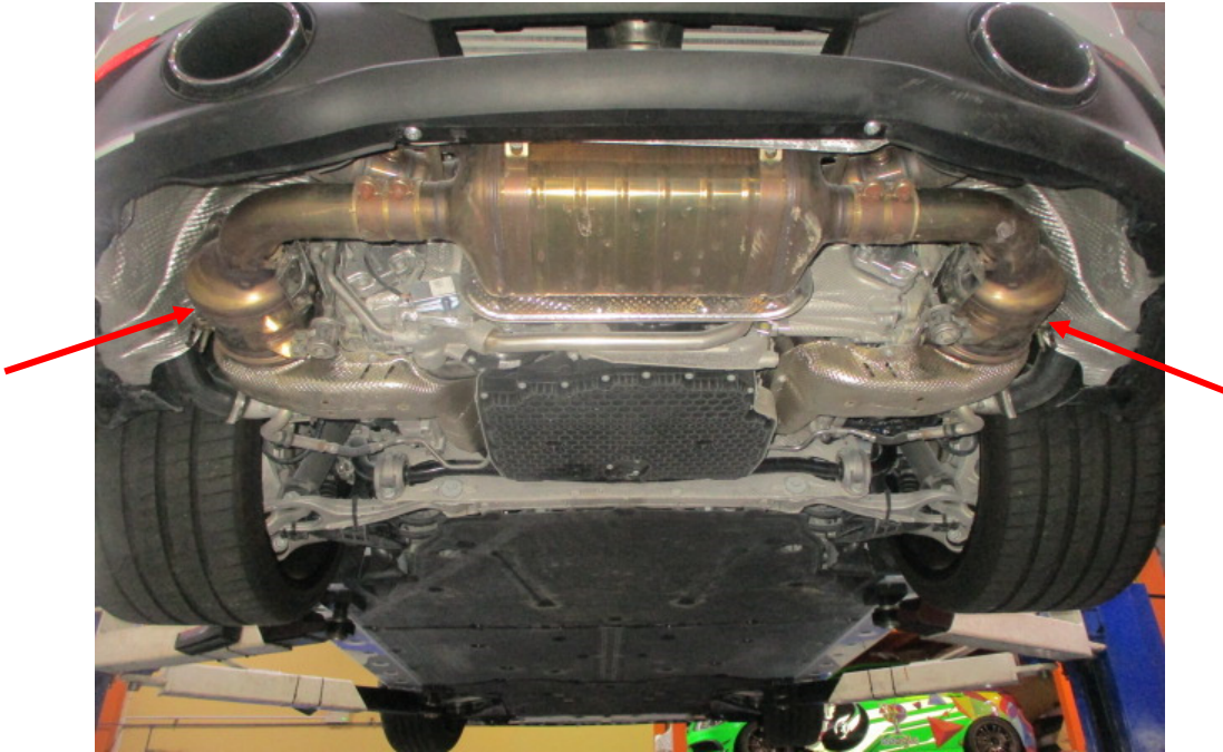
Photo 25 shows the Motor Car's exhaust system. My examination of the Motor Car's exhaust system revealed no sign(s) or indication(s) of any cut or weld marks along its exhaust pipes, on its catalytic converters (arrowed) and on its rear muffler.
