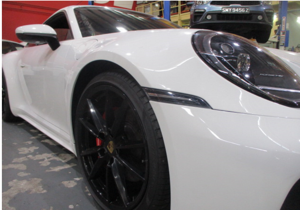
Photo 9 shows a closer view of the Motor Car's front right headlamp, front right fender, front right signal lamp and front right wheel rim. The body parts at the front right portion of the Motor Car were visually examined and it was observed that the repair/restoration works carried out to the damaged area of the Motor Car (refer to photograph 2 above) were reasonably adequate and in order.
