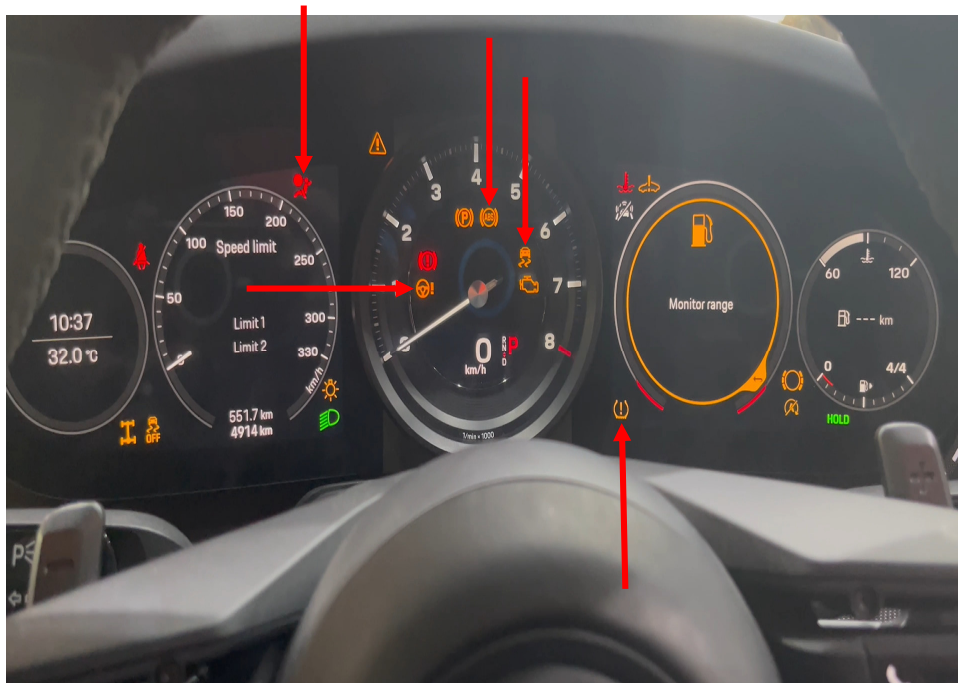
Photo 18 shows the warning lights for the various electronic safety features appearing on the instrument panel of the Motor Car during its self-test when the engine is cranked, in particular the ABS, SRS, EPS, TPM and TCS lights (arrowed).
