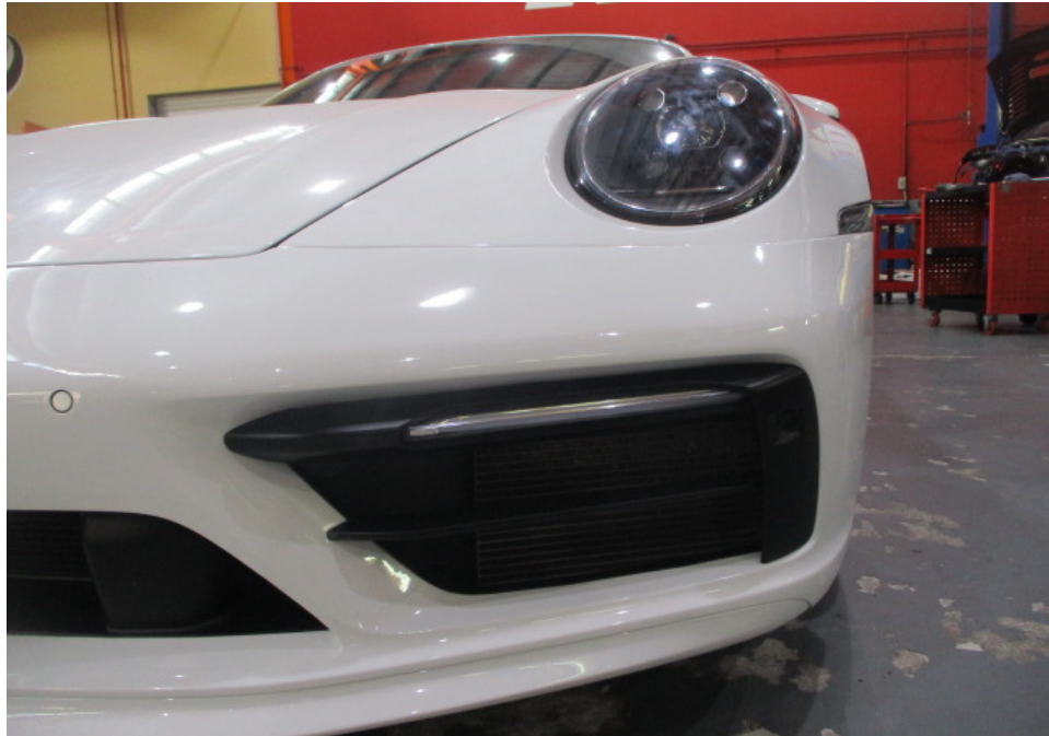
Photo 7 shows a closer view of the Motor Car's front bumper, front bumper left grille, front bumper left sensors, front left day light and front bonnet. The body parts at the front left portion of the Motor Car were visually examined and it was observed that the repair/restoration works carried out to the damaged area of the Motor Car (refer to photograph 1 above) were reasonably adequate and in order.
