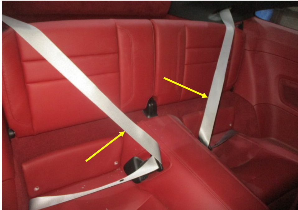
Photo 17 shows the seats of the Motor Car. All the seats of the Motor Car were secured via seat rails to the floorboard. They were also fitted with a retractable seat belt reel and a pre-tensioner. The seat belts (arrowed) were tested and were able to be fastened into the respective pre-tensions that were fitted on the side of each individual seat.
