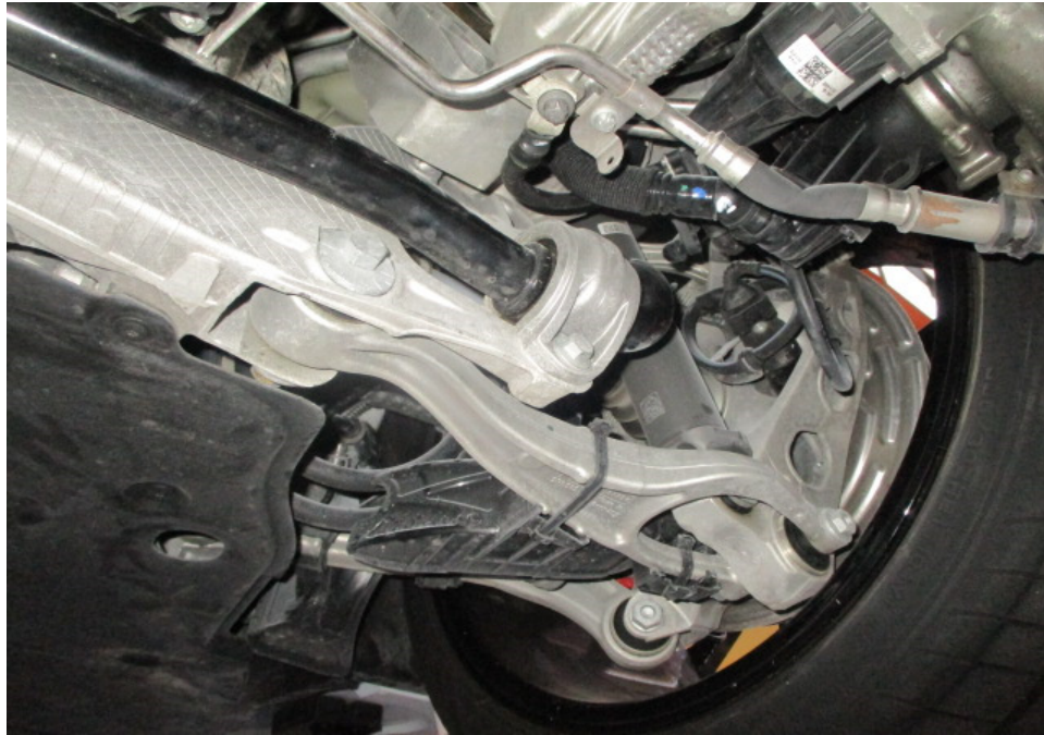
Photo 21 shows a general view of the control arms and linkages at the rear right wheel of the Motor Car. I did not observe any fluid leak and/or fluid stain on the underside of the Motor Car. All of the Motor Car's undercarriage components were observed to be intact and secured in an appropriate manner.
