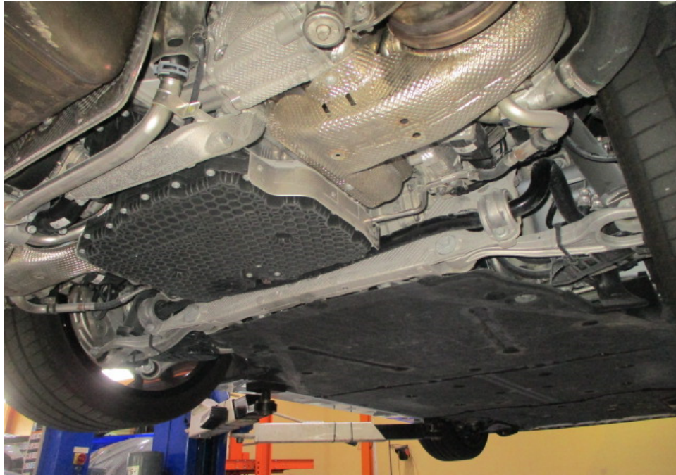
Photo 27 shows another view of the Motor Car's engine compartment. The engine compartment was at the rear underside of the Motor Car. The various parts and components inside the engine compartment were all observed to be intact and properly fitted. There was also no sign(s) or indication(s) of fluid leak and/or fluid stain found inside the engine compartment.
