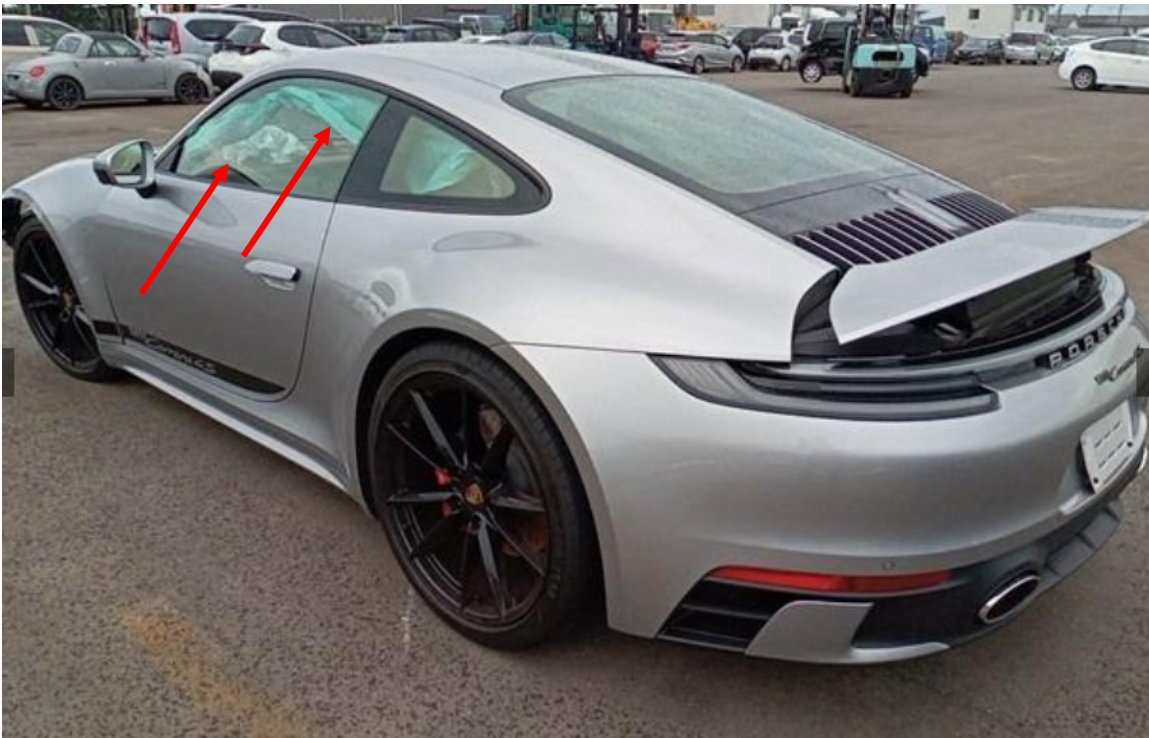
Photo 4 shows the rear left body of the Motor Car (photograph provided to me). There was no physical damage observed to other areas of the Motor Car apart for its front left portion. The front left passenger airbag and left curtain airbag were deployed (arrowed).
