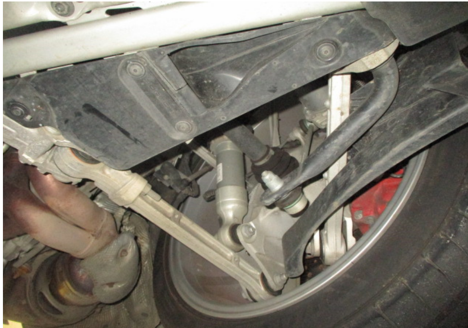
Photo 23 shows a general view of the control arms and linkages at the rear left wheel of the Motor Car. I did not observe any fluid leak and/or fluid stain on the underside of the Motor Car. All of the Motor Car's undercarriage components were observed to be intact and secured in an appropriate manner.
