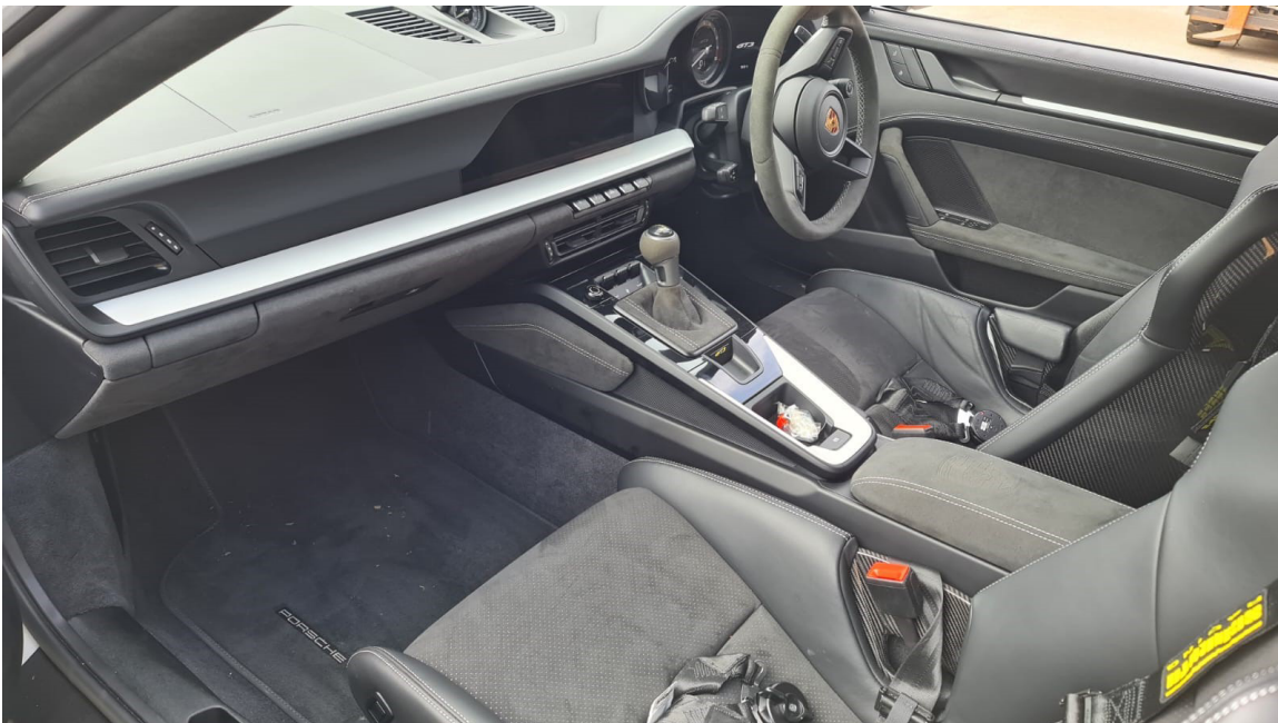
Photo 6 shows the interior compartment of the Motor Car (photograph provided to me). The various parts and components at the front of the interior compartment were all intact and unaffected. The Motor Car's airbag(s) was not deployed as seen from the photographs that were provided to me.
