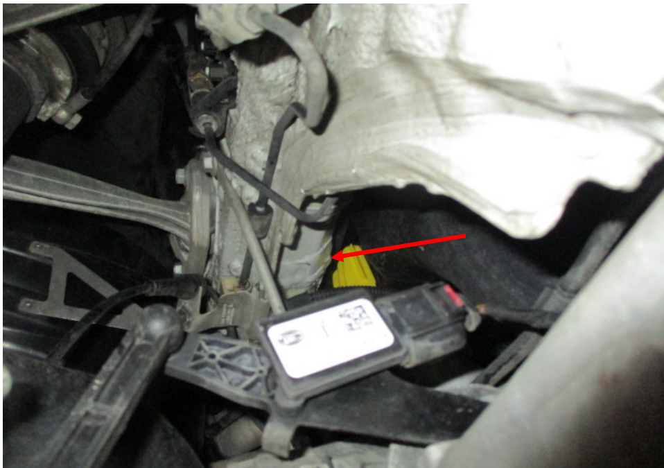
Photo 31 shows the chassis/structural body at the underside front left of the Motor Car. I did not find any weld marks other than original spot weld marks on the chassis/structural body of the Motor Car. The original factory sealant (arrowed) at the joints along the chassis/structural body was untouched, indicating no work was done on the chassis/structural body of the Motor Car and that the chassis/structural body was originally fitted.
