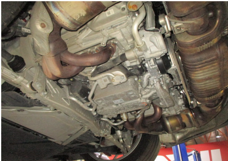
Photo 27 shows a general view of the Motor Car's engine compartment. The engine compartment was at the rear underside of the Motor Car. The various parts and components inside the engine compartment were all observed to be intact and properly fitted. There was also no sign(s) or indication(s) of fluid leak and/or fluid stain found inside the engine compartment.
