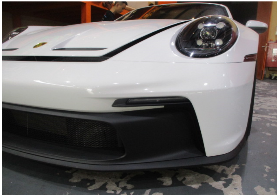
Photo 9 shows a closer view of the Motor Car's front bumper, front bumper lower cover, front bumper lower lip and front left day light. The body parts at the frontal portion of the Motor Car were visually examined and it was observed that the repair/restoration works carried out to the damaged area of the Motor Car (refer to photograph 1 & 3 above) were reasonably adequate and in order.
