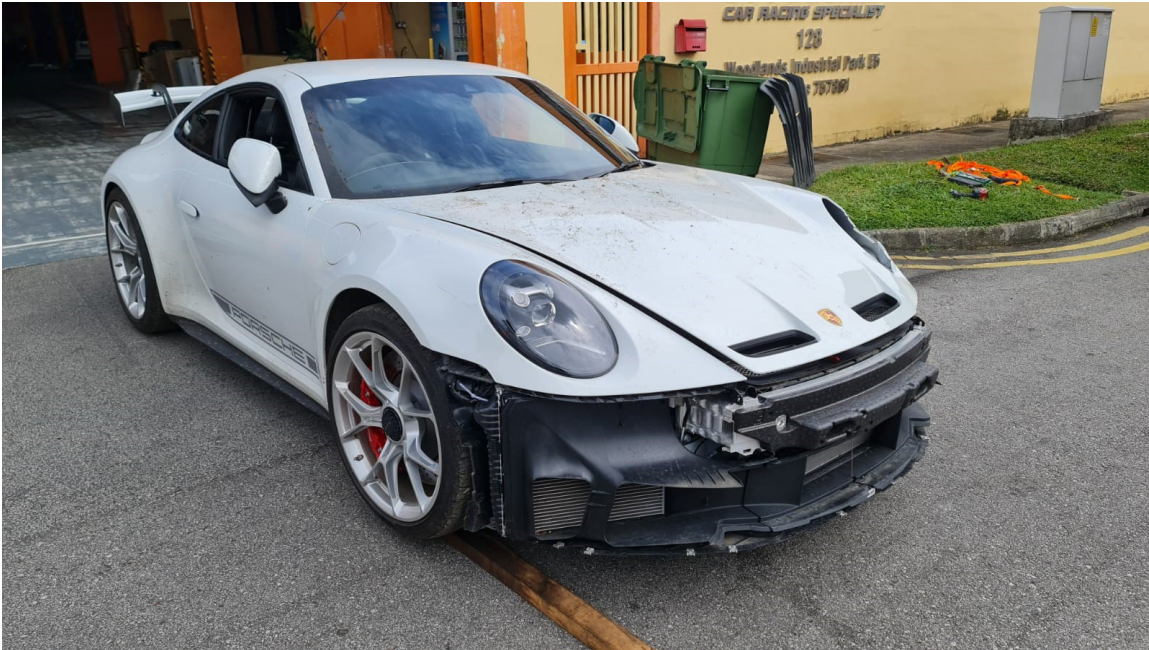
Photo 3 shows the front right body of the Motor Car (photograph provided to me). The Motor Car's front bumper and all its related parts and attachments like the front bumper lower cover, front bumper lower lip, front bumper centre lower grille, front bumper tow hook cover, front right day light and front right signal lamp amongst others, were observed to be missing/dislodged/damaged. The airbag(s) of the Motor Car was not deployed as seen from the photographs that were provided to me.
