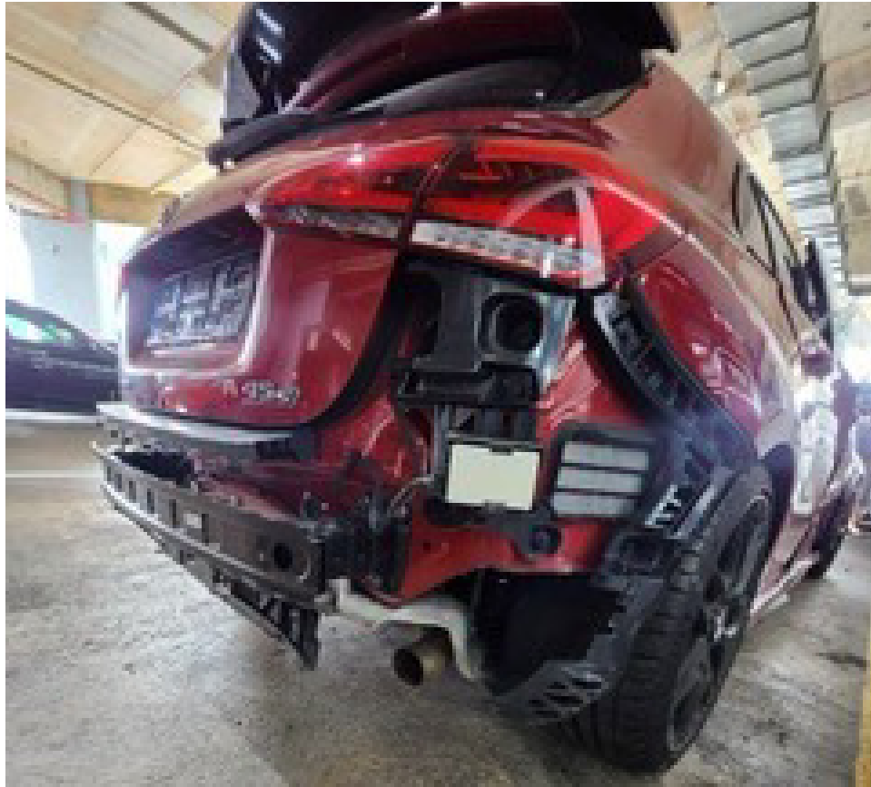
Photo 4 shows the rear right body of the Motor Car (photograph provided to me). The Motor Car's rear bumper and all its related parts and attachments like the rear bumper lower spoiler, rear bumper tow hook cover, rear bumper left reflector, rear bumper right reflector, rear bumper sensors, rear left exhaust garnish and rear right exhaust garnish amongst others, were also observed to be missing/dislodged/damaged.
