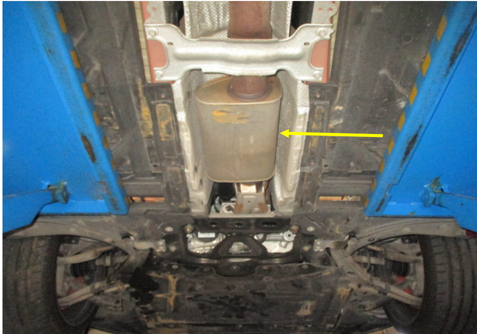
Photo 28 shows the front section of the Motor Car's exhaust system. My examination of the Motor Car's exhaust system revealed no sign(s) or indication(s) of any cut or weld marks along its exhaust pipes, on its centre resonator box (arrowed), on its rear muffler and on its catalytic converter.
