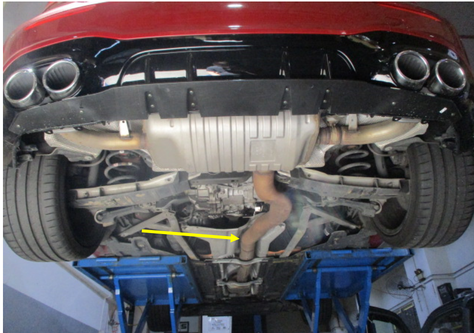
Photo 27 shows the rear section of the Motor Car's exhaust system. My examination of the Motor Car's exhaust system revealed no sign(s) or indication(s) of any cut or weld marks along its exhaust pipes (arrowed), on its centre resonator box, on its rear muffler and on its catalytic converter.
