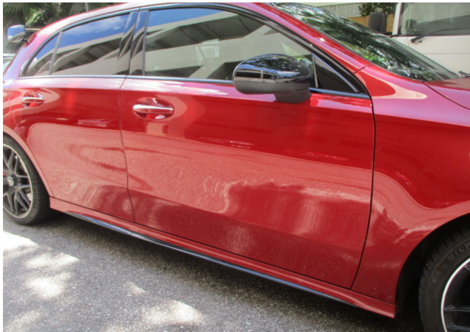
Photo 9 shows a closer view of the Motor Car's front right door, rear right door and right side rocker panel garnish. The body parts at the right side centre portion of the Motor Car were visually examined and it was observed that the repair/restoration works carried out to the damaged area of the Motor Car (refer to photograph 1 & 2 above) were reasonably adequate and in order.
