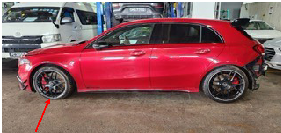
Photo 5 shows the left side body of the Motor Car (photograph provided to me). No physical damage was observed to the left side portion of the Motor Car. The orientation of the front right wheel (refer to photograph 1 above) and front left wheel (arrowed) indicates damage to the undercarriage parts at the front right wheel of the Motor Car.
