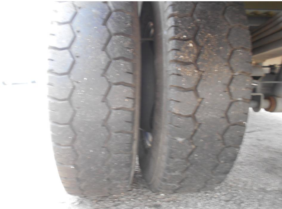
Photo 9 shows the condition of the rear left tyres of the Motor Lorry, which was observed to be in serviceable condition with remaining tread depth of approximately 3.7mm. The tyres, which were wrapped around standard steel wheel rim, were also observed to be sufficiently inflated for vehicular operation. There was also no damage found on all 6 steel wheel rims of the Motor Lorry.
