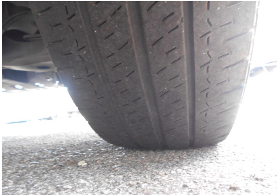
Photo 7 shows the condition of the front right tyre of the Motor Lorry, which was observed to be in serviceable condition with remaining tread depth of approximately 4mm. The tyre, which was wrapped around standard steel wheel rim, was also observed to be sufficiently inflated for vehicular operation. There was no tear, cut or burst mark(s) on the outer and the inner sidewalls as well as across the tread of the 6 tyres that were fitted on the Motor Lorry.
