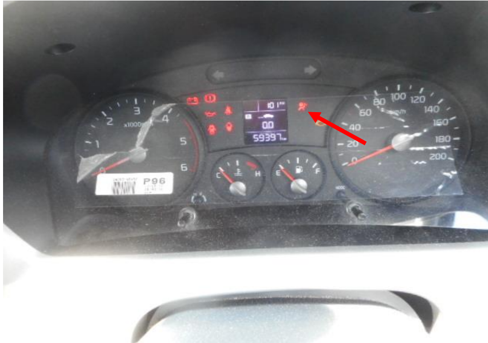
Photo 24 shows the warning light for Supplemental Restraint System (SRS) (arrowed) appearing on the instrument panel of the Motor Lorry during the self-test of its various electronic operating systems when its engine was cranked.
