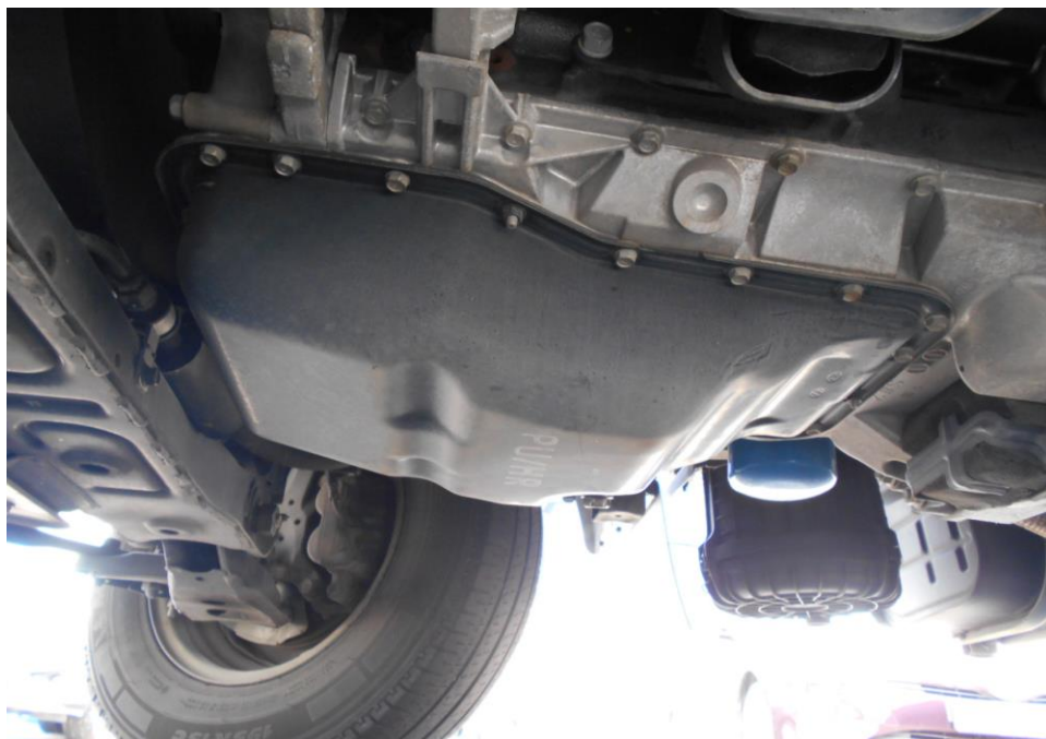
Photo 16 shows the undercarriage of the Motor Lorry, at the area where the engine housing and transmission housing are located. I did not find any sign(s) or indication(s) of fluid leak and/or fluid stain(s) on the underside of the Motor Lorry.
