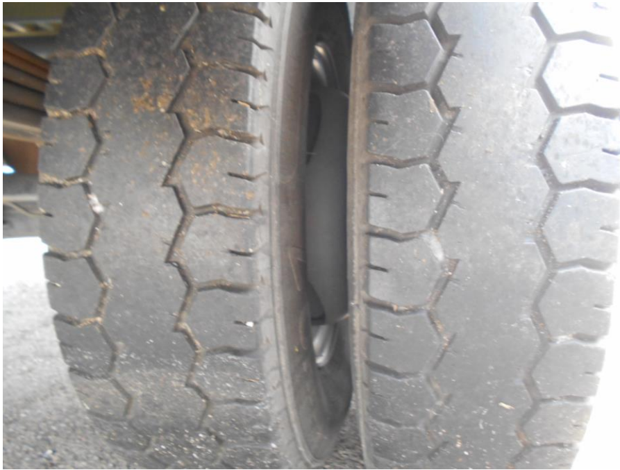
Photo 8 shows the condition of the rear right tyre of the Motor Lorry, which was observed to be in serviceable condition with remaining tread depth of approximately 4mm. The tyre, which was wrapped around standard steel wheel rim, it was observed to be sufficiently inflated for vehicular operation.
