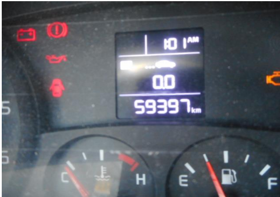
Photo 1 shows a general view of the instrument cluster of the Motor Lorry at the time of my inspection. The mileage of the Motor Lorry was 59,397km.
