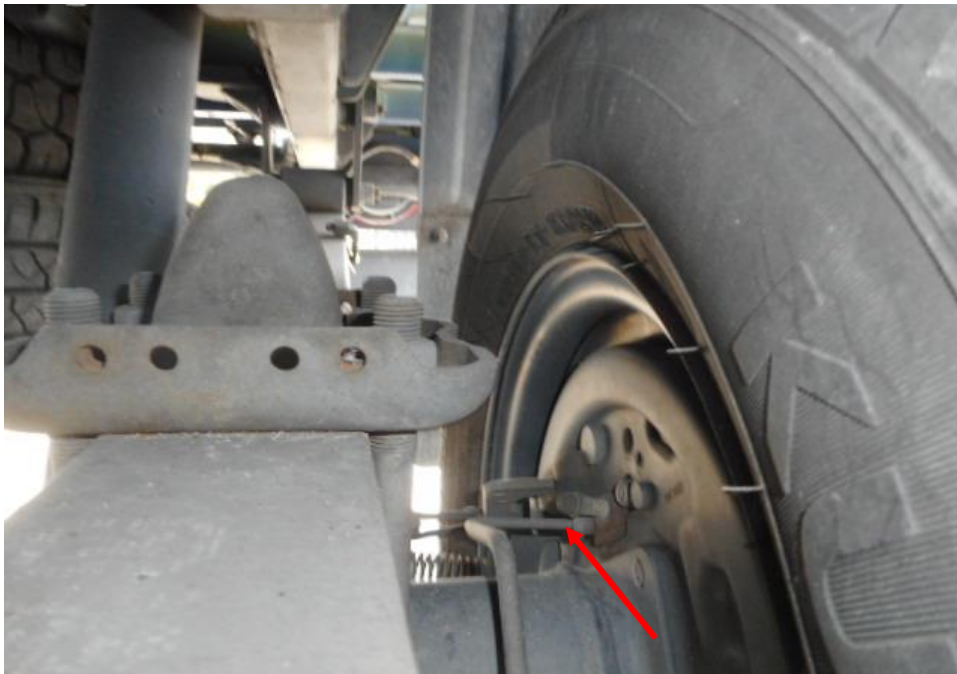
Photo 19 shows the brake pipe (arrowed) at the rear right wheel of the Motor Lorry. I did not observe any leakage of brake fluid at the time of my inspection of the Motor Lorry. My static tests of the Motor Lorry's braking system, along with my visual examination of the various mechanical components in the braking system, had indicated that there was no internal leakage of pressure/vacuum. Hence the braking system of the Motor Lorry was likely to be in serviceable condition at the material time of accident.
