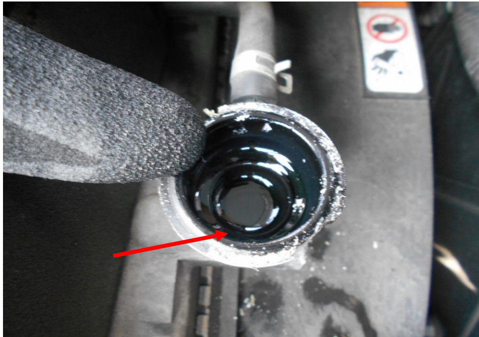
Photo 13 shows the engine coolant of the Motor Lorry at the time of my inspection. The engine coolant was observed to be of sufficient level and without any visible contamination.
