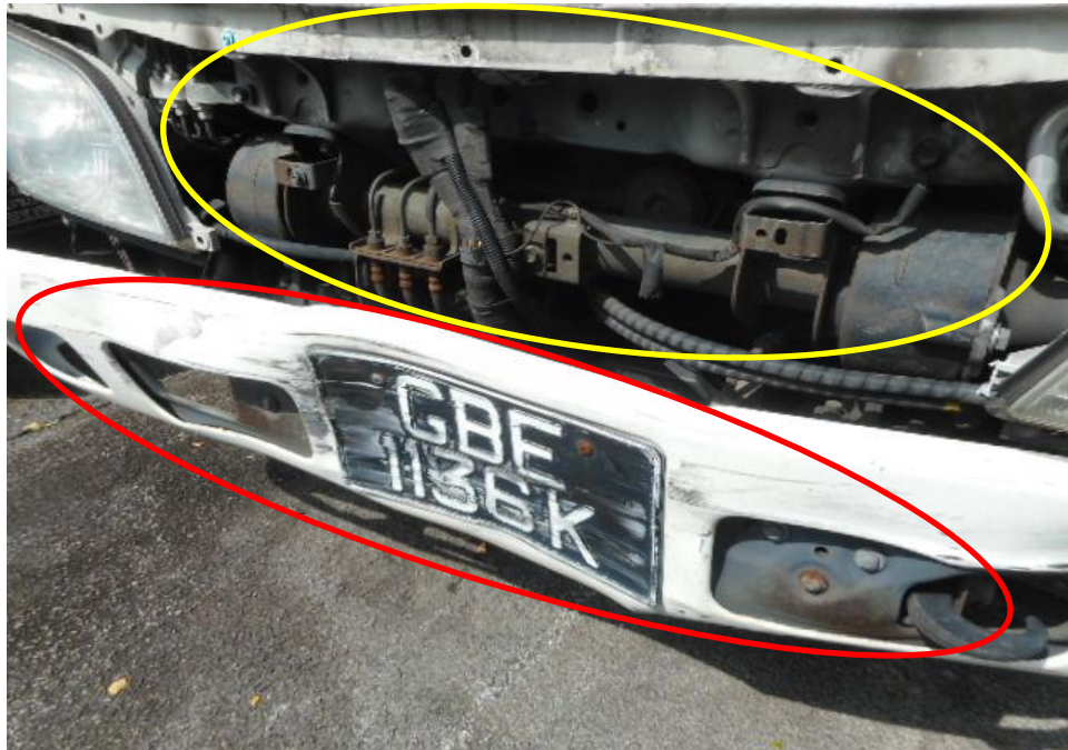
Photo 4 shows a close up view of the Motor Lorry's frontal portion at the time of my inspection. It appeared to have sustained damage at its frontal portion. Its front grille (yellow circle) and front bumper (red circle) was damage at the time of my inspection as a result of the accident.
