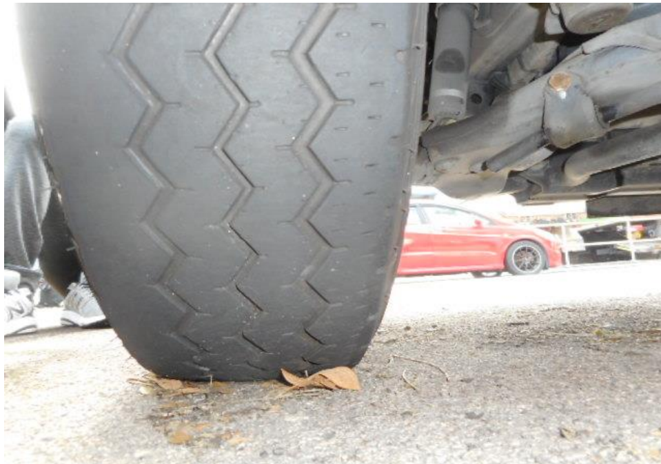
Photo 11 shows the condition of the rear right tyres of the Motor Lorry, which were observed to be in serviceable condition with remaining, tread depth of approximately 3.9mm. There was also no tear, cut or burst mark(s) on the outer and the inner sidewalls as well as across the tread of the 6 tyres that were fitted on the Motor Lorry.
