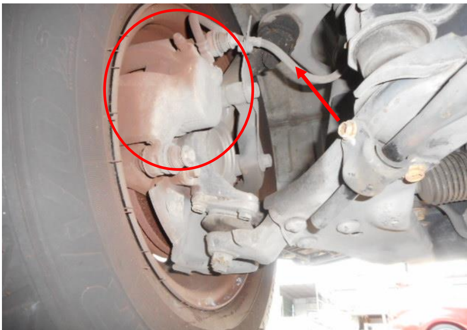
Photo 23 shows the brake hose/pipe (arrowed) at the front left wheel of the Motor Lorry. No leakage of brake fluid was observed. Visual examination of the various components of the braking system like the brake caliper (circled), brake booster, brake pedal etc had revealed all to be intact and without visible damage at the time of accident. There was also no sign of fluid stain(s) observed on the various undercarriage components.
