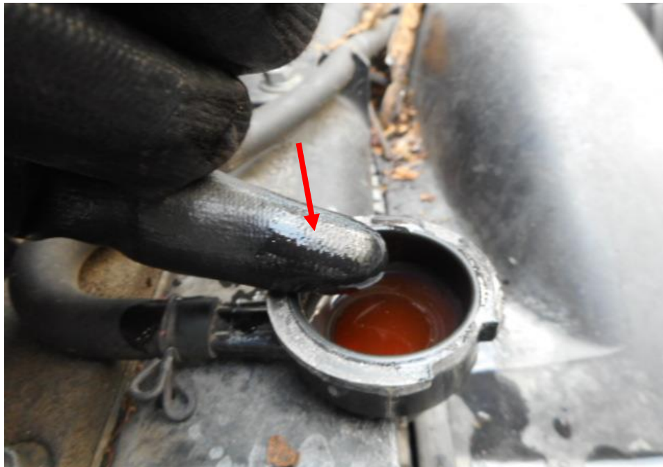
Photo 14 shows the engine coolant of the Motor Lorry at the time of my inspection. The engine coolant was observed to be of insufficient level.
