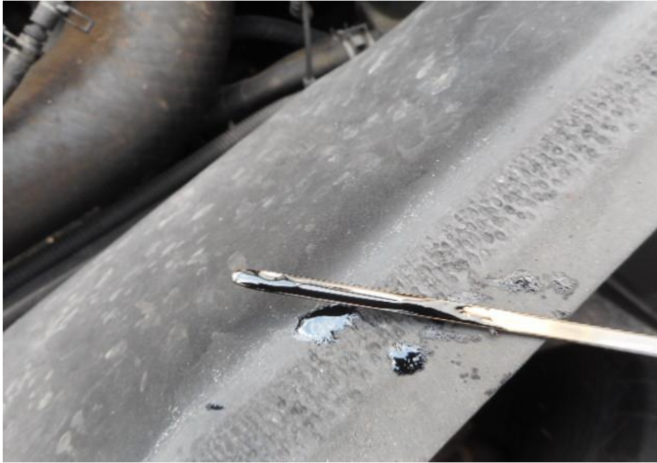
Photo 15 shows the engine oil dip stick of the Motor Lorry at the time of my inspection. The engine oil was observed to be of sufficient level and without any visible contamination.
