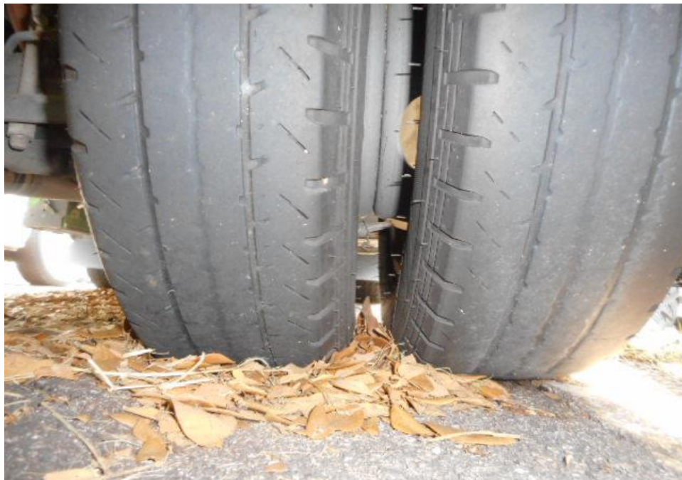
Photo 9 shows the condition of the rear right tyre of the Motor Lorry, which was observed to be in serviceable condition with remaining tread depth of approximately 1.6mm. The tyre, which was wrapped around standard steel wheel rim, it was observed to be sufficiently inflated for vehicular operation.
