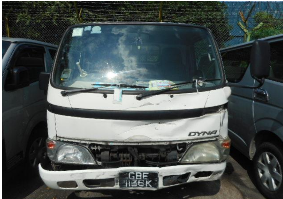
Photo 2 shows a general view of the Motor Lorry's frontal portion at the time of my inspection. It appeared to have sustained damage at its frontal portion. Its front body panel, front grille and front bumper was damaged at the time of my inspection as a result of the accident.
