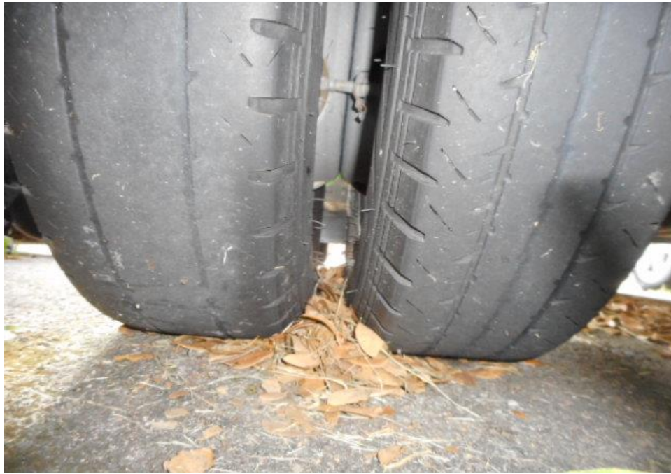
Photo 10 shows the condition of the rear left tyres of the Motor Lorry, which was observed to be in serviceable condition with remaining tread depth of approximately 1.6mm. The tyres, which were wrapped around standard steel wheel rim, were also observed to be sufficiently inflated for vehicular operation. There was also no damage found on all 6 steel wheel rims of the Motor Lorry.
