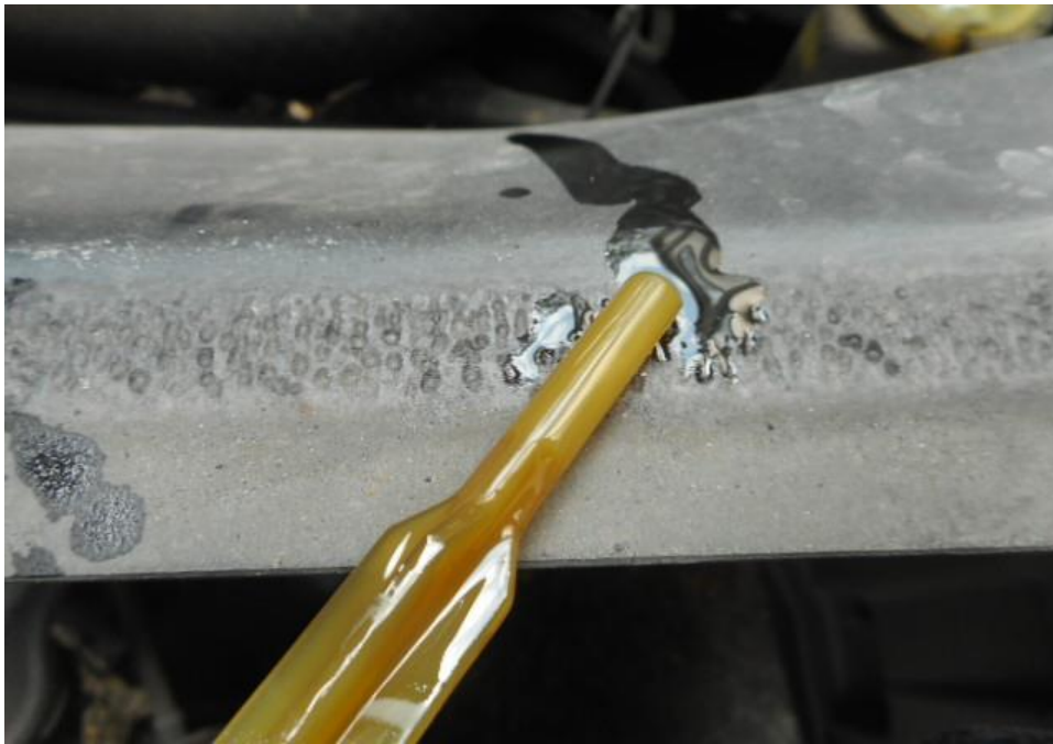
Photo 16 shows the power steering fluid dip stick of the Motor Lorry at the time of my inspection. The power steering fluid was observed to be of sufficient level and without any visible contamination.
