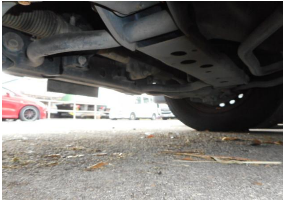
Photo 17 shows the undercarriage of the Motor Lorry, at the area where the engine housing and transmission housing are located at. We did not observe any leak and/or fluid stain(s) on the underside of the Motor Lorry.
