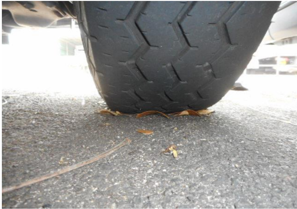
Photo 8 shows the condition of the front right tyre of the Motor Lorry, which was observed to be in serviceable condition with remaining tread depth of approximately 5mm. The tyre, which was wrapped around standard steel wheel rim, was also observed to be sufficiently inflated for vehicular operation. There was no tear, cut or burst mark(s) on the outer and the inner sidewalls as well as across the tread of the 6 tyres that were fitted on the Motor Lorry.
