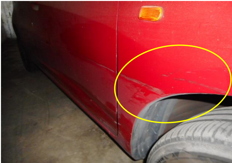
Photo 5 shows a close up view of the Motor Car's right body at the time of my inspection. The right portion of the Motor Car was observed to have sustained damage. Its right fender (circled) was the body parts that were damaged as a result of the accident.
