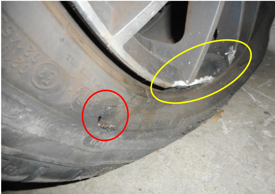
Photo 10 shows the condition of the front right tyre of the Motor Car, which was observed to be in unserviceable condition. The tyre was observed with cut mark on the outer sidewalls (red circle) and the rim was damaged (yellow circle) as a result of the accident.
