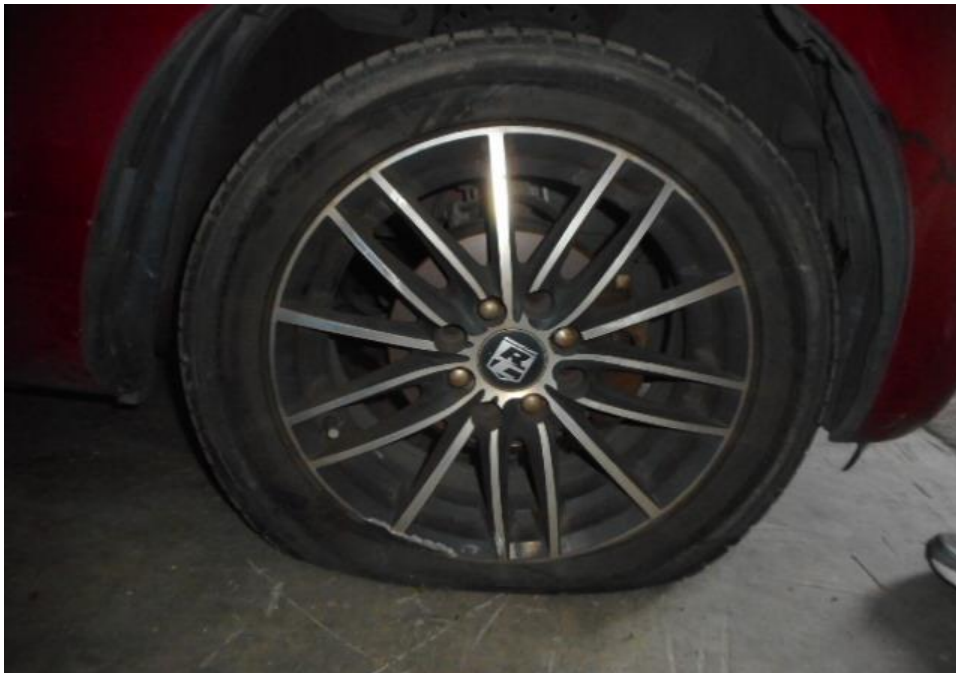
Photo 9 shows the condition of the front right tyre of the Motor Car, which was observed to be in unserviceable condition with remaining tread depth of approximately 4.4mm. The tyre was observed with cut mark on the outer sidewalls and the rim was damaged as a result of the accident.
