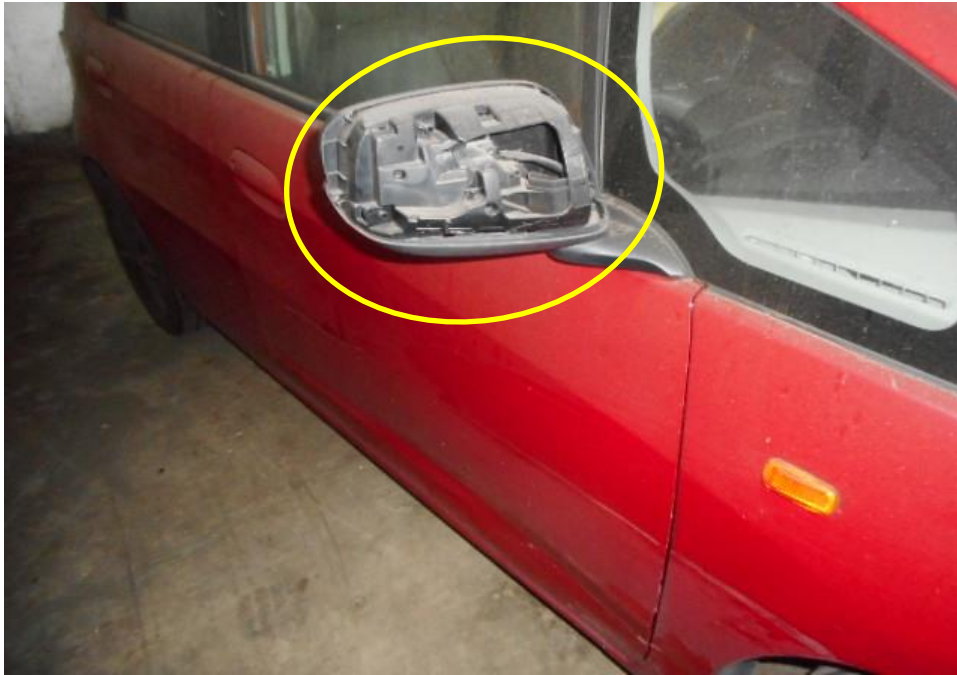
Photo 4 shows a close up view of the Motor Car's right body at the time of my inspection. The right portion of the Motor Car was observed to have sustained damage. Its right rear view mirror (circled) was the body parts that were damaged as a result of the accident.
