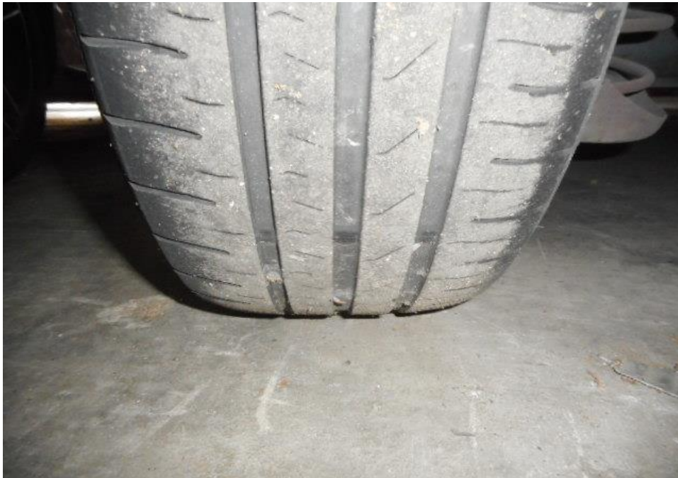
Photo 12 shows the condition of the rear left tyre of the Motor Car, which was observed to be in serviceable condition with remaining tread depth of approximately 2.7mm. The tyre, which was wrapped around steel wheel rim, was also observed to be sufficiently inflated for vehicular operation. The 4 tyres of the Motor Car were wrapped around standard steel wheel rims.
