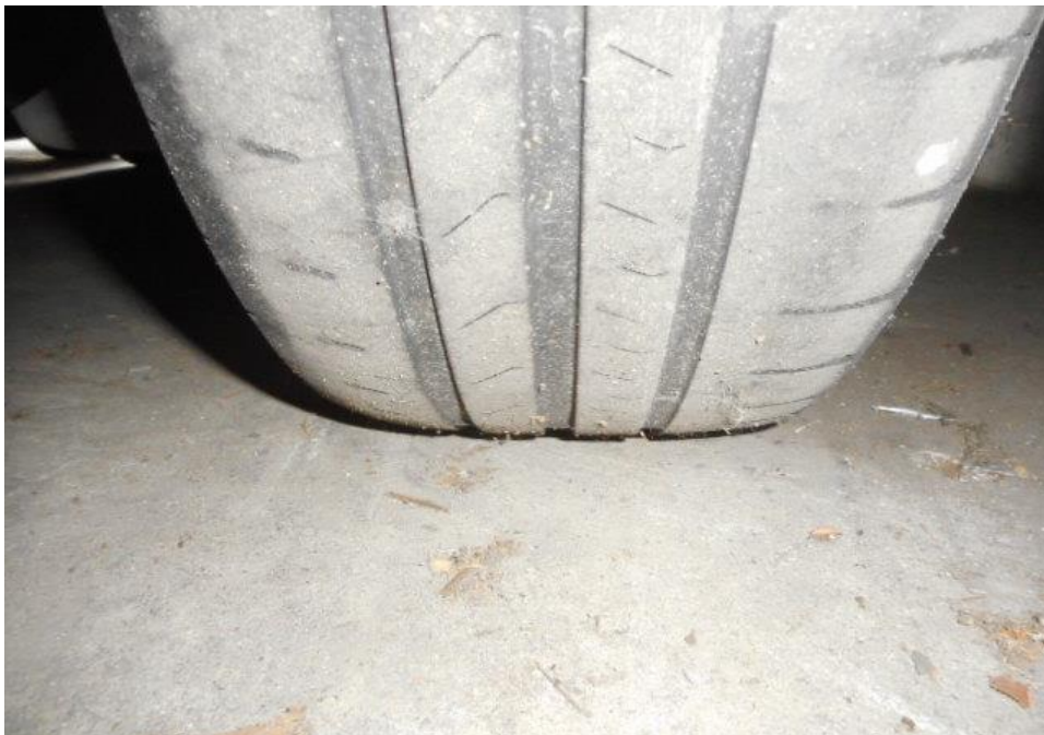
Photo 11 shows the condition of the rear right tyre of the Motor Car, which was observed to be in serviceable condition with remaining tread depth of approximately 2.7mm. The tyre was also observed to be sufficiently inflated for vehicular operation with no tear, cut or burst mark(s).
