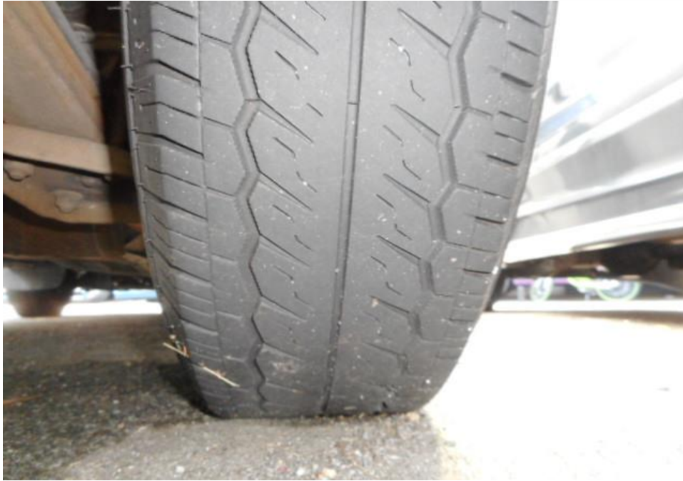
Photo 8 shows the condition of the rear right tyre of the Motor Van, which was observed to be in serviceable condition with remaining tread depth of approximately 3.3mm. The tyre, which was wrapped around standard steel wheel rim, it was observed to be sufficiently inflated for vehicular operation.
