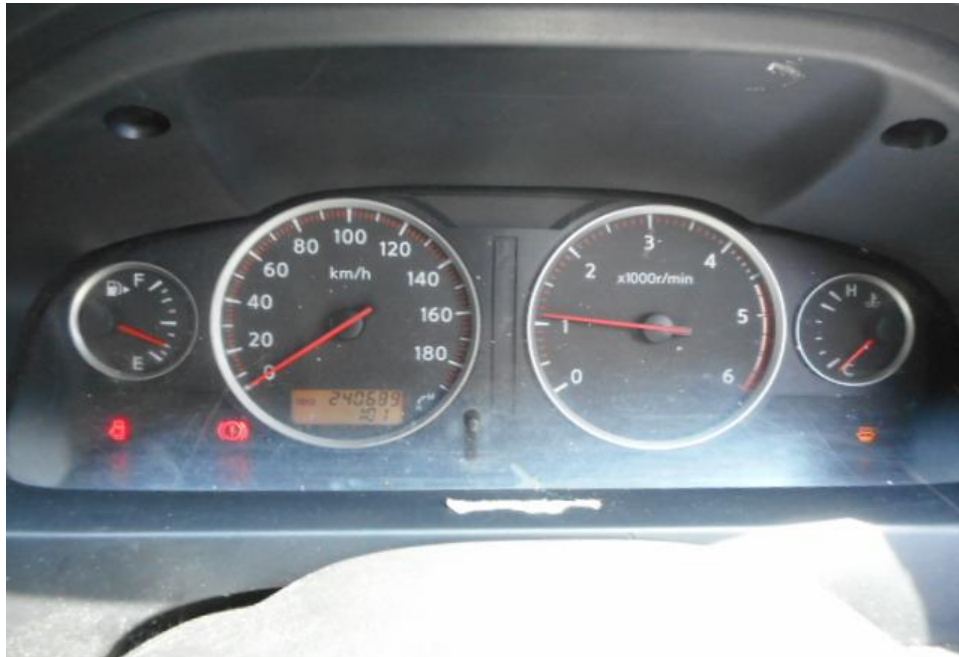
Photo 24 shows no warning lights illuminated on the instrument panel of the Motor Van after the engine was cranked. This would suggest that there was no abnormality to the electronic operating system of the Motor Van, like the ABS, SRS and etc.
