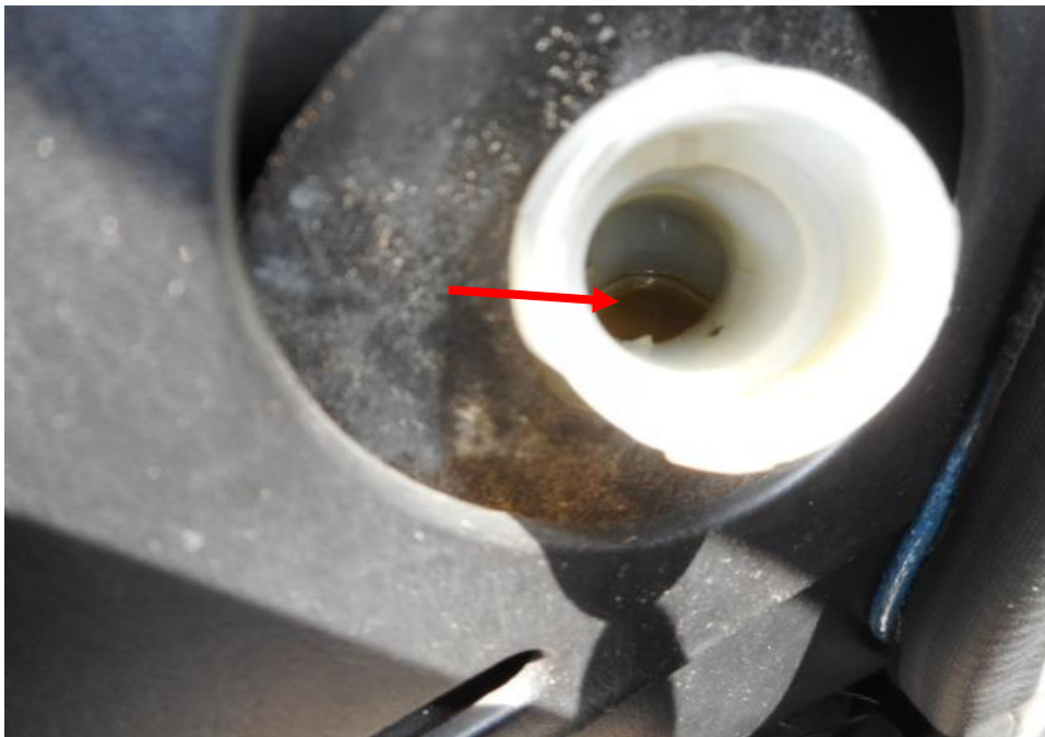
Photo 12 shows the brake fluid reservoir of the Motor Van at the time of my inspection. The brake fluid was observed to be of sufficient level (arrowed) and without any visible contamination.
