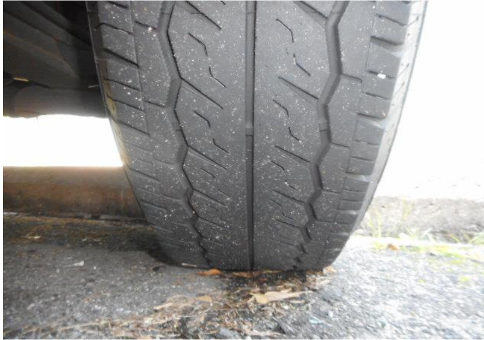
Photo 10 shows the condition of the rear right tyres of the Motor Van, which were observed to be in serviceable condition with remaining, tread depth of approximately 3mm. There was also no tear, cut or burst mark(s) on the outer and the inner sidewalls as well as across the tread of the 4 tyres that were fitted on the Motor Van.
