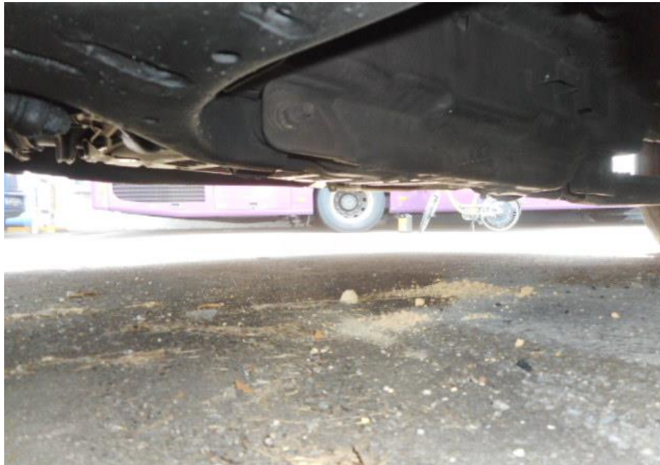
Photo 15 shows the undercarriage of the Motor Van, at the area where the engine housing and transmission housing are located at. We did not observe any leak and/or fluid stain(s) on the underside of the Motor Van.
