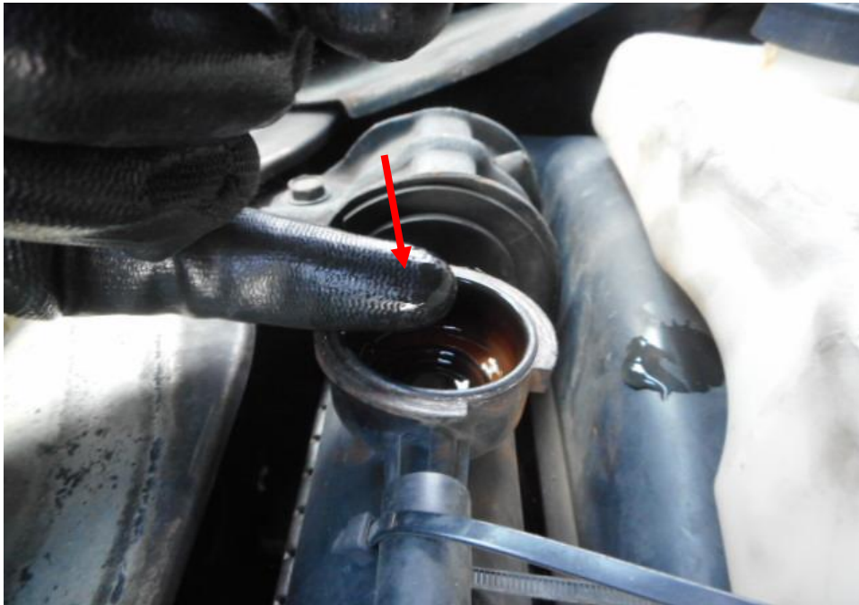
Photo 13 shows the engine coolant of the Motor Van at the time of my inspection. The engine coolant was observed to be of insufficient level.
