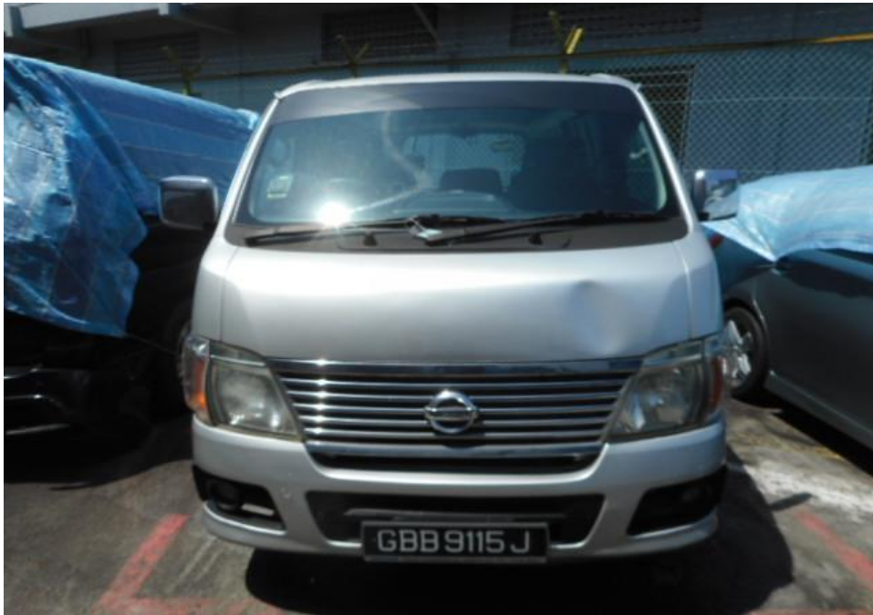
Photo 2 shows a general view of the Motor Van's frontal portion at the time of my inspection. It appeared to have sustained damage at its frontal portion. Its front body panel was damaged at the time of my inspection as a result of the accident.
