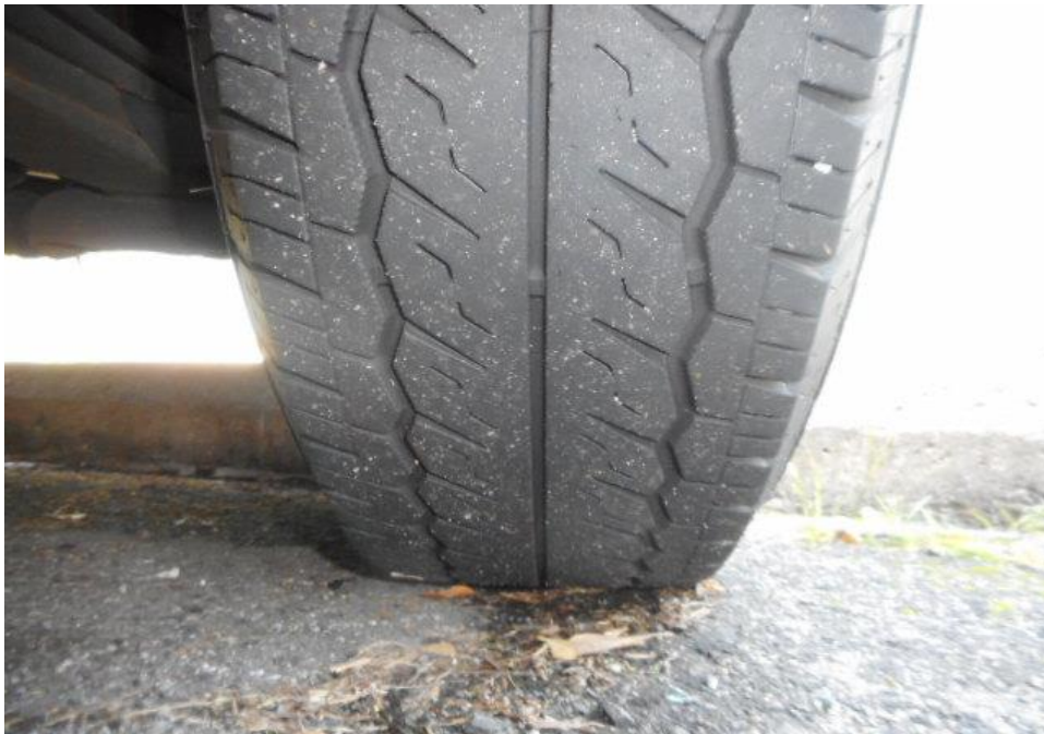
Photo 9 shows the condition of the rear left tyres of the Motor Van, which was observed to be in serviceable condition with remaining tread depth of approximately 2.7mm. The tyres, which were wrapped around standard steel wheel rim, were also observed to be sufficiently inflated for vehicular operation. There was also no damage found on all 4 steel wheel rims of the Motor Van.
