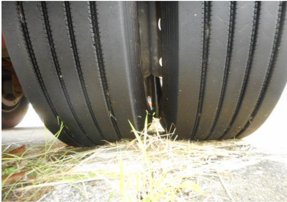
Photo 14 shows the condition of the right tyres of the trailer, which was observed to be in serviceable condition with remaining tread depth of approximately 10.5mm. There was also no tear, cut or burst mark(s) on the outer and the inner sidewalls as well as across the tread of the 8 tyres that were fitted on the trailer.
