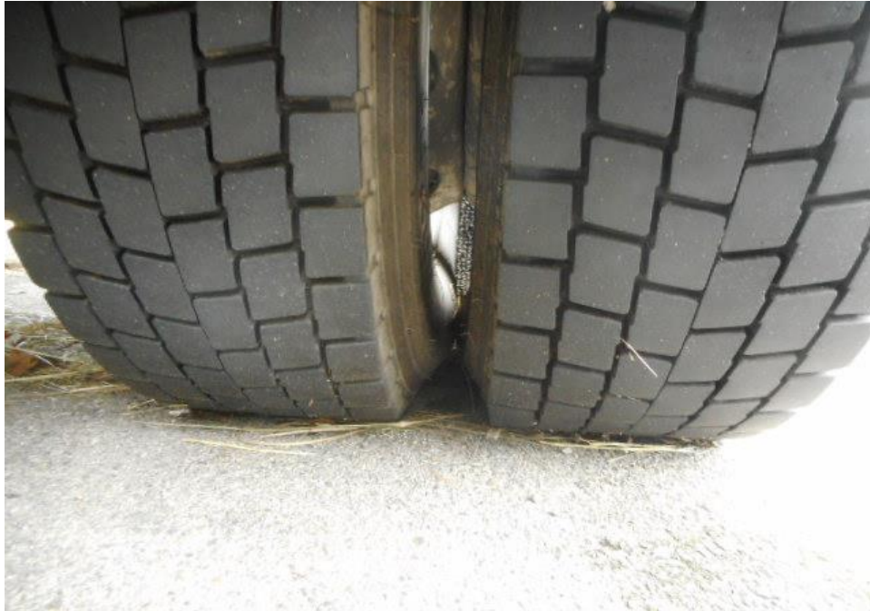
Photo 12 shows the condition of the rear left tyres of the Malaysian Trailer, which was observed to be in serviceable condition with remaining tread depth of approximately 13.8mm. The tyres, which were wrapped around standard steel wheel rim, were also observed to be sufficiently inflated for vehicular operation. There was also no damage found on all 6 steel wheel rims of the Malaysian Trailer.
