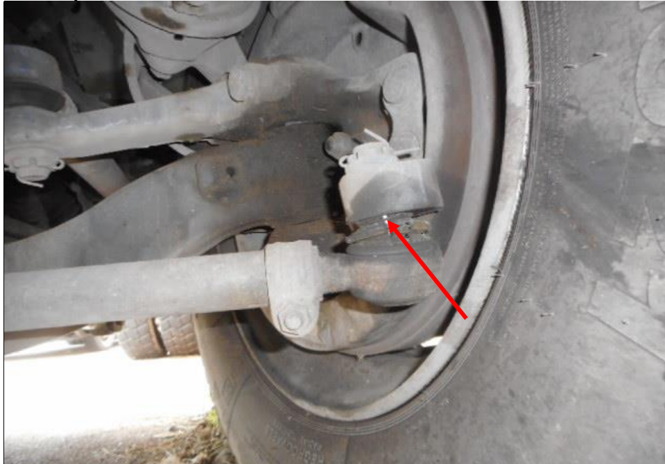
Photo 27 shows the various undercarriage components at the front right wheel of the Malaysian Trailer, in particular the steering tie rod end (arrowed). The various steering components were all found to be intact, suggesting that the steering system of the Malaysian Trailer was likely to be in serviceable condition at the material time of accident. There was also no sign of fluid stain(s) observed on the various undercarriage components.
