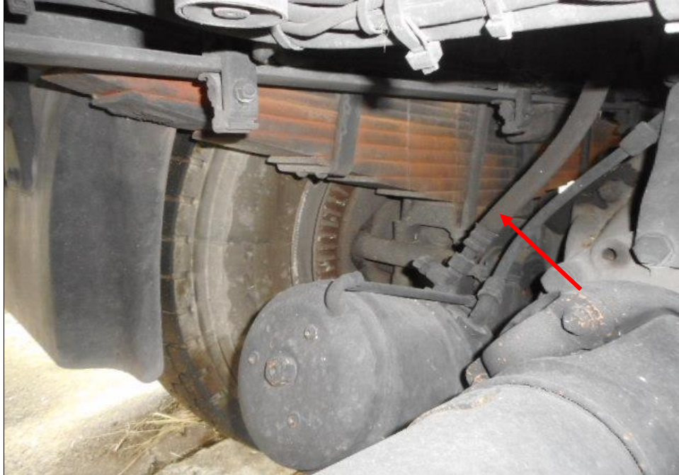
Photo 22 shows the brake pipe (arrowed) at the rear right wheel of the Malaysian Trailer. I did not observe any leakage of brake fluid at the time of my inspection of the Malaysian Trailer. My static tests of the Malaysian Trailer's braking system, along with my visual examination of the various mechanical components in the braking system, had indicated that there was no internal leakage of pressure/vacuum. Hence the braking system of the Malaysian Trailer was likely to be in serviceable condition at the material time of accident.
