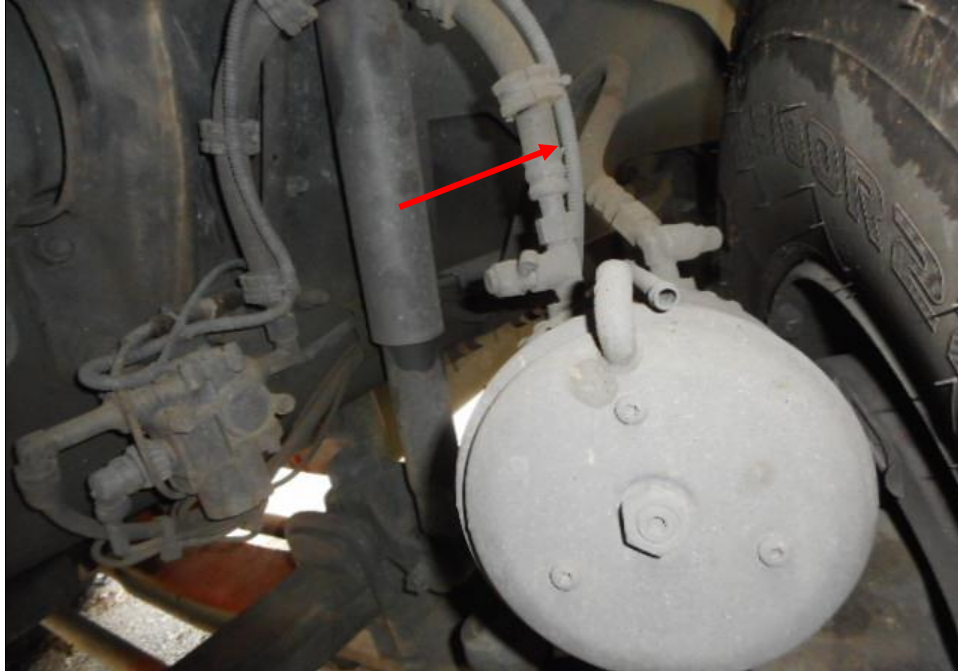
Photo 24 shows the brake pipe (arrowed) at the front right wheel of the Malaysian Trailer. I did not observe any leakage of brake fluid at the time of my inspection of the Malaysian Trailer. My static tests of the Malaysian Trailer's braking system, along with my visual examination of the various mechanical components in the braking system, had indicated that there was no internal leakage of pressure/vacuum. Hence the braking system of the Malaysian Trailer was likely to be in serviceable condition at the material time of accident.
