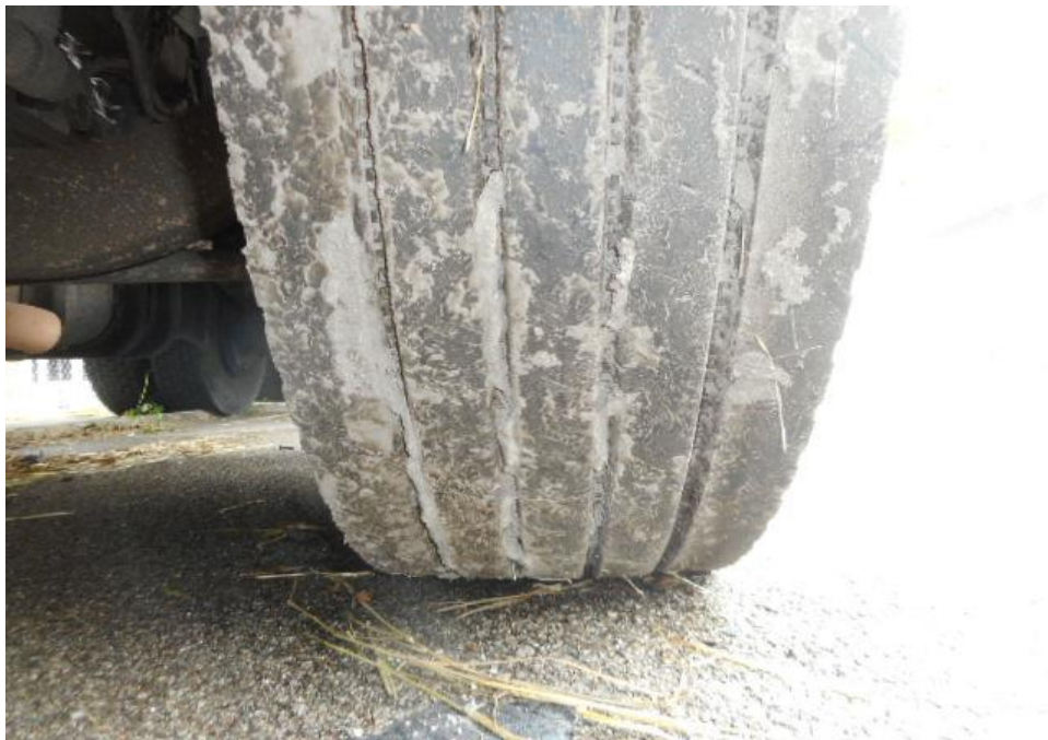
Photo 13 shows the condition of the front left tyres of the Malaysian Trailer, which were observed to be in serviceable condition with remaining tread depth of approximately 11.9mm. There was also no tear, cut or burst mark(s) on the outer and the inner sidewalls as well as across the tread of the 6 tyres that were fitted on the Malaysian Trailer.
