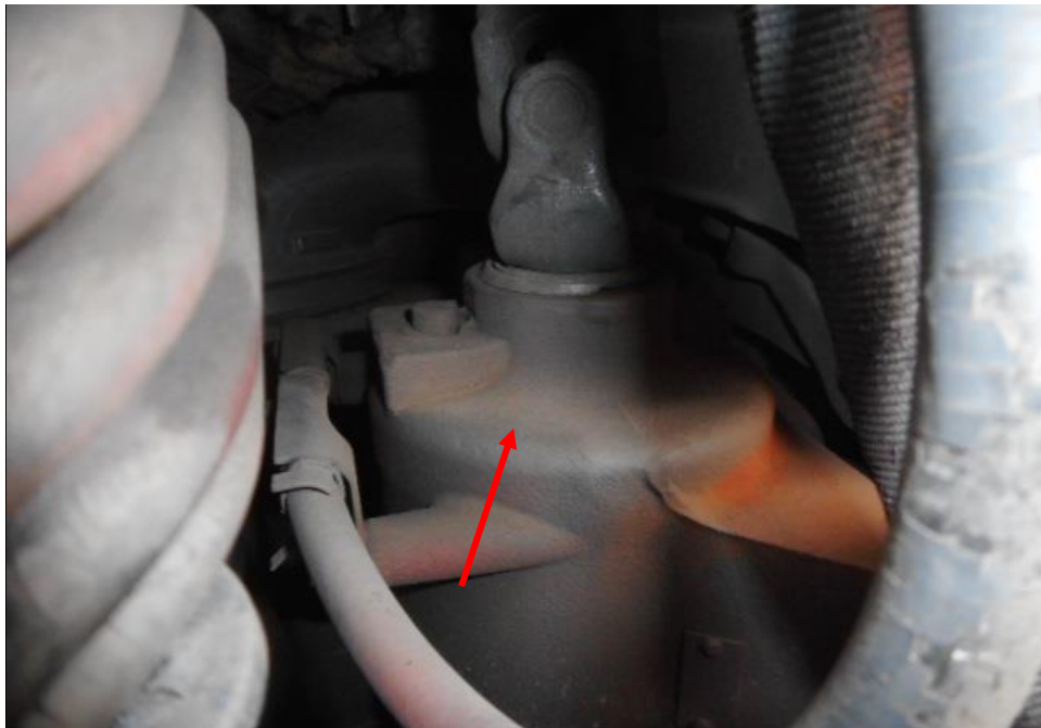
Photo 29 shows the steering box component (arrowed) at the undercarriage of the Malaysian Trailer was found to be intact without any visible damage. There was also no sign of fluid stain(s) observed on the various undercarriage components.
