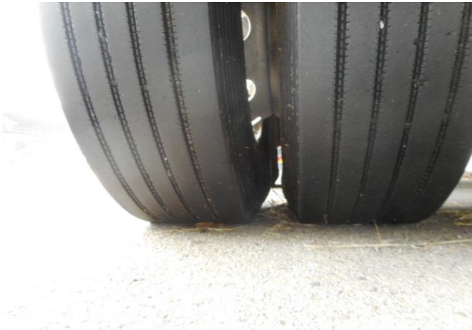
Photo 15 shows the condition of the left tyres of the trailer, which was observed to be in serviceable condition with remaining tread depth of approximately 5.9mm. There was also no tear, cut or burst mark(s) on the outer and the inner sidewalls as well as across the tread of the 8 tyres that were fitted on the trailer.
