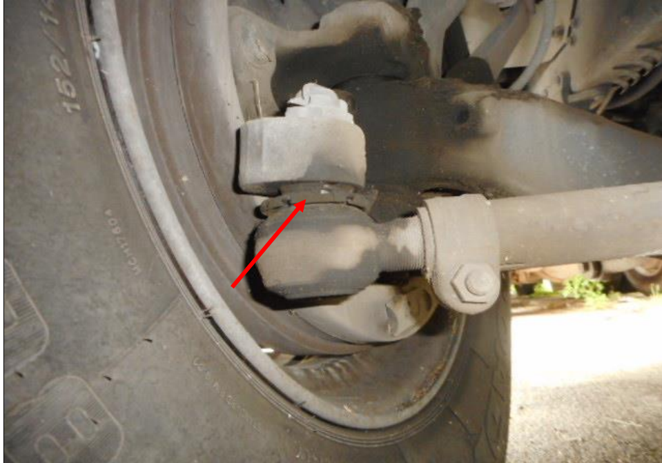
Photo 28 shows the various undercarriage components at the front left wheel of the Malaysian Trailer, in particular the steering tie rod end (arrowed). The various undercarriage components of the Malaysian Trailer were all found to be intact without any visible damage. There was also no sign of fluid stain(s) observed on the various undercarriage components.
