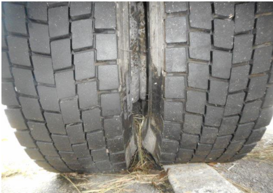
Photo 11 shows the condition of the rear right tyre of the Malaysian Trailer, which was observed to be in serviceable condition with remaining tread depth of approximately 10.9mm. The tyre, which was wrapped around standard steel wheel rim, was also observed to be sufficiently inflated for vehicular operation.
