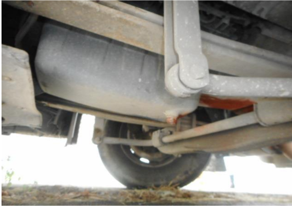
Photo 21 shows the undercarriage of the Malaysian Trailer, at the area where the engine housing located. I did not find any sign(s) or indication(s) of fluid leak, however old fluid stain(s) was observed on the underside of the Malaysian Trailer.
