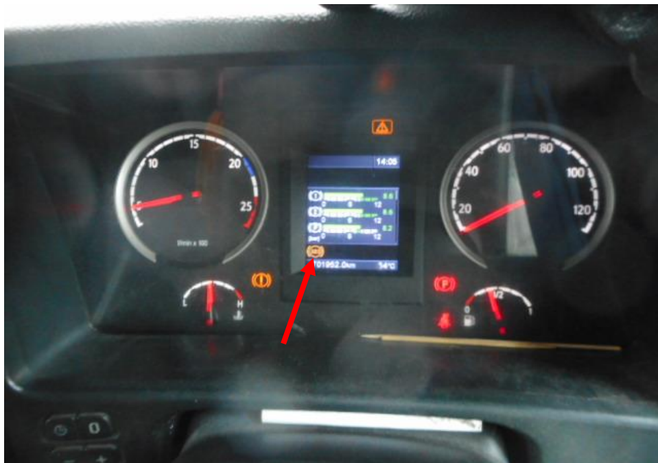
Photo 32 shows the Anti-Lock Brake System (ABS) (arrowed) warning lights illuminated on the instrument panel of the Malaysian Trailer after the engine was cranked. However, there was no abnormalities to the braking system during our operational test.
