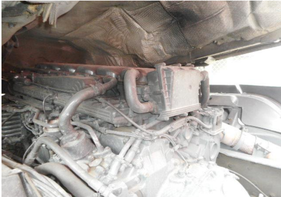
Photo 16 shows a general view of the Malaysian Trailer's engine compartment, which was accessed by lifting the front cabin of the Malaysian Trailer. The various parts and components inside the engine compartment were unaffected by the accident. There was also no sign(s) or indication(s) of fresh fluid leakage and/or fluid stain within the engine compartment
