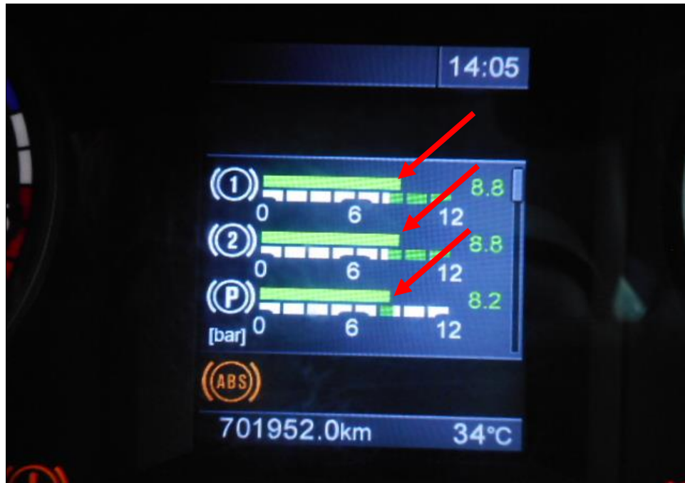
Photo 17 shows the air in the air brake cylinders of the Malaysian Trailer at the time of my inspection. The air in the cylinder was observed to be of sufficient level & serviceable at the time of the accident.
