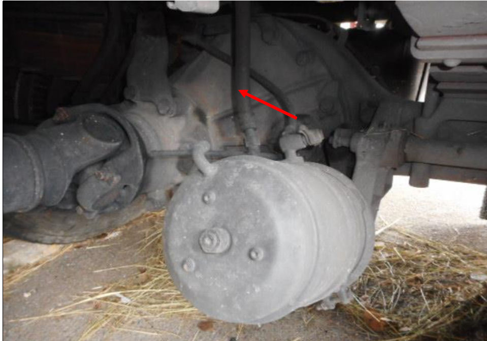
Photo 23 shows the brake pipe (arrowed) at the rear left wheel of the Malaysian Trailer. I did not observe any leakage of brake fluid at the time of my inspection of the Malaysian Trailer. My static tests of the Malaysian Trailer's braking system, along with my visual examination of the various mechanical components in the braking system, had indicated that there was no internal leakage of pressure/vacuum. Hence the braking system of the Malaysian Trailer was likely to be in serviceable condition at the material time of accident.
