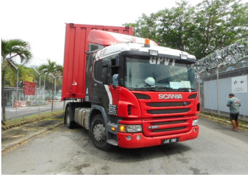
Photo 30 shows the front right wheel of the Malaysian Trailer turned to its full left. During my steering system test, I did not experience any abnormal free play and/or resistance when I had turned the steering wheel towards full left and full right. This would suggest that the steering system of the Malaysian Trailer was likely to be in serviceable condition at the material time of accident.
