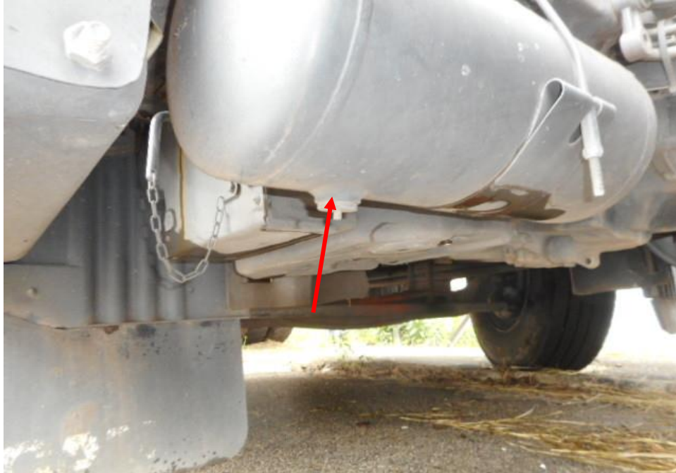
Photo 26 shows the air brake cylinders (arrowed) at the undercarriage of the Malaysian Trailer. I did not observe any leakage of air brake fluid at the time of my inspection of the Malaysian Trailer. My static tests of the Malaysian Trailer's braking system, along with my visual examination of the various mechanical components in the braking system had indicated that there was no internal leakage of pressure/vacuum. Hence the braking system of the Malaysian Trailer was likely to be in serviceable condition at the material time of accident.
