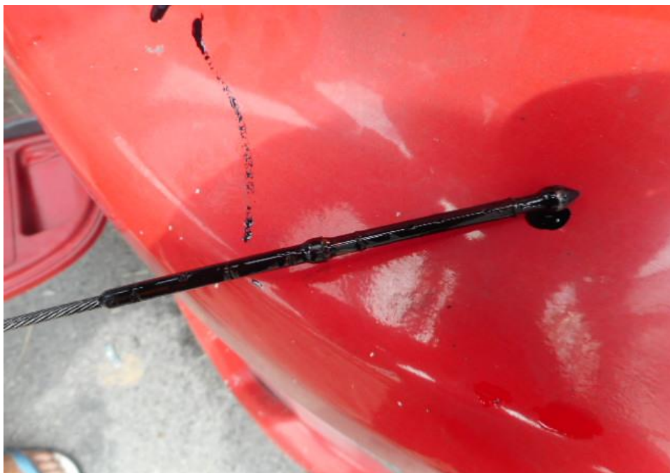
Photo 20 shows the engine oil dip stick of the Malaysian Trailer at the time of my inspection. The engine oil was observed to be of insufficient level at the time of our inspection.
