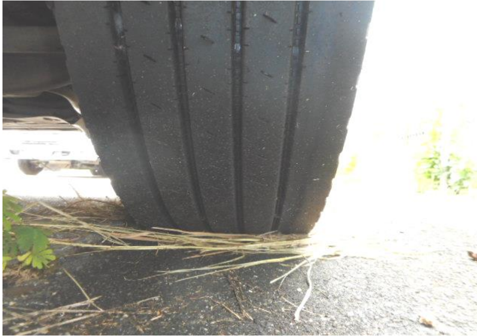
Photo 10 shows the condition of the front right tyre of the Malaysian Trailer, which was observed to be in serviceable condition with remaining tread depth of approximately 9mm. The tyre, which was wrapped around standard steel wheel rim, was also observed to be sufficiently inflated for vehicular operation. There was no tear, cut or burst mark(s) on the outer and the inner sidewalls as well as across the tread of the 6 tyres that were fitted on the Malaysian Trailer.
