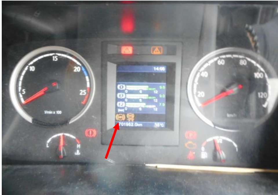
Photo 31 shows the warning light for Anti-Lock Brake System (ABS) (arrowed) appearing on the instrument panel of the Malaysian Trailer during the self-test of its various electronic operating systems when its engine was cranked.
