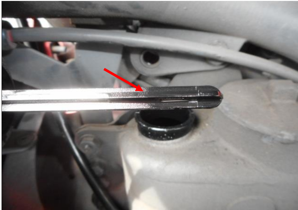
Photo 19 shows the power steering fluid reservoir of the Malaysian Trailer at the time of my inspection. The power steering fluid was observed to be of sufficient level (arrowed) and without any visible contamination.
