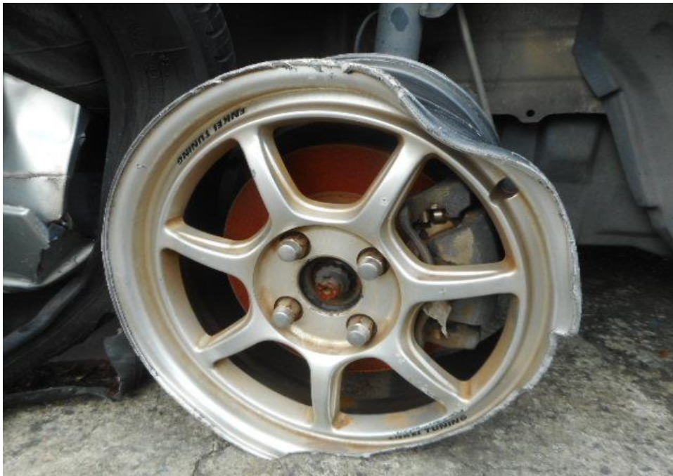
Photo 10 shows the close up condition of the front right wheel rim of the Motor Car, which was observed to be damaged as a result of the accident
