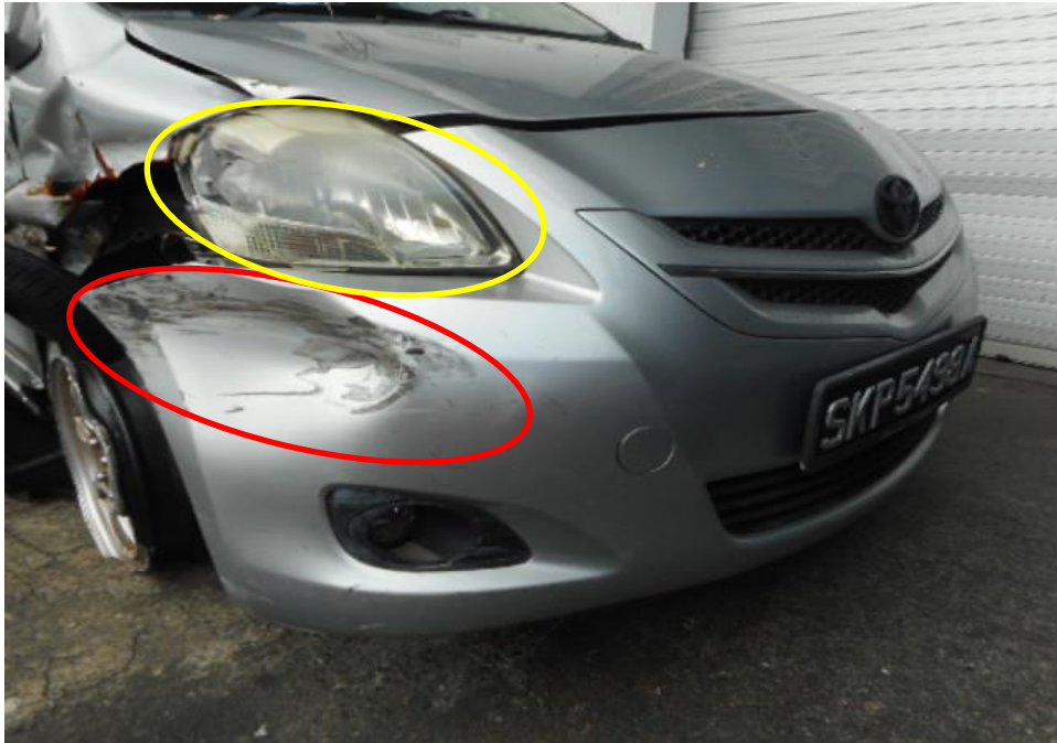
Photo 3 shows the close up view of the Motor Car's front body at the time of my inspection. The Motor car was observed to have sustained damage at its front portion. Its front bumper (red circle) and its front right headlamp (yellow circle) was damaged as a result of the accident.
