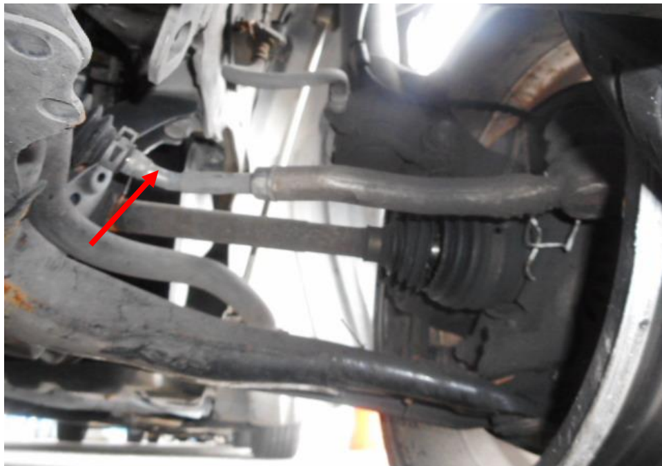
Photo 24 shows the various undercarriage components at the front left wheel of the Motor Car, in particular the steering tie rod was observed to be damaged as a result of the accident (arrowed).
