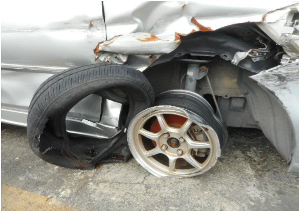
Photo 9 shows the condition of the front right tyre and wheel rim of the Motor Car, which was observed to be damaged and deflated as a result of the accident with remaining tread depth of approximately 3.8mm.
