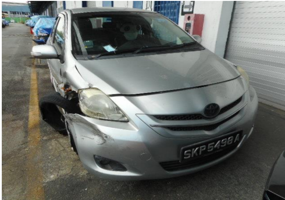
Photo 2 shows a general view of the Motor Car's front body at the time of my inspection. The Motor car was observed to have sustained damage at its front and right portion. Its front bonnet, front bumper, front right fender, front right headlamp and right doors was amongst the body parts that were damaged as a result of the accident. The Supplemental Restraint System (SRS) was activated as a result of the accident.
