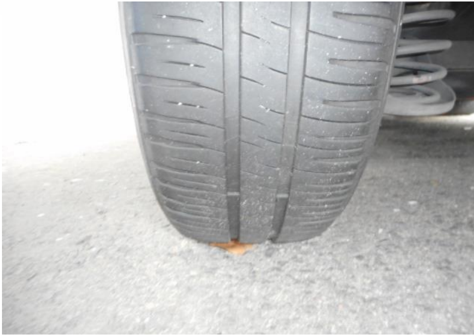
Photo 13 shows the condition of the rear left tyre of the Motor Car, which was observed to be in serviceable condition with remaining tread depth of approximately 4.4mm. The tyre was also observed to be sufficiently inflated for vehicular operation with no tear, cut or burst mark(s).
