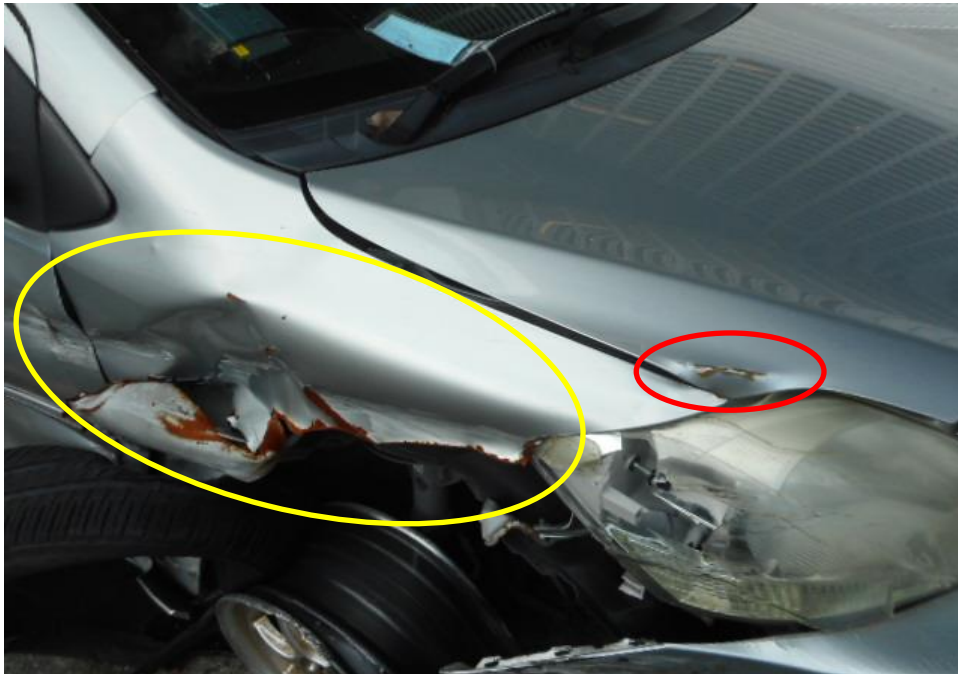
Photo 4 shows the close up view of the Motor Car's front body at the time of my inspection. The Motor car was observed to have sustained damage at its front portion. Its front bonnet (red circle) and its front right fender (yellow circle) was damaged as a result of the accident.
