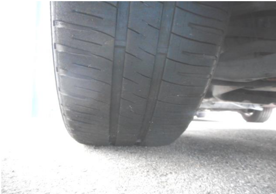
Photo 14 shows the condition of the front left tyre of the Motor Car, which was observed to be in serviceable condition with remaining tread depth of approximately 3.2mm. The tyre was also observed to be sufficiently inflated for vehicular operation with no tear, cut or burst mark(s).
