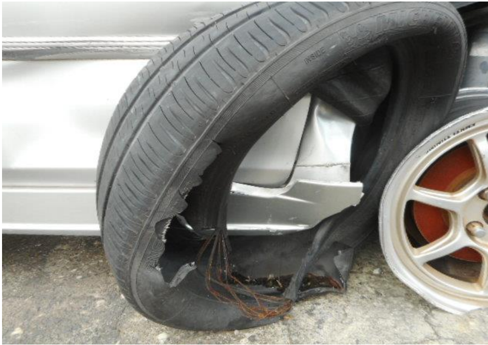
Photo 11 shows the close up condition of the front right wheel rim of the Motor Car, which was observed to be damaged as a result of the accident with remaining tread depth of approximately 3.8mm.
