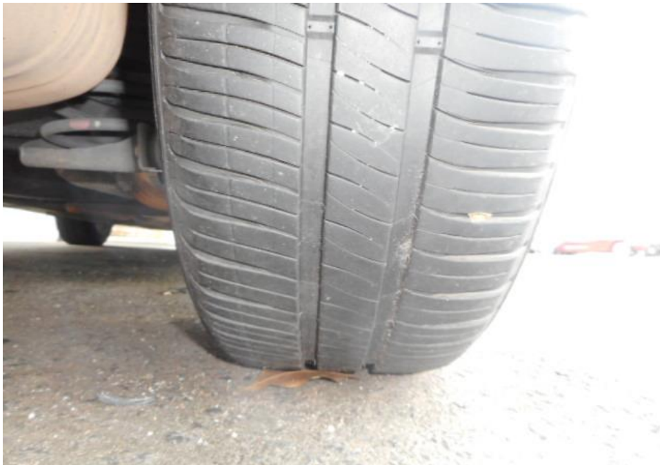
Photo 12 shows the condition of the rear right tyre of the Motor Car, which was observed to be in serviceable condition with remaining tread depth of approximately 5.5m. The tyre was also observed to be sufficiently inflated for vehicular operation with no tear, cut or burst mark(s).
