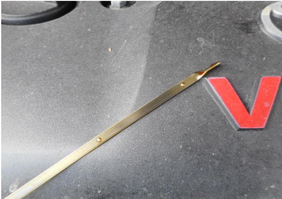
Photo 18 shows the engine oil level dipstick of the Motor Car at the time of my inspection. The engine oil was observed to be of sufficient level and without any visible contamination.
