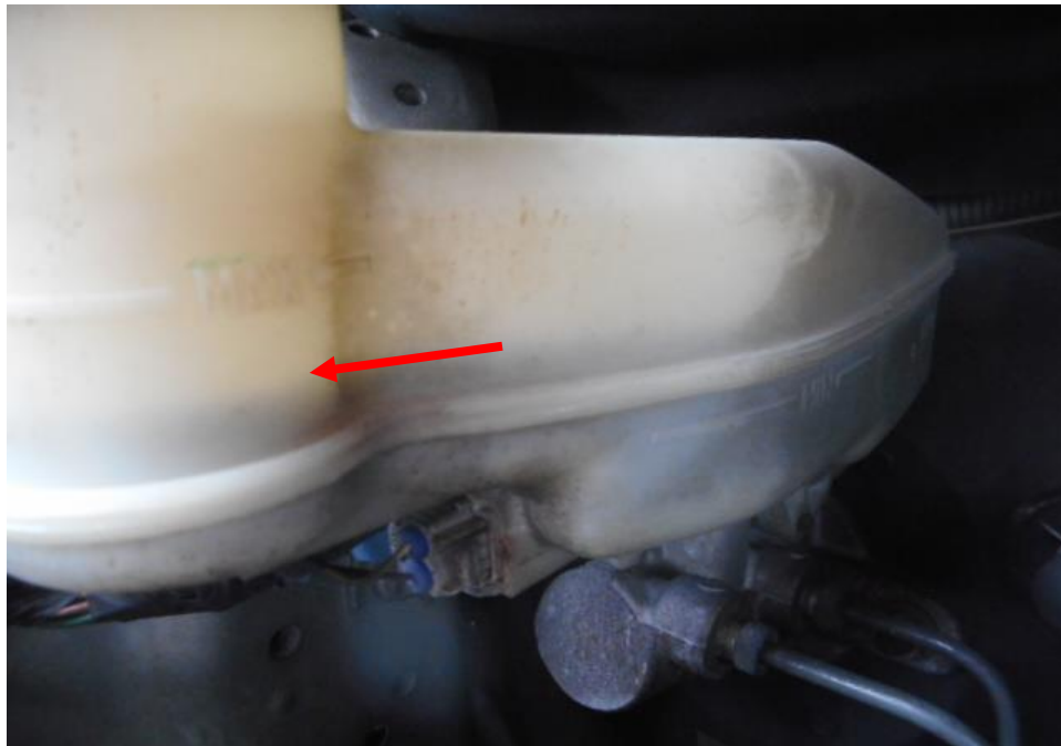
Photo 17 shows the brake fluid reservoir of the Motor Car at the time of my inspection. The brake fluid was observed to be of sufficient level (arrowed) and without any visible contamination.
