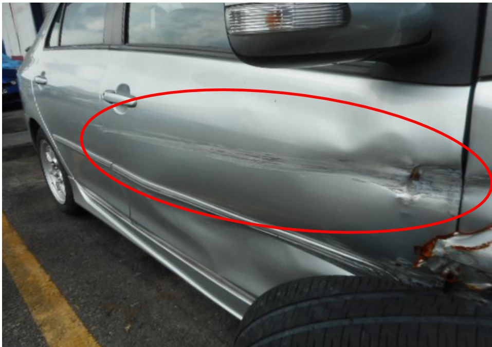
Photo 6 shows a close up view of the Motor Car's right body at the time of my inspection. The Motor car was observed to have sustained damage at its right portion. Its right doors (circled) was damaged as a result of the accident.
