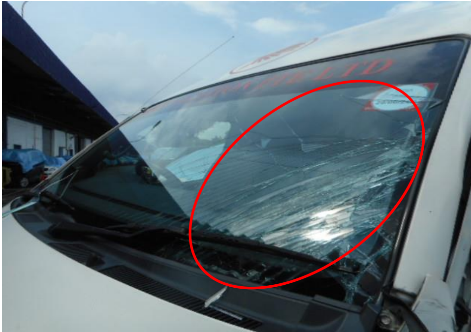
Photo 4 shows a close up view of the Motor Van's frontal portion at the time of my inspection. It appeared to have sustained damage at its frontal portion. Its front windscreen (circled) was damage at the time of my inspection as a result of the accident.
