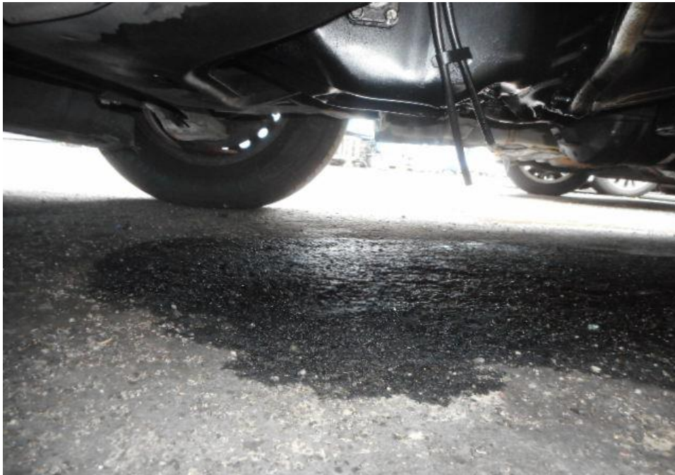
Photo 18 shows the undercarriage of the Motor Van, at the area where the engine housing and transmission housing are located. . We engine oil leak and/or fluid stain(s) on the underside of the Motor Van.
