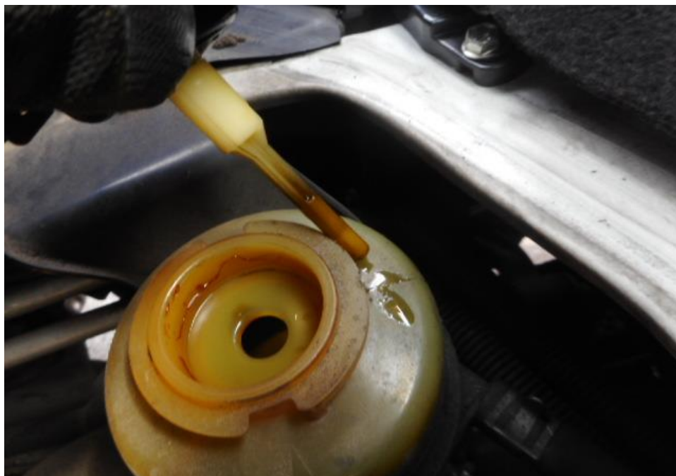
Photo 16 shows the power steering fluid dip stick of the Motor Van at the time of my inspection. The steering fluid was observed to be of sufficient level and without any visible contamination.
