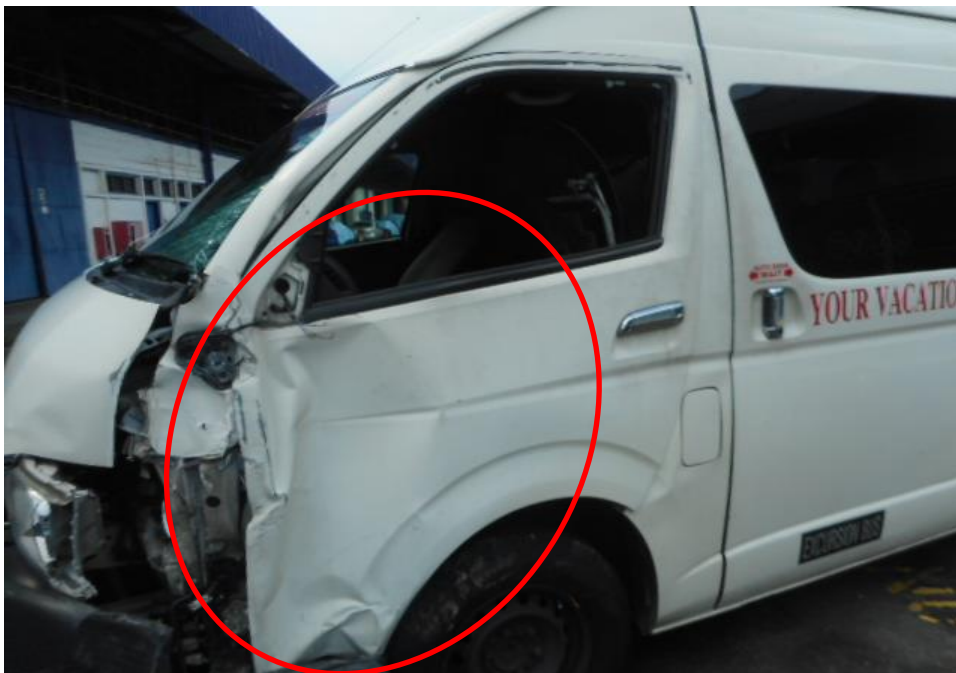
Photo 7 shows a general view of the left body of the Motor Van at the time of my inspection. It appeared to have sustained damage at its left portion. Its front left door (circled) was damage at the time of my inspection as a result of the accident.
