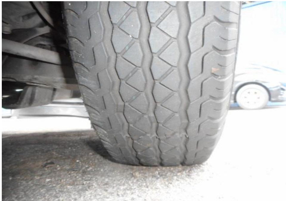
Photo 9 shows the condition of the front right tyre of the Motor Van, which was observed to be in serviceable condition with remaining tread depth of approximately 5.1mm. The tyre, which was wrapped around standard steel wheel rim, was also observed to be sufficiently inflated for vehicular operation. There was no tear, cut or burst mark(s) on the outer and the inner sidewalls as well as across the tread of the 4 tyres that were fitted on the Motor Van.
