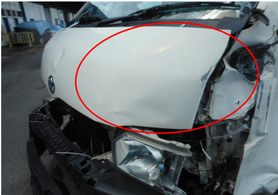
Photo 5 shows a close up view of the Motor Van's frontal portion at the time of my inspection. It appeared to have sustained damage at its frontal portion. Its front body panel (circled) was damage at the time of my inspection as a result of the accident.
