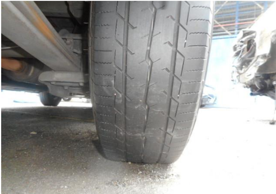
Photo 10 shows the condition of the rear right tyre of the Motor Van, which was observed to be in serviceable condition with remaining tread depth of approximately 2.5mm. The tyre, which was wrapped around standard steel wheel rim, it was observed to be sufficiently inflated for vehicular operation.
