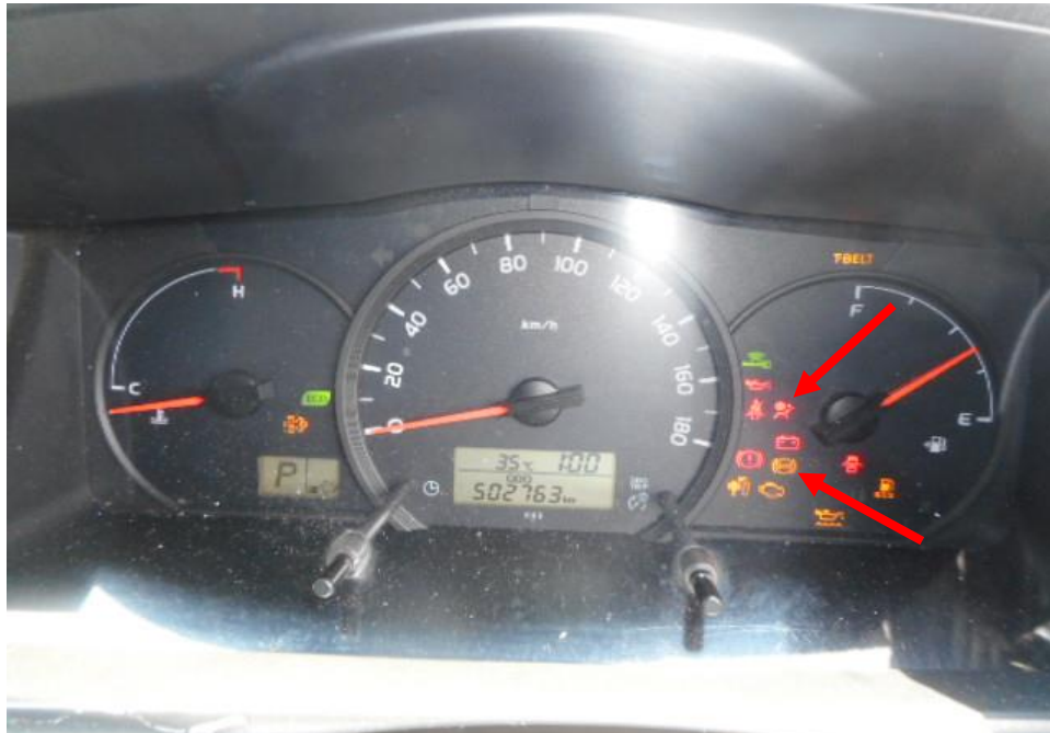
Photo 26 shows the warning light for Anti-Lock Brake System (ABS) and Supplemental Restraint System (SRS) (arrowed) appearing on the instrument panel of the Motor Van during the self-test of its various electronic operating systems when its engine was cranked.
