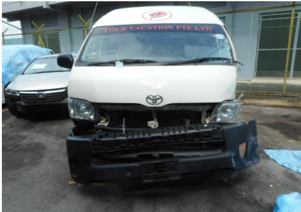
Photo 3 shows a general view of the Motor Van's frontal portion at the time of my inspection. It appeared to have sustained damage at its frontal portion. Its front windscreen, front body panel, front bumper and front left headlamp as well as its front left door was damaged at the time of my inspection as a result of the accident.
