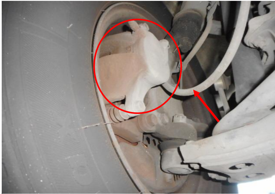
Photo 24 shows the brake hose/pipe (arrowed) at the front left wheel of the Motor Van. No leakage of brake fluid was observed. Visual examination of the various components of the braking system like the brake caliper (circled), brake booster, brake pedal etc had revealed all to be intact and without visible damage at the time of accident. There was also no sign of fluid stain(s) observed on the various undercarriage components.
