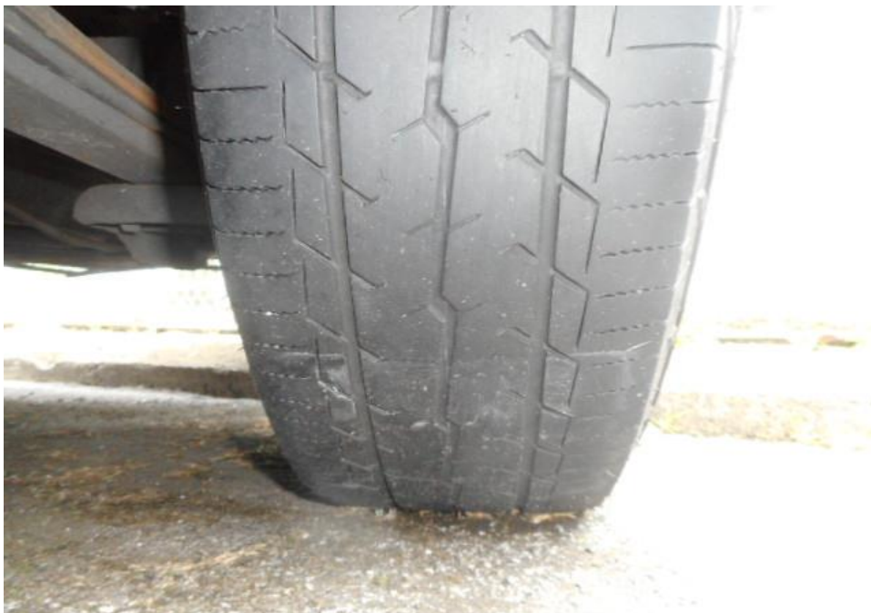
Photo 11 shows the condition of the rear left tyres of the Motor Van, which was observed to be in serviceable condition with remaining tread depth of approximately 2mm. The tyres, which were wrapped around standard steel wheel rim, were also observed to be sufficiently inflated for vehicular operation. There was also no damage found on all 4 steel wheel rims of the Motor Van.
