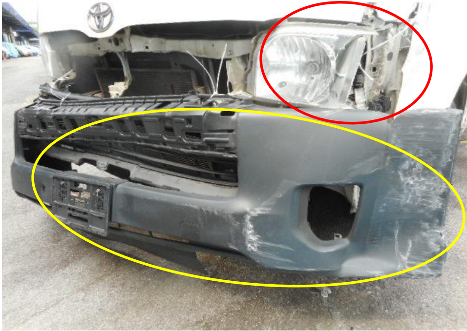
Photo 6 shows a close up view of the Motor Van's frontal portion at the time of my inspection. It appeared to have sustained damage at its frontal portion. Its front bumper (yellow circle) and front left headlamp (red circle) was damage at the time of my inspection as a result of the accident.
