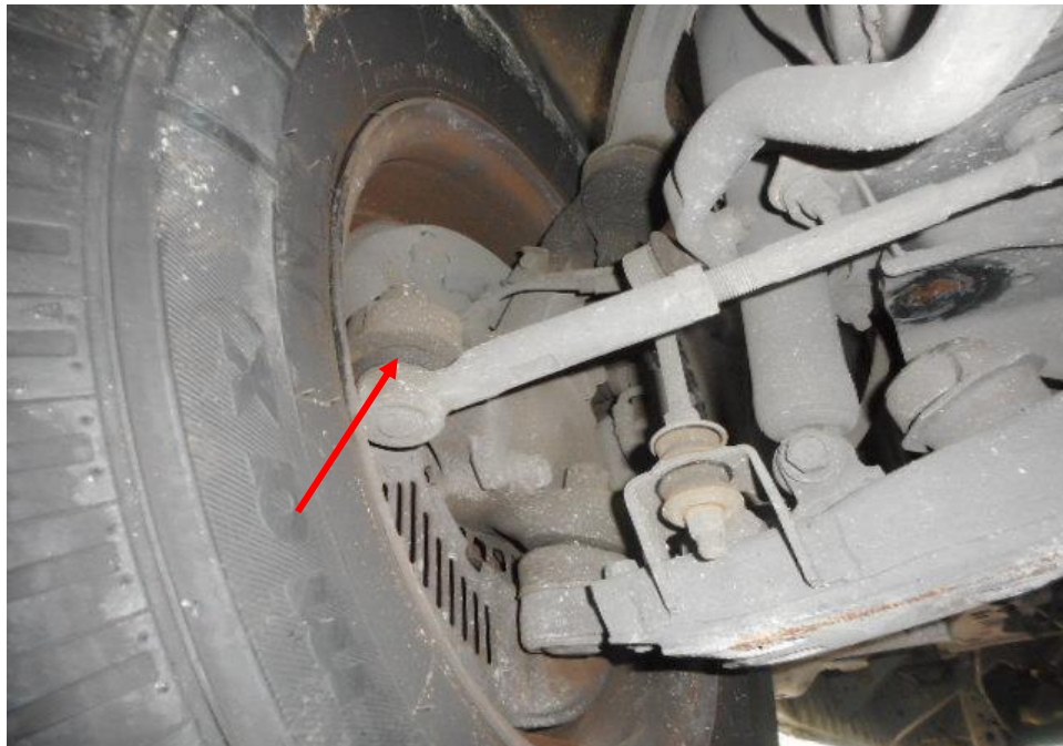
Photo 19 shows the various undercarriage components at the front right wheel of the Motor Van, in particular the steering tie rod end (arrowed). The various steering components were all found to be intact, suggesting that the steering system of the Motor Van was likely to be in serviceable condition at the material time of accident. There was also no sign of fluid stain(s) observed on the various undercarriage components.
