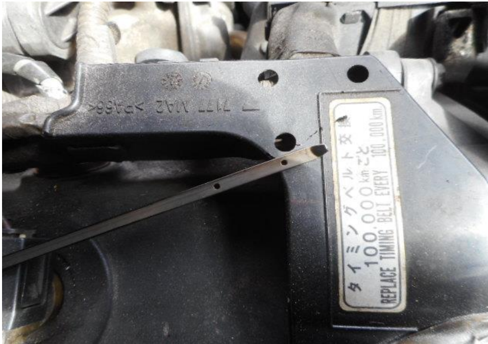
Photo 17 shows the engine oil dip stick of the Motor Van at the time of my inspection. The engine oil was observed to be of insufficient level.
