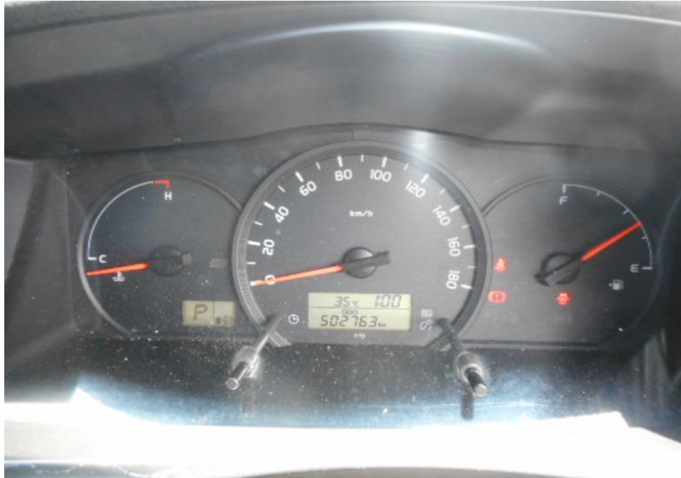
Photo 27 shows no warning lights illuminated on the instrument panel of the Motor Van after the engine was cranked. This would suggest that there was no abnormality to the electronic operating system of the Motor Van, like the ABS, SRS and etc.
