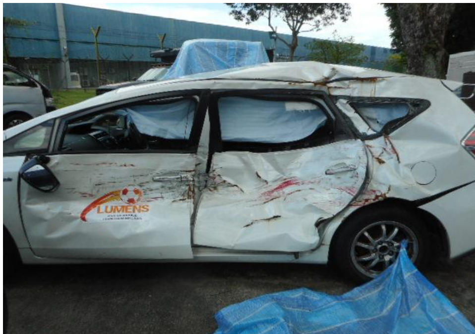
Photo 2 shows a general view of the Motor Car's front body at the time of my inspection. The Motor car was observed to have sustained damage at its left and vehicle chassis portion. Its left doors, left rear view mirror and left vehicle chassis was amongst the body parts damaged as a result of the accident. The Supplemental Restraint System (SRS) was activated as a result of the accident.
