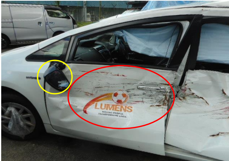
Photo 3 shows the close up view of the Motor Car's left body at the time of my inspection. The Motor car was observed to have sustained damage at its left portion. Its left door (red circle) and its left rear view mirror (yellow circle) was damaged as a result of the accident.
