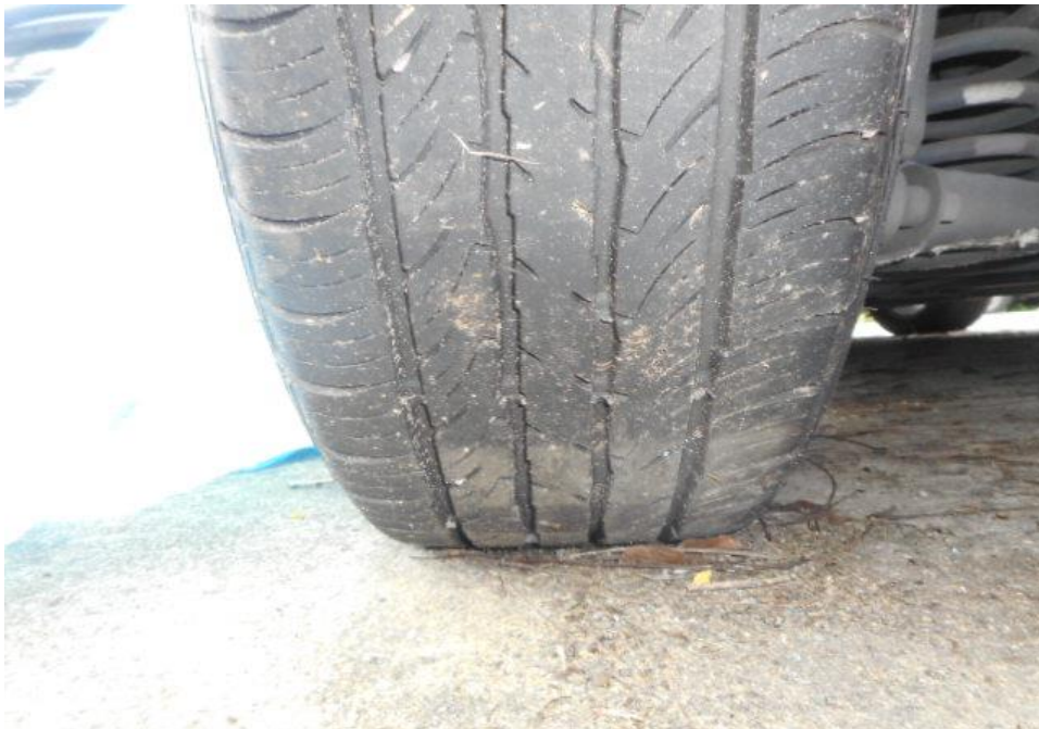
Photo 10 shows the condition of the rear left tyre of the Motor Car, which was observed to be in serviceable condition with remaining tread depth of approximately 5.7m. The tyre was also observed to be sufficiently inflated for vehicular operation with no tear, cut or burst mark(s).
