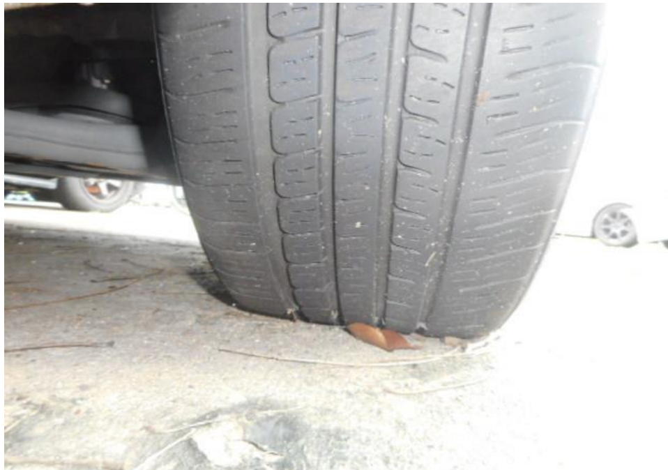
Photo 8 shows the condition of the front right tyre of the Motor Car, which was observed to be in serviceable condition with remaining tread depth of approximately 4.7mm. The tyre was also observed to be sufficiently inflated for vehicular operation with no tear, cut or burst mark(s).
