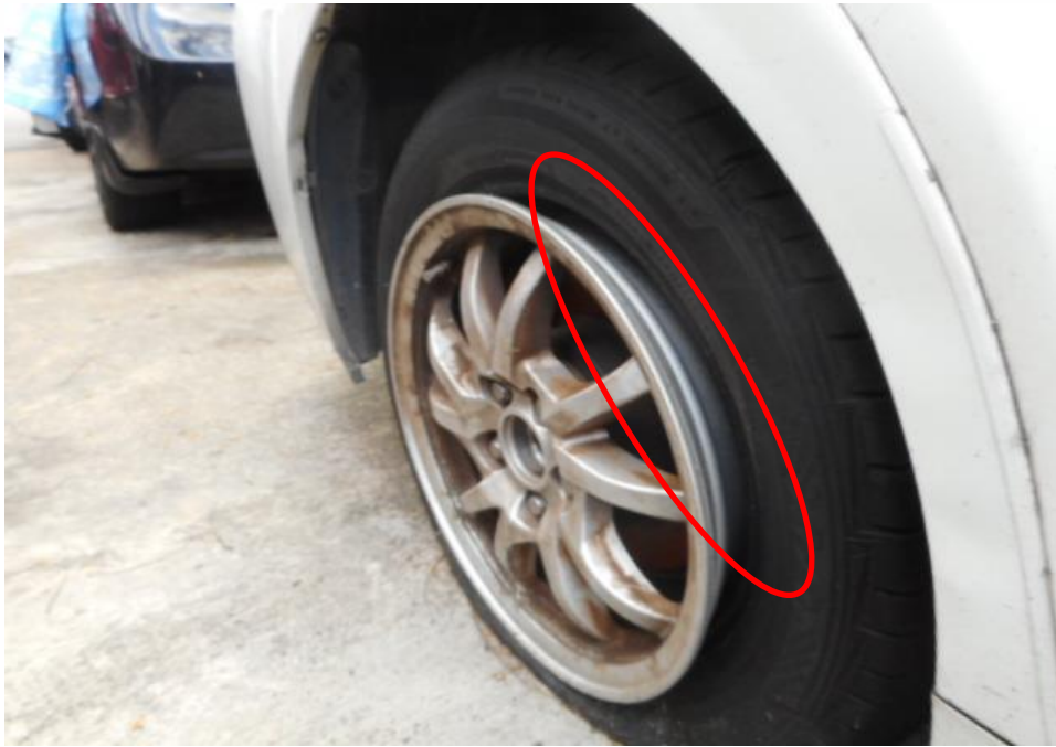
Photo 9 shows the condition of the rear right tyre and wheel rim of the Motor Car, which was observed to slip off the wheel rim and deflated (circled) due to the induce impact sustained as a result of the accident. The remaining tread depth is approximately 5.5mm.
