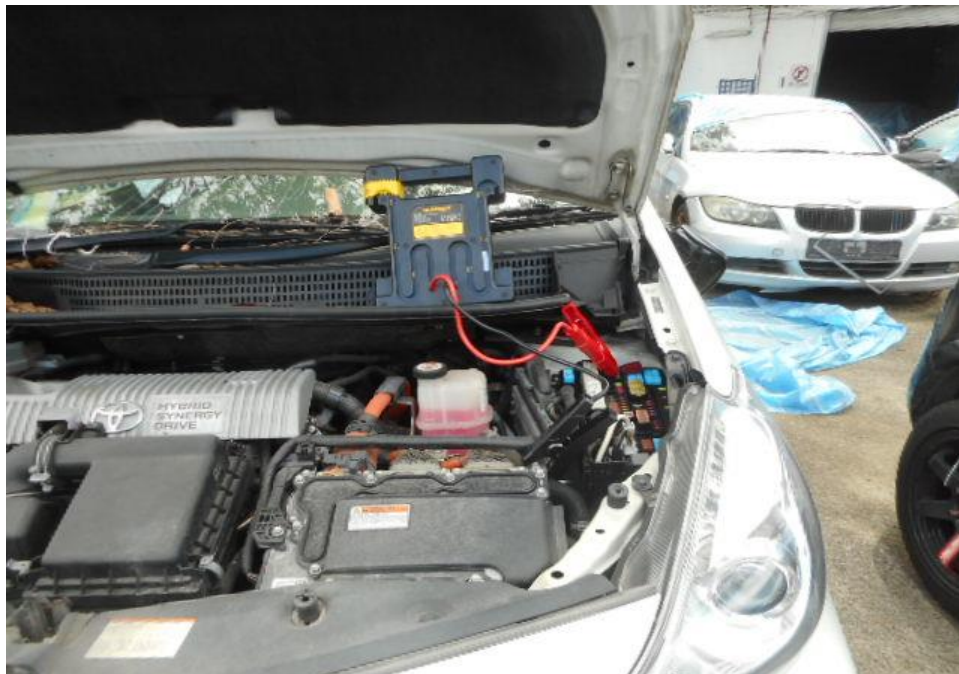
Photo 24 shows the jumpstarting of the Motor Car using a jump starter. The engine of the Motor Car was unable to be started up despite multiple attempts in jumpstarting it.
