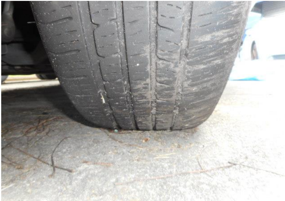
Photo 11 shows the condition of the front left tyre of the Motor Car, which was observed to be in serviceable condition with remaining tread depth of approximately 4.2mm. The tyre was also observed to be sufficiently inflated for vehicular operation with no tear, cut or burst mark(s).
