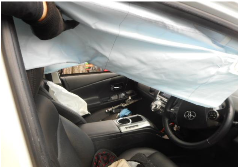
Photo 12 shows the deployment of the Supplemental Restraint System (SRS) airbag in the Motor Car as a result of the accident.
