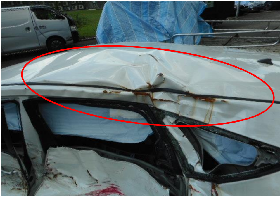
Photo 5 shows the close up view of the Motor Car's left vehicle chassis portion at the time of my inspection. The Motor car was observed to have sustained damage at its chassis portion. Its left chassis (circled) was damaged as a result of the accident.
