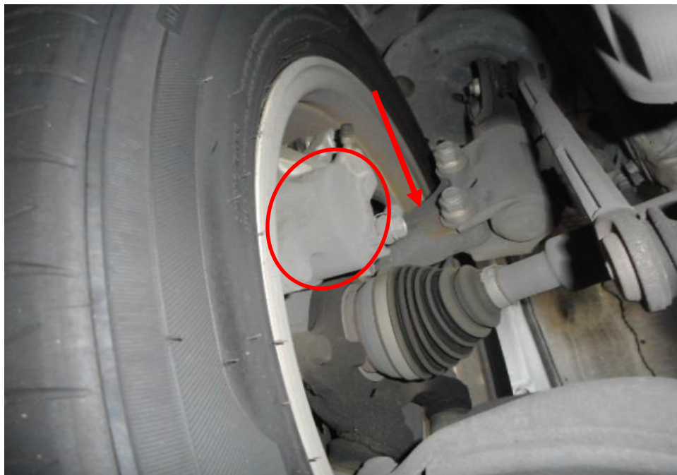
Photo 20 shows the brake hose/pipe (arrowed) at the front right wheel of the Motor Car. I did not observe any leakage of brake fluid at the time of my inspection of the Motor Car. Static tests of the Motor Car's braking system had indicated that there was no internal leakage of pressure/vacuum.
