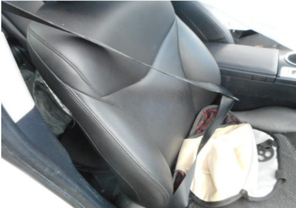
Photo 26 shows that the seat belt on the right seat were able to be fastened securely into the respective pre-tensioners that were fitted at the sides of each seat.
