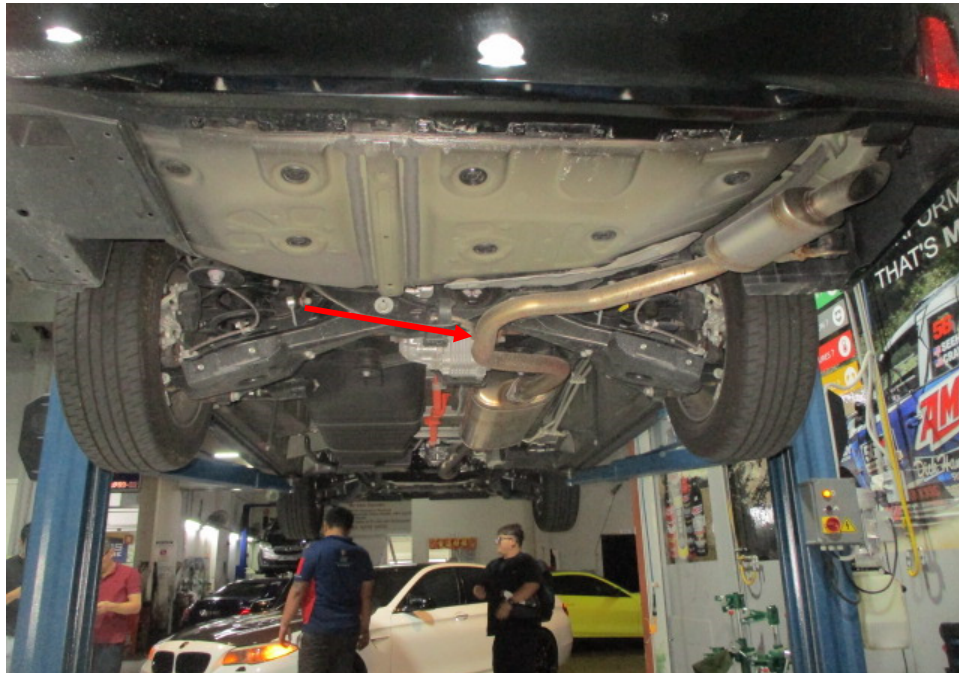
Photo 25 shows a general view of the rear section of the Motor Car's exhaust system. My examination of the Motor Car's exhaust system revealed no sign(s) or indication(s) of any cut or weld marks along its exhaust pipe (arrowed), on its catalytic converter, on its centre resonator box and on its rear muffler.
