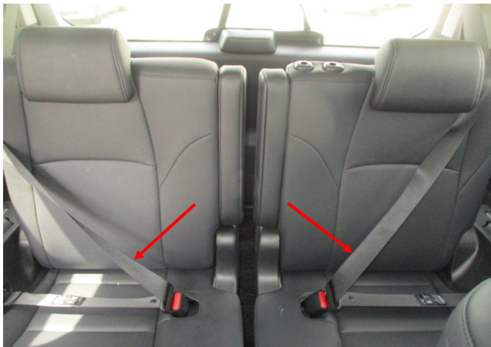
Photo 17 shows the rear seats at the 2 nd row of the Motor Car. All the seats of the Motor Car were secured via seat rails to the floorboard. They were also fitted with a retractable seat belt reel and a pre-tensioner. The seat belts (arrowed) were tested and were able to be fastened into the respective pre-tensions that were fitted on the side of each individual seat.
