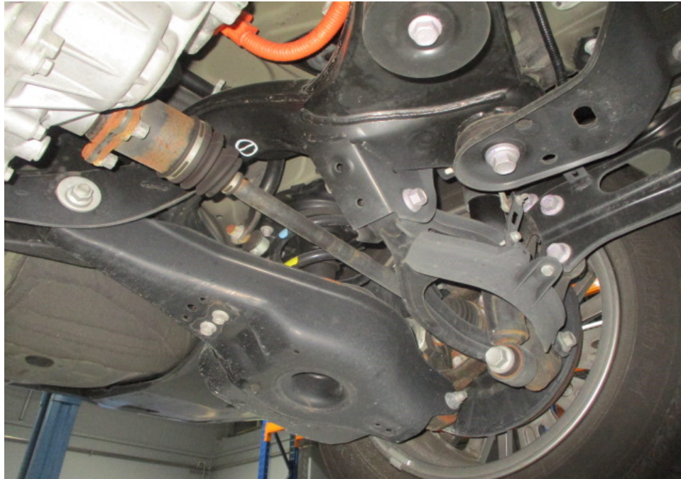
Photo 22 shows a general view of the control arms and linkages at the rear left wheel of the Motor Car. I did not observe any fluid leak and/or fluid stain on the underside of the Motor Car. All of the Motor Car's undercarriage components were observed to be intact and secured in an appropriate manner.
