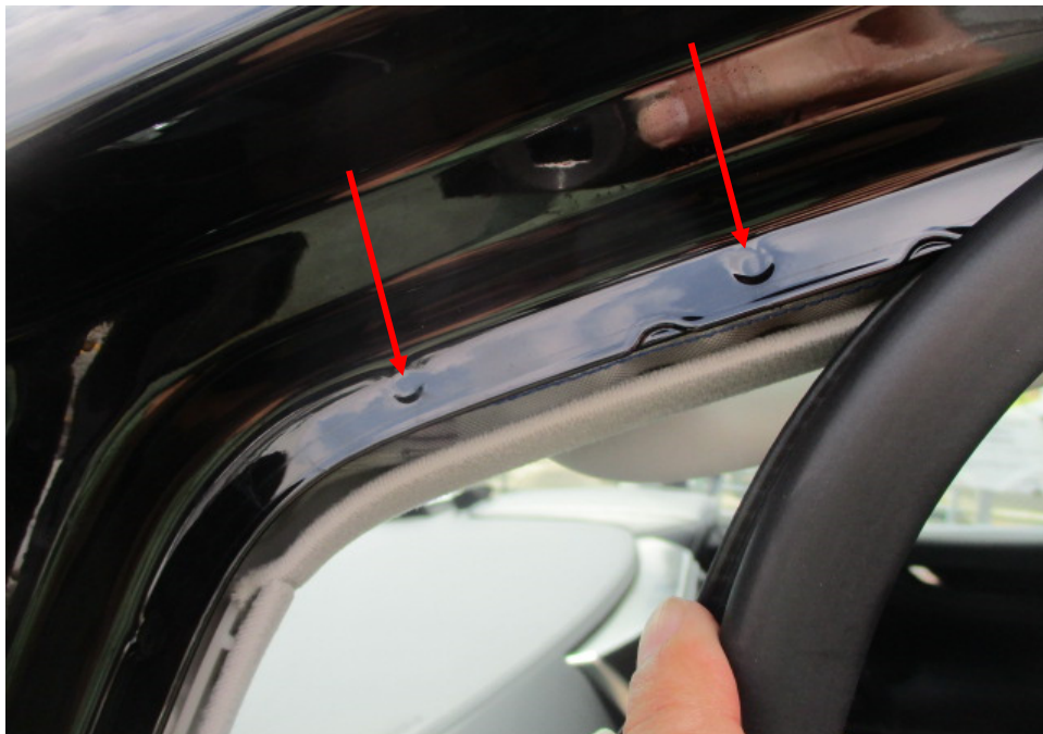
Photo 33 shows the left side "A" pillar of the Motor Car. I did not find any weld marks other than original spot weld marks (arrowed) on the left side "A" pillar of the Motor Car, which indicates that there was no re-welding works carried out. In general, I had found all the non-detachable body panels of the Motor Car to be originally fitted at the time of my inspection.
