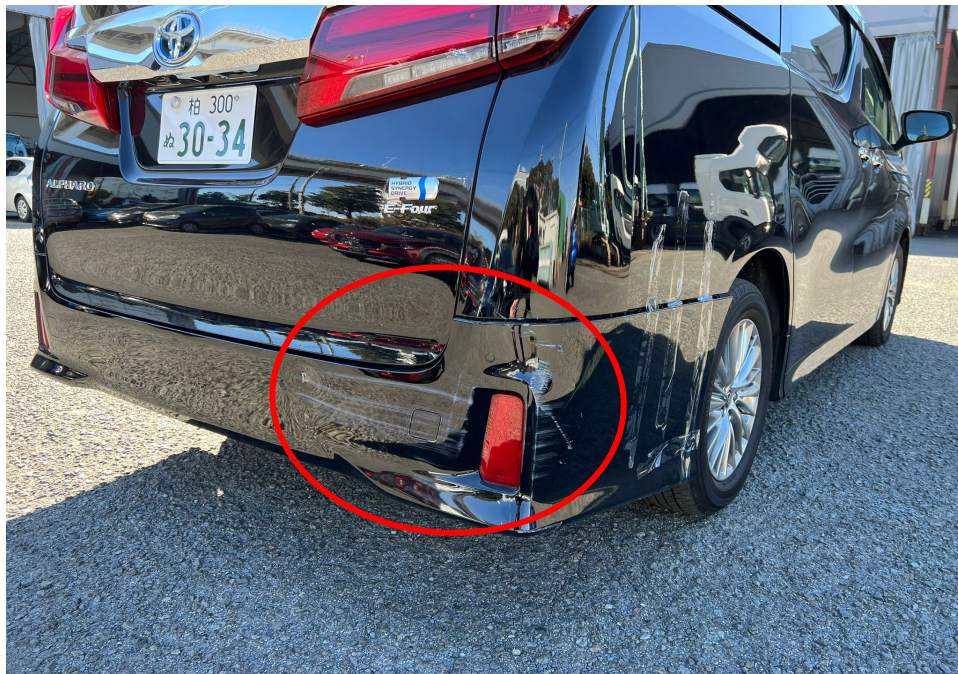
Photo 2 shows a closer view of the damage at the rear right portion (circled) of the Motor Car (photograph provided to me). The rear bumper, rear bumper tow hook cover and rear right taillamp lower panel were observed to be damaged.
