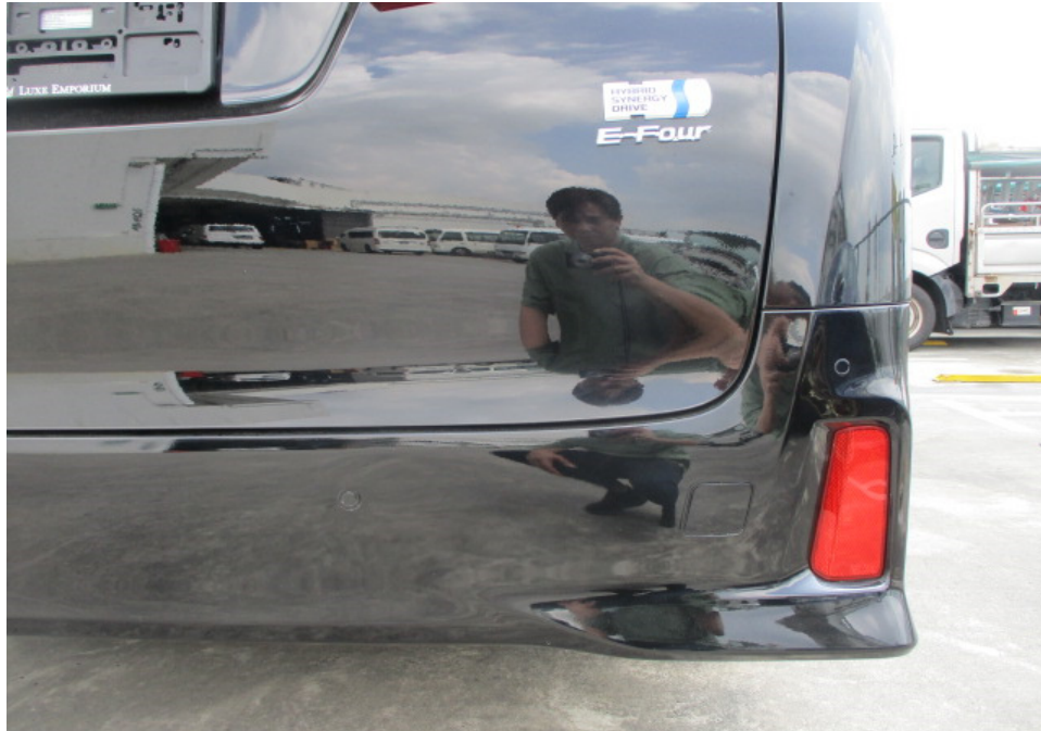
Photo 8 shows a closer view of the Motor Car's rear bumper, rear bumper tow hook cover, rear bumper right sensors, rear bumper right reflector, rear right taillamp lower panel and rear tailgate. The body parts at the rear right portion of the Motor Car were visually examined and it was observed that the repair/restoration works carried out to the damaged area of the Motor Car (refer to photograph 1 & 2 above) were reasonably adequate and in order.
