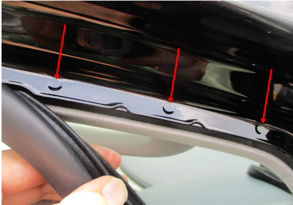
Photo 32 shows the right side "A" pillar of the Motor Car. I did not find any weld marks other than original spot weld marks (arrowed) on the right side "A" pillar of the Motor Car, which indicates that there was no re-welding works carried out. In general, I had found all the non-detachable body panels of the Motor Car to be originally fitted at the time of my inspection.
