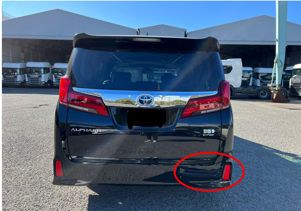
Photo 1 shows the rear body of the Motor Car (photograph provided to me). The Motor Car was observed to have sustained damage at its rear right portion (circled). The rear bumper, rear bumper tow hook cover and rear right taillamp lower panel were observed to be damaged.
