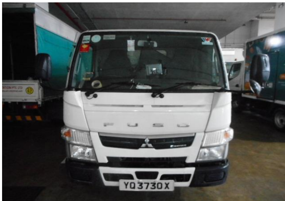
Photo 2 shows the front view of the Insured Vehicle at the time of our inspection. The front cabin portion of the Insured Vehicle was relatively unaffected by the fire.
