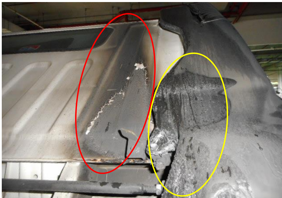
Photo 7 shows the close up view of the Insured Vehicle front cabin rear portion at the time of our inspection. The front cabin rear panel (red circle) and air intake filter box (yellow circle) of the Insured Vehicle had both sustained heat and smoke damages as a result of the fire.
