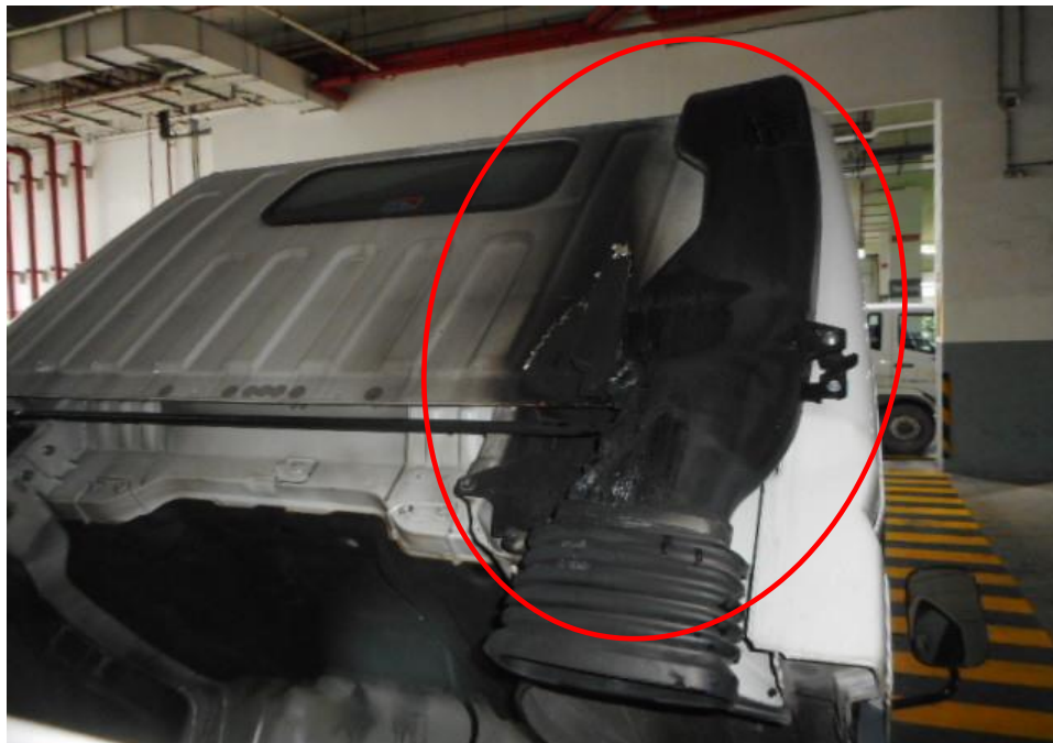
Photo 6 shows the general view of the Insured Vehicle front cabin rear portion at the time of our inspection. The front cabin rear panel and air intake filter box of the Insured Vehicle had both sustained heat and smoke damages as a result of the fire (circled).
