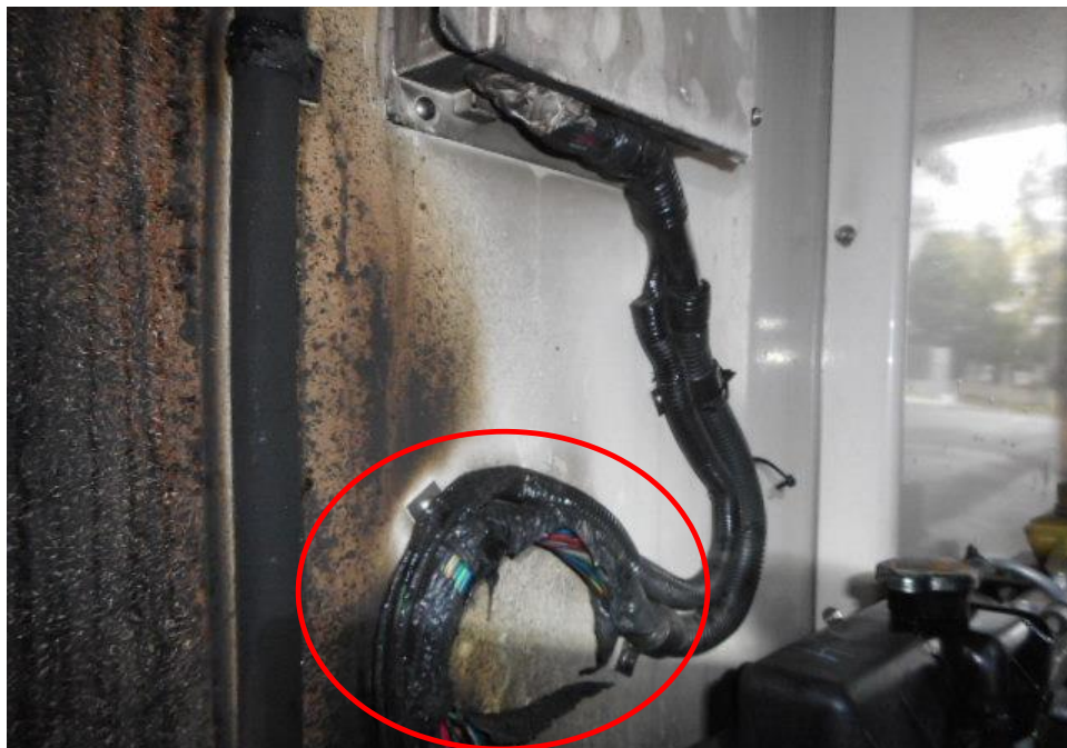
Photo 10 shows the close up view of the Insured Vehicle fridge front body panel at the time of our inspection. The electrical wirings of the fridge control panel (circled) of the Insured Vehicle had sustained heat and smoke damages as a result of the fire.
