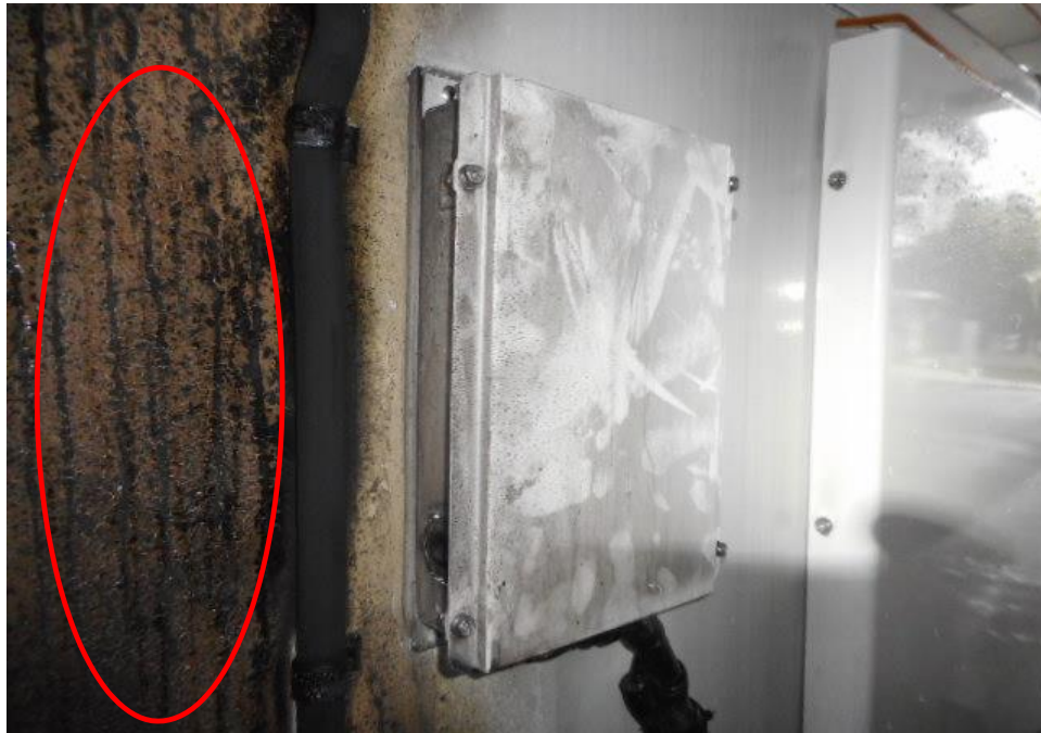
Photo 9 shows the close up view of the Insured Vehicle fridge front body panel at the time of our inspection. The fridge front body panel (circled) of the Insured Vehicle had sustained heat and smoke damages as a result of the fire.
