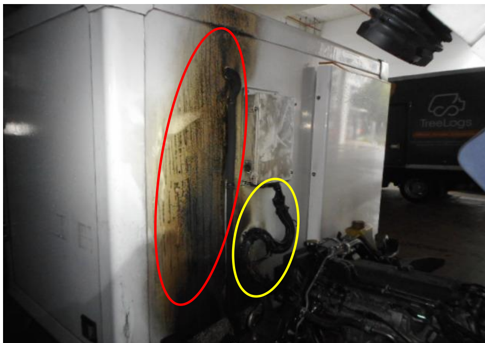
Photo 8 shows the general view of the Insured Vehicle fridge front body panel at the time of our inspection. The fridge front body panel (red circle) and the electrical wirings of the fridge control panel (yellow circle) of the Insured Vehicle had both sustained heat and smoke damages as a result of the fire.
