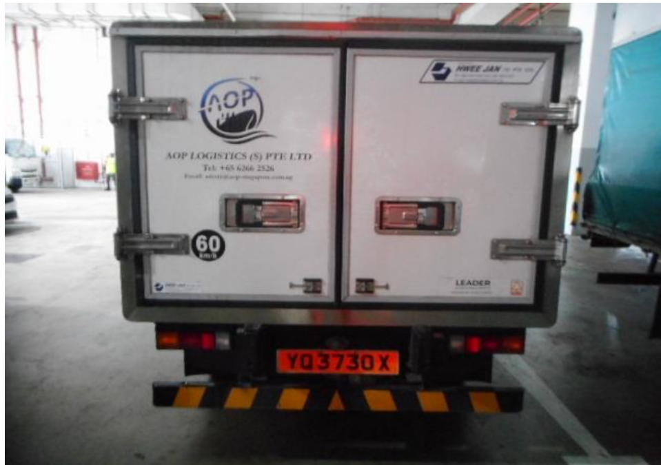
Photo 5 shows the rear view of the Insured Vehicle at the time of our inspection. The rear portion of the Insured Vehicle was relatively unaffected by the fire.
