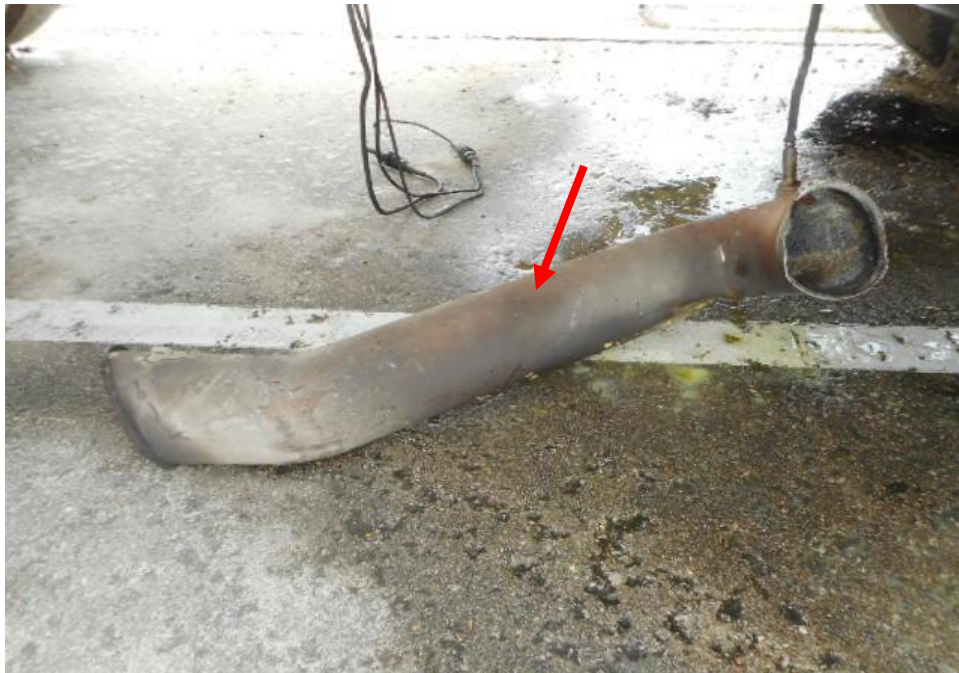
Photo 26 shows a close up view of the rear right portion of the Prime Mover at the time of my inspection. The engine components located at the right rear portion of the Prime Mover was observed to have sustained damage. Its engine exhaust piping (arrowed) as a result of the accident.
