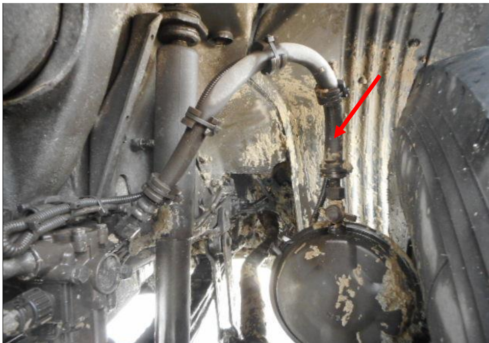
Photo 32 shows the brake pipe (arrowed) at the front right wheel of the Prime Mover. I did not observe any leakage of air brake at the time of my inspection of the Prime Mover. My visual examination of the various mechanical components in the braking system components were generally intact.
