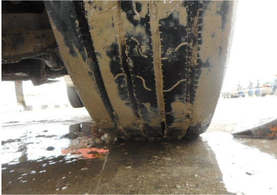
Photo 7 shows the condition of the front right tyre of the Prime Mover, which was observed to be in serviceable condition with remaining tread depth of approximately 12.5 mm. The tyre, which was wrapped around standard steel wheel rim, was also observed to be sufficiently inflated for vehicular operation. There was no tear, cut or burst mark(s) on the outer and the inner sidewalls as well as across the tread of the 6 tyres that were fitted on the Prime Mover.
