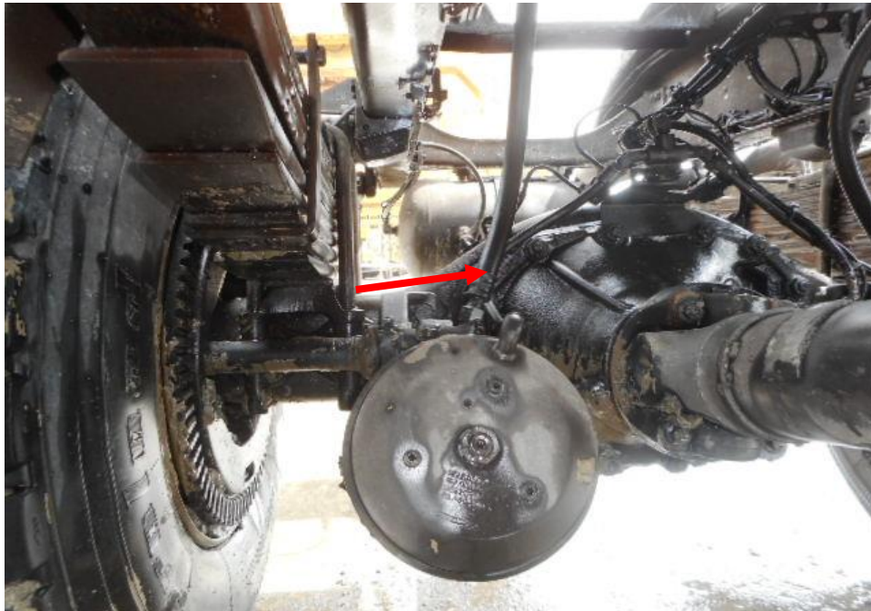
Photo 30 shows the brake pipe (arrowed) at the rear right wheel of the Prime Mover. I did not observe any leakage of air brake at the time of my inspection of the Prime Mover. My visual examination of the various mechanical components in the braking system components were generally intact.
