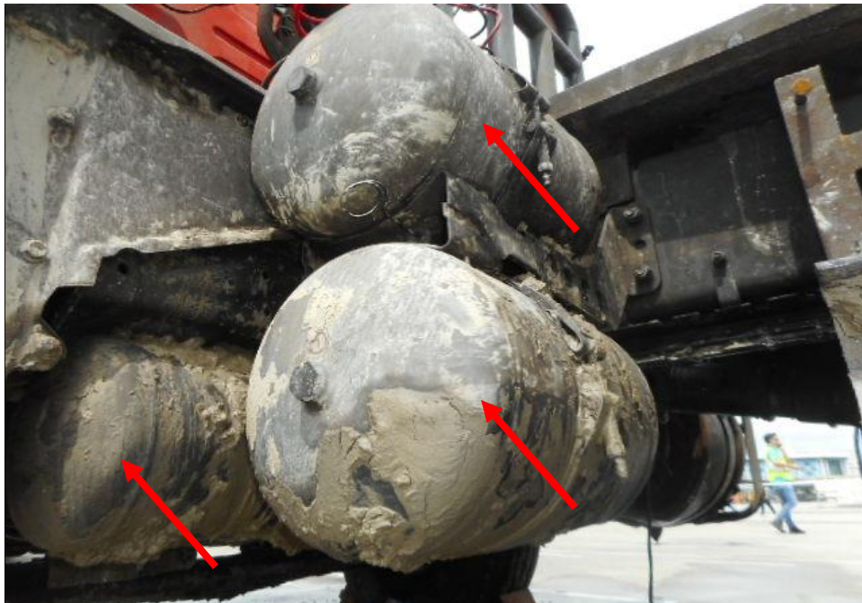
Photo 34 shows the air brake cylinders (arrowed) at the undercarriage of the Prime Mover. I did not observe any leakage of air brake at the time of my inspection of the Prime Mover. My visual examination of the various mechanical components in the braking system components were generally intact.
