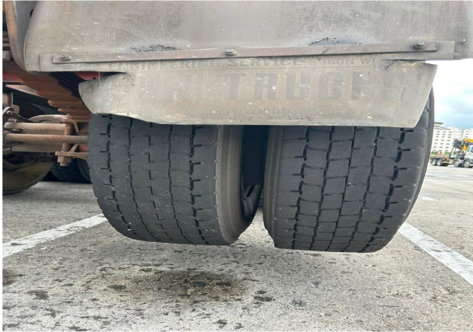
Photo 17 shows the condition of the right tyres of the Trailer Bed, which was observed to be in serviceable condition with remaining tread depth of approximately 10.2mm. The tyre, which was wrapped around standard steel wheel rim, was also observed to be sufficiently inflated for vehicular operation.
