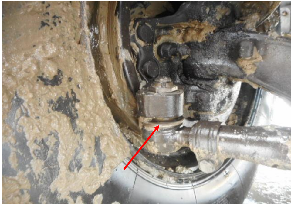
Photo 28 shows the various undercarriage components at the front left wheel of the Prime Mover, in particular the steering tie rod end (arrowed). The various undercarriage components of the Prime Mover were all found to be intact without any visible damage. There was also no sign of fluid stain(s) observed on the various undercarriage components.
