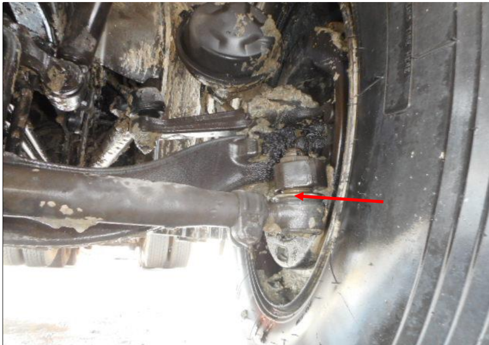
Photo 27 shows the various undercarriage components at the front right wheel of the Prime Mover, in particular the steering tie rod end (arrowed). The various steering components were all found to be intact, suggesting that the steering system of the Prime Mover was likely to be in serviceable condition at the material time of accident. There was also no sign of fluid stain(s) observed on the various undercarriage components.
