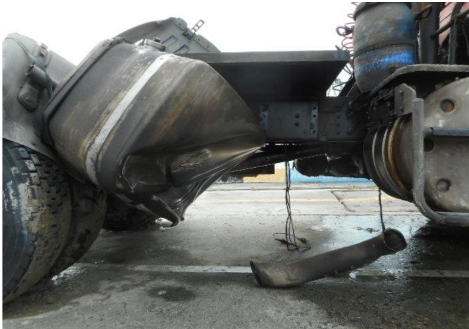
Photo 24 shows a close up view of the right rear portion of the Prime Mover at the time of my inspection. The engine components located at the right rear portion of the Prime Mover was observed to have sustained damage. Its fuel tank and engine exhaust piping was damaged as a result of the accident.
