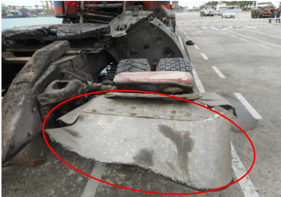
Photo 2 shows a close up view of the rear body of the Prime Mover at the time of my inspection. The Prime Mover was observed to have sustained damage at its rear portion. Its rear right wheel panel (circled) were amongst the body parts that were damaged as a result of the accident.
