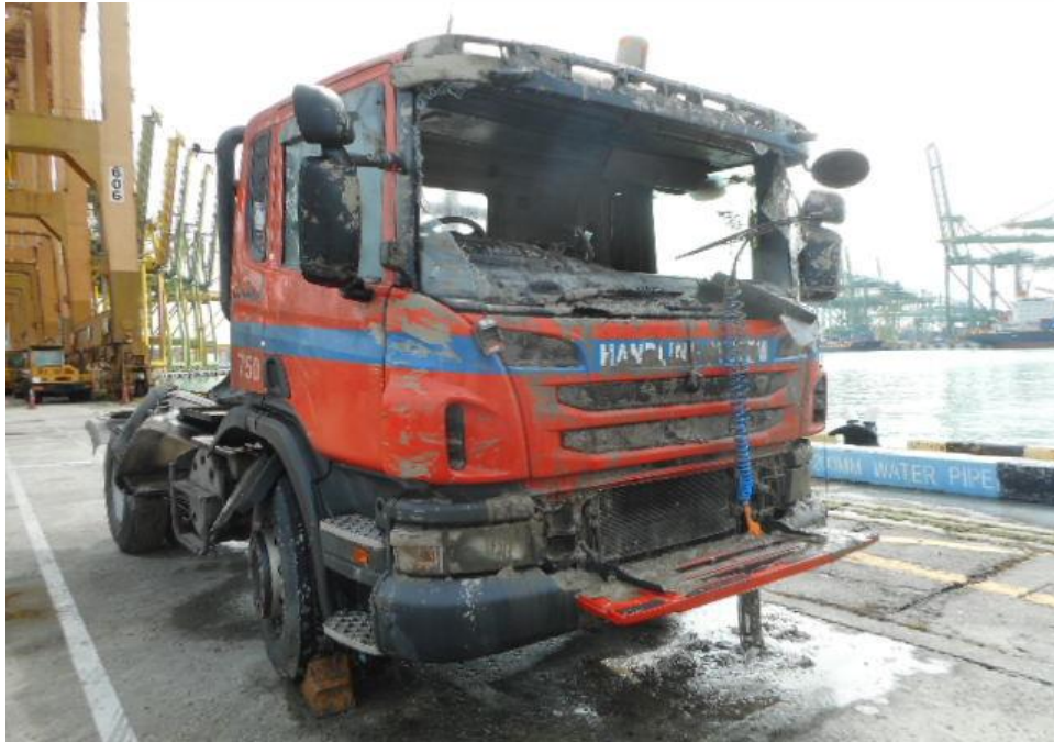
Photo 3 shows a general view of the front body of the Prime Mover at the time of my inspection. The Prime Mover was observed to have sustained damage at its front portion. Its front windscreen, were amongst the body parts that were damaged as a result of the accident.
