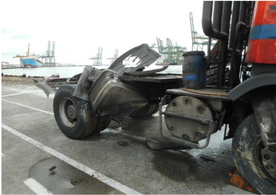
Photo 23 shows a general view of the right rear portion of the Prime Mover at the time of my inspection. The engine components located at the right rear portion of the Prime Mover was observed to have sustained damage. Its fuel tank and engine exhaust piping was damaged as a result of the accident.
