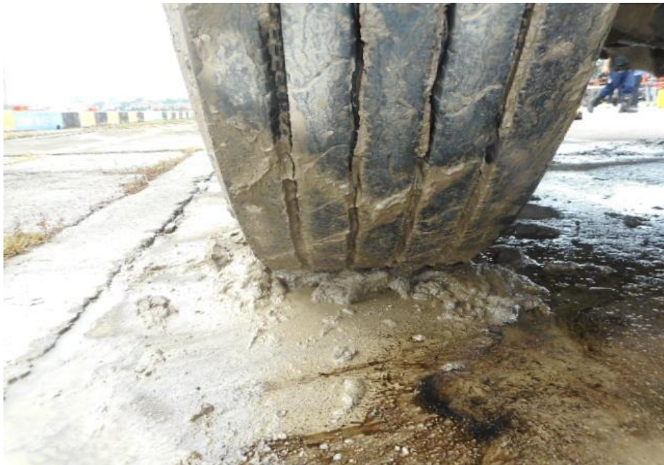
Photo 10 shows the condition of the front left tyres of the Prime Mover, which were observed to be in serviceable condition with remaining tread depth of approximately 12.7mm. There was also no tear, cut or burst mark(s) on the outer and the inner sidewalls as well as across the tread of the 6 tyres that were fitted on the Prime Mover.
