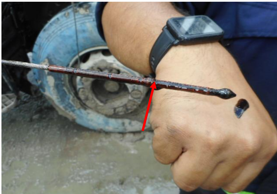
Photo 20 shows checks being carried out to the engine oil of the Prime Mover at the time of my inspection. The engine oil on the dipstick was observed to be of sufficient level (arrowed) and without any visible contamination.
