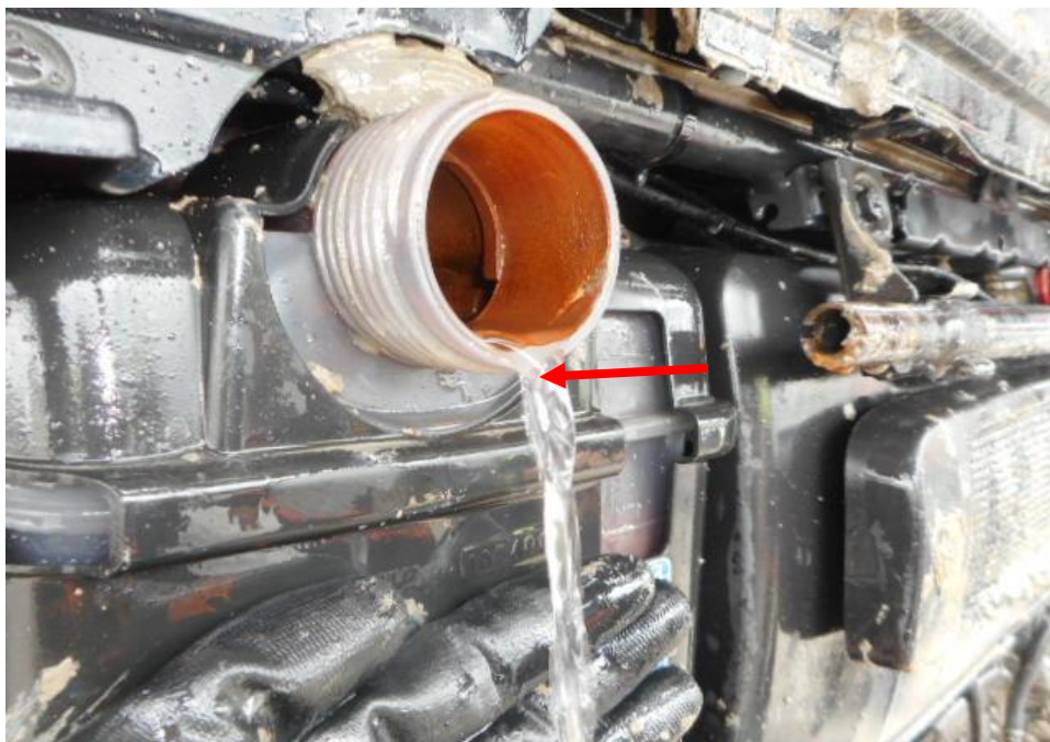
Photo 22 shows checks being carried out to the engine coolant of the Prime Mover at the time of my inspection. The engine coolant was observed to be of sufficient level (arrowed) and without any visible contamination.
