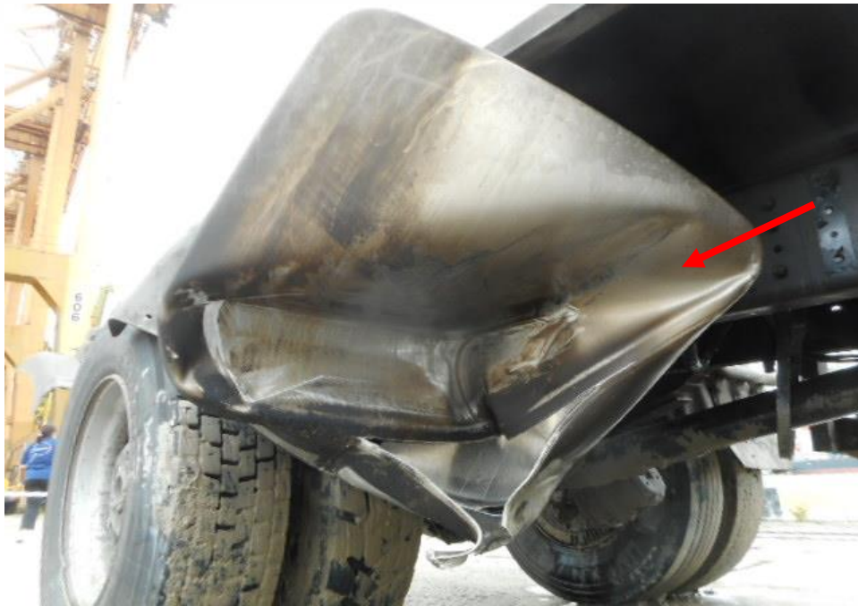
Photo 25 shows a close up view of the right rear portion of the Prime Mover at the time of my inspection. The engine components located at the right rear portion of the Prime Mover was observed to have sustained damage. Its fuel tank (arrowed) as a result of the accident.
