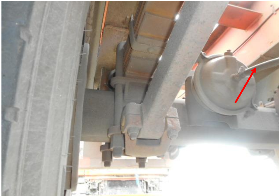
Photo 35 shows the brake pipe (arrowed) at the right wheels of the Trailer Bed. I did not observe any leakage of air brake at the time of my inspection of the Trailer Bed and the various mechanical components was observed to be intact.
