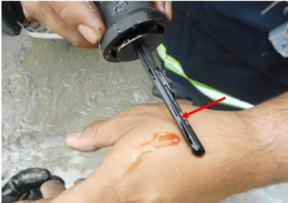
Photo 21 shows checks being carried out to the power steering fluid of the Prime Mover at the time of my inspection. The power steering fluid on the dipstick was observed to be of sufficient level (arrowed) and without any visible contamination.
