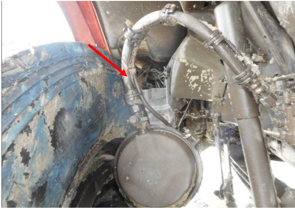
Photo 33 shows the brake pipe (arrowed) at the front left wheel of the Prime Mover. I did not observe any leakage of air brake at the time of my inspection of the Prime Mover. My visual examination of the various mechanical components in the braking system components were generally intact.
