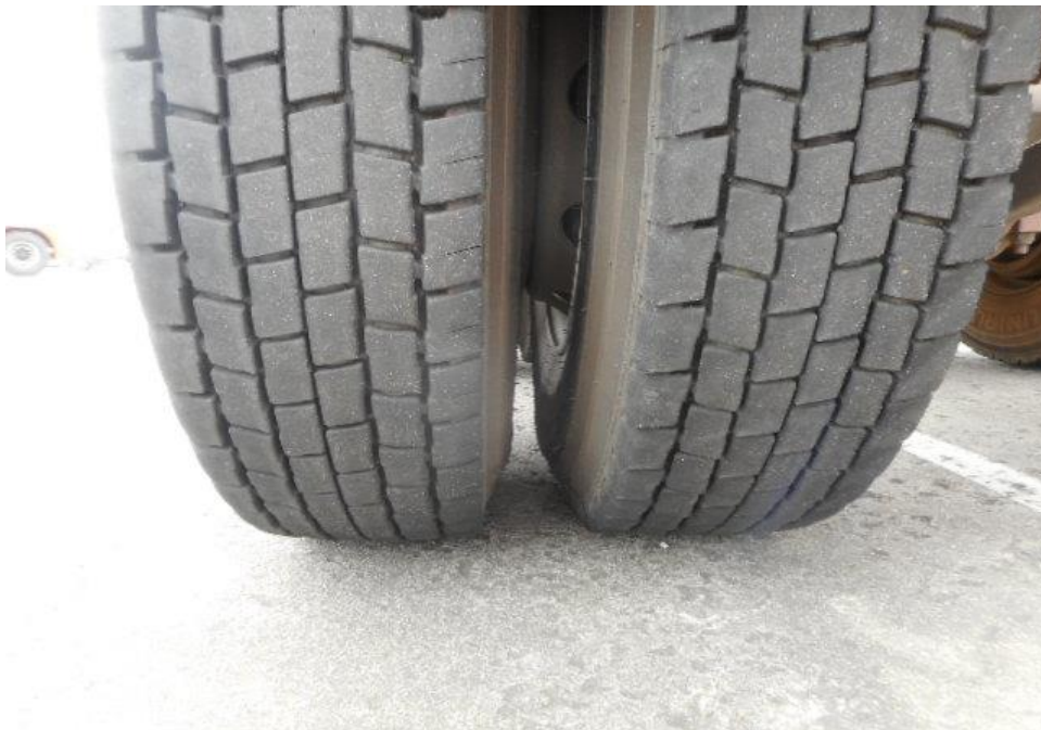
Photo 18 shows the condition of the left tyres of the Trailer Bed, which was observed to be in serviceable condition with remaining tread depth of approximately 10.2mm. The tyres, which were wrapped around standard steel wheel rim, were also observed to be sufficiently inflated for vehicular operation. There was also no damage found on all 12 steel wheel rims of the Trailer Bed.
