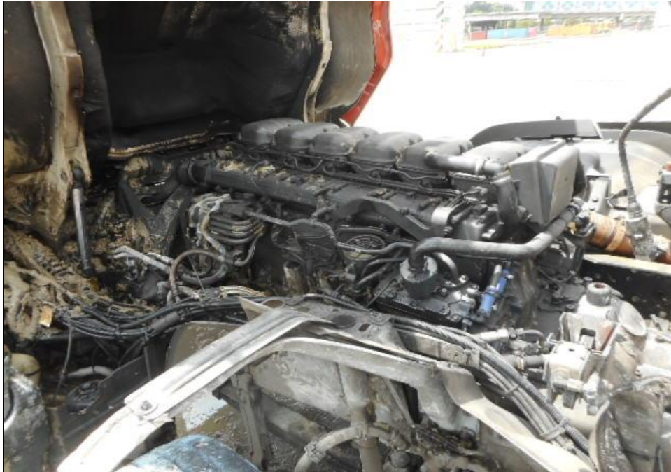
Photo 19 shows the general view of the Prime Mover's engine compartment, which was accessed by lifting the front cabin of the Prime Mover. The various parts and components inside the engine compartment were unaffected by the accident. There was also no sign(s) or indication(s) of fresh fluid leakage and/or fluid stain within the engine compartment
