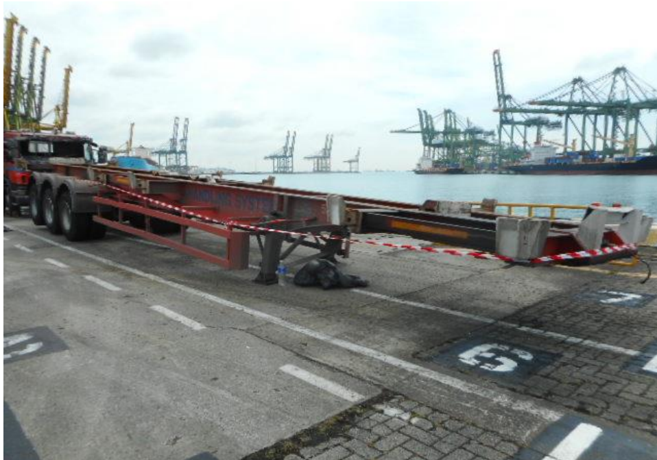
Photo 12 shows a general view of the right body of the Trailer Bed at the time of my inspection. The right support stand of the Trailer Bed was observed to be damaged as a result of the accident.
