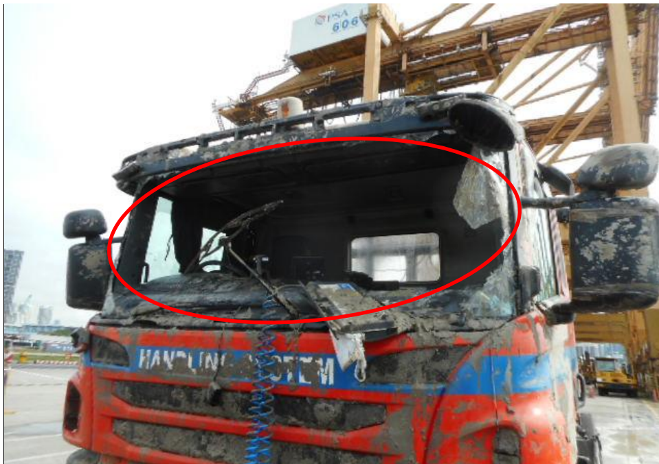
Photo 4 shows the close up view of the Prime Mover front body at the time of my inspection. The Prime Mover was observed to have sustained damage at its front windscreen (circled), as a result of the accident.
