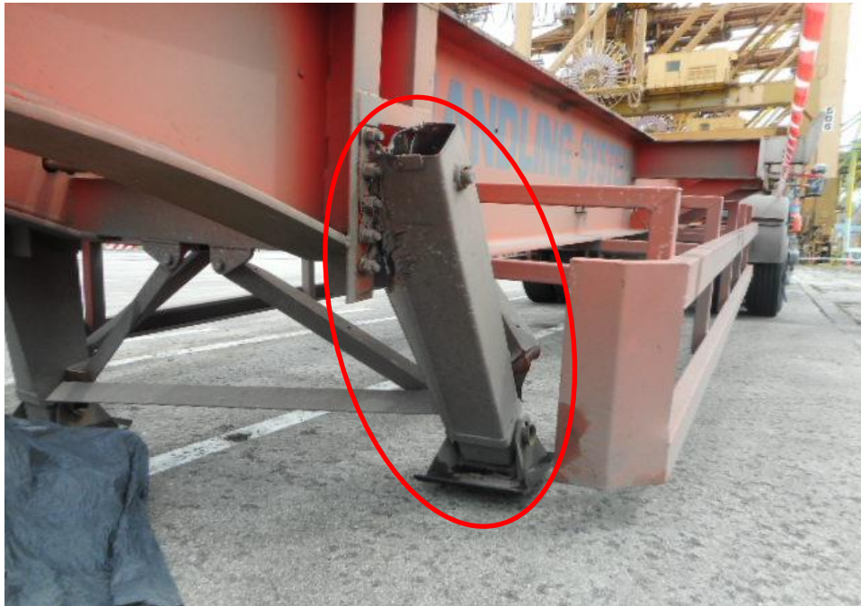
Photo 15 shows a close up view of the right body of the Trailer Bed at the time of my inspection. The right support stand (circled) of the Trailer Bed was observed to be damaged as a result of the accident.
