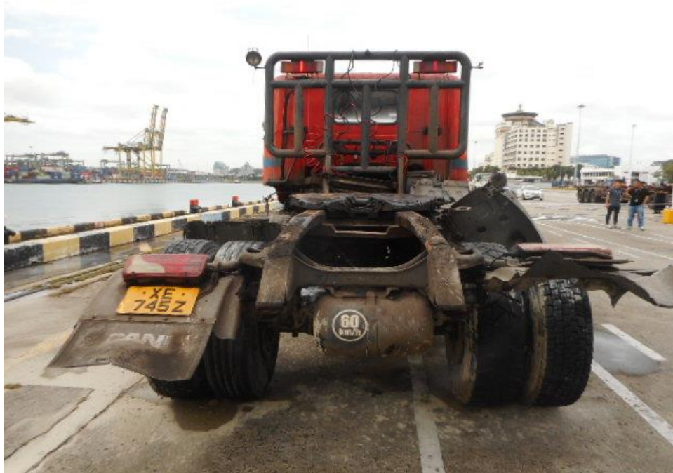
Photo 1 shows a general view of the rear body of the Prime Mover at the time of my inspection. The Prime Mover was observed to have sustained damage at its rear portion. Its rear right wheel panel were amongst the body parts that were damaged as a result of the accident.
