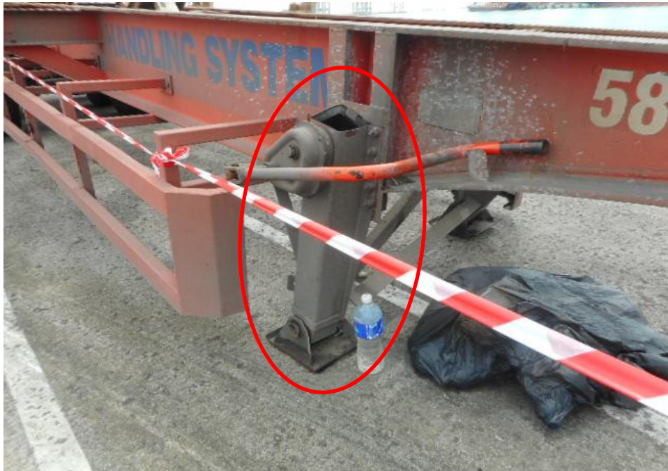
Photo 13 shows a close up view of the right body of the Trailer Bed at the time of my inspection. The right support stand (circled) of the Trailer Bed was observed to be damaged as a result of the accident.
