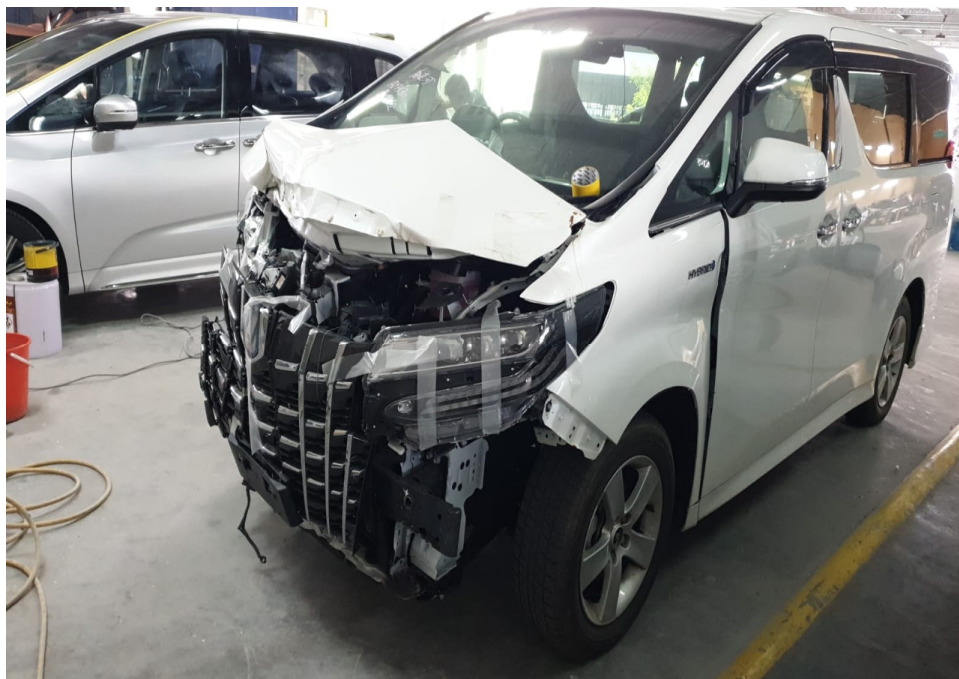
Photo 3 shows the front left body of the Motor Car (photograph provided to me). The Motor Car was observed to have sustained damage at its frontal portion. The front bumper, front bumper left lower grille, front bumper left fog lamp, front bumper left chrome garnish, front bumper left bracket, front bonnet, front left headlamp, front left headlamp top panel and front left fender were amongst the body parts at the frontal portion that were observed to have been damaged.
