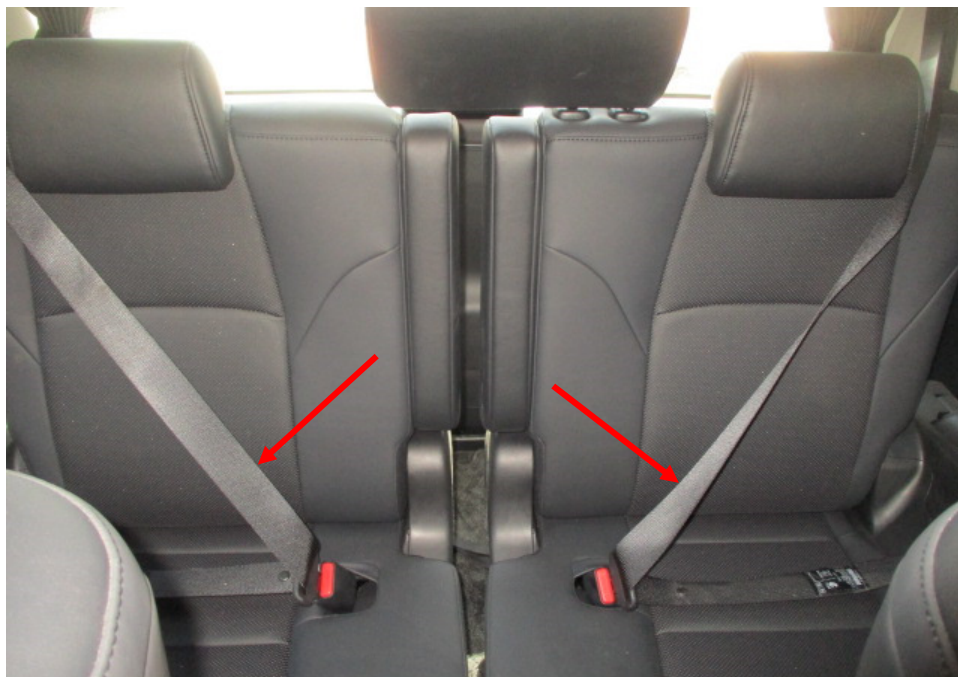
Photo 20 shows the rear seats at the 2 nd row of the Motor Car. All the seats of the Motor Car were secured via seat rails to the floorboard. They were also fitted with a retractable seat belt reel and a pre-tensioner. The seat belts (arrowed) were tested and were able to be fastened into the respective pre-tensions that were fitted on the side of each individual seat.
