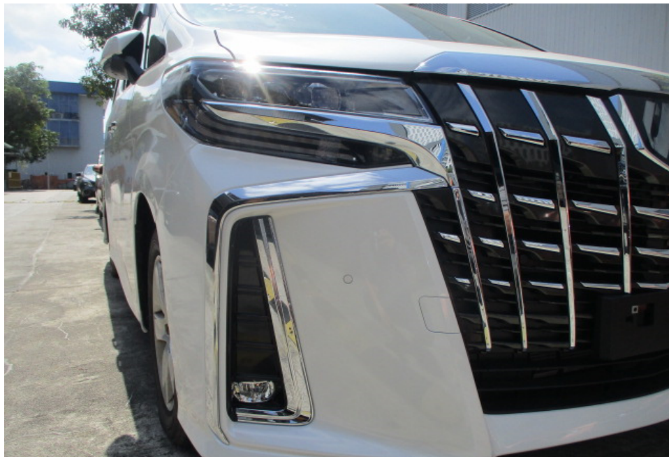
Photo 8 shows a closer view of the Motor Car's front bumper, front bumper right lower grille, front bumper right fog lamp, front bumper right chrome garnish, front bumper tow cover, front right headlamp, front right headlamp chrome moulding and front grille. The body parts at the frontal portion of the Motor Car were visually examined and it was observed that the repair/restoration works carried out to the damaged area of the Motor Car (refer to photograph 1 - 4 above) were reasonably adequate and in order.
