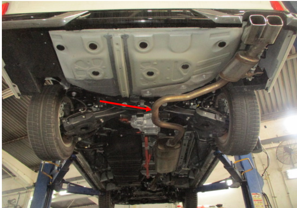
Photo 28 shows a general view of the rear section of the Motor Car's exhaust system. My examination of the Motor Car's exhaust system revealed no sign(s) or indication(s) of any cut or weld marks along its exhaust pipe (arrowed), on its catalytic converter, on its centre resonator box and on its rear muffler.
