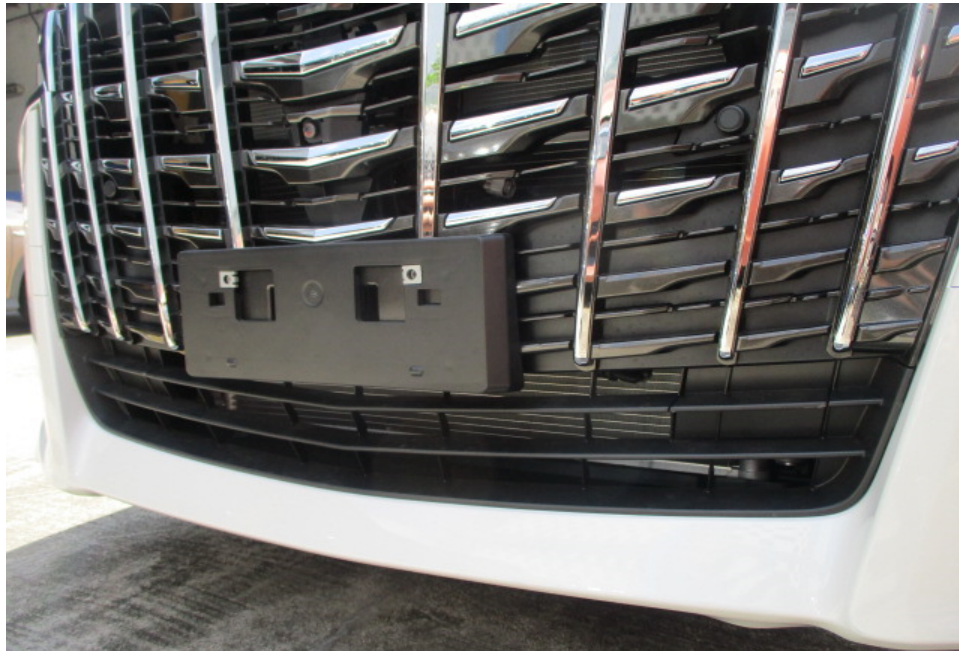
Photo 12 shows a closer view of the Motor Car's front bumper centre lower grille, front number plate garnish and front grille. The body parts at the frontal portion of the Motor Car were visually examined and it was observed that the repair/restoration works carried out to the damaged area of the Motor Car (refer to photograph 1 - 4 above) were reasonably adequate and in order.
