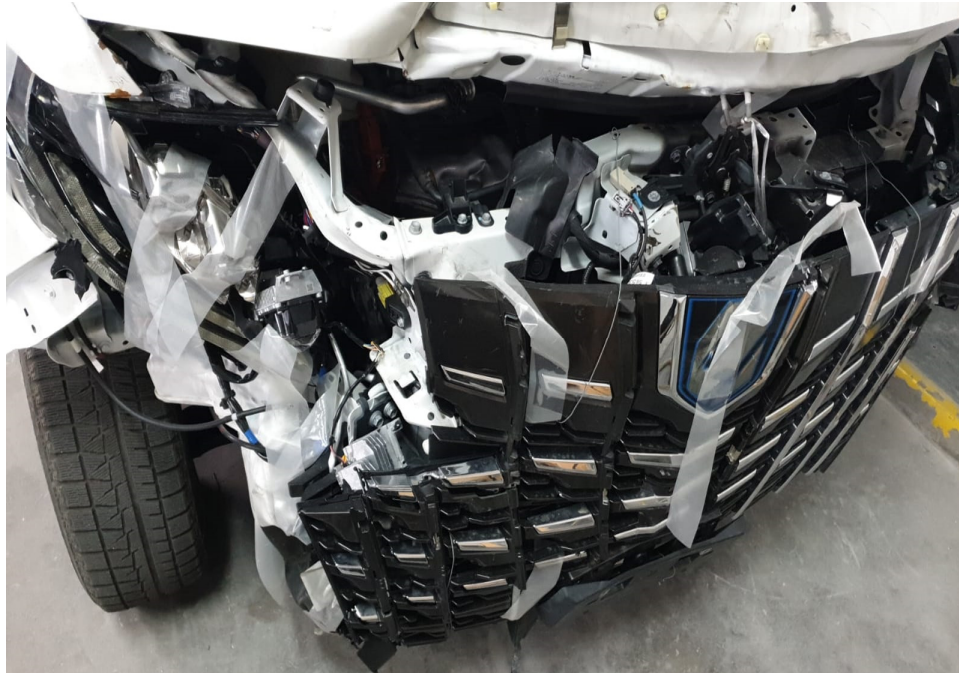
Photo 2 shows a closer view of the damage at the frontal portion of the Motor Car (photograph provided to me). The front bumper, front grille, front bonnet, front bonnet lock, front right headlamp, front right headlamp top panel, front support panel top cover, front support panel, aircon condenser and radiator were amongst the body parts that were observed to have been damaged.
