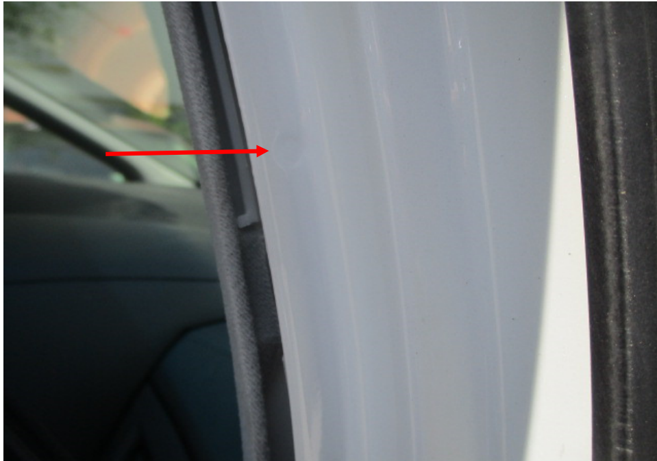
Photo 35 shows the right side "A" pillar of the Motor Car. I did not find any weld marks other than original spot weld marks (arrowed) on the right side "A" pillar of the Motor Car, which indicates that there was no re-welding works carried out. In general, I had found all the non-detachable body panels of the Motor Car to be originally fitted at the time of my inspection.
