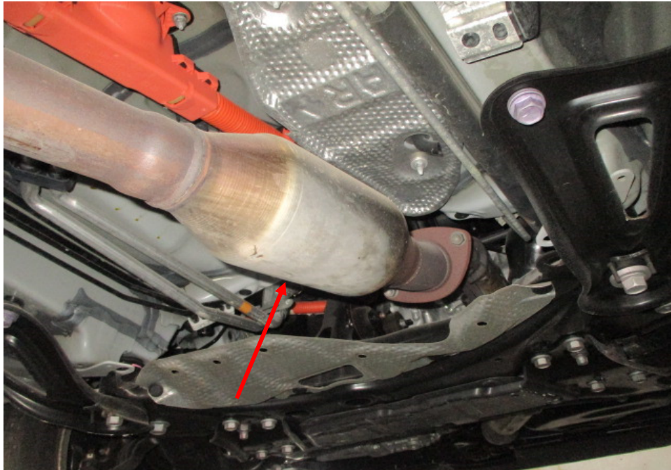
Photo 29 shows a general view of the front section of the Motor Car's exhaust system. My examination of the Motor Car's exhaust system revealed no sign(s) or indication(s) of any cut or weld marks along its exhaust pipe, on its catalytic converter (arrowed), on its centre resonator box and on its rear muffler.
