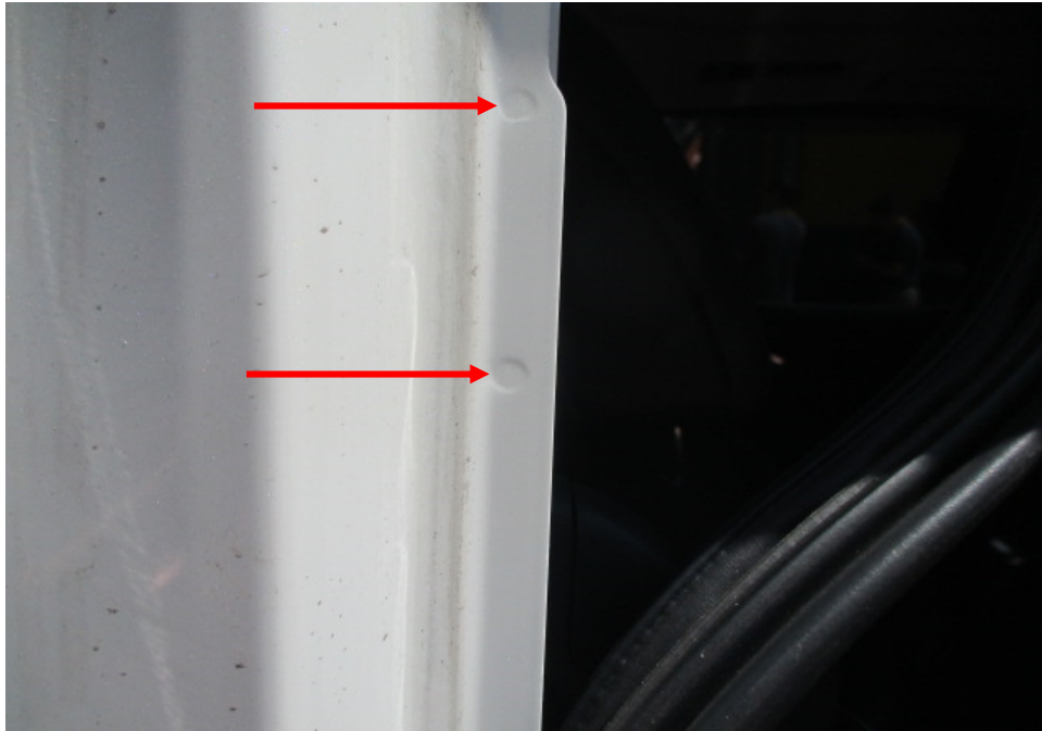
Photo 37 shows the left side "B" pillar of the Motor Car. I did not find any weld marks other than original spot weld marks (arrowed) on the left side "B" pillar of the Motor Car, which indicates that there was no re-welding works carried out. In general, I had found all the non-detachable body panels of the Motor Car to be originally fitted at the time of my inspection.
