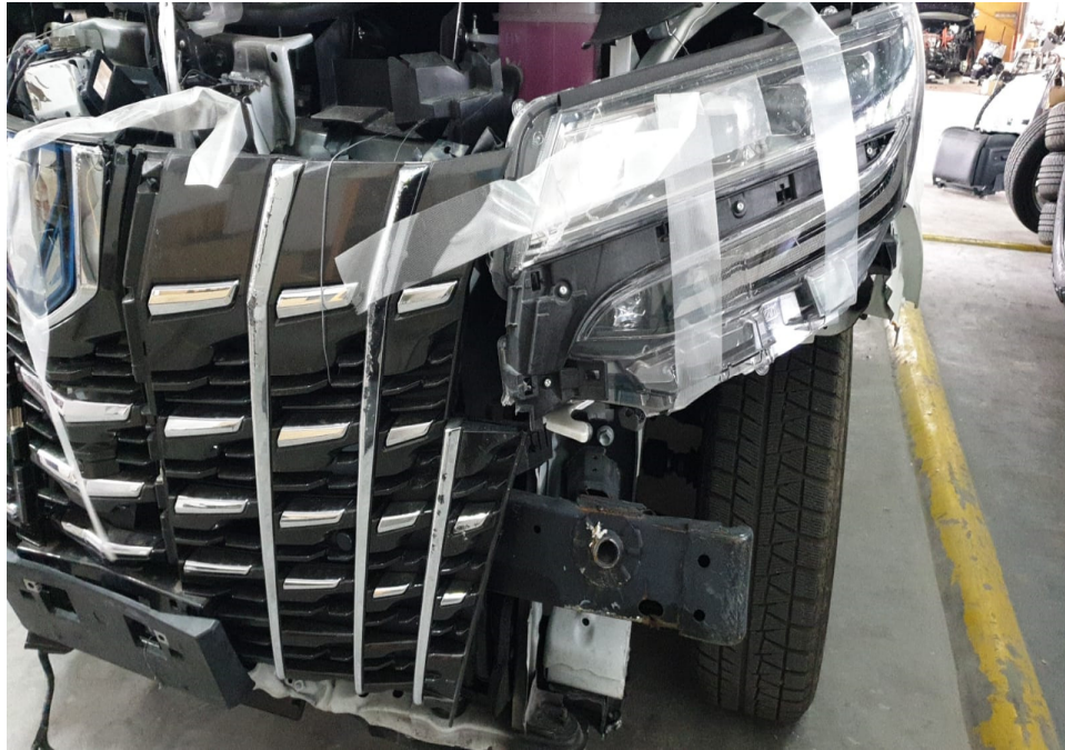
Photo 4 shows a closer view of the damage at the frontal portion of the Motor Car (photograph provided to me). The front bumper, front bumper reinforcement, front bumper left lower grille, front bumper left fog lamp, front bumper left chrome garnish, front grille, front left headlamp, front left headlamp chrome moulding, front left headlamp top panel, front left fender inner shield, front support panel top cover and front support were amongst the body parts that were observed to have been damaged.
