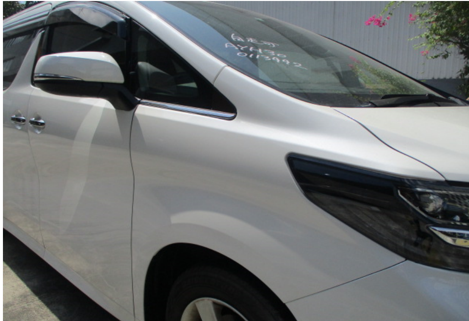
Photo 7 shows a closer view of the Motor Car's front right headlamp, front right fender and front right door. The body parts at the frontal portion of the Motor Car were visually examined and it was observed that the repair/restoration works carried out to the damaged area of the Motor Car (refer to photograph 1 - 4 above) were reasonably adequate and in order.
