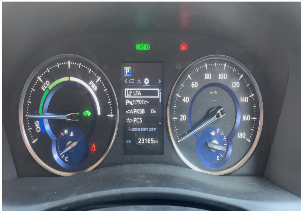
Photo 22 shows the respective warning lights no longer illuminated, indicating that there is no fault detected to the ABS, SRS, EPS, VSC and the various collision prevention systems of the Motor Car during the self-test. These electronic systems were hence in working condition at the time of my inspection.
