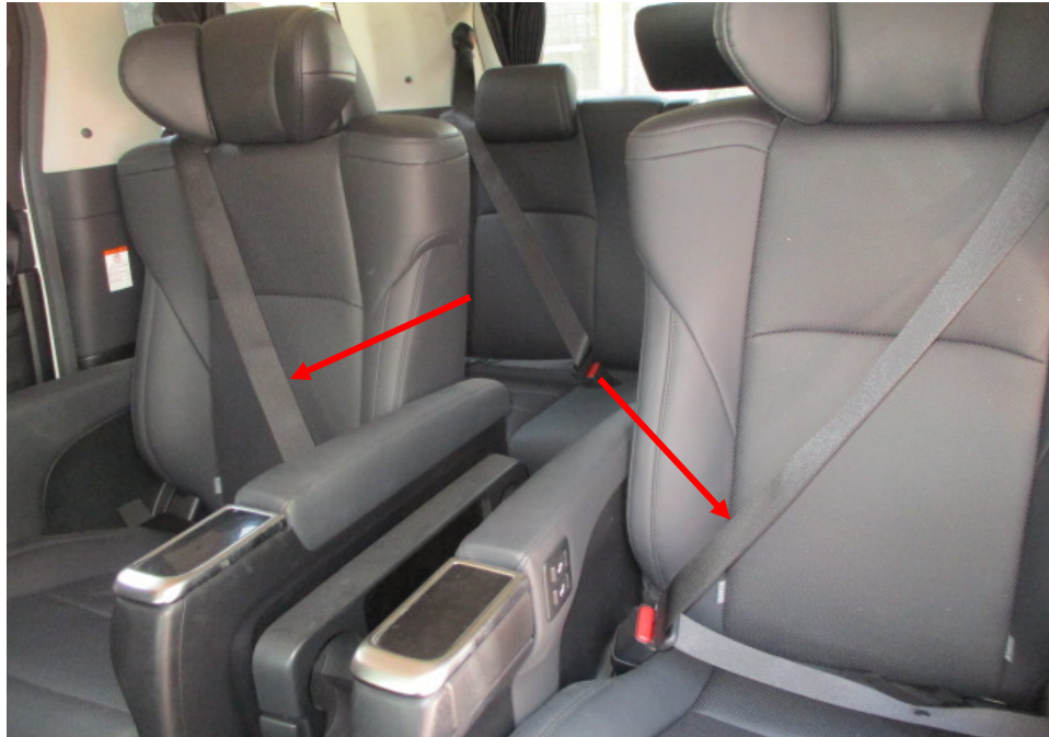
Photo 19 shows the rear seats at the 1 st row of the Motor Car. All the seats of the Motor Car were secured via seat rails to the floorboard. They were also fitted with a retractable seat belt reel and a pre-tensioner. The seat belts (arrowed) were tested and were able to be fastened into the respective pre-tensions that were fitted on the side of each individual seat.
