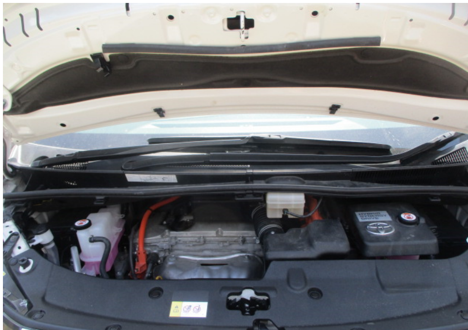
Photo 16 shows a general view of the engine compartment of the Motor Car at the time of my inspection. The various parts and components inside the engine compartment were all observed to be intact and properly fitted. There was no sign(s) or indication(s) of fluid leak and/or fluid stain found inside the engine compartment. The repair/restoration works carried out to the various parts within the engine compartment like the front headlamp top panels, front support panel, front support panel top cover, aircon condenser, radiator, cooling fan and aircon pipes amongst others, were reasonably adequate and in order.
