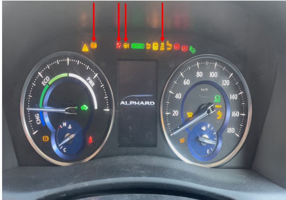
Photo 21 shows the warning lights for the various electronic safety features appearing on the instrument panel of the Motor Car during its self-test when the engine is cranked, in particular the lights for the ABS, SRS, EPS, VSC (arrowed) and the various collision prevention systems.
