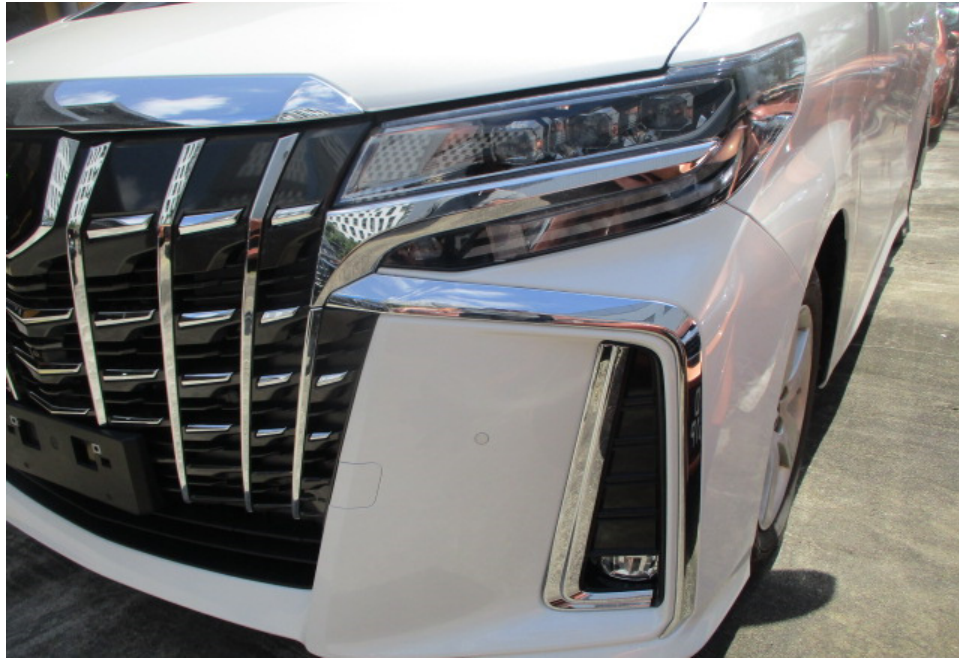
Photo 11 shows a closer view of the Motor Car's front bumper, front bumper left lower grille, front bumper left fog lamp, front bumper left chrome garnish, front left headlamp, front left headlamp chrome moulding, front bonnet and front bonnet chrome moulding. The body parts at the frontal portion of the Motor Car were visually examined and it was observed that the repair/restoration works carried out to the damaged area of the Motor Car (refer to photograph 1 - 4 above) were reasonably adequate and in order.
