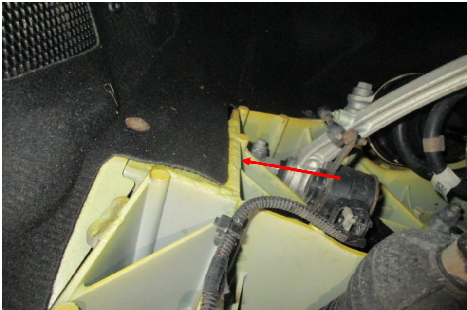
Photo 36 shows the aluminium chassis/structural body at the underside front left of the Motor Car. The original factory sealant (arrowed) at the joints along the aluminium chassis/structural body was observed to be untouched. In general, I had found no work was carried out on the aluminium chassis/structural body of the Motor Car. The aluminium chassis/structural body of the Motor Car was originally fitted.
