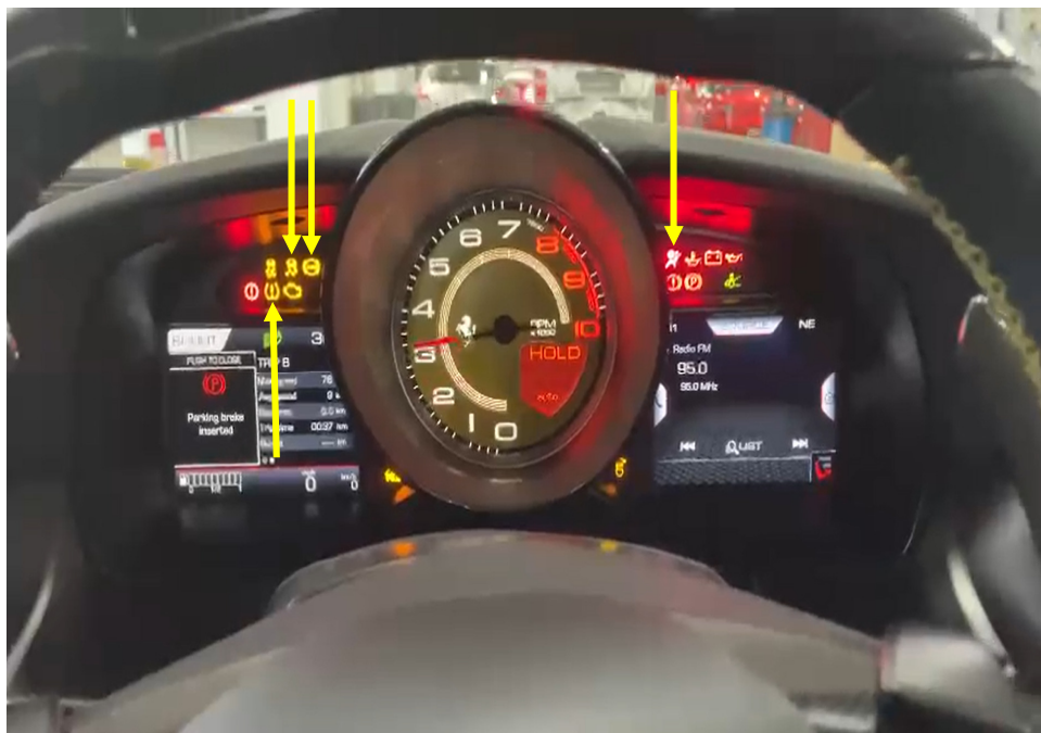
Photo 24 shows the warning lights for the various electronic safety features appearing on the instrument panel of the Motor Car during its self-test when the engine is cranked, in particular the ABS, SRS, TPM and TCS lights (arrowed).
