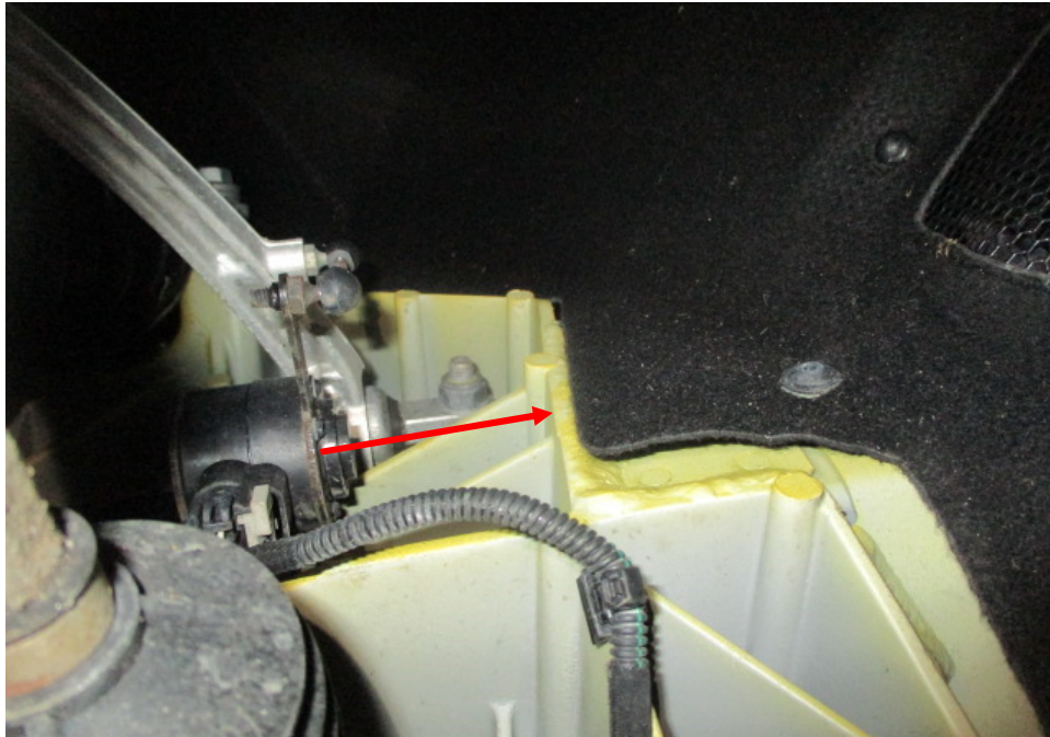
Photo 37 shows the aluminium chassis/structural body at the underside front right of the Motor Car. I did not find any weld marks other than original spot weld marks on the aluminium chassis/structural body of the Motor Car. The original factory sealant (arrowed) at the joints along the aluminium chassis/structural body was untouched, indicating no work was done on the aluminium chassis/structural body of the Motor Car and that the aluminium chassis/structural body was originally fitted.
