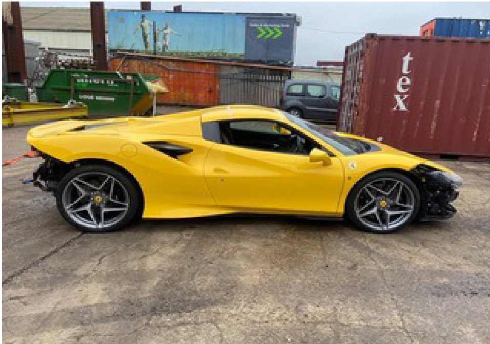
Photo 4 shows the right side body of the Motor Car (photograph provided to me). Apart for the rear portion, the Motor Car's front bumper and all its related parts and attachments like the front bumper centre garnish, front bumper sensors and front bumper right lower lip amongst others were missing/dislodged/damaged.
