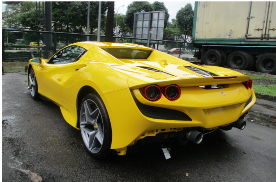
Photo 6 shows a general view of the rear left body of the Motor Car at the time of my inspection, with its rear bumper lower diffuser and rear under cover removed to facilitate checks of its engine compartment and exhaust system. The body parts at the rear portion of the Motor Car were visually examined and it was observed that the repair/restoration works carried out to the damaged area of the Motor Car (refer to photograph 1 & 2 above) were reasonably adequate and in order.
