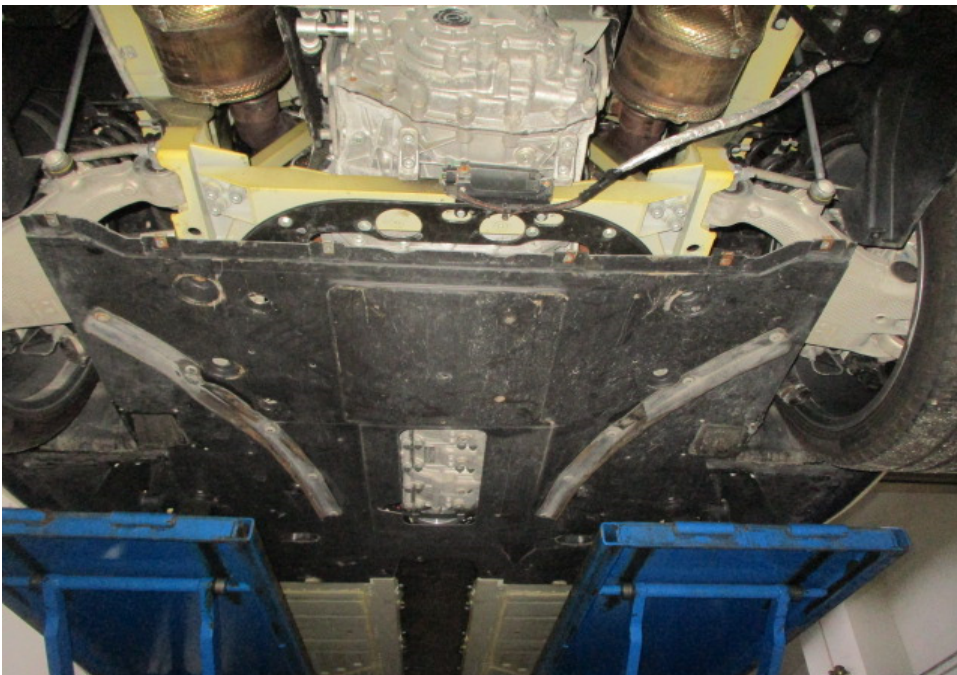
Photo 32 shows the Motor Car's engine compartment as viewed from the rear underside of the Motor Car. The various parts and components inside the engine compartment were all observed to be intact and properly fitted. There was also no sign(s) or indication(s) of fluid leak and/or fluid stain found inside the engine compartment.
