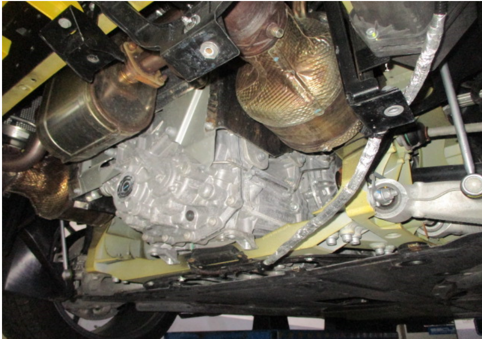
Photo 33 shows another view of the Motor Car's engine compartment as viewed from the rear underside of the Motor Car. The various parts and components inside the engine compartment were all observed to be intact and properly fitted. There was also no sign(s) or indication(s) of fluid leak and/or fluid stain found inside the engine compartment.
