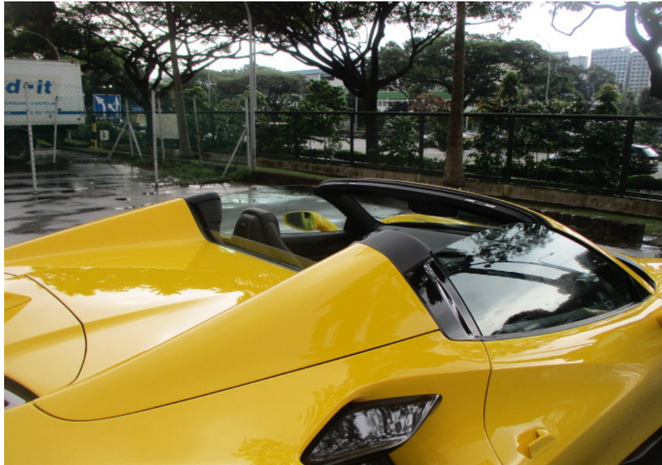
Photo 23 shows the Motor Car with its hard top roof completely folded. It was observed that as a safety feature, the hard top roof could only open and close when the Motor Car was in a stationary position or at low travelling speed. When opened, the hard top roof is completely folded into the rear compartment with no parts protruding out of the Motor Car's body. The hard top roof was also found adequately secured to the "A" pillar after closing.
