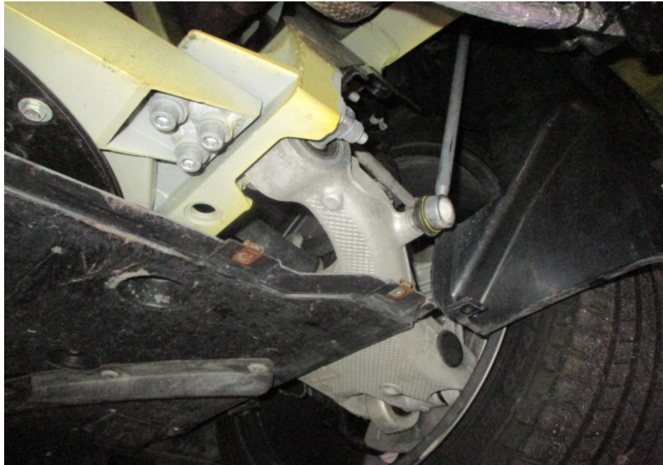
Photo 27 shows a general view of the control arms and linkages at the rear right wheel of the Motor Car. I did not observe any fluid leak and/or fluid stain on the underside of the Motor Car. All of the Motor Car's undercarriage components were observed to be intact and secured in an appropriate manner.
