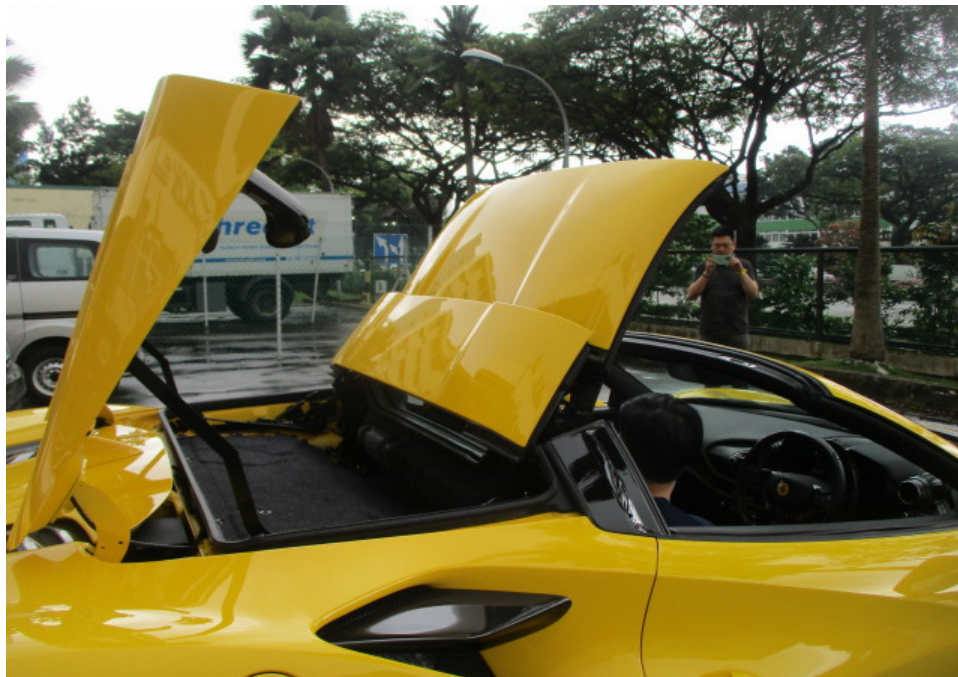
Photo 22 shows the Motor Car's hard top roof being tested. It was observed that as a safety feature, the hard top roof could only open and close when the Motor Car was in a stationary position or at low travelling speed. When opened, the hard top roof is completely folded into the rear compartment with no parts protruding out of the Motor Car's body. The hard top roof was also found adequately secured to the "A" pillar after closing.
