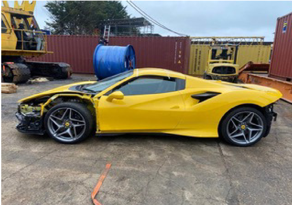
Photo 3 shows the left side body of the Motor Car (photograph provided to me). Apart for the rear portion, the Motor Car's front left fender, front left headlamp, front bumper and all its related parts and attachments like the front bumper centre garnish and front bumper left lower lip amongst others were missing/dislodged/damaged.
