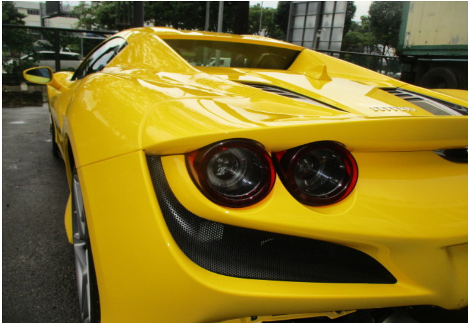
Photo 7 shows a closer view of the Motor Car's rear bumper, rear bumper left air grille, rear left outer taillamp and rear left inner taillamp. The body parts at the rear portion of the Motor Car were visually examined and it was observed that the repair/restoration works carried out to the damaged area of the Motor Car (refer to photograph 1 & 2 above) were reasonably adequate and in order.
