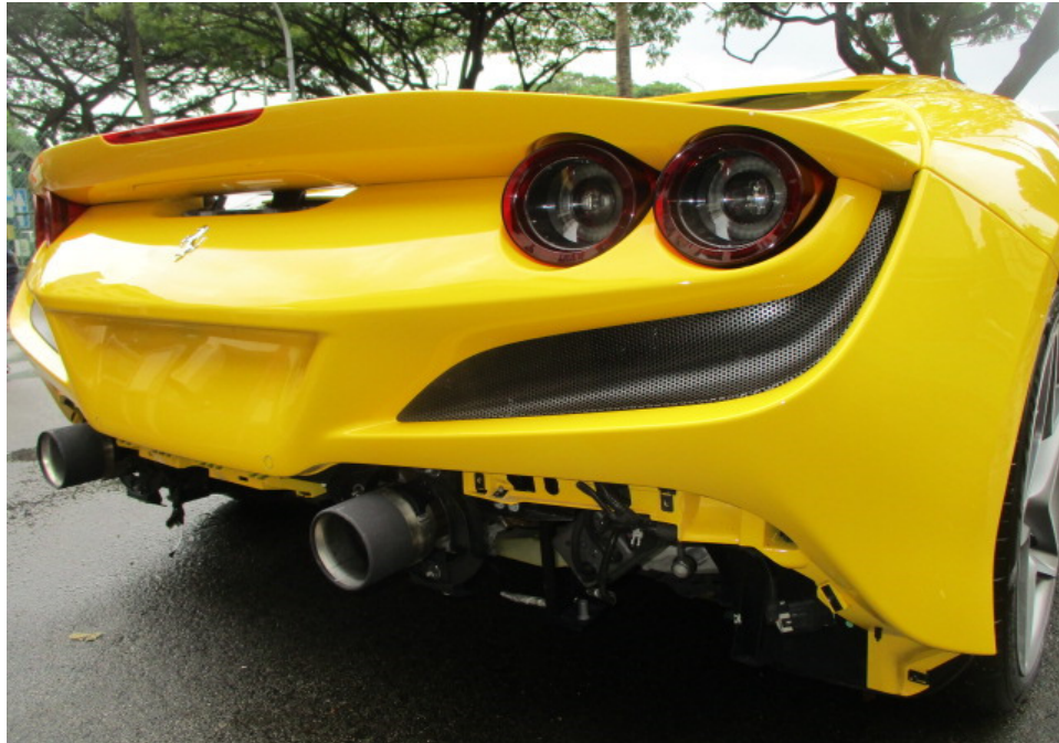
Photo 9 shows a closer view of the Motor Car's rear bumper, rear bumper right air grille, rear right outer taillamp and rear right inner taillamp. The body parts at the rear portion of the Motor Car were visually examined and it was observed that the repair/restoration works carried out to the damaged area of the Motor Car (refer to photograph 1 & 2 above) were reasonably adequate and in order.
