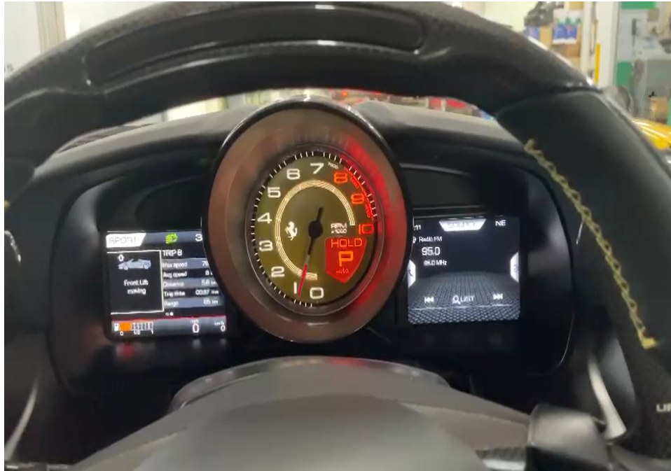
Photo 25 shows the respective warning lights no longer illuminated, indicating that there is no fault detected to the ABS, SRS TPM and TCS systems of the Motor Car during the self-test. These electronic systems were hence in working condition at the time of my inspection.
