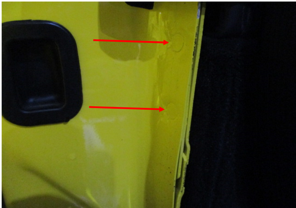
Photo 40 shows the left side "A" pillar of the Motor Car. I did not find any weld marks other than original spot weld marks (arrowed) on the left side "A" pillar of the Motor Car, which indicates that there was no re-welding works carried out. In
