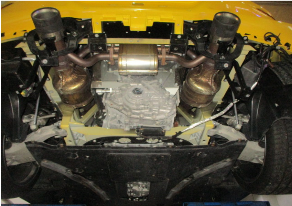
Photo 31 shows the Motor Car's exhaust system after removal of the rear bumper diffuser and rear under cover. In general, my examination of the Motor Car's exhaust system revealed no sign(s) or indication(s) of any cut or weld marks along its exhaust pipes, on its catalytic converters and on its rear mufflers.
