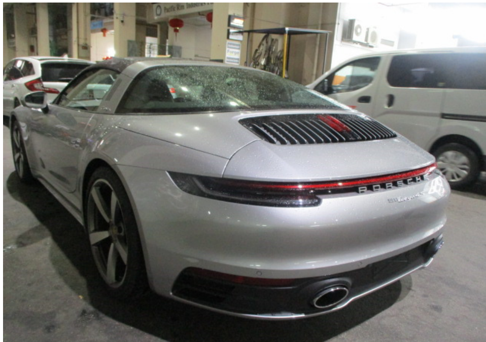
Photo 16 shows a general view of the rear left body of the Motor Car at the time of my inspection. The Motor Car was observed to be in a relatively good general condition with no loose exterior fittings observed. The body parts at the rear portion of the Motor Car were visually examined and it was observed that the repair/restoration works carried out to the damaged area of the Motor Car (refer to photograph 4 above) were reasonably adequate and in order.
