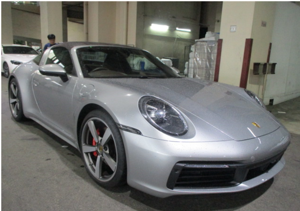
Photo 10 shows a general view of the front right body of the Motor Car at the time of my inspection. The Motor Car was observed to be in a relatively good general condition with no loose exterior fittings observed. The body parts at the frontal portion of the Motor Car were visually examined and it was observed that the repair/restoration works carried out to the damaged area of the Motor Car (refer to photograph 2 above) were reasonably adequate and in order.
