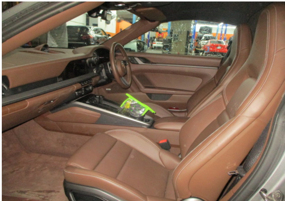
Photo 20 shows the interior compartment of the Motor Car. The front dashboard, steering wheel, seats, upholstery and trims etc were all observed to be intact and properly fitted. The body parts within the interior compartment of the Motor Car were visually examined and it was observed that the repair/restoration works carried out to the damaged area of the Motor Car (refer to photograph 5 above) were reasonably adequate and in order.
