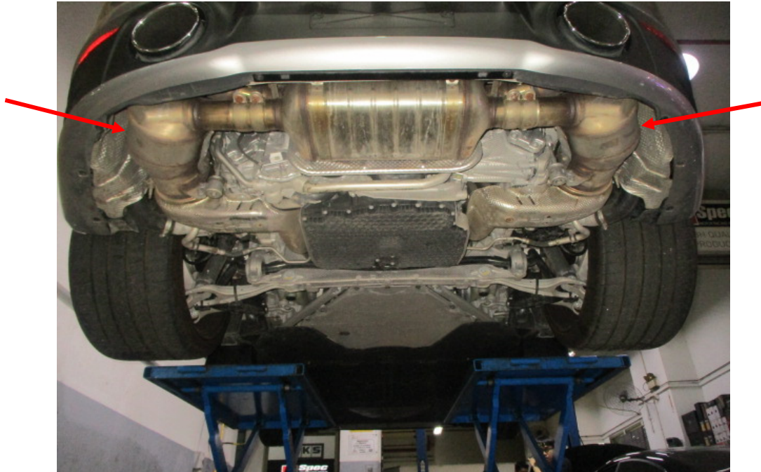
Photo 31 shows the Motor Car's exhaust system. My examination of the Motor Car's exhaust system revealed no sign(s) or indication(s) of any cut or weld marks along its exhaust pipes, on its catalytic converters (arrowed) and on its rear muffler.
