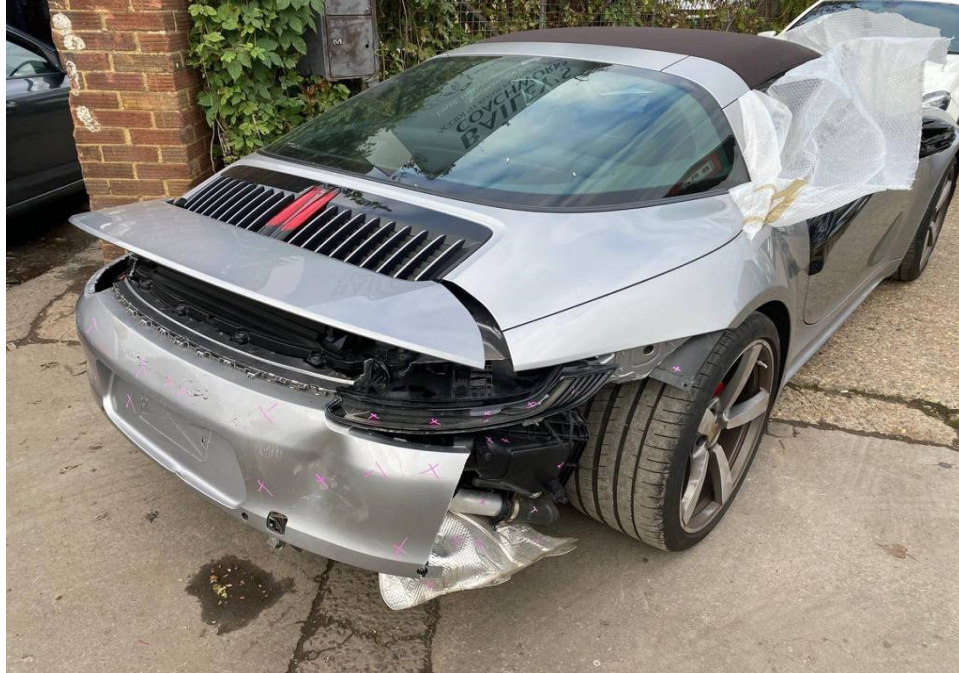
Photo 3 shows the rear right body of the Motor Car (photograph provided to me). The rear right taillamp, rear top centre reflector, rear right exhaust garnish, rear bumper lower cover, rear bumper right reflector, rear bumper tow cover and rear bumper sensors amongst others were missing/dislodged/damaged. The Motor Car's rear bumper was dented.
