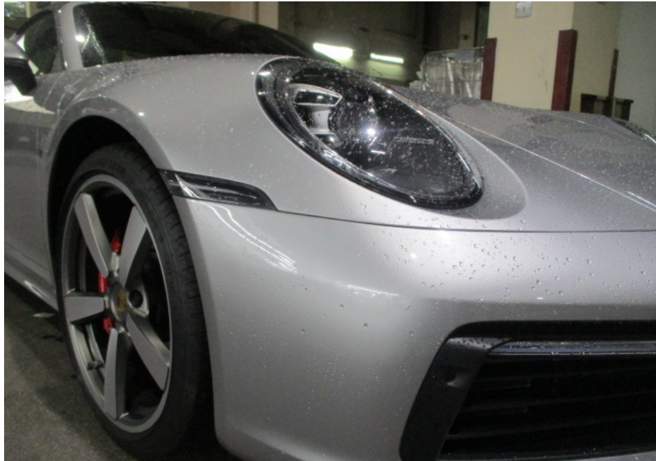
Photo 11 shows a closer view of the Motor Car's front bumper, front bumper right lower grille, front right day light, front right headlamp and front right signal lamp. The body parts at the frontal portion of the Motor Car were visually examined and it was observed that the repair/restoration works carried out to the damaged area of the Motor Car (refer to photograph 2 above) were reasonably adequate and in order.
