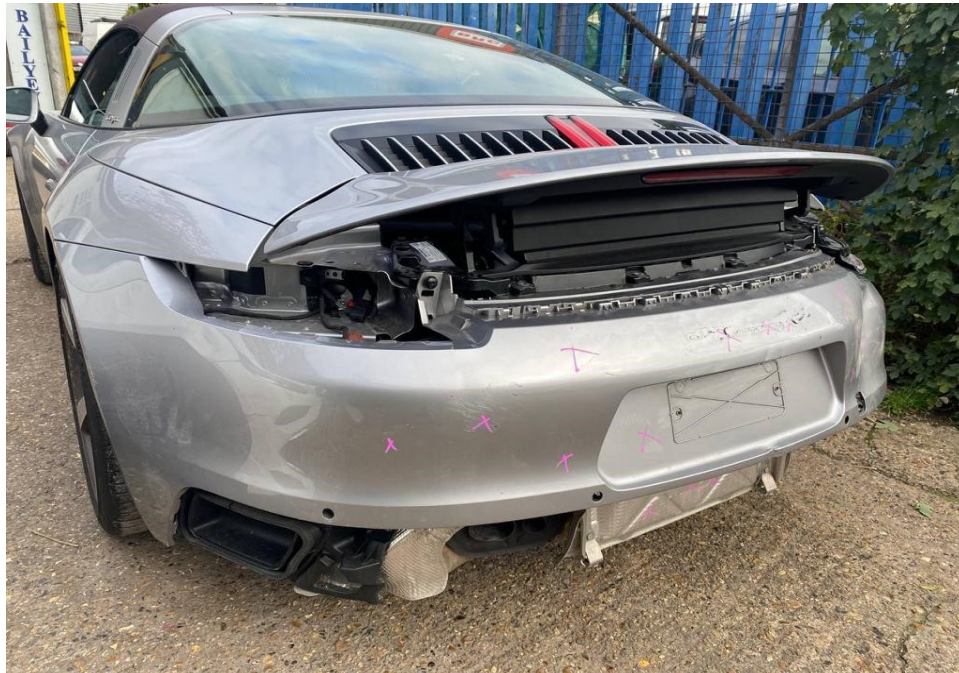
Photo 4 shows the rear left body of the Motor Car (photograph provided to me). The rear left taillamp, rear top centre reflector, rear left exhaust garnish, rear bumper lower cover, rear bumper left reflector and rear bumper sensors amongst others were missing/dislodged/damaged.
