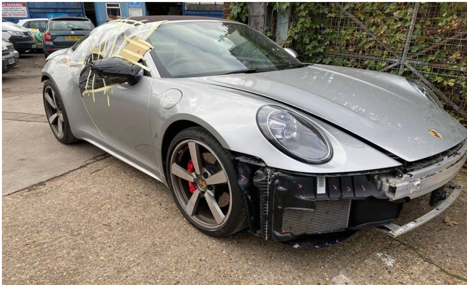
Photo 2 shows the front right body of the Motor Car (photograph provided to me). The front right signal lamp, front right day light, front bumper and all its related parts and attachments like the front bumper lower lip, front bumper sensors, front bumper tow cover, front bumper centre lower air guide and front bumper right lower grille amongst others were observed to be missing/dislodged/damaged. The Motor Car's front right door window was also observed to be shattered.
