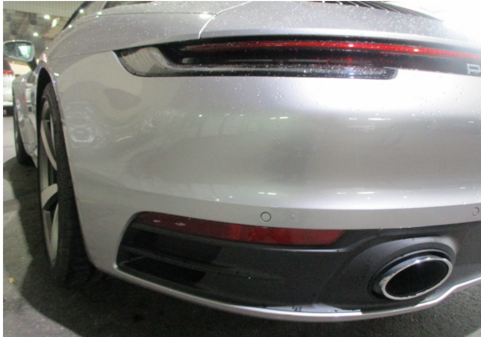
Photo 17 shows a closer view of the Motor Car's rear bumper, rear bumper left reflector, rear bumper sensor, rear left exhaust garnish and rear left taillamp. The body parts at the rear portion of the Motor Car were visually examined and it was observed that the repair/restoration works carried out to the damaged area of the Motor Car (refer to photograph 4 above) were reasonably adequate and in order.
