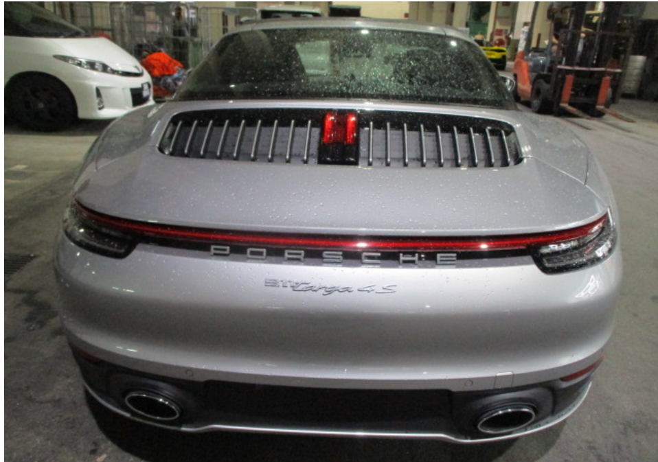
Photo 15 shows a closer view of the Motor Car's rear bumper, rear bumper lower cover and rear top centre reflector. The body parts at the rear portion of the Motor Car were visually examined and it was observed that the repair/restoration works carried out to the damaged area of the Motor Car (refer to photograph 3 & 4 above) were reasonably adequate and in order.
