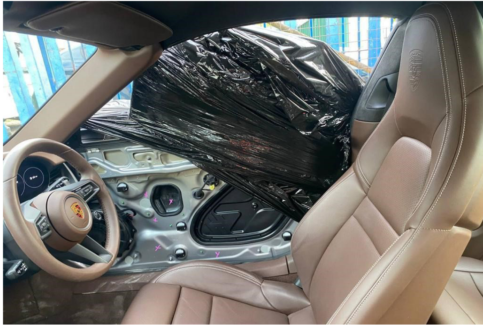
Photo 5 shows the interior compartment of the Motor Car (photograph provided to me). I had observed the front right door window shattered and the front right door inner trimboard missing/dislodged/damaged.
