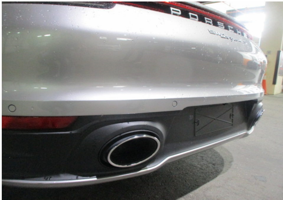
Photo 18 shows a closer view of the Motor Car's rear bumper, rear bumper lower cover, rear bumper sensors and rear left exhaust garnish. The body parts at the rear portion of the Motor Car were visually examined and it was observed that the repair/restoration works carried out to the damaged area of the Motor Car (refer to photograph 4 above) were reasonably adequate and in order.
