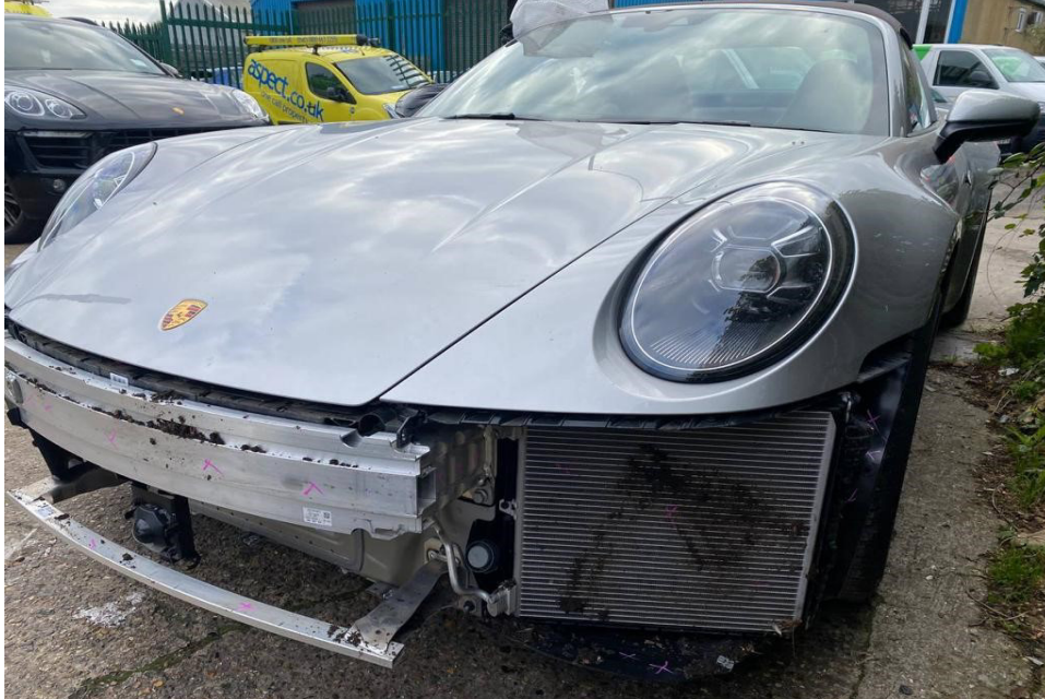
Photo 1 shows the front left body of the Motor Car (photograph provided to me). The front left signal lamp, front left day light, front bumper and all its related parts and attachments like the front bumper lower lip, front bumper sensors, front bumper tow cover, front bumper centre lower air guide and front bumper left lower grille amongst others were observed to be missing/dislodged/damaged.
