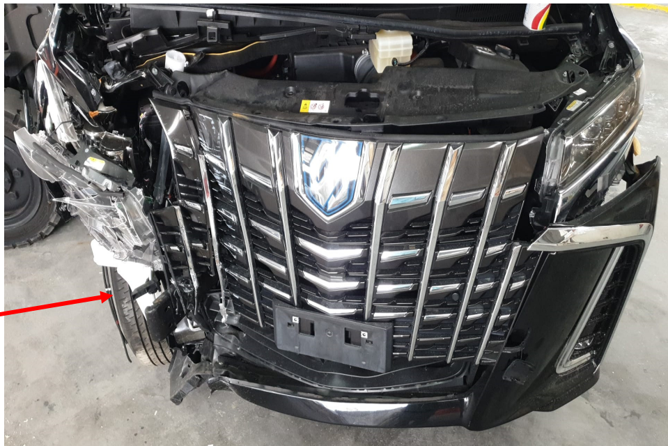
Photo 2 shows a closer view of the damage at the front right portion of the Motor Car (photograph provided to me). The front bumper, front grille, front right headlamp, front right headlamp top panel, front support panel top cover, aircon condenser and radiator were amongst the body parts that were observed to have been damaged. The front right wheel (arrowed) and front left wheel (refer to photograph 4 below) were both orientated inwards, suggesting damage to the undercarriage parts at the front right wheel of the Motor Car.
