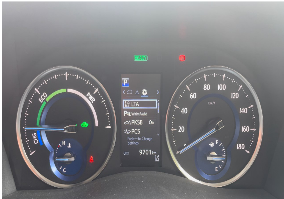
Photo 21 shows the respective warning lights no longer illuminated, indicating that there is no fault detected to the ABS, SRS, EPS, VSC and the various collision prevention systems of the Motor Car during the self-test. These electronic systems were hence in working condition at the time of my inspection.
