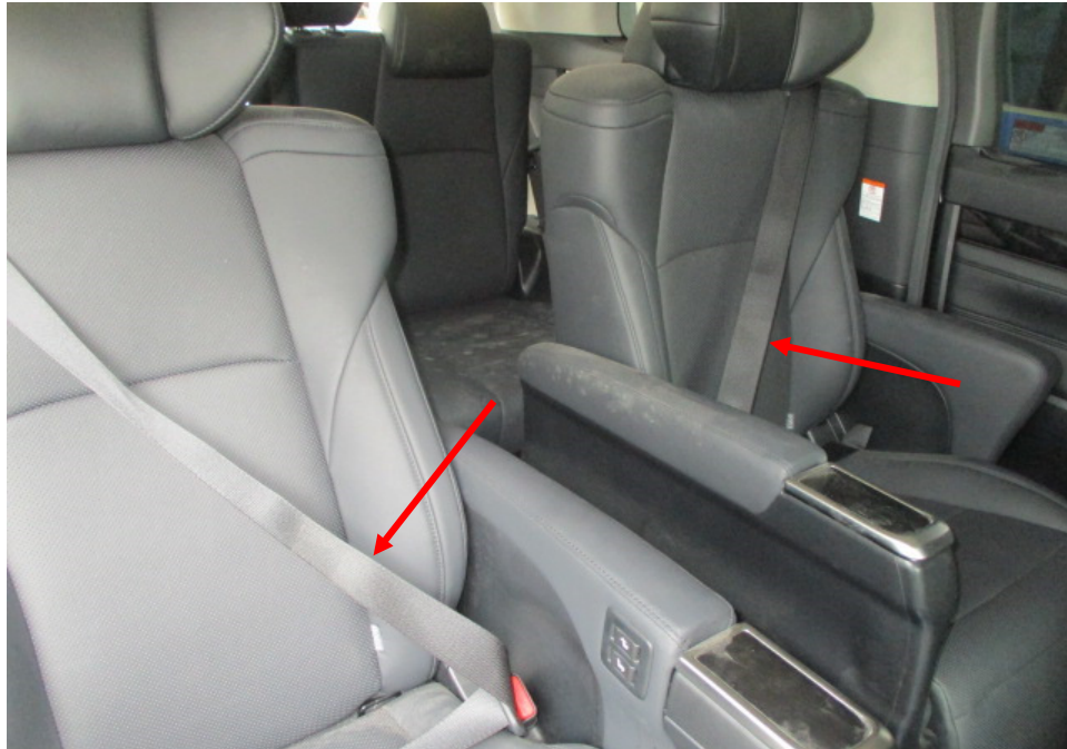
Photo 18 shows the rear seats at the 1 st row of the Motor Car. All the seats of the Motor Car were secured via seat rails to the floorboard. They were also fitted with a retractable seat belt reel and a pre-tensioner. The seat belts (arrowed) were tested and were able to be fastened into the respective pre-tensions that were fitted on the side of each individual seat.
