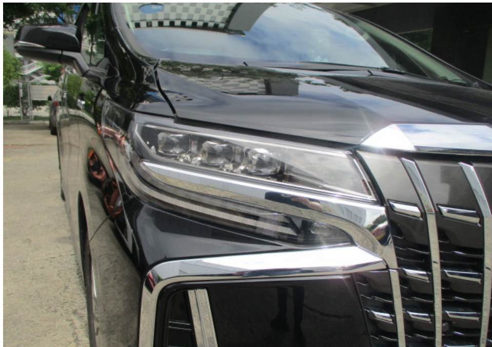
Photo 9 shows a closer view of the Motor Car's front bonnet, front right headlamp and front right headlamp chrome moulding. The body parts at the front right portion of the Motor Car were visually examined and it was observed that the repair/restoration works carried out to the damaged area of the Motor Car (refer to photograph 1 - 3 above) were reasonably adequate and in order.
