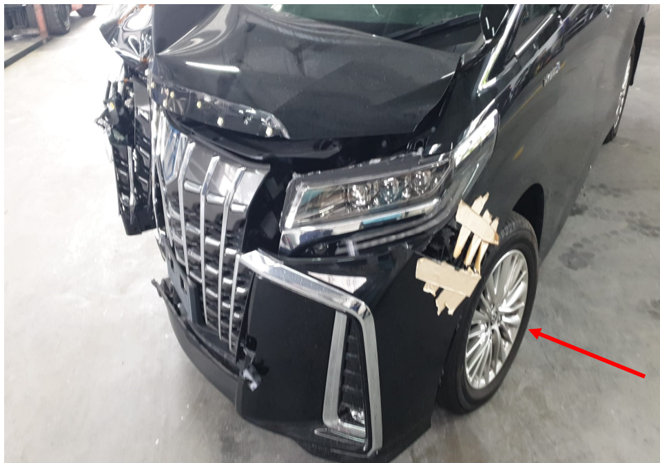
Photo 4 shows the front left body of the Motor Car (photograph provided to me). The front left wheel (arrowed) and front right wheel (refer to photograph 2 above) were both orientated inwards, suggesting damage to the undercarriage parts at the front right wheel of the Motor Car.
