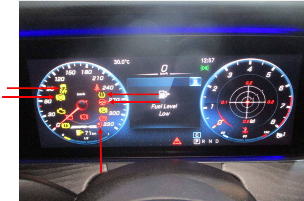
Photo 20 shows the warning lights for the various electronic safety features appearing on the instrument panel of the Motor Car during its self-test when the engine is cranked, in particular the ABS, SRS, EPS, TPM and TCS lights (arrowed).
