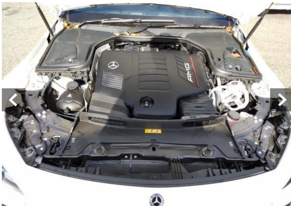
Photo 6 shows the engine compartment of the Motor Car (photograph provided to me). The various parts and components within the engine compartment were all intact and unaffected.
