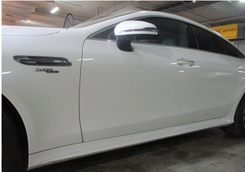
Photo 12 shows a closer view of the Motor Car's front left door, left side rocker panel garnish and left side wing mirror. The body parts at the front left portion of the Motor Car were visually examined and it was observed that the repair/restoration works carried out to the damaged area of the Motor Car (refer to photograph 1 & 2 above) were reasonably adequate and in order.
