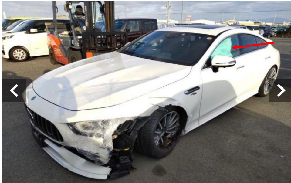
Photo 1 shows the front left body of the Motor Car (photograph provided to me). The photographs provided to me had showed damage to the front left portion of the Motor Car. The front bumper, front bumper centre lower garnish, front bumper left bracket, front bumper left lower grille, front bumper left lower grille garnish, front bumper left sensors, front left headlamp and front left fender were amongst the body parts that were observed to have been damaged. The left curtain airbag was deployed (arrowed).
