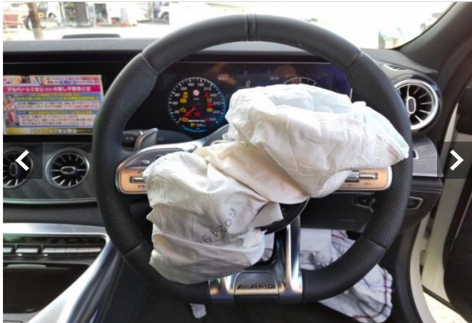
Photo 7 shows the interior compartment of the Motor Car (photograph provided to me). The driver's airbag and driver's knee airbag were deployed.
