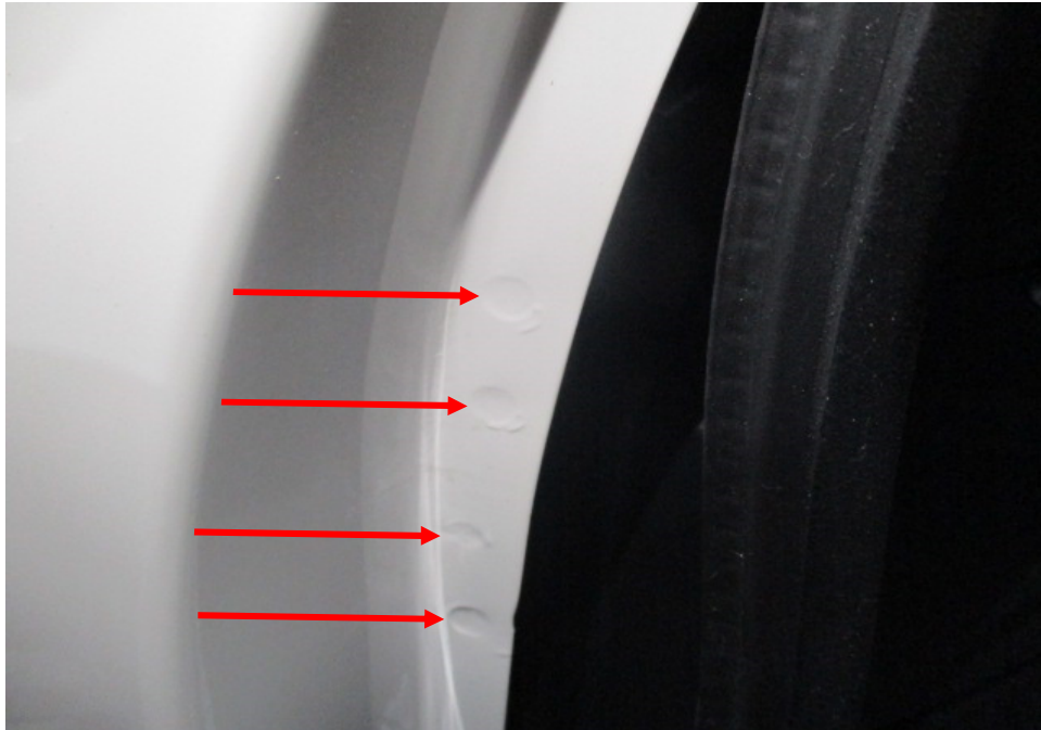
Photo 34 shows the left side "A" pillar of the Motor Car. I did not find any weld marks other than original spot weld marks (arrowed) on the left side "A" pillar of the Motor Car, which indicates that there was no re-welding works carried out. In general, I had found all the non-detachable body panels of the Motor Car to be originally fitted at the time of my inspection.
