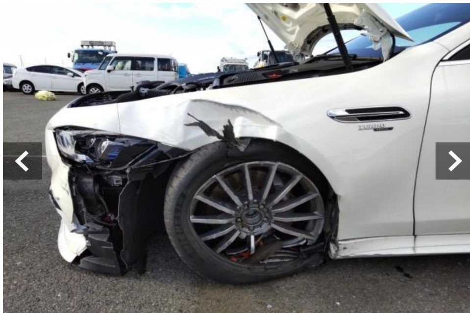
Photo 2 shows a closer view of the damage at the front left body of the Motor Car (photograph provided to me). The front bumper, front left headlamp, front left fender, front left fender inner shield, front left wheel rim, front left tyre and left side rocker panel garnish were amongst the body parts that were observed to have been damaged. The front left wheel was observed to be pushed backwards, contacting onto the body of the Motor Car. This would indicate damage to the undercarriage parts at the front left wheel of the Motor Car.
