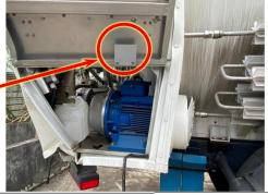
P4. Motor power cable need to disconnect out & rewiring after done repair job
