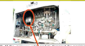
P2. All the necessary cable need to disconnect for repairing tanker canopy including from motor control pannel
