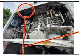
P3. Anti TOW Limit switch need to dismantle out & rewiring after done repair job
