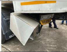
P10. Power cable storage enclosure with bracket need to dismantle out & install back with new after done repair job
