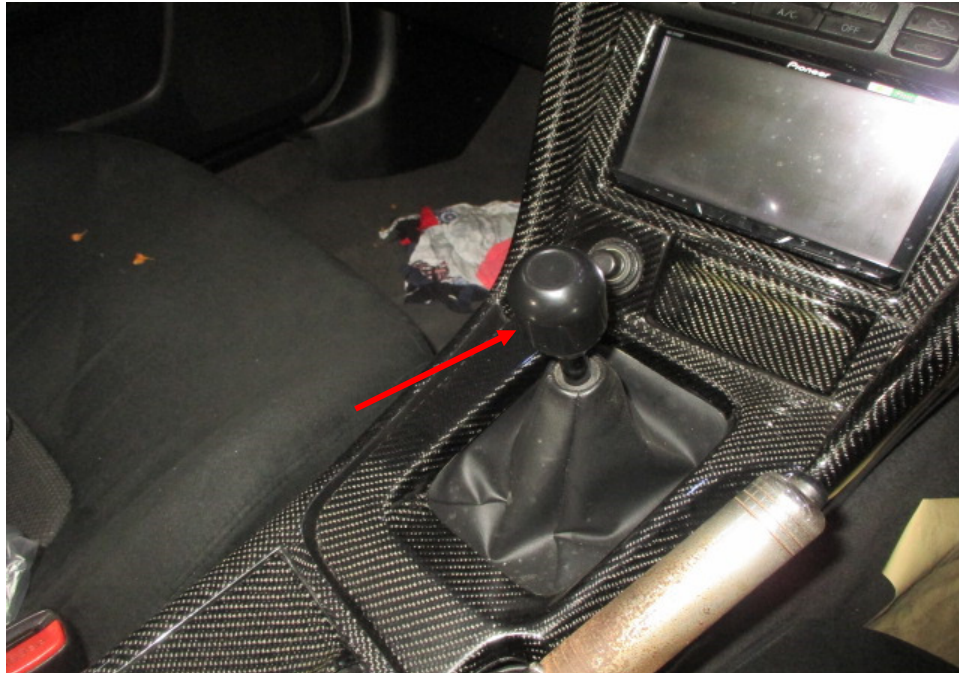
Photo 8 shows the manual gear shifter (arrowed) for manually selecting the transmission gear to be engaged.
