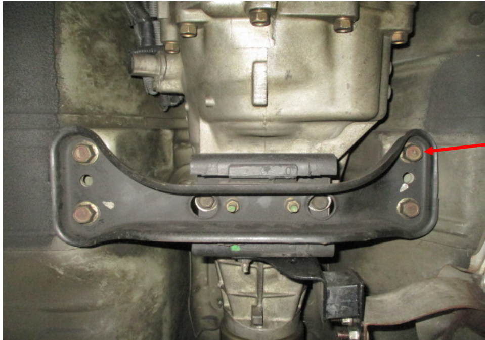
Photo 6 shows the bracket mounted to the underside of the Motor Car's floorboard, via bolts and nuts (arrowed).
