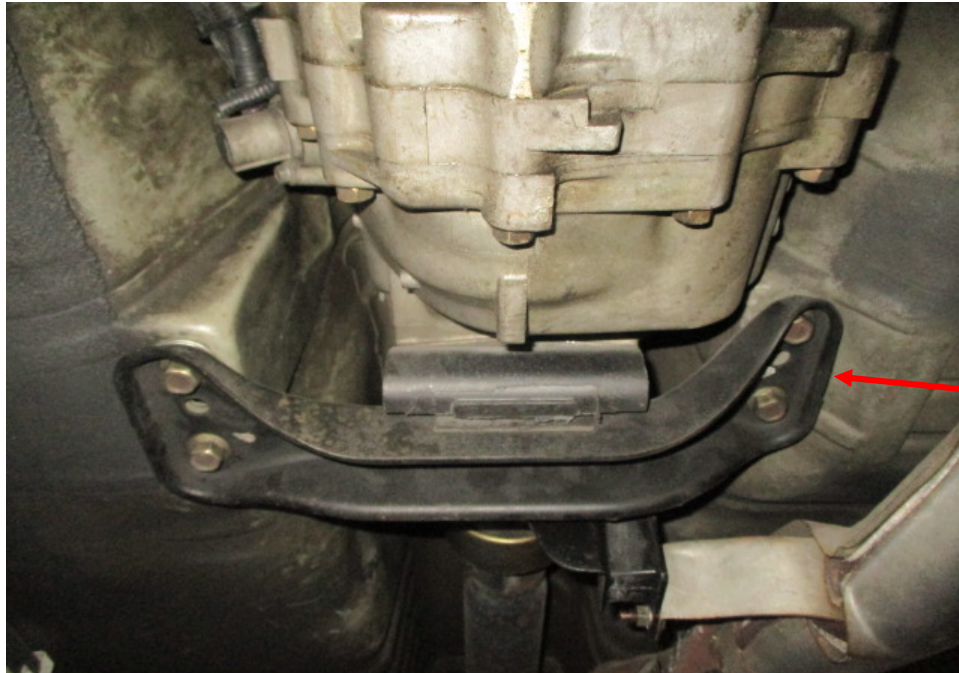
Photo 4 shows a closer view of the bracket (arrowed) that was mounted to the underside of the Motor Car's floorboard, via bolts and nuts. The bracket supports the rear (output) side of the transmission assembly. The bracket was also with rubber bushings that absorbs any vibrations arising from the rotation of the transmission gears, minimising any stress to the bracket.
