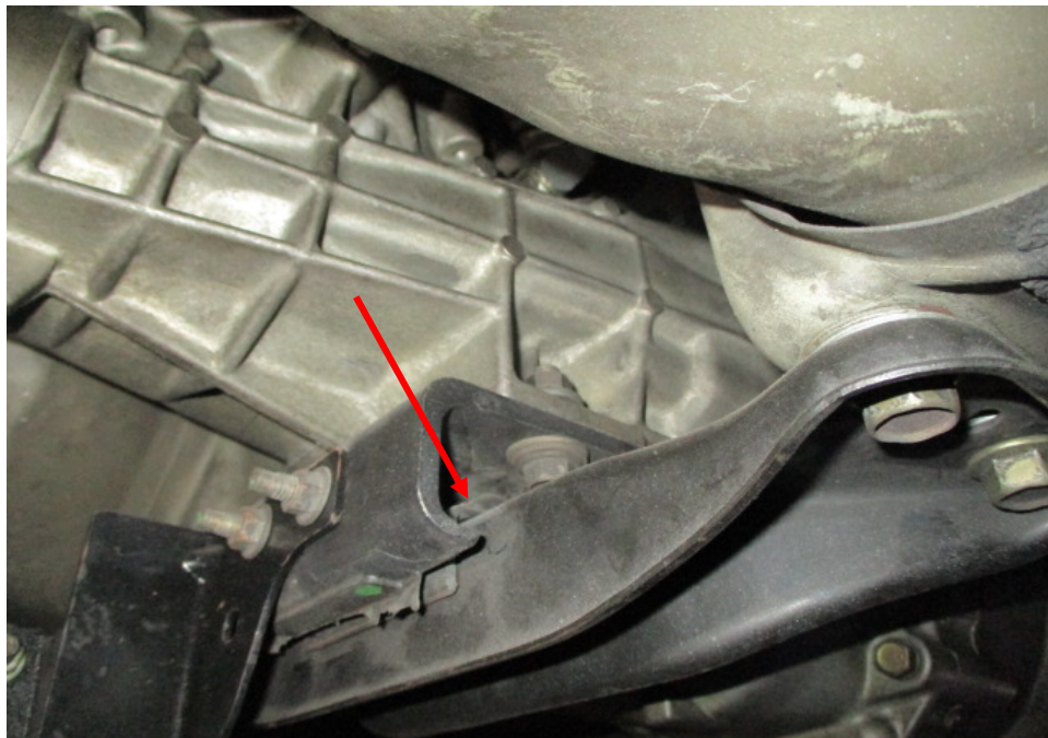
Photo 5 shows the rubber bushing (arrowed), sitting between the transmission assembly and the bracket. The rubber bushing absorbs any vibrations arising from the rotation of the transmission gears, minimising any stress to the bracket.
