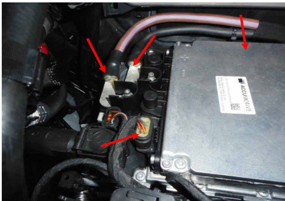
Photo 7 shows the close up view of the 48v battery and its components (arrowed) in the engine compartment portion of the Insured Vehicle at the time of our inspection. The 48v battery and its components is observed to be unaffected and by any signs of accident.
