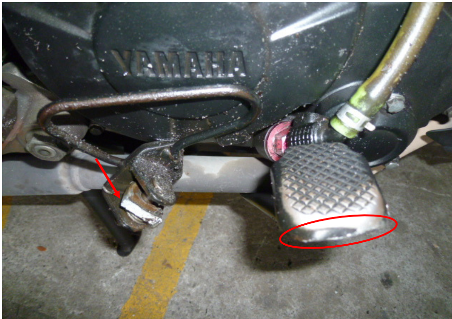
Photo 14 shows the grazed rear brake pedal (circled) and broken right front footrest (arrowed) of the Motorcycle as a result of the accident.
