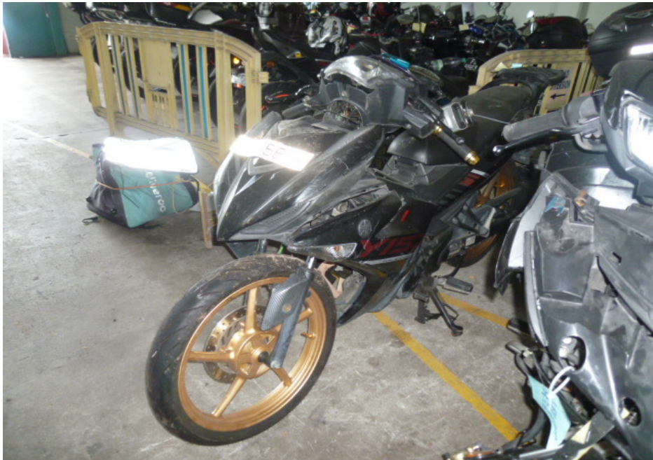
Photo 4 shows a general view of the left body of the Motorcycle at the time of our inspection. The Motorcycle was observed to have sustained damages all around. The body parts that were found to have been damaged include its headlight assembly, steering stem, side cowlings, front brake lever, centre cover, left rear side cover, exhaust muffler heat shield and top box, amongst others.
