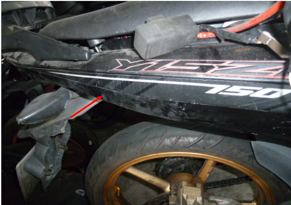
Photo 12 shows a closer view of the grazed right rear side cover of the Motorcycle as a result of the accident (arrowed).
