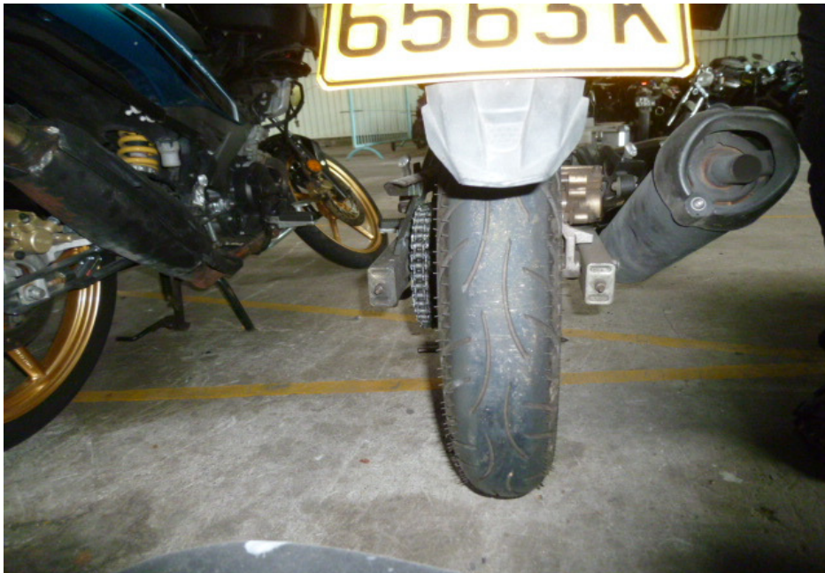
Photo 17 shows the condition of the Motorcycle's rear tyre. The pattern of the tread was clearly visible with remaining tread depth of approximately 2mm. We did not observe any tear, burst mark(s) and/or punctured hole(s) on the sidewalls as well as across the tread of the rear tyre. The tyre was also observed to be sufficiently inflated for vehicular operation.
