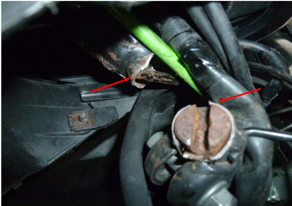
Photo 24 shows a close up view of the broken steering stem of the Motorcycle as a result of the accident (arrowed). We were hence not able to conduct any tests on the steering system of the Motorcycle.
