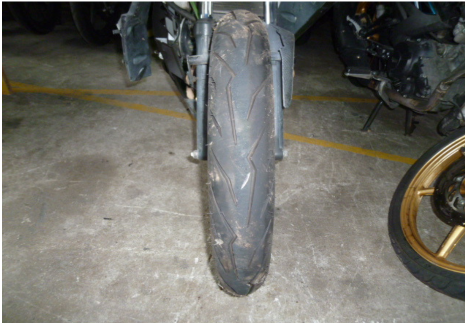
Photo 16 shows the condition of the Motorcycle's front tyre. The front tyre was observed to be in serviceable condition with remaining tread depth of approximately 4mm. The tyre was also observed to be sufficiently inflated for vehicular operation. We did not observe any tear, burst mark(s) and/or punctured hole(s) on the sidewalls as well as across the tread of the front tyre.
