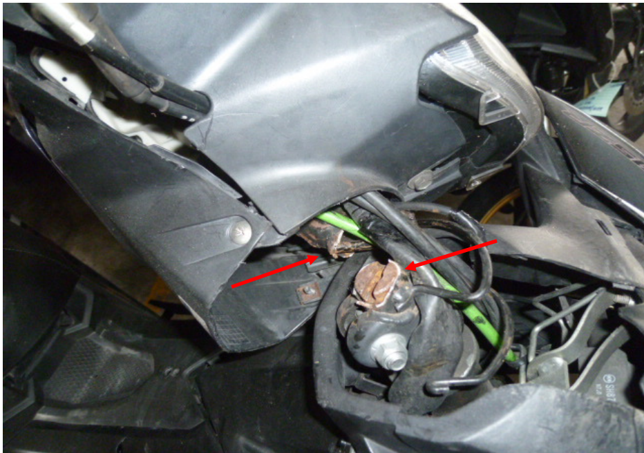
Photo 23 shows the steering stem of the Motorcycle. The steering stem was observed to be broken as a result of the accident (arrowed). We were hence not able to conduct any tests on the steering system of the Motorcycle.
