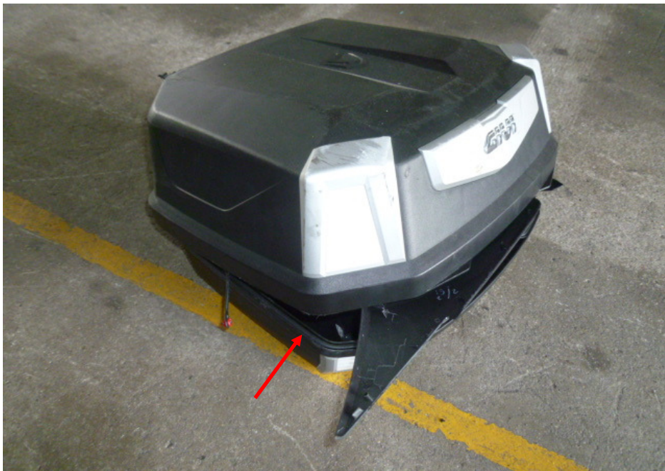
Photo 13 shows the broken top box (arrowed) of the Motorcycle a result of the accident.
