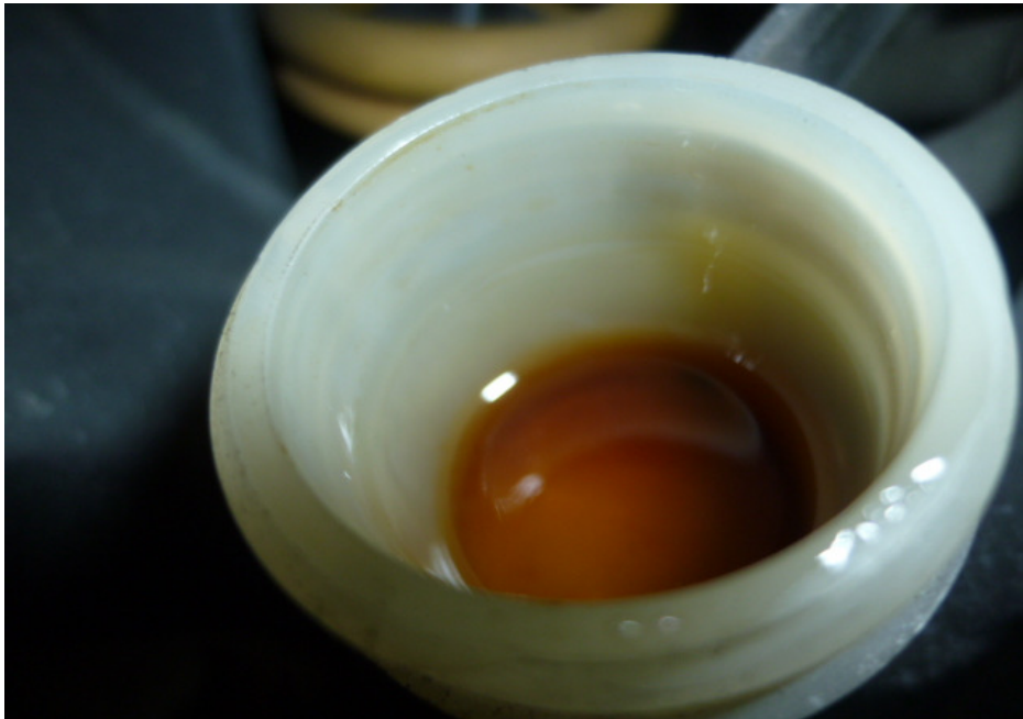
Photo 29 shows the brake fluid reservoir for the rear brake of the Motorcycle. The brake fluid was observed to be of sufficient level for operating purposes and without any contamination.
