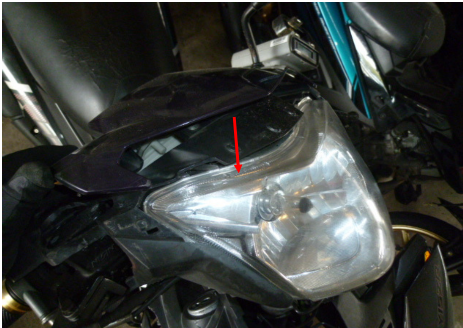
Photo 6 shows the dislodged headlight assembly (arrowed) of the Motorcycle as a result of the accident.
