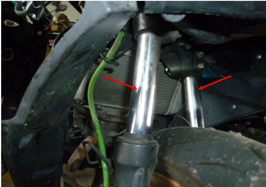
Photo 22 shows the front forks of the Motorcycle. The front forks were observed to be bent as a result of the accident (arrowed). We were hence not able to conduct any tests on the steering system of the Motorcycle.
