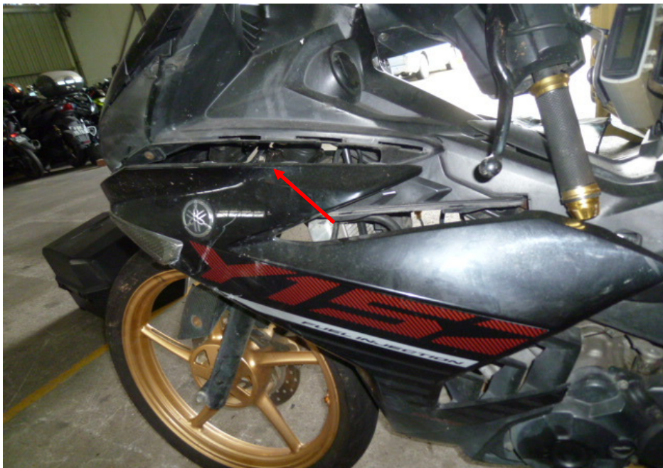
Photo 11 shows a closer view of the dislodged left cowling of the Motorcycle as a result of the accident (arrowed).
