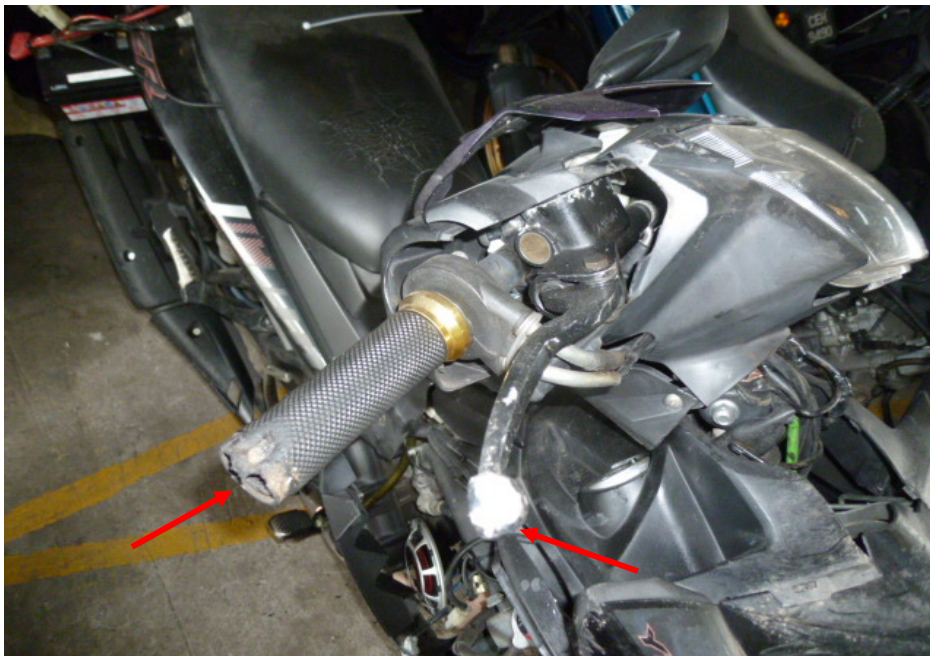
Photo 9 shows the right handlebar end and front brake lever (arrowed), which were amongst the body parts of the Motorcycle that had sustained damage as a result of the accident.
