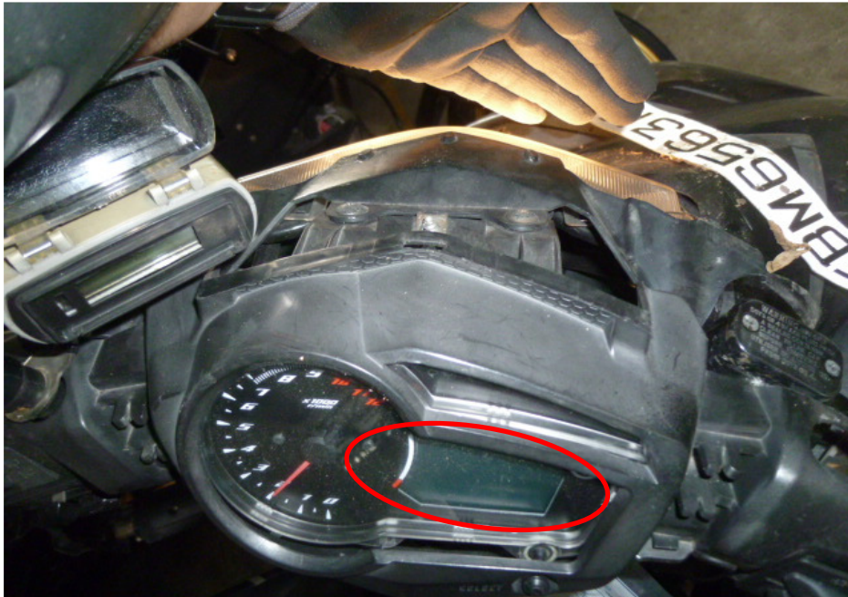
Photo 1 shows the speedometer gauge of the Motorcycle. The mileage of the Motorcycle could not be recorded at the time of our inspection due to a damaged display screen (circled).
