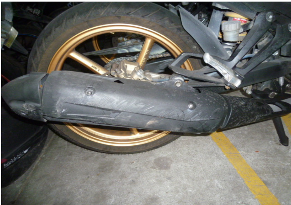
Photo 15 shows the grazed exhaust muffler heat shield of the Motorcycle as a result of the accident.
