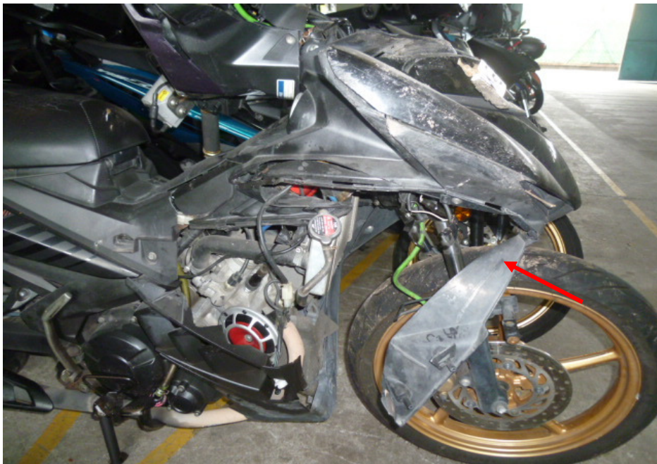
Photo 7 shows a closer view of the cracked right cowling of the Motorcycle as a result of the accident (arrowed).
