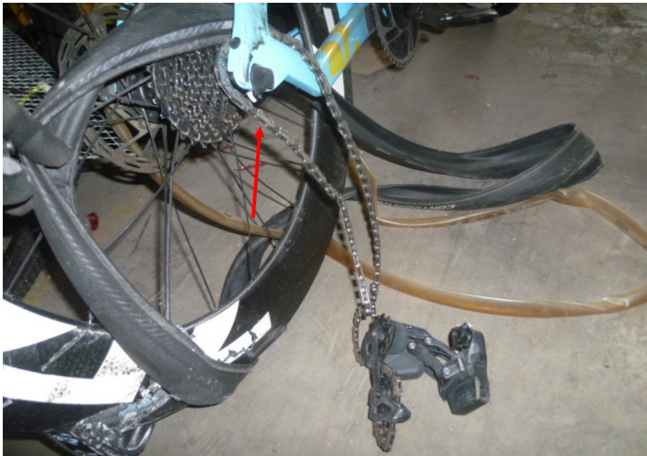
Photo 15 shows a close up view of the dislodged chain of the Bicycle as a result of the accident (arrowed). No free play tension test can be conducted due to the extensive damages.
