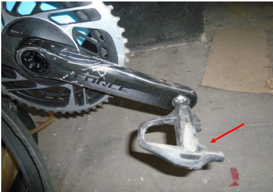
Photo 8 shows a close-up view of the broken right pedal of the Bicycle as a result of the accident (arrowed).
