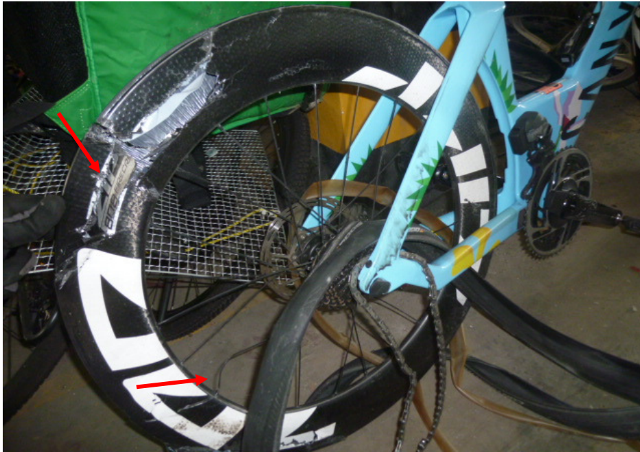
Photo 13 shows the bent spokes and broken rear wheel rim of the Bicycle at the time of our inspection (arrowed).
