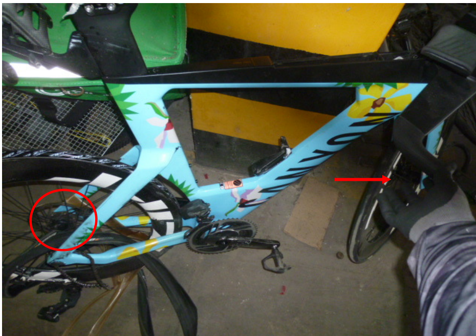
Photo 19 shows a static brake test conducted on the Bicycle's rear brake. There was no resistance felt upon pressing the right hand brake lever (arrowed). It also shows that the rear brake clamps had not responded to the gripping action (circled) after depressing the right hand brake lever.
