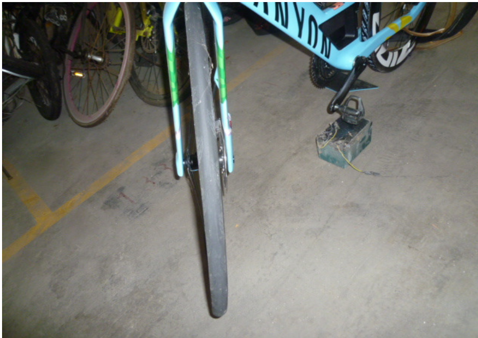
Photo 10 shows the front tyre of the Bicycle most likely as a result of the accident. The pattern of the tread was clearly visible. There was no tear, burst mark(s) and/or punctured hole(s) on the sidewalls as well as across the tread of the front tyre.
