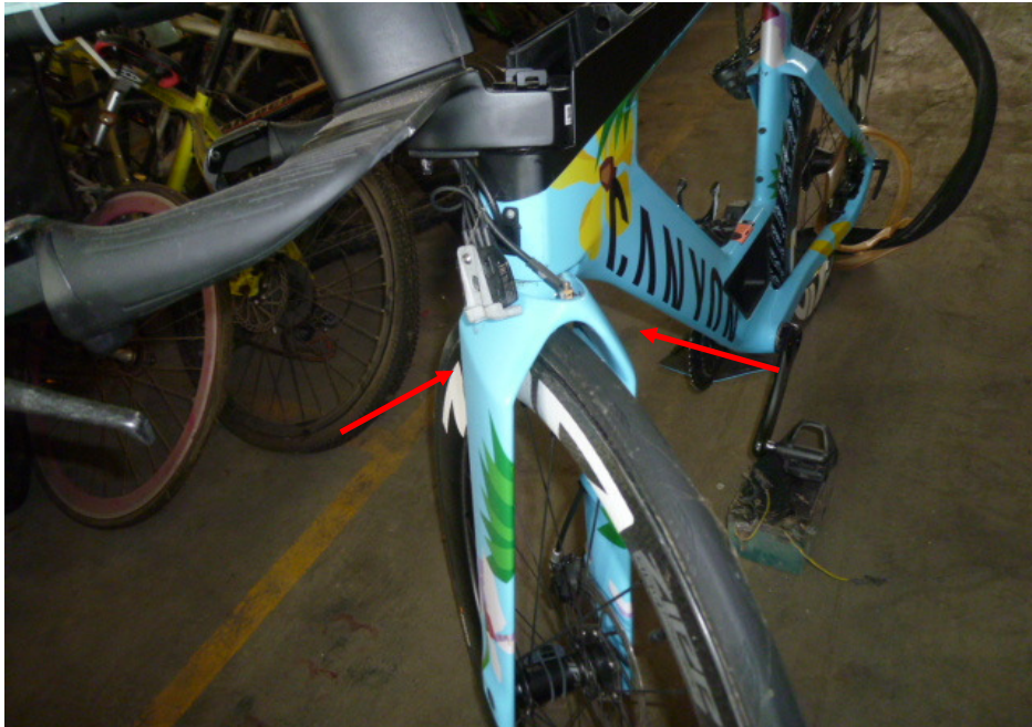
Photo 16 shows the front fork assembly (arrowed) of the Bicycle. The front forks and fork bracket of the Bicycle were both found to be bent as a result of the accident, hence causing the whole steering system to be out of alignment and rendering the Bicycle immobile for any static or operational tests.
