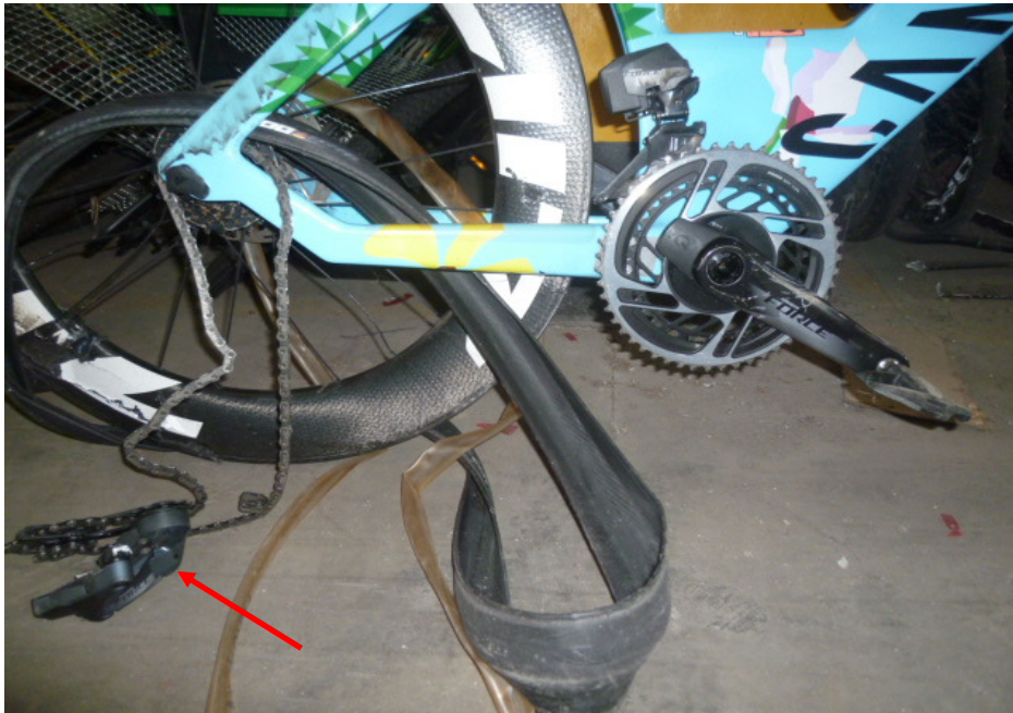
Photo 14 shows the general view of the gear train of the Bicycle which was found to be broken as a result of the accident (arrowed). The chain was also observed to be dislodged from the gear train most likely as a result of the accident.
