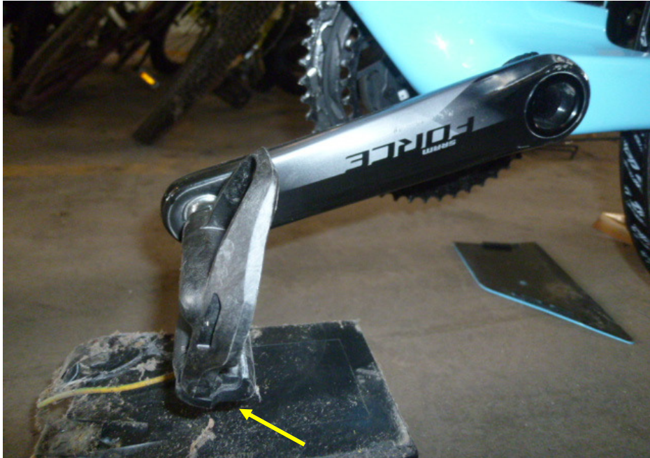
Photo 7 shows the grazed left pedal of the Bicycle as a result of the accident (arrowed).
