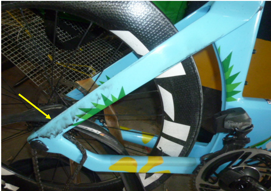
Photo 9 shows the grazed right rear sub frame of the Bicycle as a result of the accident (arrowed).
