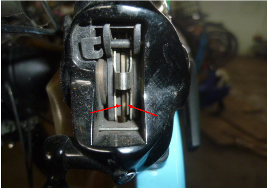
Photo 20 shows a close up view of the rear brake pads not responding to the gripping action. The rear brake pads did not press against the rear brake disc (arrowed) upon depressing the right hand brake lever. This had appeared to indicate that the rear brake of the Bicycle was not in serviceable condition.
