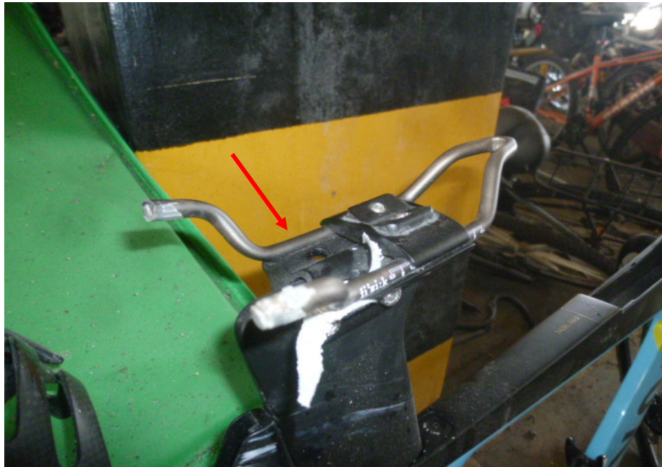
Photo 5 shows the dislodged seat of the Bicycle at the time of our inspection (arrowed).
