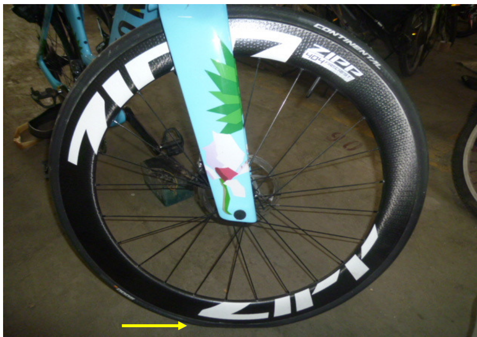
Photo 11 shows the deflated front tyre of the Bicycle at the time of our inspection (arrowed).
