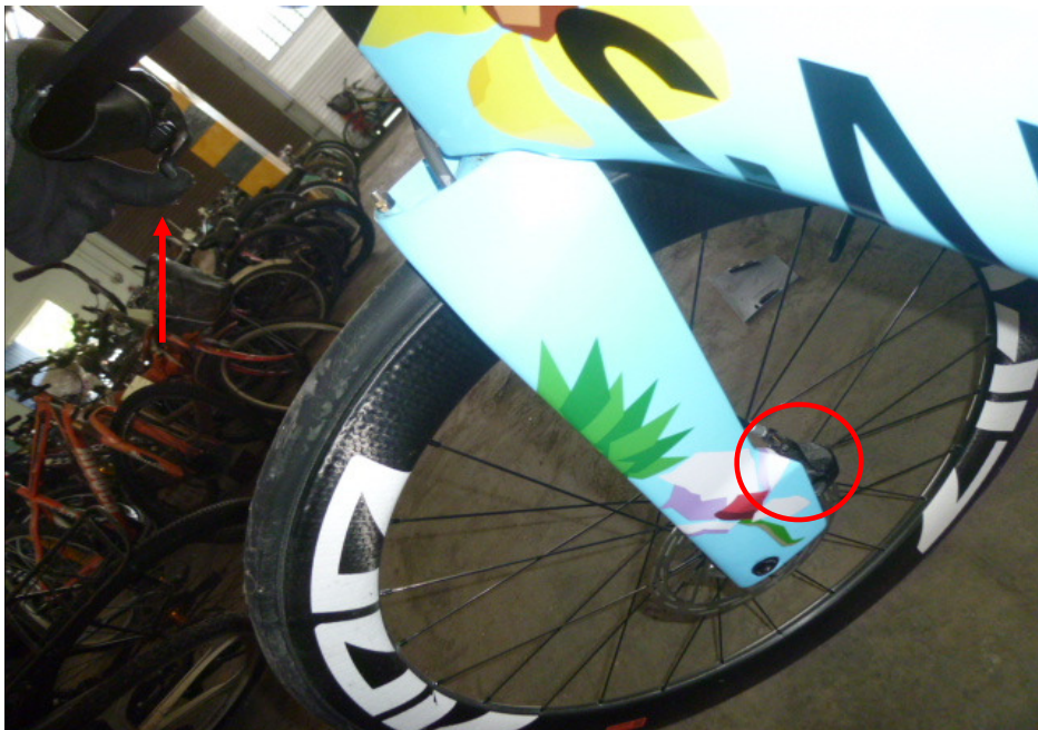
Photo 17 shows a static brake test conducted on the Bicycle's front brake. There was no resistance felt upon pressing the left hand brake lever (arrowed). It also shows that the front brake clamps had not responded to the gripping action (circled) after depressing the left hand brake lever.
