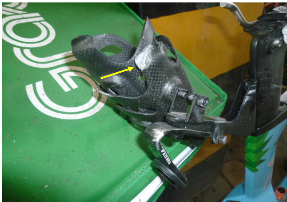
Photo 6 shows a close-up view of the deformed water bottle holder of the Bicycle as a result of the accident (arrowed).
