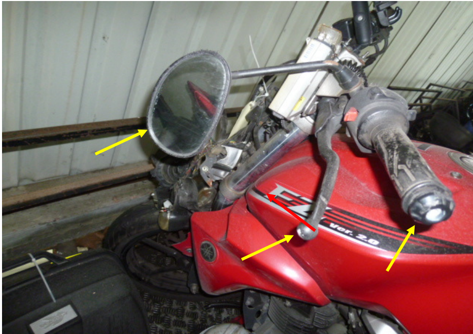
Photo 11 shows the left side mirror, clutch lever and left handlebar end (arrowed) of the Motorcycle that had sustained damage as a result of the accident.
