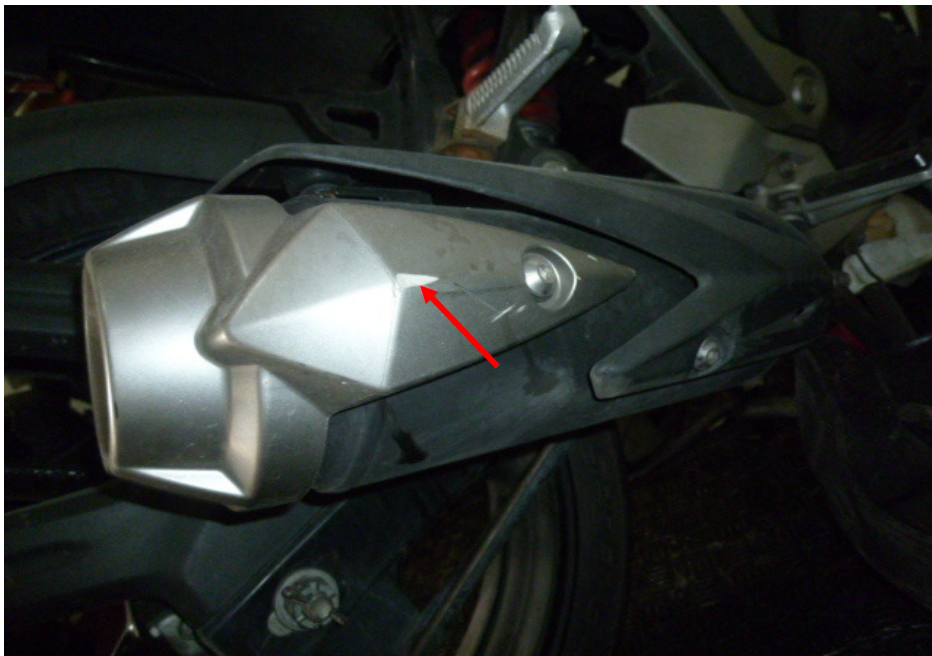
Photo 12 shows a closer view of the exhaust muffler heat shield which was amongst the body parts of the Motorcycle that had sustained damages of grazing nature as a result of the accident (arrowed).
