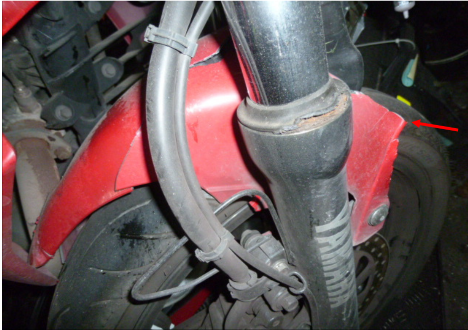
Photo 5 shows a closer view of the cracked front mudguard of the Motorcycle as
