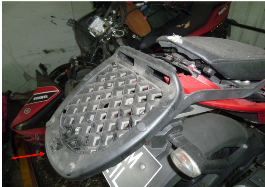
Photo 10 shows the deformed top box rack (arrowed) of the Motorcycle as a result of the accident.
