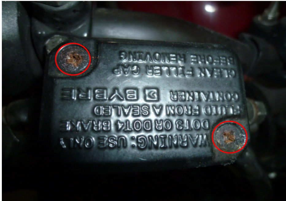
Photo 22 shows the brake fluid reservoir cover for the front brake of the Motorcycle. We were unable to examine whether the front brake fluid was without contamination due to worn out screws (circled).
