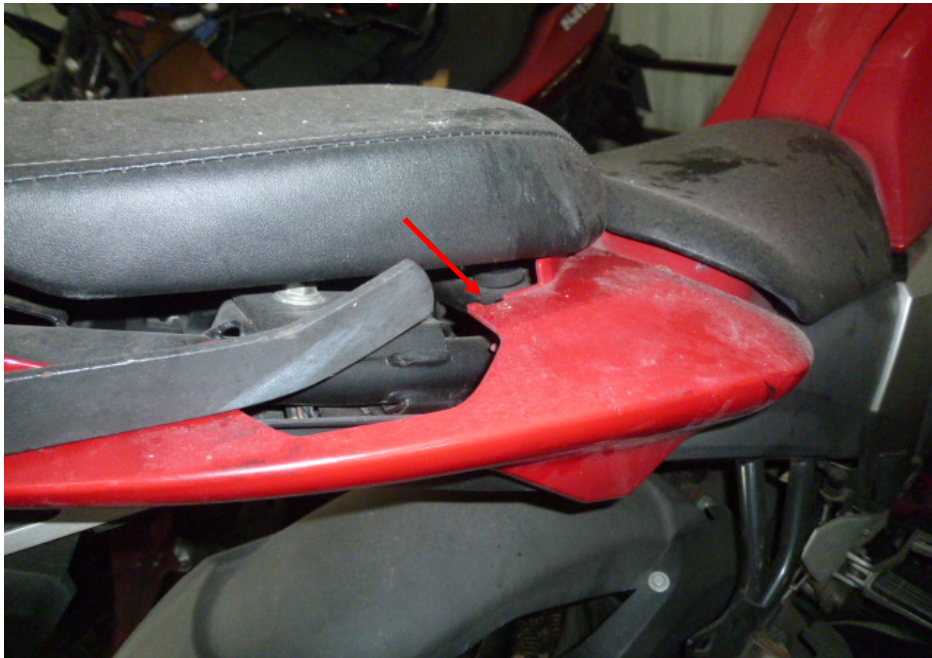
Photo 7 shows a closer view of the dislodged right rear side cover (arrowed) of the Motorcycle as a result of the accident.
