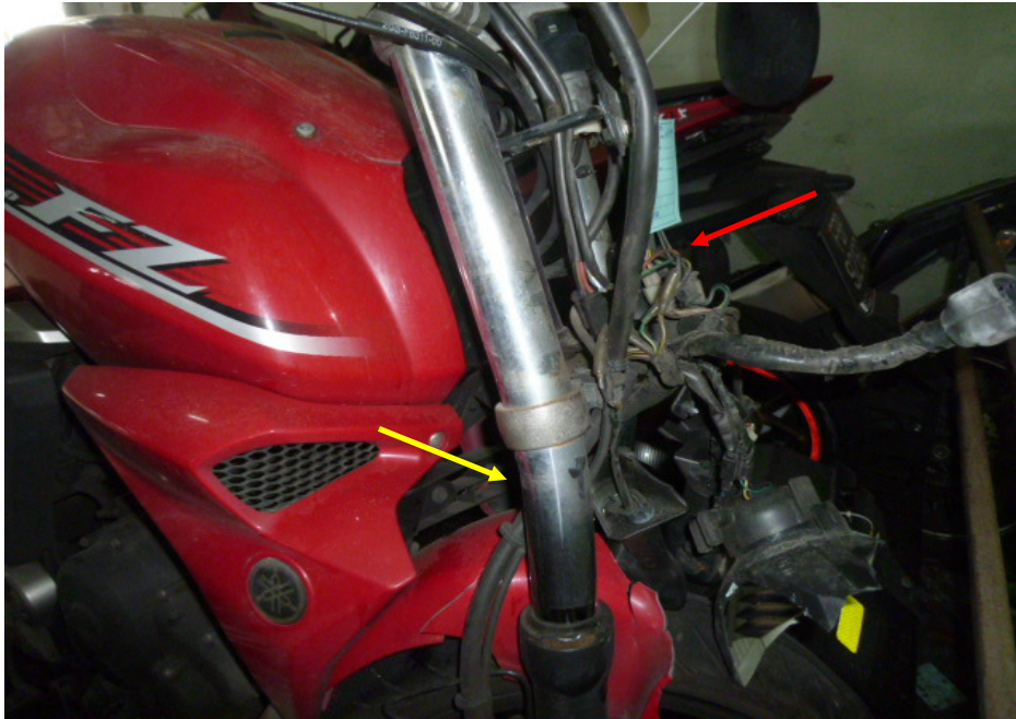
Photo 20 shows the front forks of the Motorcycle. The front forks were observed to be bent inwards as a result of the accident (arrowed). We were hence not able to conduct any tests on the steering system of the Motorcycle.
