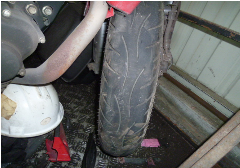
Photo 13 shows the condition of the Motorcycle's front tyre. The front tyre was observed to be in serviceable condition with remaining tread depth of approximately 3mm. There was no tear, burst mark(s) and/or punctured hole(s) on the sidewalls as well as across the tread of the front tyre. However the front tyre was observed to be deflated..
