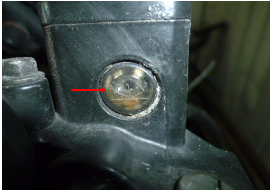
Photo 23 shows a close up view of the brake fluid reservoir for the front brake of the Motorcycle. The brake fluid was observed to be of sufficient level for operational purposes (arrowed).
