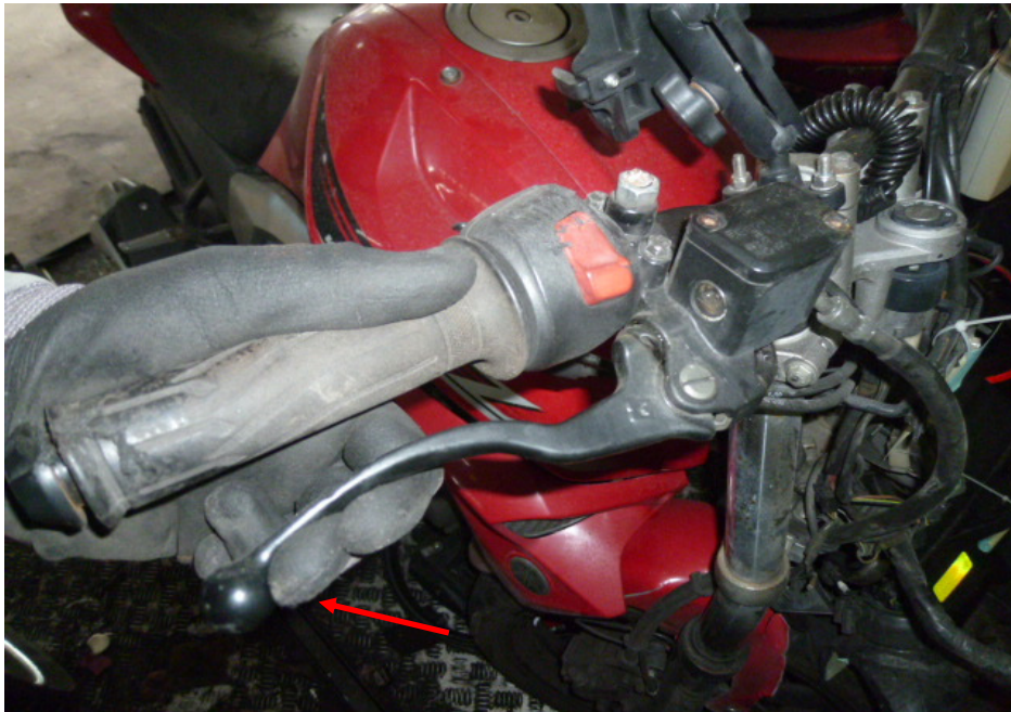
Photo 24 shows the front brake lever being depressed. There was some resistance felt (spongy like feel) upon pressing the front brake lever (arrowed). This would indicate that there is no leakage of pressure/vacuum in the brake system.
