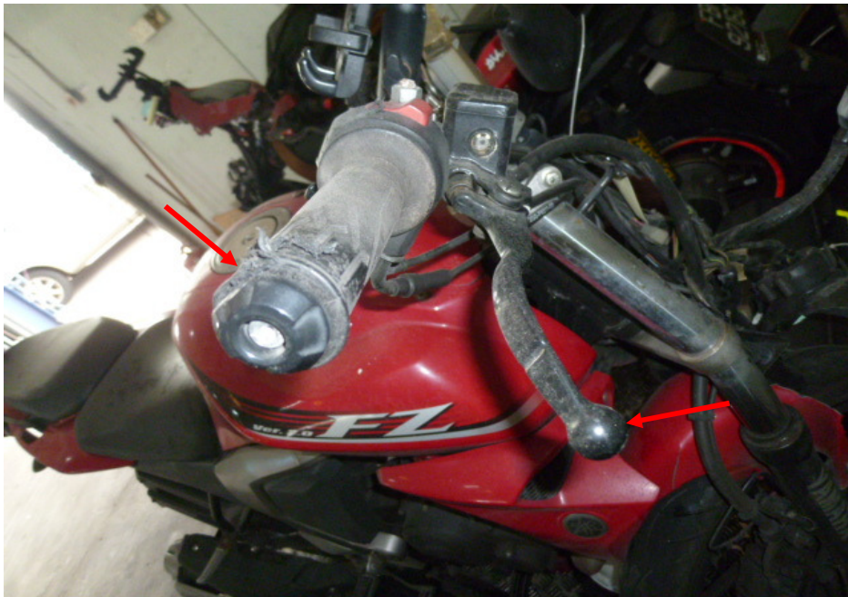
Photo 6 shows the front brake lever and right handlebar end (arrowed), which were amongst the body parts of the Motorcycle that had sustained damage as a result of the accident.
