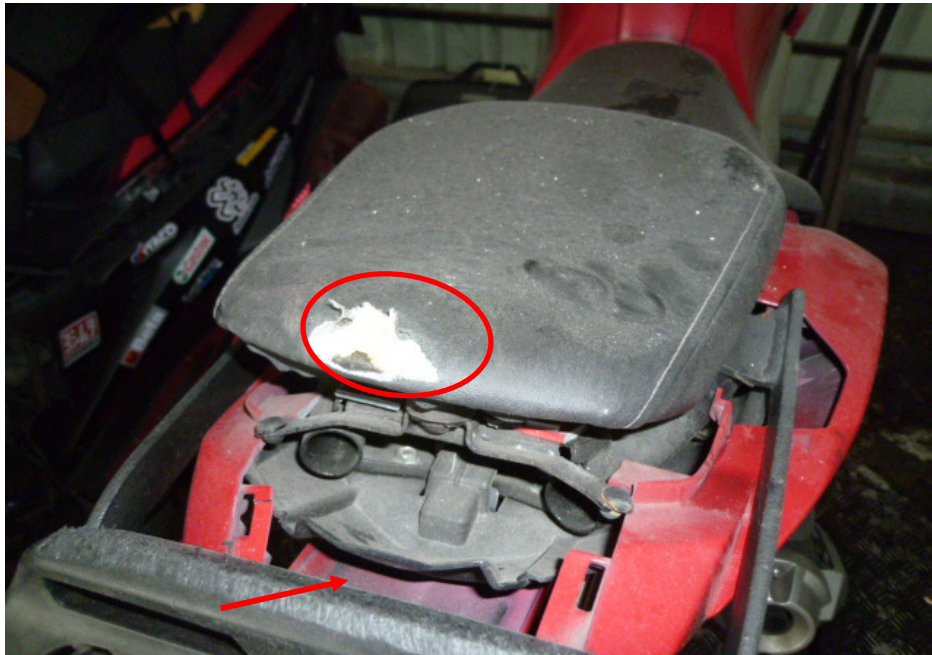
Photo 9 shows a closer view of the torn pillion seat circled) and missing tail light cover (arrowed) of the Motorcycle as a result of the accident.
