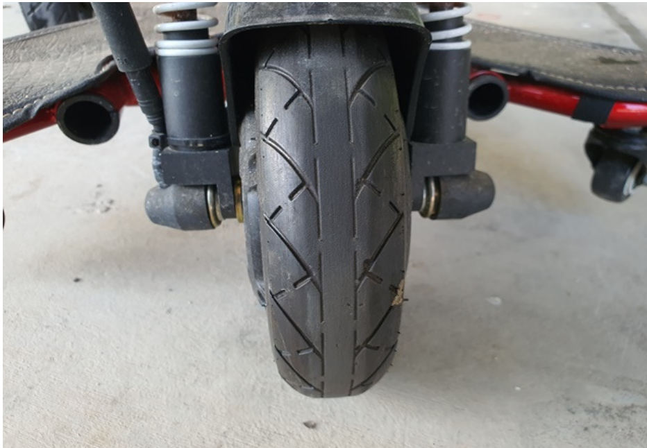
Photo 8 shows the condition of the PMA's front tyre. The front tyre was observed to be in serviceable condition. There was no tear, burst mark(s) and/or punctured hole(s) on the sidewalls as well as across the tread of the front tyre. However the front tyre was observed to be bald.
