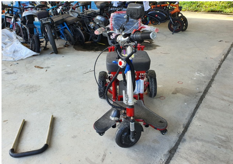
Photo 16 shows the front wheel of the PMA turned towards its full right. Turning the PMA's steering handlebar towards the right did not produce any abnormal free play and/or resistance. This would indicate that the steering system of the PMA was in serviceable condition at the time of our inspection.
