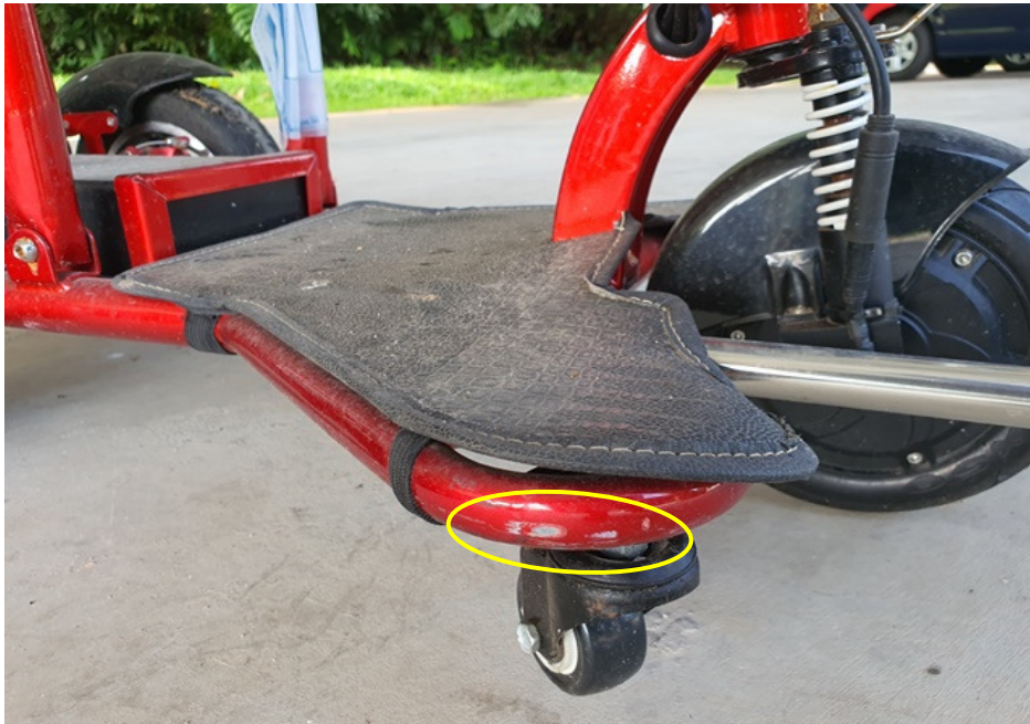
Photo 6 shows a closer view of the right bottom cowling (circled) of the PMA which was observed to be damaged due to the accident.
