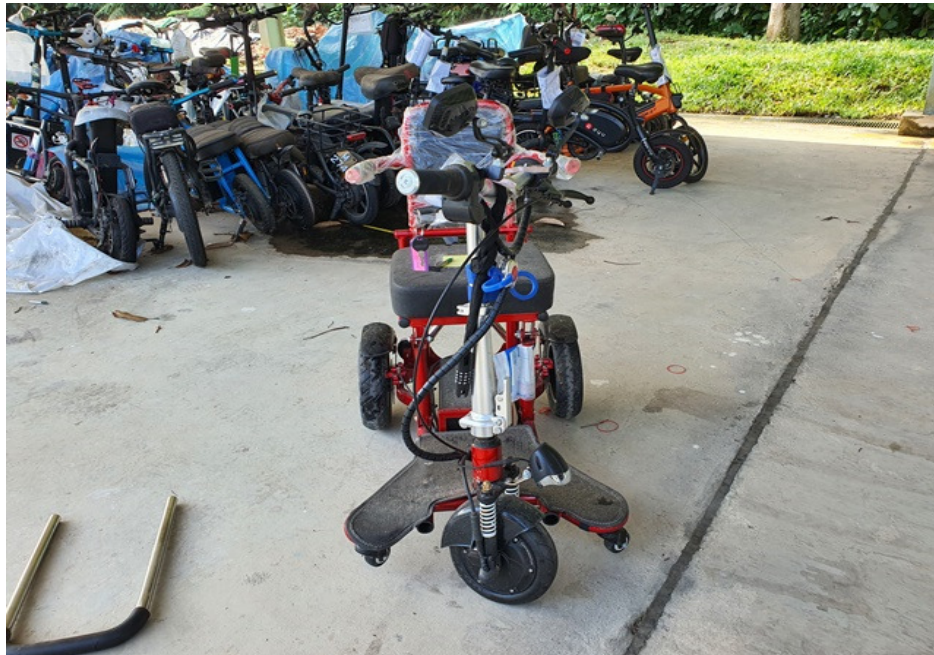
Photo 17 shows the front wheel of the PMA turned towards its full left. Turning the PMA's steering handlebar towards the left did not produce any abnormal free play and/or resistance. This would indicate that the steering system of the PMA was in serviceable condition at the time of our inspection.
