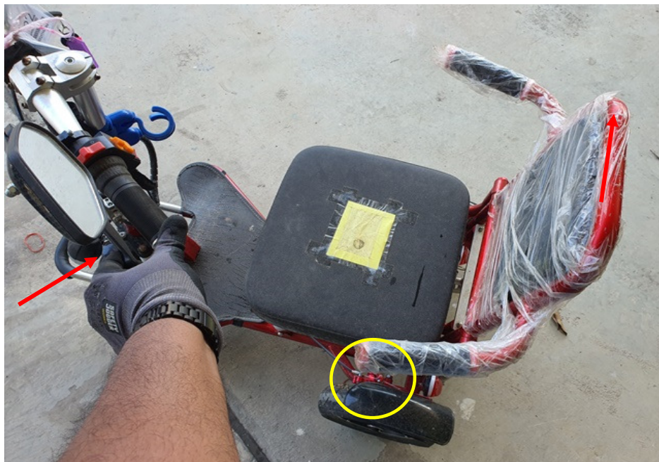
Photo 22 shows a static brake test conducted on the PAB's left rear brake. There was some resistance felt upon pressing the left hand brake lever (arrowed). It also shows that the rear left brake pads responded to the gripping action (circled) after depressing the left hand brake lever.
