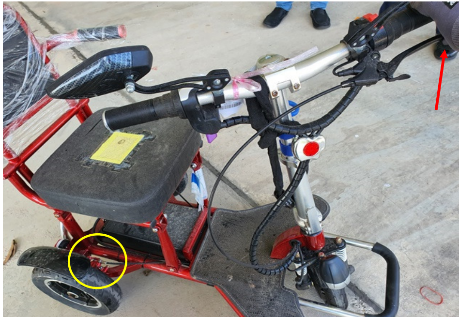
Photo 19 shows a static brake test conducted on the PAB's rear right brake. There was some resistance felt upon pressing the left hand brake lever (arrowed). It also shows that the rear brake pads responded to the gripping action (circled) after depressing the left hand brake lever.
