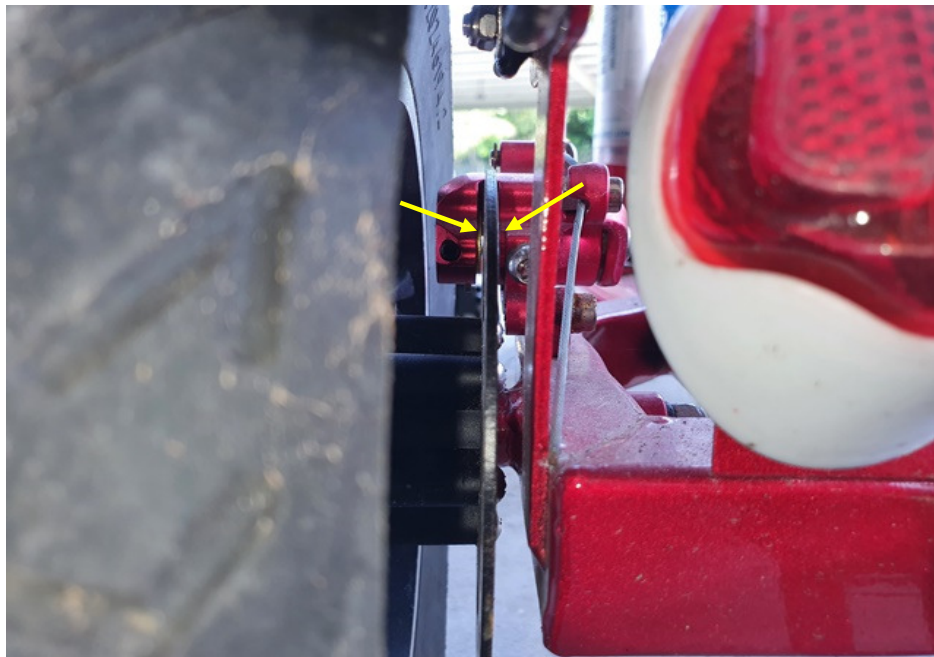
Photo 23 shows a close up view of the left rear brake pads responding to the gripping action. The left rear brake pads pressed against the left rear brake disc (arrowed) upon depressing the left hand brake lever. This had appeared to indicate that the left rear brake of the PMA was in serviceable condition.
