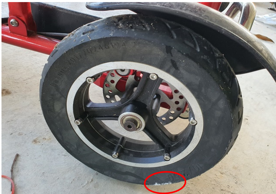
Photo 11 shows the left rear wheel rim and tyre of the PMA at the time of our inspection. Marks of grazing nature were observed on the left sidewall of the left rear tyre of the PMA (circled).
