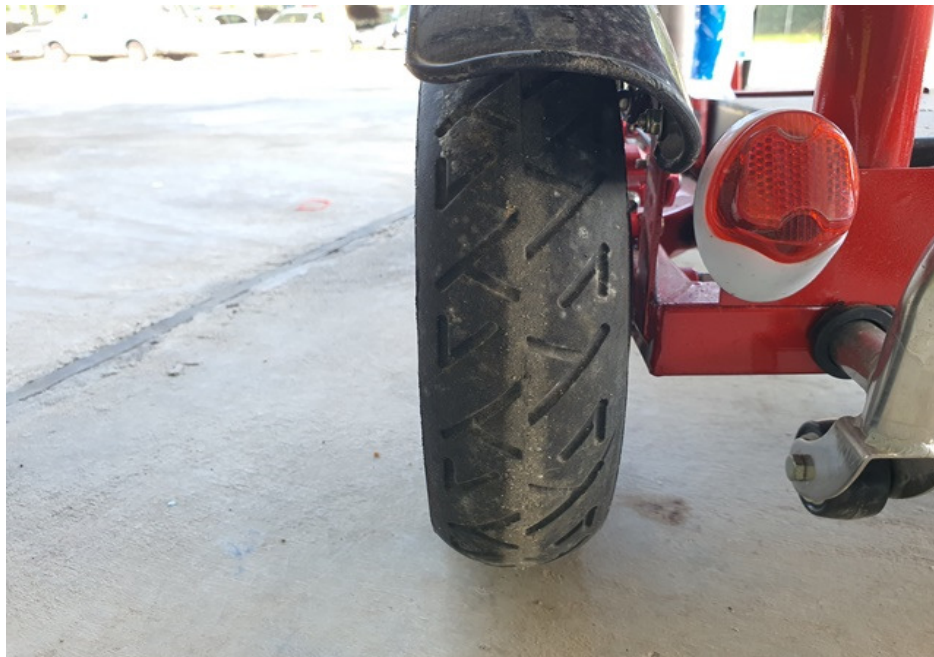
Photo 10 shows the condition of the PMA's left rear tyre. The left rear tyre was observed to have remaining tread depth of approximately 2mm. The left rear tyre was also observed to be sufficiently inflated for vehicular operation. However we found the left sidewall of the left rear tyre to be grazed.
