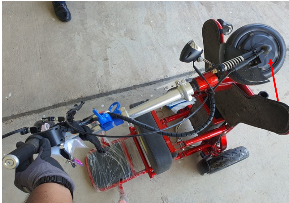
Photo 13 shows the general view of the brushless motor of the PMA which was observed to be in operational condition (arrowed).
