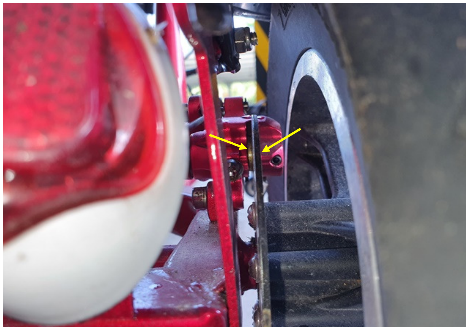
Photo 20 shows a close up view of the right rear brake pads responding to the gripping action. The rear right brake pads pressed against the right rear brake disc (arrowed) upon depressing the left hand brake lever. This had appeared to indicate that the right rear brake of the PMA was in serviceable condition.
