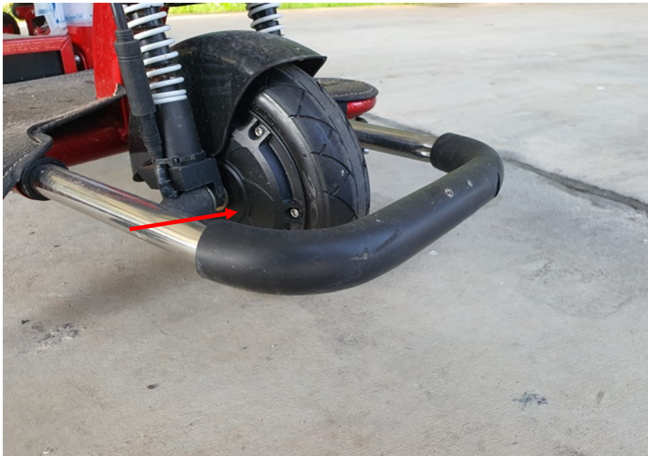
Photo 12 shows the general view of the brushless motor (arrowed) of the PMA which was observed to be intact with no misalignment.
