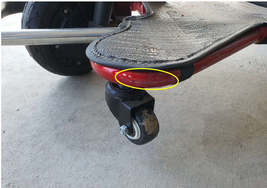
Photo 5 shows a closer view of the left bottom cowl (circled) of the PMA which was observed to be damaged due to the accident.
