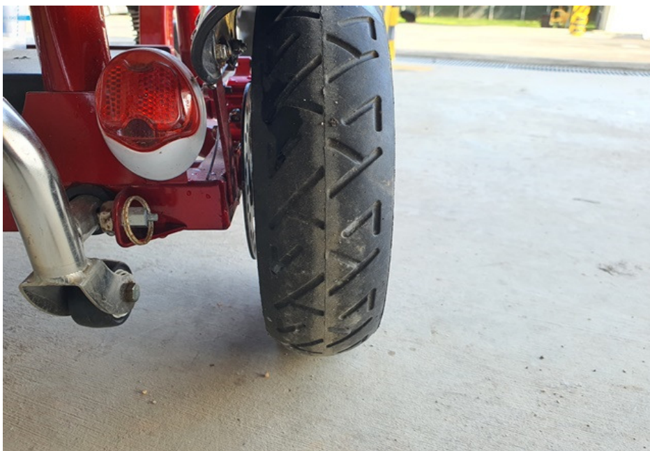
Photo 9 shows the condition of the PMA's right rear tyre. The right rear tyre was observed to be in serviceable condition with remaining tread depth of approximately 2mm. The right rear tyre was also observed to be sufficiently inflated for vehicular operation. There was no tear, burst mark(s) and/or punctured hole(s) on the sidewalls as well as across the tread of the right rear tyre.
