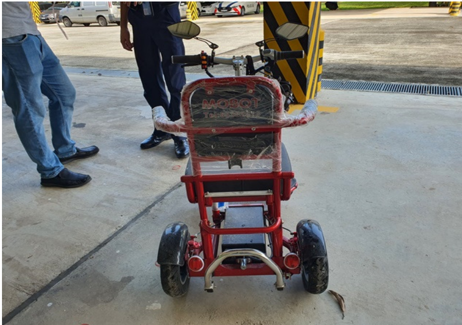
Photo 4 shows a general view of the rear portion of the PMA at the time of our inspection. The PMA was observed to have sustained damages all around. The body parts that were found to have been damaged include its right handlebar end, right side mirror and bottom cowlings, amongst others as a result of the accident.
