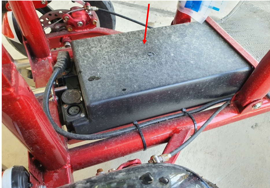
Photo 14 shows the wireless battery pack of the PMA (arrowed) which was found to be intact without any misalignment.
