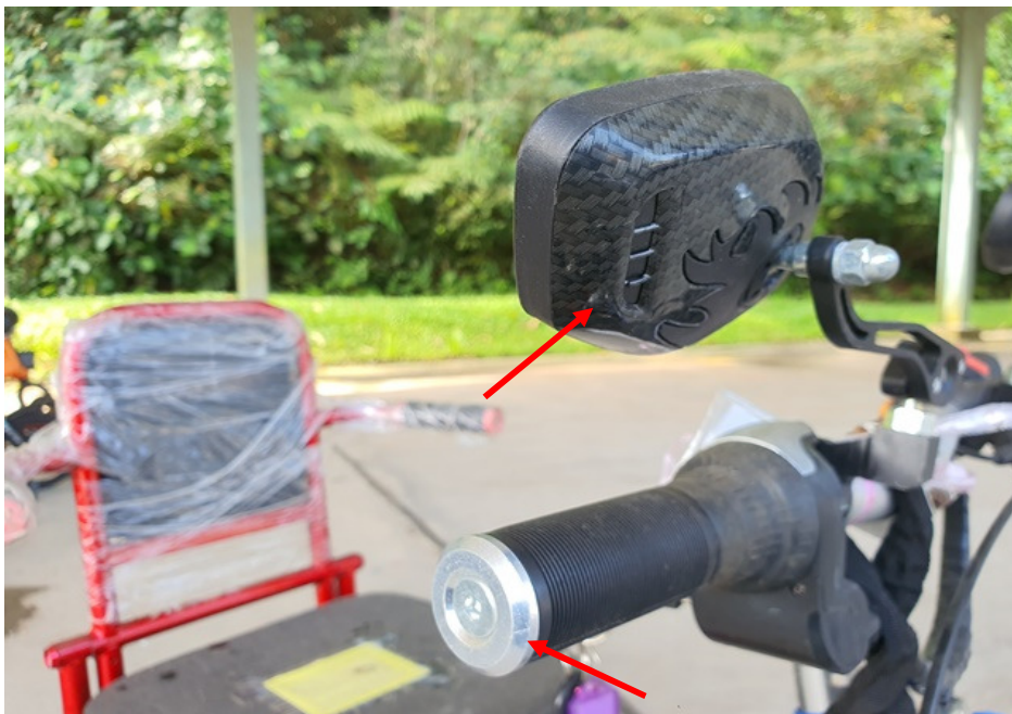
Photo 7 shows a closer view of the right handlebar end and right side mirror (arrowed) of the PMA which were observed to be damaged due to the accident
