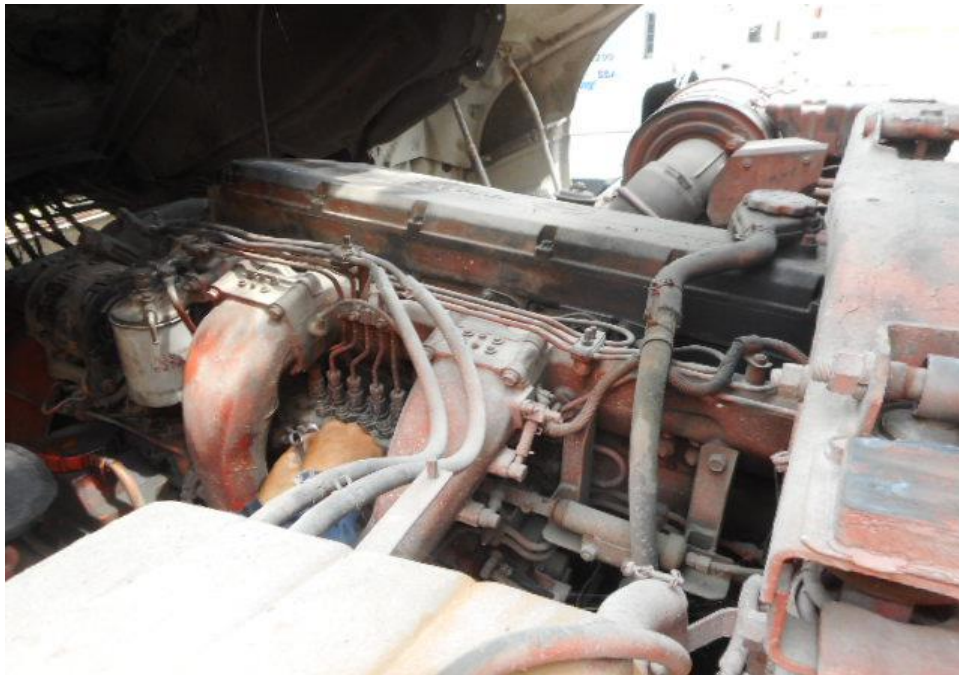
Photo 11 shows a general view of the Malaysian Tipper's engine compartment, which was accessed by lifting the front cabin of the Malaysian Tipper. The various parts and components inside the engine compartment were unaffected by the accident. There was also no sign(s) or indication(s) of fresh fluid leakage and/or fluid stain within the engine compartment
