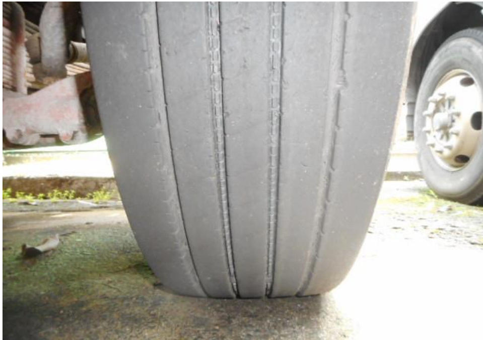
Photo 7 shows the condition of the front right tyre of the Malaysian Tipper, which was observed to be in serviceable condition with remaining tread depth of approximately 7.2mm. The tyre, which was wrapped around standard steel wheel rim, was also observed to be sufficiently inflated for vehicular operation. There was no tear, cut or burst mark(s) on the outer and the inner sidewalls as well as across the tread of the 12 tyres that were fitted on the Malaysian Tipper.
