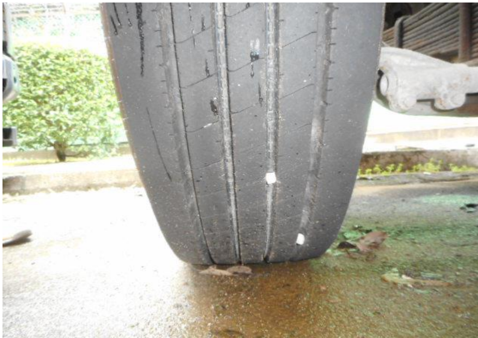
Photo 10 shows the condition of the front left tyres of the Malaysian Tipper, which were observed to be in serviceable condition with remaining tread depth of approximately 11.6mm. There was also no tear, cut or burst mark(s) on the outer and the inner sidewalls as well as across the tread of the 12 tyres that were fitted on the Malaysian Tipper.
