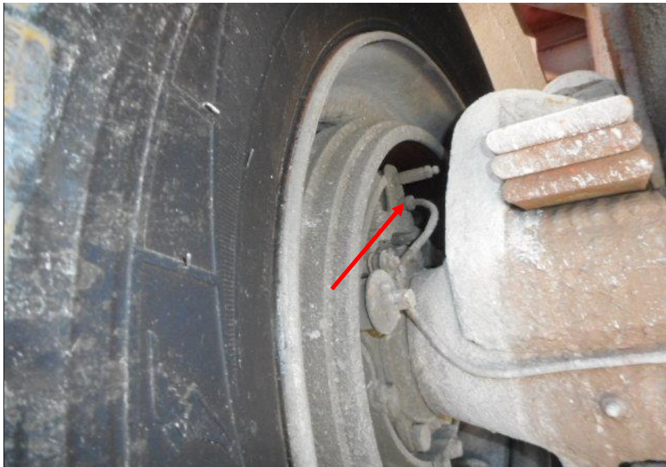
Photo 18 shows the brake pipe (arrowed) at the rear left wheel of the Malaysian Tipper. I did not observe any leakage of brake fluid at the time of my inspection of the Malaysian Tipper. My static tests of the Malaysian Tipper's braking system, along with my visual examination of the various mechanical components in the braking system, had indicated that there was no internal leakage of pressure/vacuum. Hence the braking system of the Malaysian Tipper was likely to be in serviceable condition at the material time of accident.
