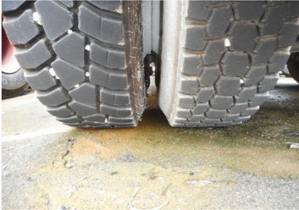
Photo 9 shows the condition of the rear left tyres of the Malaysian Tipper, which was observed to be in serviceable condition with remaining tread depth of approximately 12.7mm. The tyres, which were wrapped around standard steel wheel rim, were also observed to be sufficiently inflated for vehicular operation. There was also no damage found on all 12 steel wheel rims of the Malaysian Tipper.
