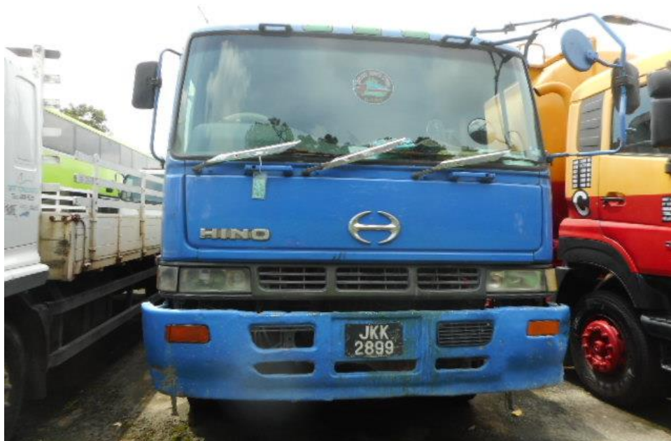
Photo 2 shows a general view of the front body of the Malaysian Tipper at the time of my inspection. The Malaysian Tipper was observed to sustain damaged at its front portion. Its front bumper left portion was damaged at the time of my inspection.
