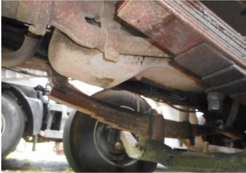
Photo 16 shows the undercarriage of the Malaysian Tipper, at the area where the engine housing located. I did not find any sign(s) or indication(s) of fluid leak on the underside of the Malaysian Tipper.
