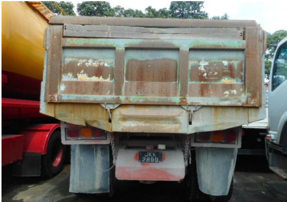
Photo 6 shows a general view of the Malaysian Tipper's rear body at the time of my inspection. The Malaysian Tipper was observed to be intact and unaffected by the accident.
