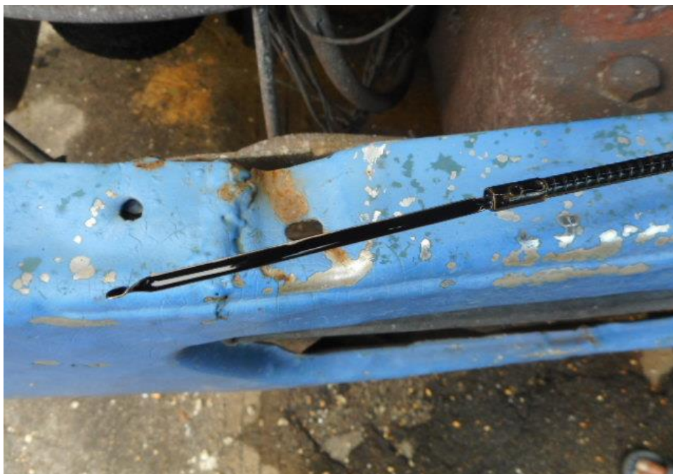
Photo 15 shows the engine oil dip stick of the Malaysian Tipper at the time of my inspection. The engine oil was observed to be of insufficient level at the time of our inspection.
