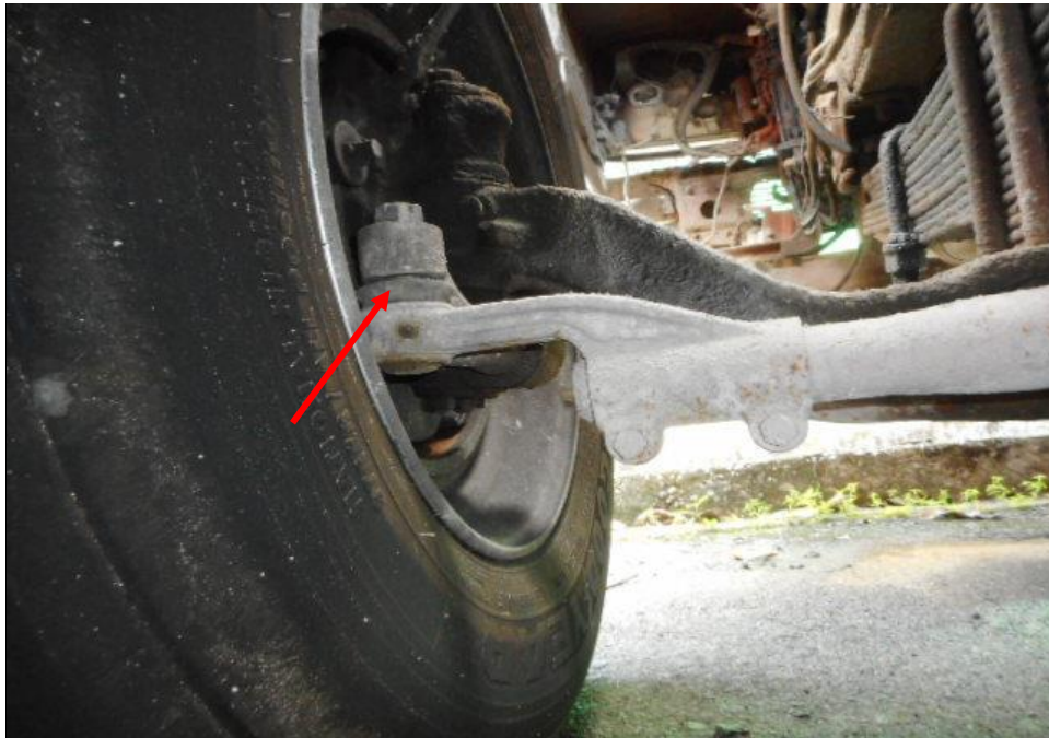
Photo 23 shows the various undercarriage components at the front left wheel of the Malaysian Tipper, in particular the steering tie rod end (arrowed). The various undercarriage components of the Malaysian Tipper were all found to be intact without any visible damage. There was also no sign of fluid stain(s) observed on the various undercarriage components.
