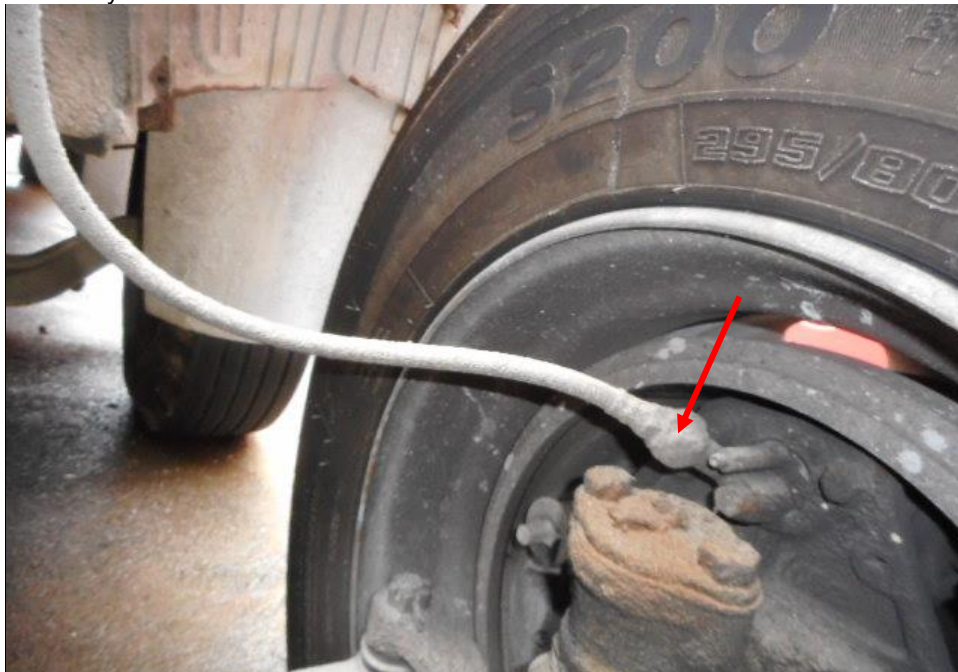
Photo 20 shows the brake pipe (arrowed) at the front left wheel of the Malaysian Tipper. I did not observe any leakage of brake fluid at the time of my inspection of the Malaysian Tipper. My static tests of the Malaysian Tipper's braking system, along with my visual examination of the various mechanical components in the braking system had indicated that there was no internal leakage of pressure/vacuum. Hence the braking system of the Malaysian Tipper was likely to be in serviceable condition at the material time of accident.
