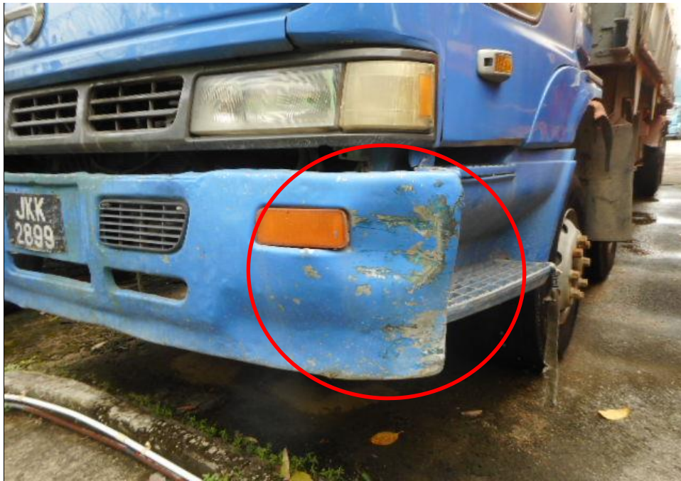
Photo 3 shows a general view of the front body of the Malaysian Tipper at the time of my inspection. The Malaysian Tipper was observed to sustain damaged on its front portion. Its front bumper left portion (circled) was damaged at the time of my inspection.
