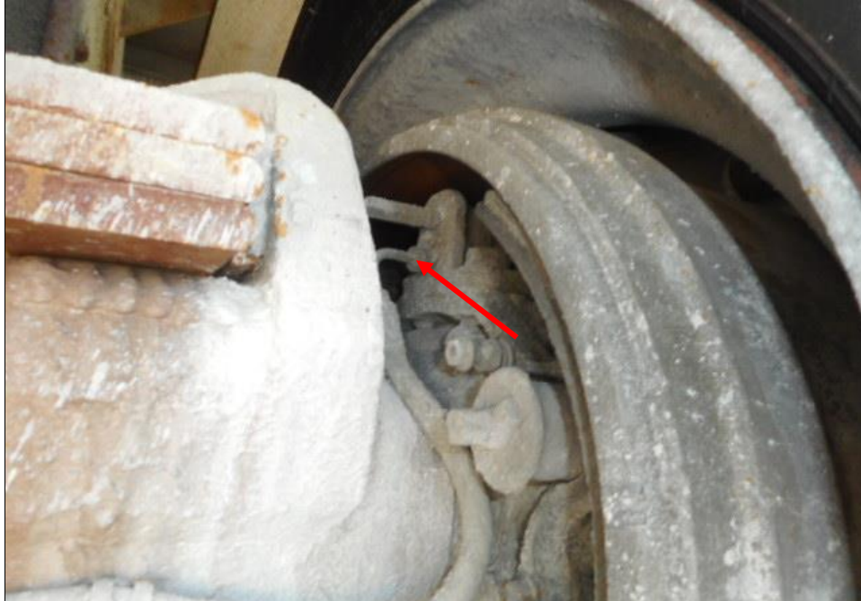
Photo 17 shows the brake pipe (arrowed) at the rear right wheel of the Malaysian Tipper. I did not observe any leakage of brake fluid at the time of my inspection of the Malaysian Tipper. My static tests of the Malaysian Tipper's braking system, along with my visual examination of the various mechanical components in the braking system, had indicated that there was no internal leakage of pressure/vacuum. Hence the braking system of the Malaysian Tipper was likely to be in serviceable condition at the material time of accident.
