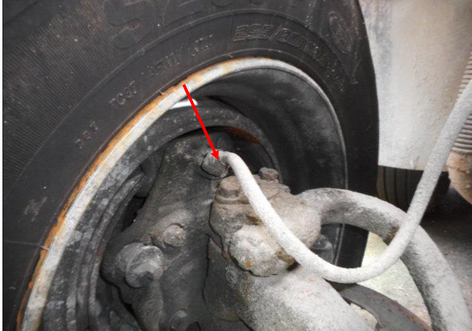
Photo 19 shows the brake pipe (arrowed) at the front right wheel of the Malaysian Tipper. I did not observe any leakage of brake fluid at the time of my inspection of the Malaysian Tipper. My static tests of the Malaysian Tipper's braking system, along with my visual examination of the various mechanical components in the braking system, had indicated that there was no internal leakage of pressure/vacuum. Hence the braking system of the Malaysian Tipper was likely to be in serviceable condition at the material time of accident.
