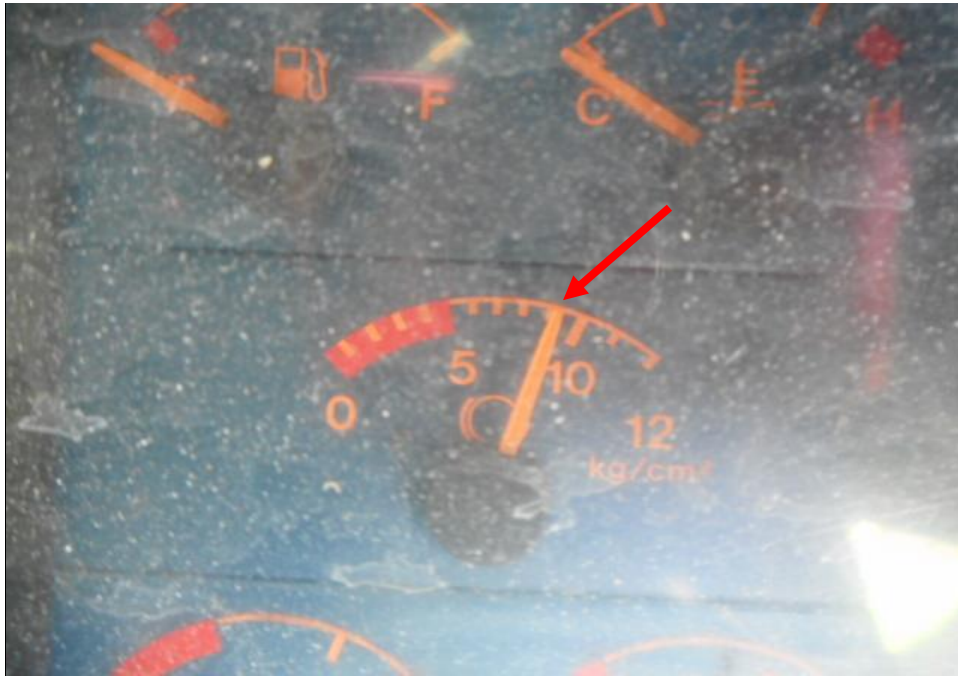
Photo 12 shows the air in the air brake cylinders of the Malaysian Tipper at the time of my inspection. The air in the cylinder was observed to be of sufficient level & serviceable at the time of the accident.
