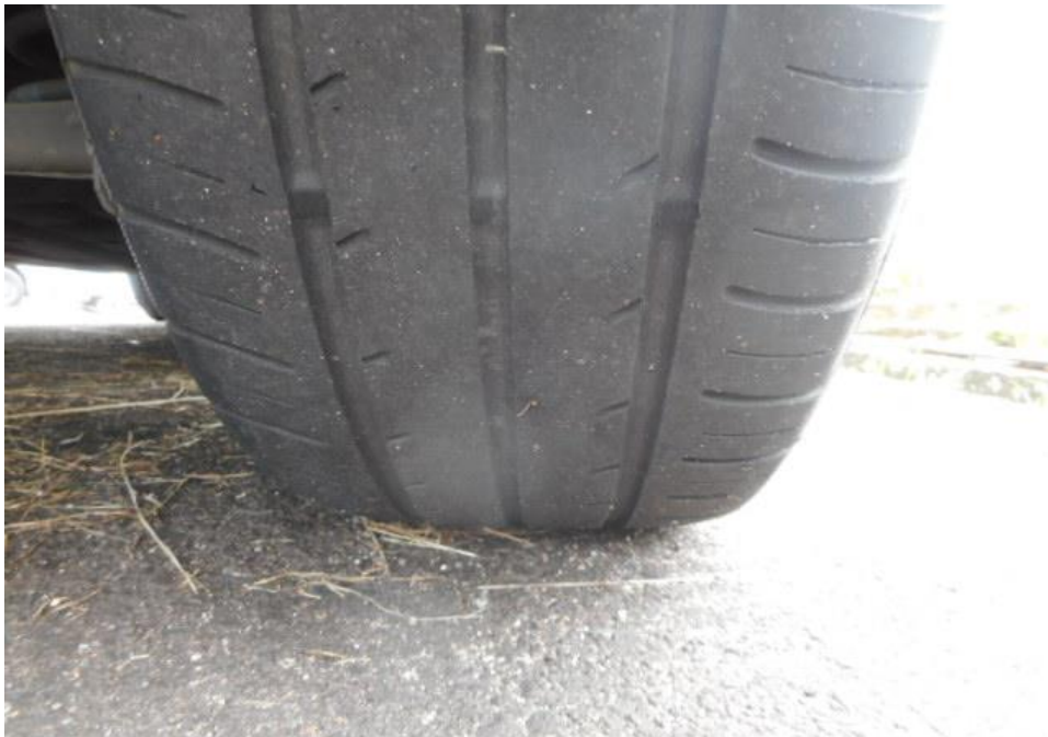
Photo 11 shows the condition of the rear right tyre of the Motor Car, which was observed to be in serviceable condition with remaining tread depth of approximately 2.6mm. The tyre was also observed to be sufficiently inflated for vehicular operation with no tear, cut or burst mark(s).
