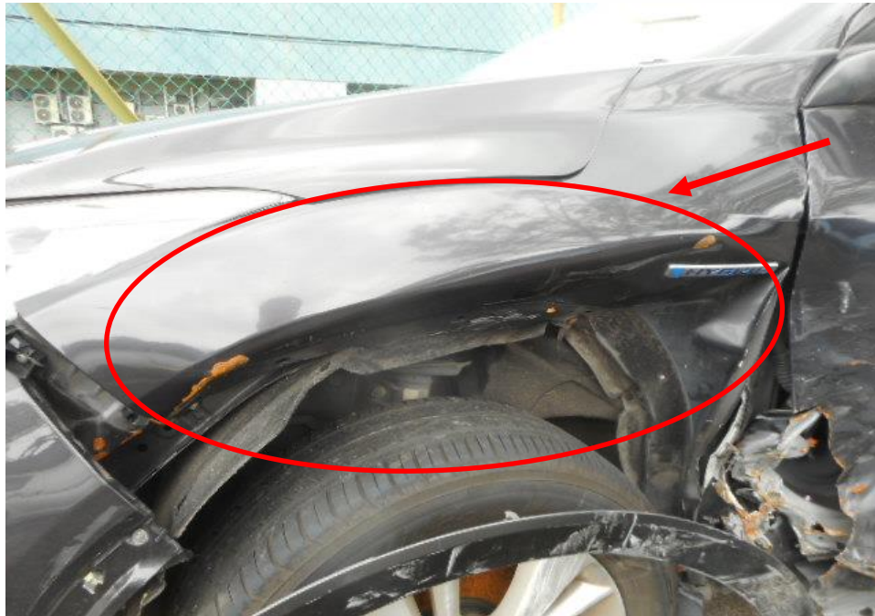
Photo 4 shows a close up view of the Motor Car's left body at the time of my inspection. The left portion of the Motor Car was observed to have sustained damage. Its left front fender (circled) was the body parts that were damaged as a result of the accident.
