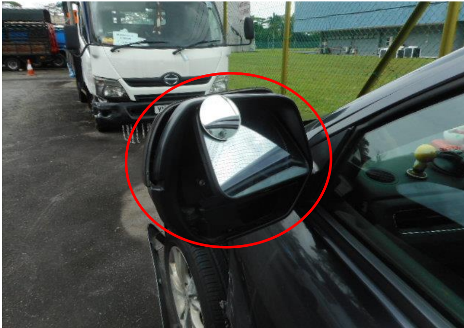
Photo 6 shows a close up view of the Motor Car's left body at the time of my inspection. The left portion of the Motor Car was observed to have sustained damage. Its left rear view mirror (circled) was the body parts that were damaged as a result of the accident.
