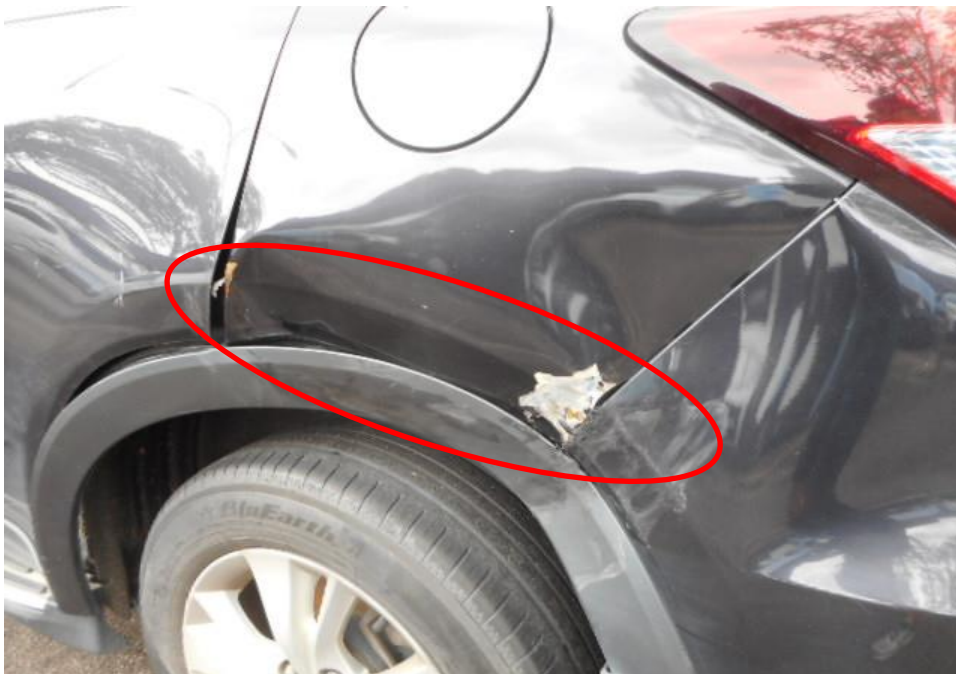
Photo 7 shows a close up view of the Motor Car's left body at the time of my inspection. The left portion of the Motor Car was observed to have sustained damage. Its left rear fender (circled) was the body parts that were damaged as a result of the accident.
