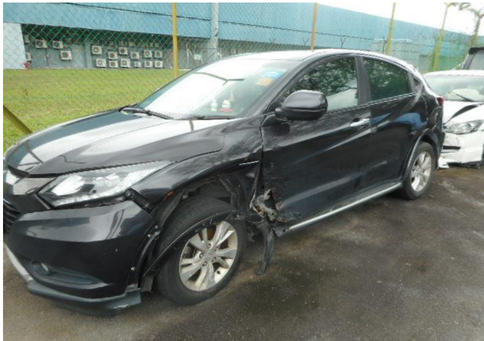
Photo 3 shows a general view of the Motor Car's left body at the time of my inspection. The Motor Car was observed to have sustained damage at its left portion. Its front and rear left fender, left front door, left rear view mirror was the body parts that were damaged as a result of the accident.
