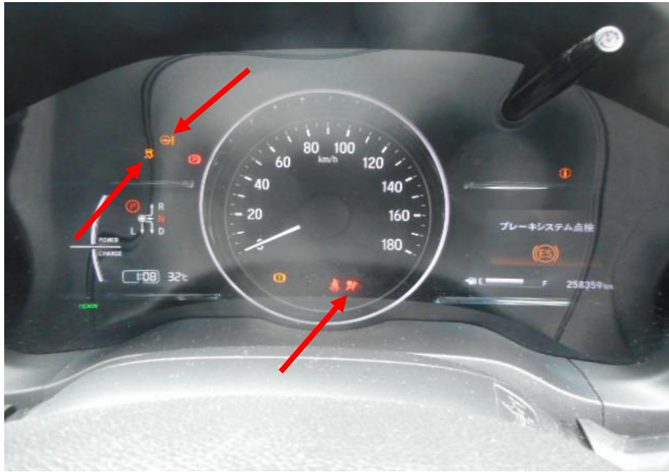
Photo 26 shows the Electronic Power Steering System (EPS), Traction Control System (TCS), and Supplemental Restraint System (SRS) (arrowed) warning lights remained illuminated on the instrument panel of the Motor Car after the engine was cranked. This was due to the damages sustained to the steering rack and pinion, steering column where these components are located inside.
