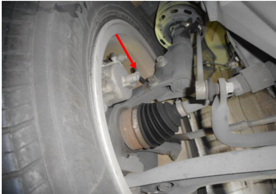
Photo 21 shows the brake hose/pipe (arrowed) at the front right wheel of the Motor Car. I did not observe any leakage of brake fluid at the time of my inspection of the Motor Car. Static tests of the Motor Car's braking system had indicated that there was no internal leakage of pressure/vacuum.
