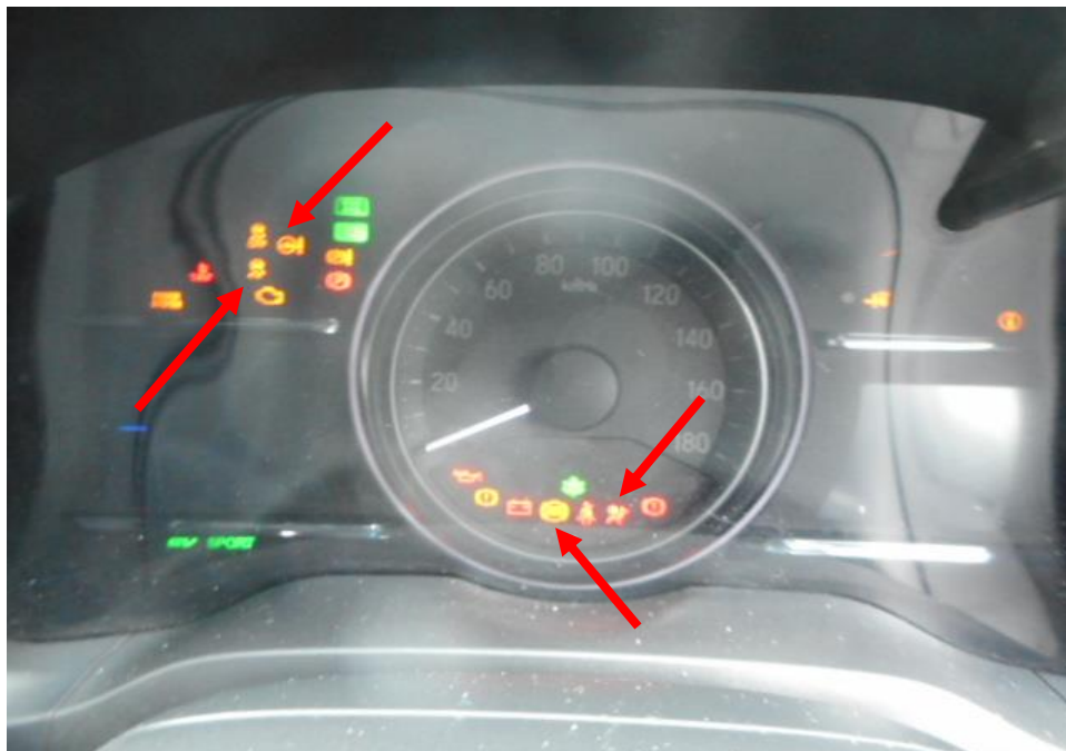
Photo 25 shows the warning light for Anti-Lock Brake System (ABS), Electronic Power Steering System (EPS), Traction Control System (TCS), and Supplemental Restraint System (SRS) (arrowed) appearing on the instrument panel of the Motor Car during the self-test of its various electronic operating systems when its engine was cranked.
