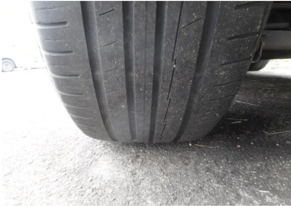
Photo 12 shows the condition of the rear left tyre of the Motor Car, which was observed to be in serviceable condition with remaining tread depth of approximately 3.7mm. The tyre, which was wrapped around alloy wheel rim, was also observed to be sufficiently inflated for vehicular operation. The 4 tyres of the Motor Car were wrapped around standard alloy wheel rims.
