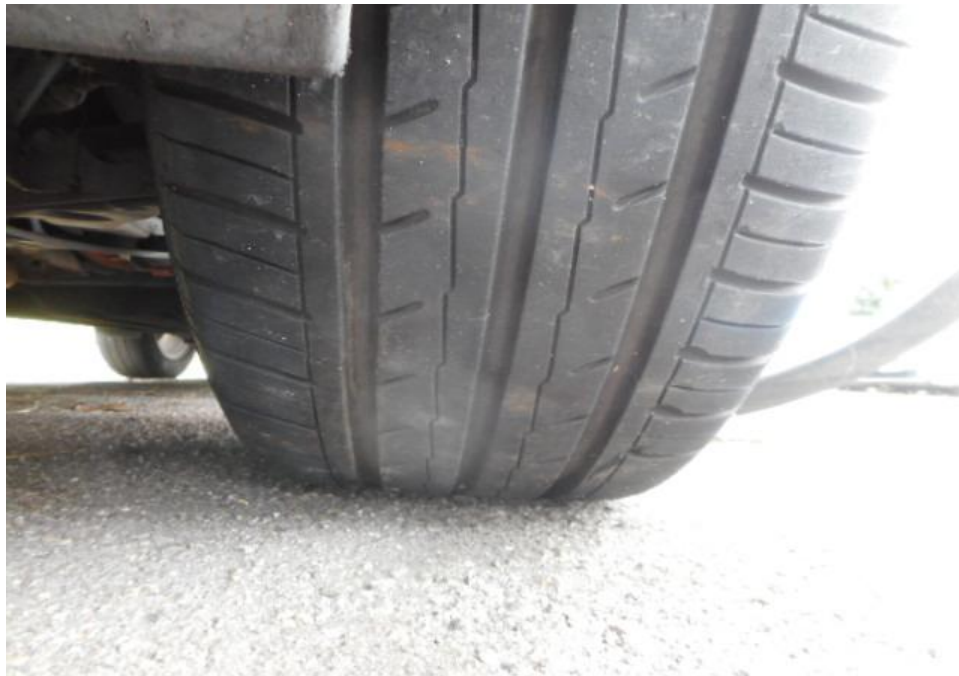
Photo 13 shows the condition of the front left tyre of the Motor Car, which was observed to be in serviceable condition with remaining tread depth of approximately 4.1mm. There was also no tear, cut or burst mark(s) on the outer and the inner sidewalls as well as across the tread of the Motor Car's 4 tyres.
