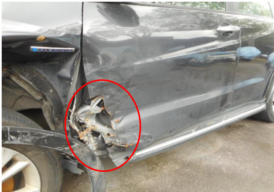
Photo 5 shows a close up view of the Motor Car's left body at the time of my inspection. The left portion of the Motor Car was observed to have sustained damage. Its front left door (circled) was the body parts that were damaged as a result of the accident.
