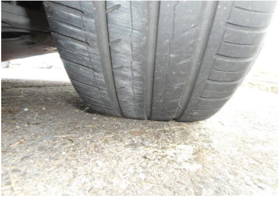
Photo 10 shows the condition of the front right tyre of the Motor Car, which was observed to be in serviceable condition with remaining tread depth of approximately 3.4mm. The tyre was also observed to be sufficiently inflated for vehicular operation with no tear, cut or burst mark(s).
