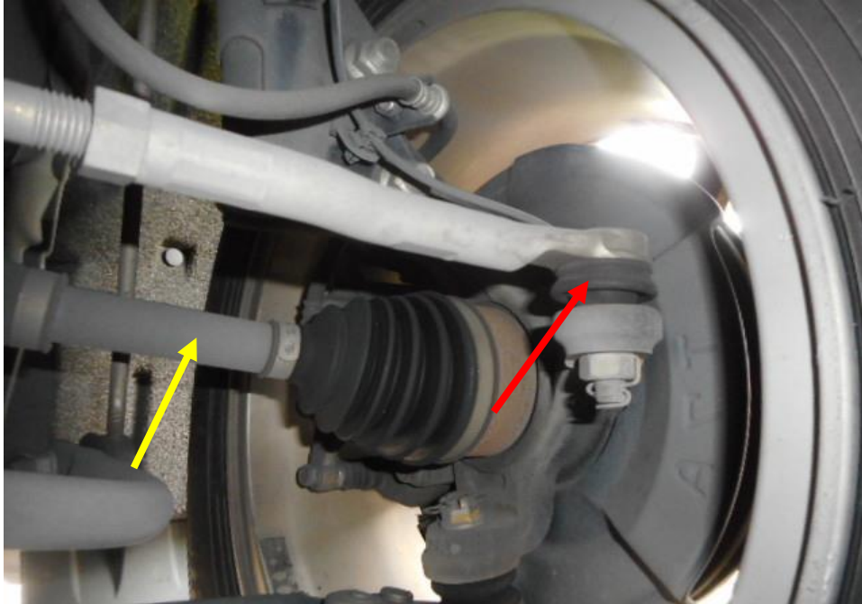
Photo 23 shows the various undercarriage components at the front right wheel of the Motor Car, in particular the steering tie rod (red arrow) and in particular the drive shaft (yellow arrow). The various steering components were all found to be intact, suggesting that the steering system of the Motor Car was likely to be in serviceable condition at the material time of accident. There was also no sign of fluid stain observed on the various undercarriage components at the front right wheel of the Motor Car.
