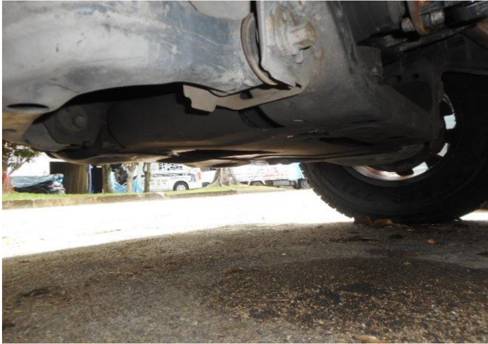
Photo 15 shows the undercarriage of the Pick-up truck, at the area where the engine housing and transmission housing are located. . I did not find any sign(s) or indication(s) of fluid leak and/or fluid stain(s) on the underside of the Pick-up truck.
