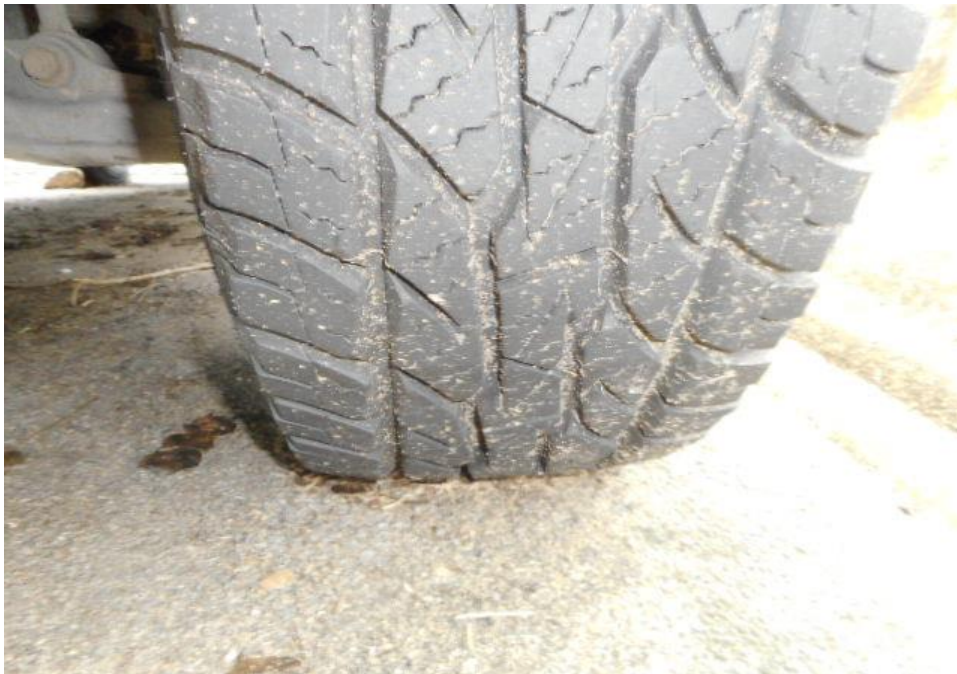
Photo 9 shows the condition of the rear right tyres of the Pick-up truck, which were observed to be in serviceable condition with remaining, tread depth of approximately 9.4mm. There was also no tear, cut or burst mark(s) on the outer and the inner sidewalls as well as across the tread of the 4 tyres that were fitted on the Pick-up truck.
