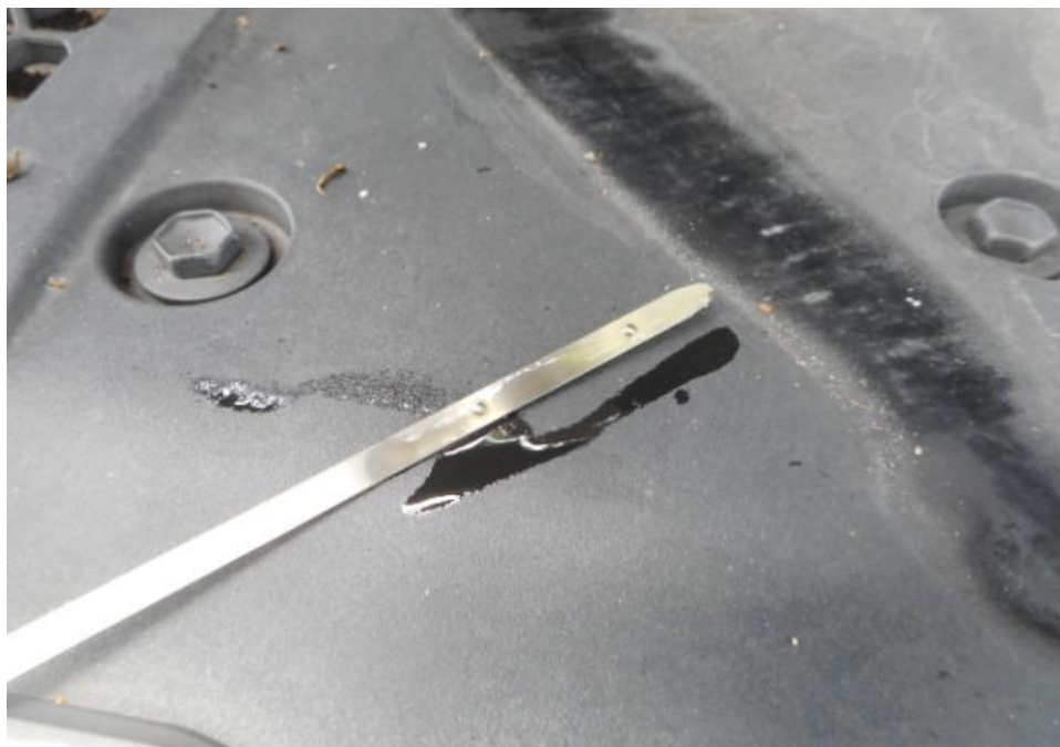
Photo 14 shows the engine oil dip stick of the Pick-up truck at the time of my inspection. The engine oil was observed to be of sufficient level and without any visible contamination.
