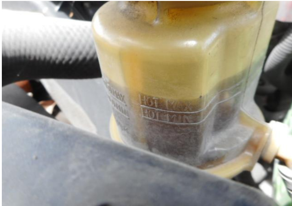
Photo 13 shows the power steering fluid of the Pick-up truck at the time of my inspection. The power steering fluid was observed to be of sufficient level and without any visible contamination.
