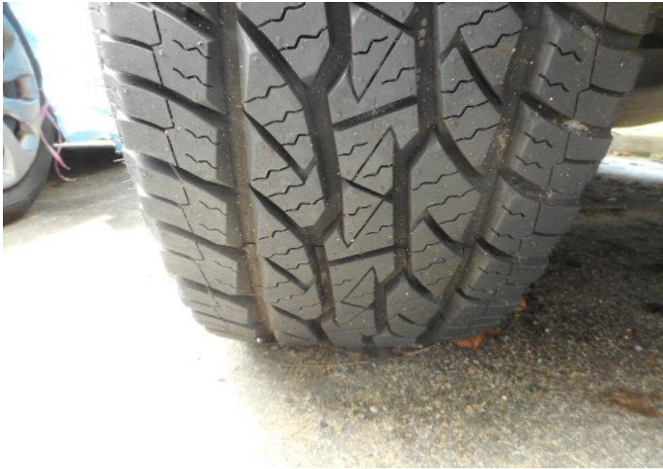
Photo 6 shows the condition of the front right tyre of the Pick-up truck, which was observed to be in serviceable condition with remaining tread depth of approximately 9.4mm. The tyre, which was wrapped around standard alloy wheel rim, was also observed to be sufficiently inflated for vehicular operation. There was no tear, cut or burst mark(s) on the outer and the inner sidewalls as well as across the tread of the 4 tyres that were fitted on the Pick-up truck.
