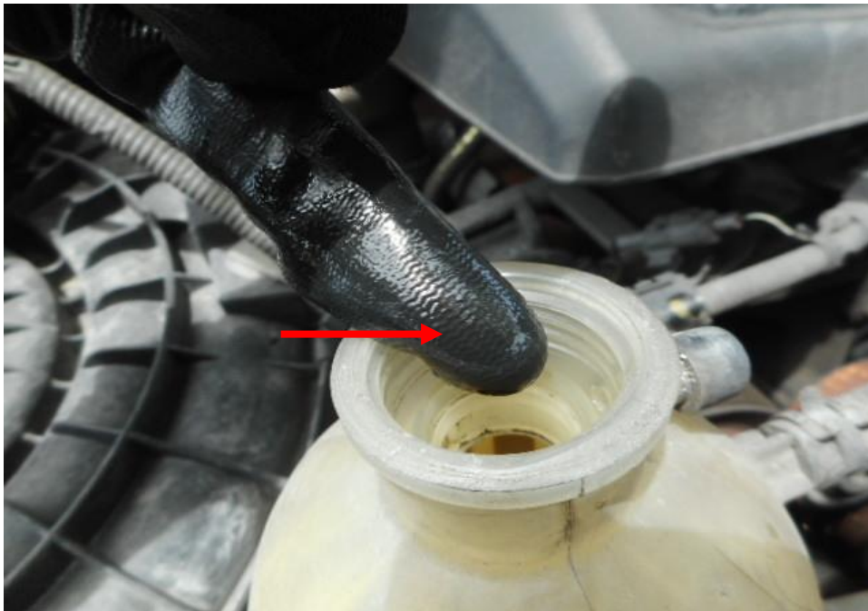
Photo 12 shows the engine coolant reservoir of the Pick-up truck at the time of my inspection. The engine coolant was observed to be of sufficient level (arrowed) and without any visible contamination.
