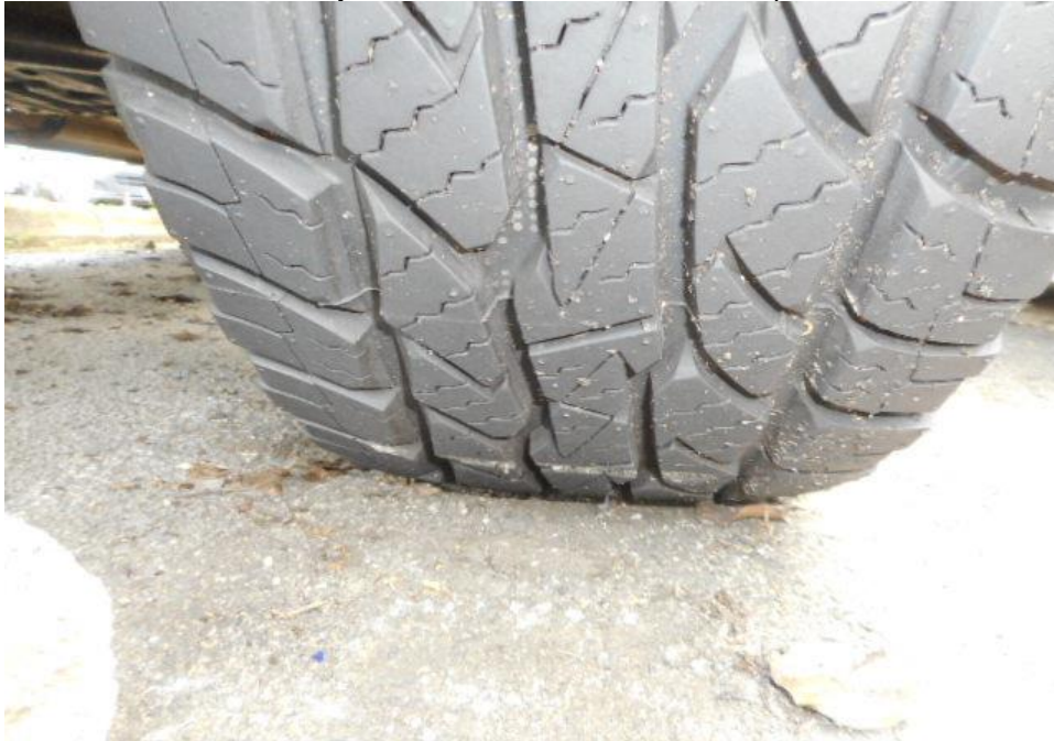
Photo 7 shows the condition of the rear right tyre of the Pick-up truck, which was observed to be in serviceable condition with remaining tread depth of approximately 9.6mm. The tyre, which was wrapped around standard alloy wheel rim, was also observed to be sufficiently inflated for vehicular operation.
