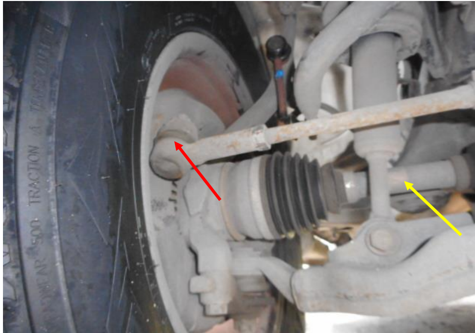
Photo 16 shows the various undercarriage components at the front right wheel of the Pick-up truck, in particular the steering tie rod end (red arrowed) and drive shaft (yellow arrow). The various steering components were all found to be intact, suggesting that the steering system of the Pick-up truck was likely to be in serviceable condition at the material time of accident. There was also no sign of fluid stain(s) observed on the various undercarriage components.
