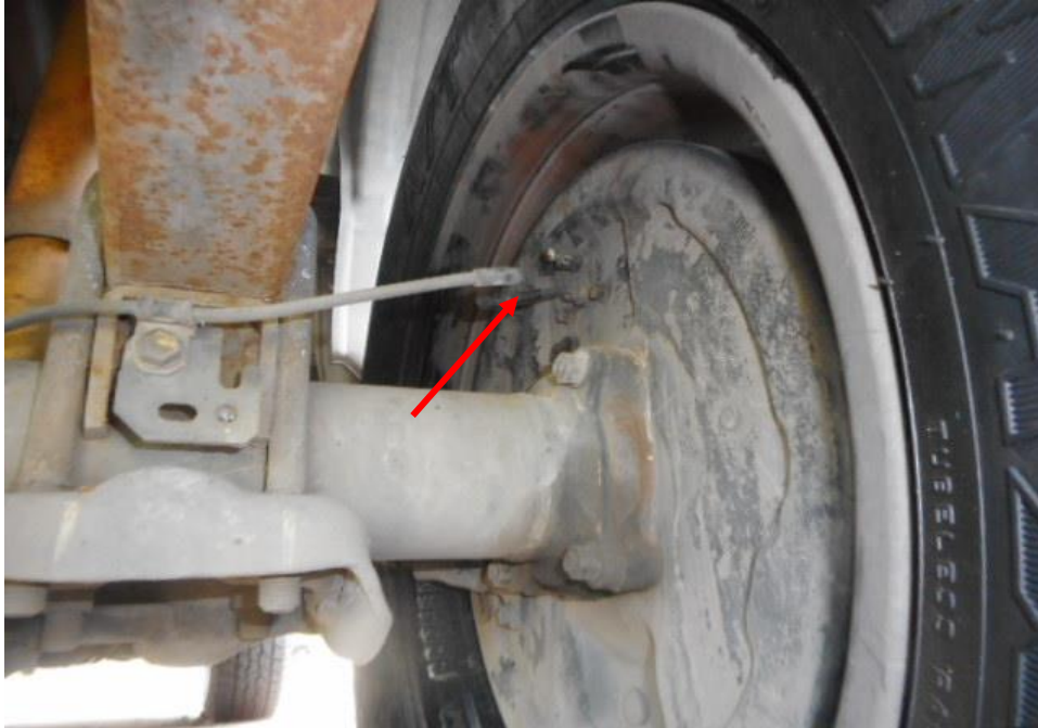
Photo 18 shows the brake pipe (arrowed) at the rear right wheel of the Pick-up truck. I did not observe any leakage of brake fluid at the time of my inspection of the Pick-up truck. My static tests of the Pick-up truck's braking system, along with my visual examination of the various mechanical components in the braking system, had indicated that there was no internal leakage of pressure/vacuum. Hence the braking system of the Pick-up truck was likely to be in serviceable condition at the material time of accident.
