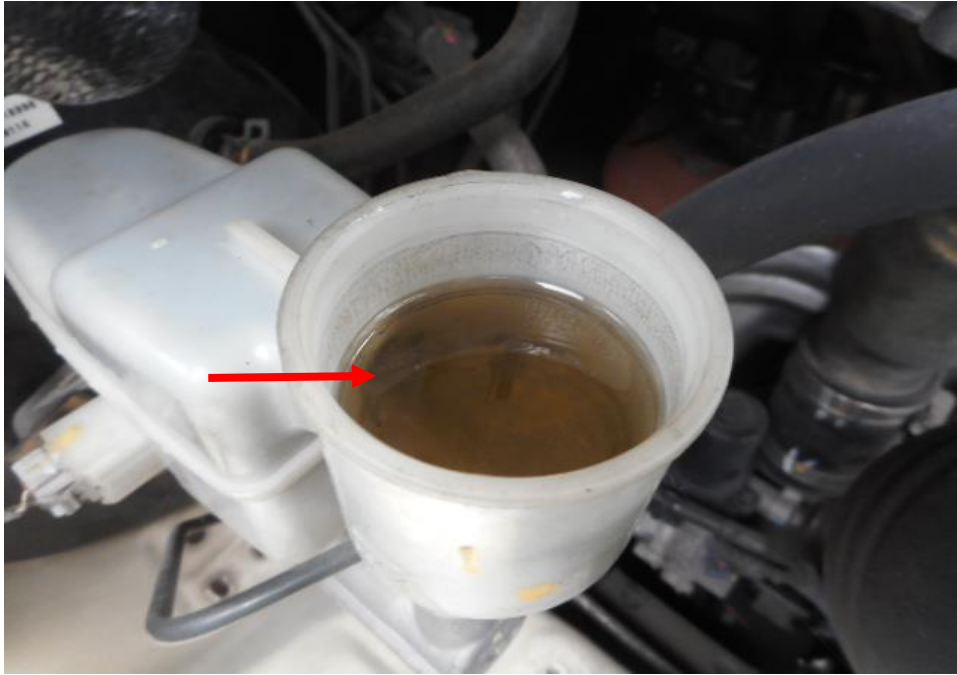
Photo 11 shows the brake fluid reservoir of the Pick-up truck at the time of my inspection. The brake fluid was observed to be of sufficient level (arrowed) and without any visible contamination.
