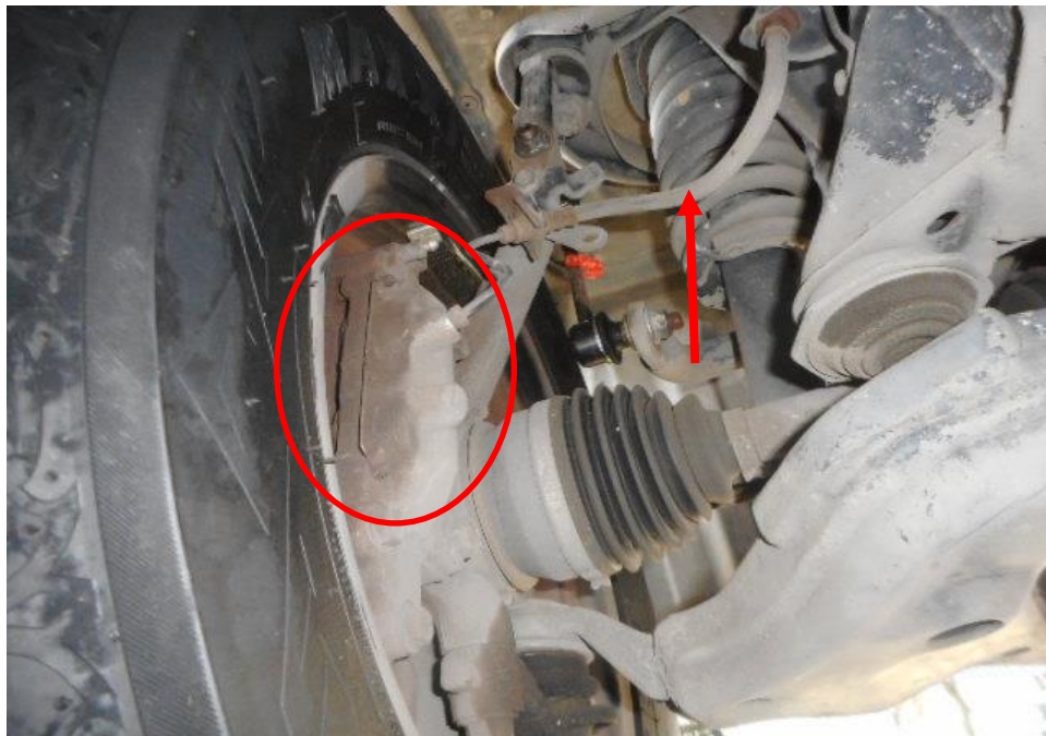
Photo 21 shows the brake hose/pipe (arrowed) at the front left wheel of the Pick-up truck. No leakage of brake fluid was observed. Visual examination of the various components of the braking system like the brake caliper (circled), brake booster, brake pedal etc had revealed all to be intact and without visible damage at the time of accident. There was also no sign of fluid stain(s) observed on the various undercarriage components.
