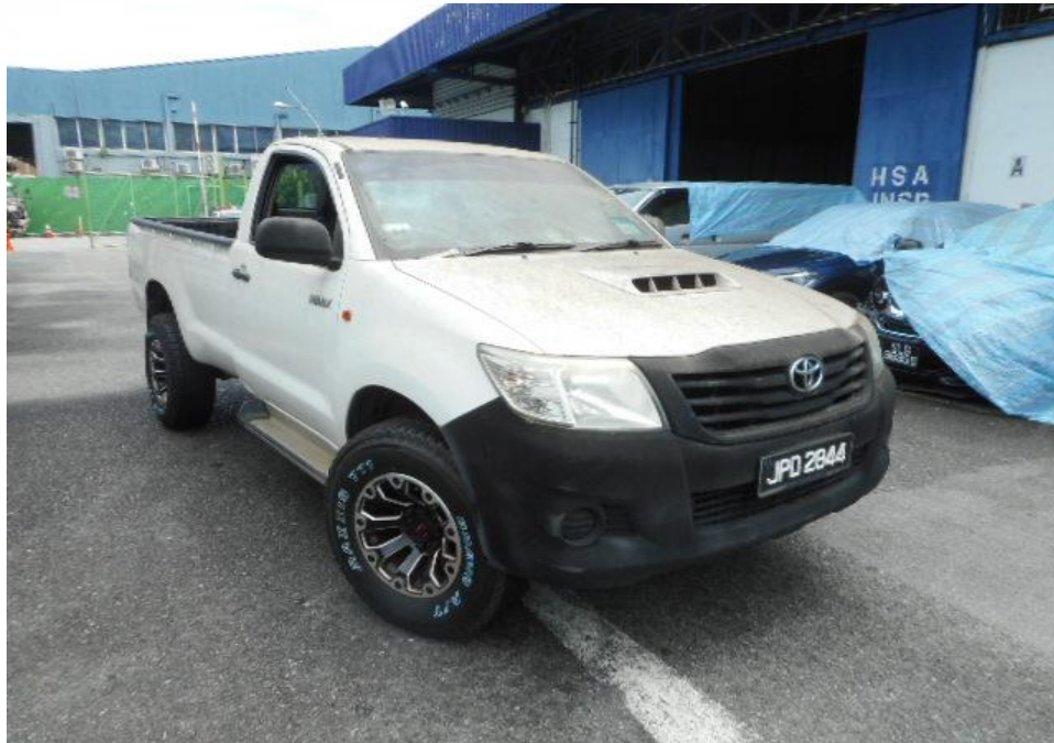
Photo 22 shows the front right wheel of the Pick-up truck turned to its full left. During my steering system test, I did not experience any abnormal free play and/or resistance when I had turned the steering wheel towards full left and full right. This would suggest that the steering system of the Pick-up truck was likely to be in serviceable condition at the material time of accident.
