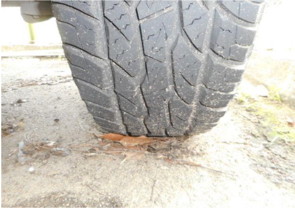
Photo 8 shows the condition of the rear left tyres of the Pick-up truck, which was observed to be in serviceable condition with remaining tread depth of approximately 9.6mm. The tyres, which were wrapped around standard alloy wheel rim, were also observed to be sufficiently inflated for vehicular operation. There was also no damage found on all 4 alloy wheel rims of the Pick-up truck.
