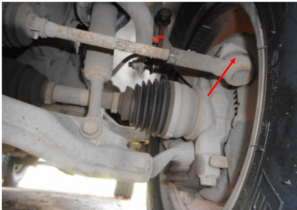
Photo 17 shows the various undercarriage components at the front left wheel of the Pick-up truck, in particular the steering tie rod end (arrowed). The various Undercarriage components of the Pick-up truck were all found to be intact without any visible damage. There was also no sign of fluid stain(s) observed on the various undercarriage components.
