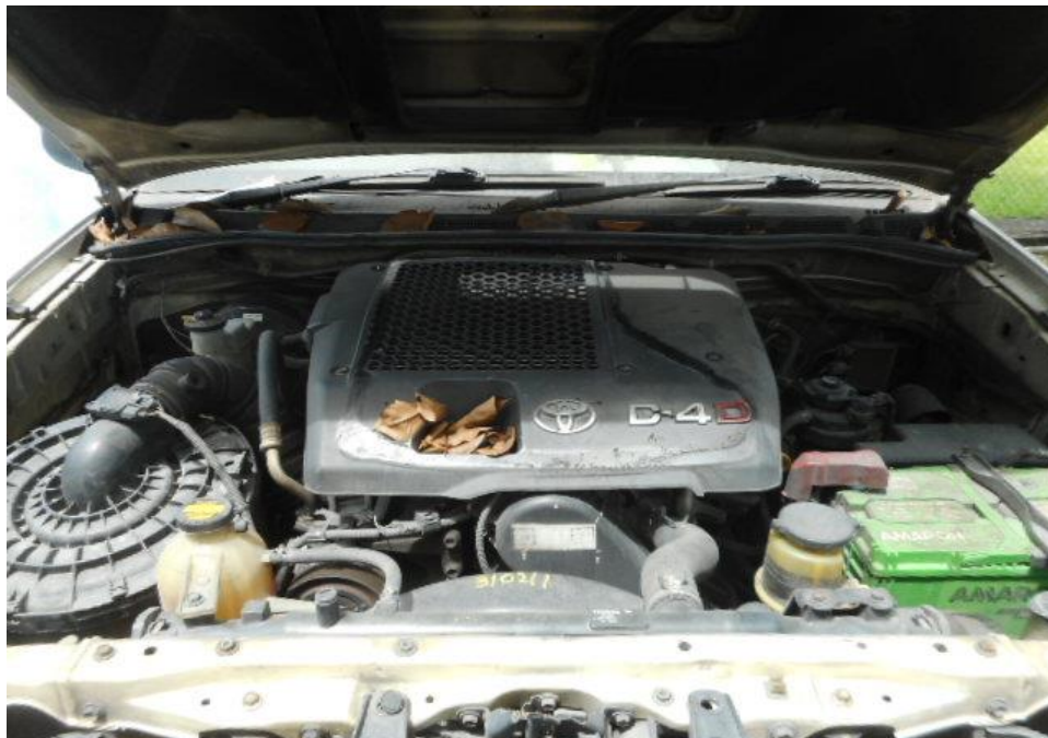
Photo 10 shows a general view of the Pick-up truck's engine compartment, which was accessed by lifting the front cabin of the Pick-up truck. The various parts and components inside the engine compartment were unaffected by the accident. There was also no sign(s) or indication(s) of fresh fluid leakage and/or fluid stain within the engine compartment
