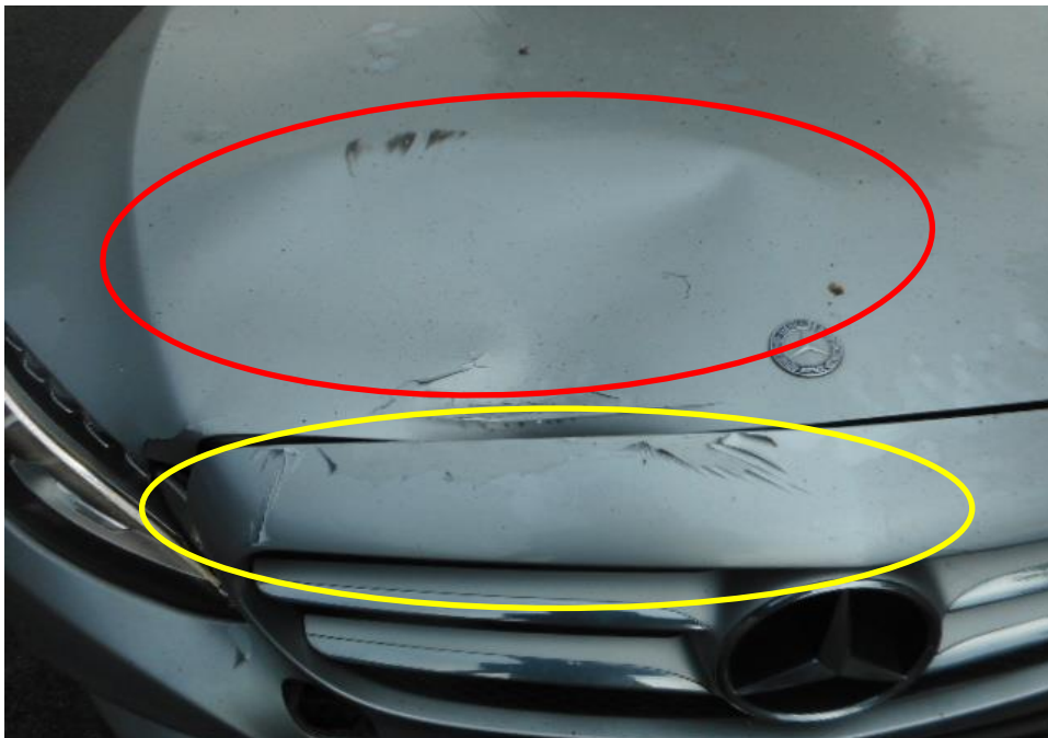
Photo 5 shows a close up view of the Motor Car's front body at the time of my inspection. The front portion of the Motor Car was observed to have sustained damage. Its front bonnet (red circle) and front bumper (yellow circle) was the body parts that were damaged as a result of the accident.
