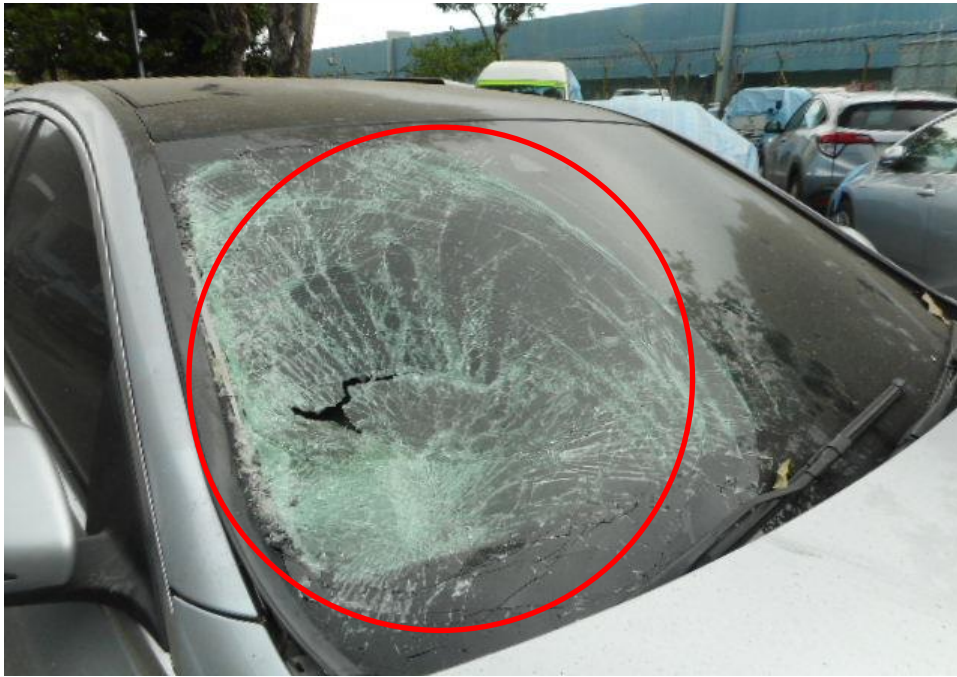
Photo 4 shows a close up view of the Motor Car's front body at the time of my inspection. The front portion of the Motor Car was observed to have sustained damage. Its front windscreen (circled) was the body parts that were damaged as a result of the accident.
