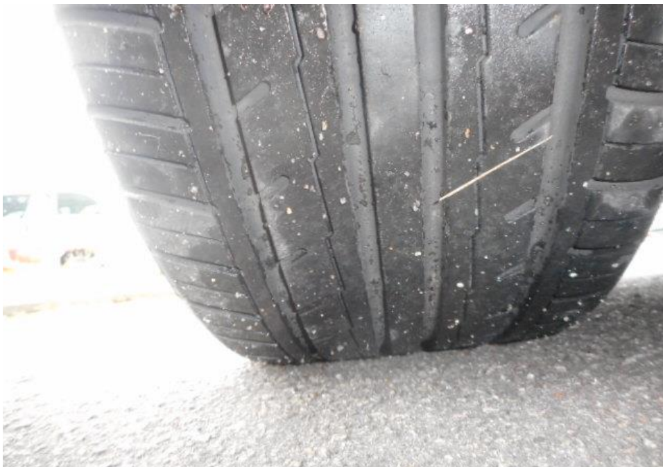
Photo 11 shows the condition of the front left tyre of the Motor Car, which was observed to be in serviceable condition with remaining tread depth of approximately 5.7mm. There was also no tear, cut or burst mark(s) on the outer and the inner sidewalls as well as across the tread of the Motor Car's 4 tyres.
