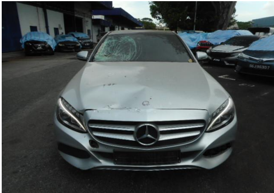
Photo 3 shows a general view of the Motor Car's front body at the time of my inspection. The front portion of the Motor Car was observed to have sustained damage. Its front windscreen, front bonnet and front bumper was amongst the body parts that were damaged as a result of the accident.
