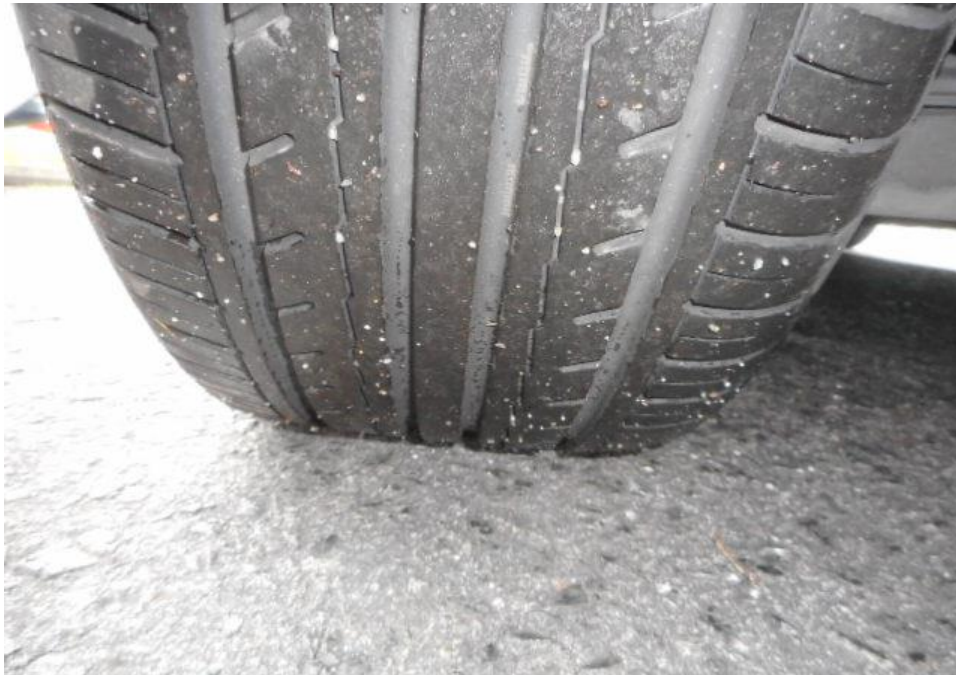
Photo 10 shows the condition of the rear left tyre of the Motor Car, which was observed to be in serviceable condition with remaining tread depth of approximately 5.8mm. The tyre, which was wrapped around alloy wheel rim, was also observed to be sufficiently inflated for vehicular operation. The 4 tyres of the Motor Car were wrapped around standard alloy wheel rims.
