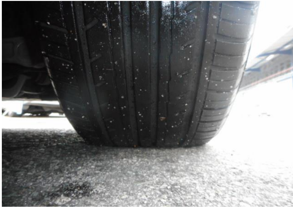
Photo 8 shows the condition of the front right tyre of the Motor Car, which was observed to be in serviceable condition with remaining tread depth of approximately 5.9mm. The tyre was sufficiently inflated for vehicular operation with no tear, cut or burst mark(s) on the outer and the inner sidewalls as well as across the tread. The 4 tyres of the Motor Car were wrapped around standard alloy wheel rims without any damage.
