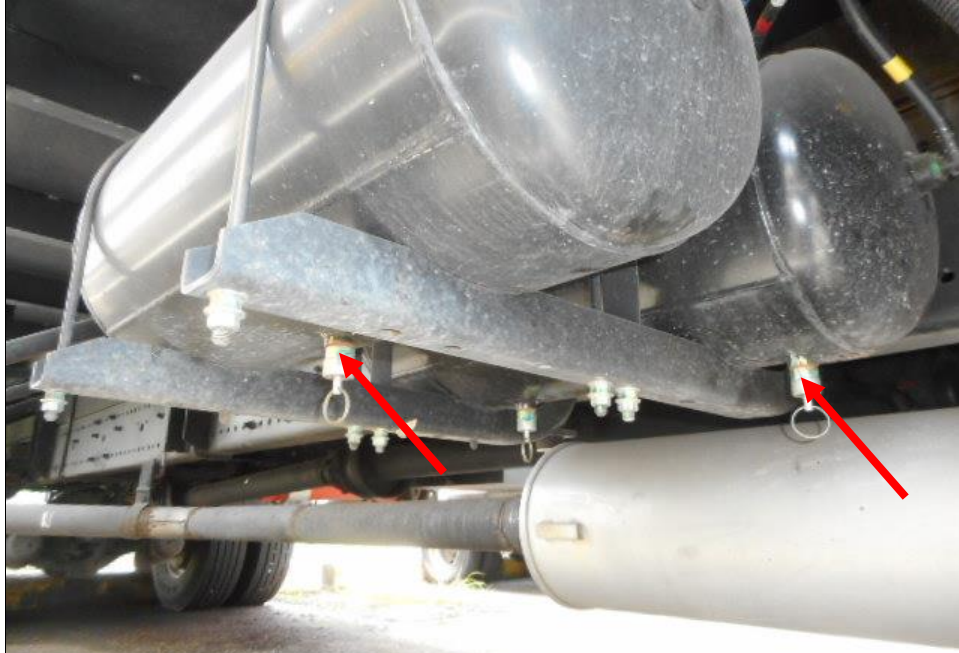
Photo 13 shows the air brake cylinders (arrowed) at the undercarriage of the Lorry. I did not observe any leakage of air brake fluid at the time of my inspection of the Lorry. My visual examination of the various mechanical components in the braking system had indicated that there was no internal leakage of pressure/vacuum and these components were generally in good condition.
