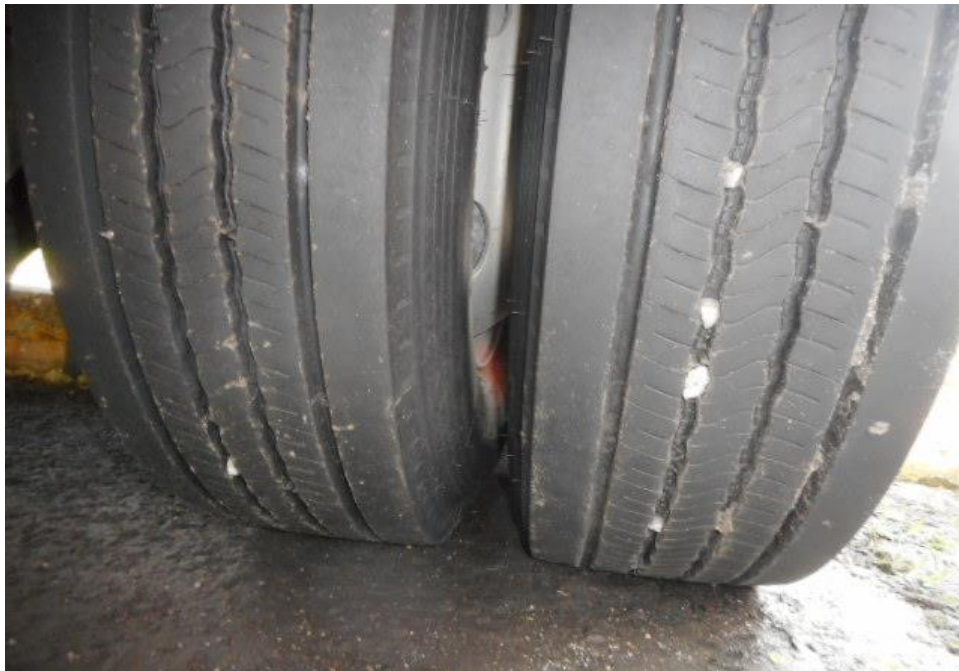
Photo 7 shows the condition of the rear left tyres of the Lorry, which was observed to be in serviceable condition with remaining tread depth of approximately 1.4mm. The tyres, which were wrapped around standard steel wheel rim, were also observed to be sufficiently inflated for vehicular operation. There was also no damage found on all 6 steel wheel rims of the Lorry.
