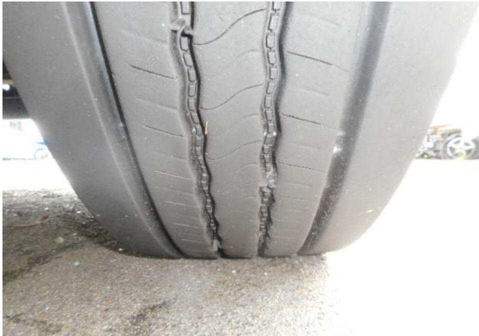
Photo 5 shows the condition of the front right tyre of the Lorry, which was observed to be in serviceable condition with remaining tread depth of approximately 12.7 mm. The tyre, which was wrapped around standard steel wheel rim, was also observed to be sufficiently inflated for vehicular operation. There was no tear, cut or burst mark(s) on the outer and the inner sidewalls as well as across the tread of the 6 tyres that were fitted on the Lorry.
