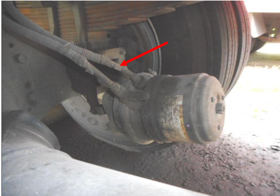
Photo 9 shows the brake pipe (arrowed) at the rear right wheel of the Lorry. I did not observe any leakage of brake fluid at the time of my inspection of the Lorry. My visual examination of the various mechanical components in the braking system, had indicated that there was no internal leakage of pressure/vacuum and there components were generally in good condition.
