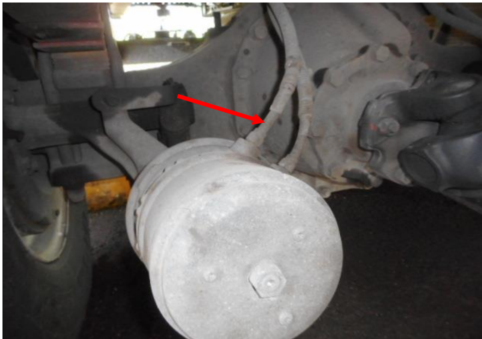
Photo 10 shows the brake pipe (arrowed) at the rear left wheel of the Lorry. I did not observe any leakage of brake fluid at the time of my inspection of the Lorry. My static tests of the Lorry's braking system, along with my visual examination of the various mechanical components in the braking system, had indicated that there was no internal leakage of pressure/vacuum and there components were generally in good condition.
