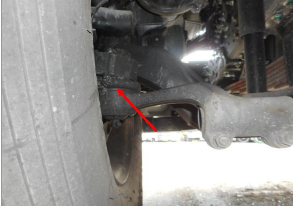
Photo 15 shows the various undercarriage components at the front left wheel of the Lorry, in particular the steering tie rod end (arrowed). The various undercarriage components of the Lorry were all found to be intact without any visible damage. There was also no sign of fluid stain(s) observed on the various undercarriage components.
