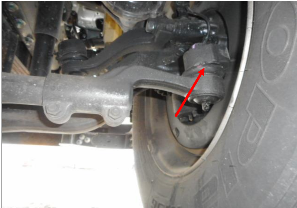
Photo 14 shows the various undercarriage components at the front right wheel of the Lorry, in particular the steering tie rod end (arrowed). The various steering components were all found to be intact, suggesting that the steering system of the Lorry was likely to be in serviceable condition at the material time of accident. There was also no sign of fluid stain(s) observed on the various undercarriage components.
