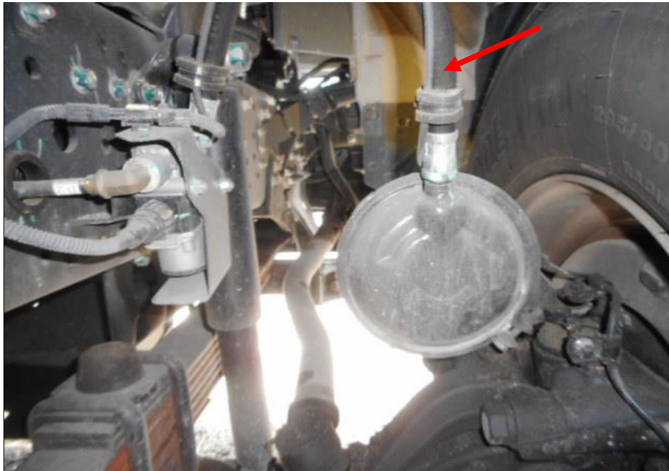
Photo 11 shows the brake pipe (arrowed) at the front right wheel of the Lorry. I did not observe any leakage of brake fluid at the time of my inspection of the Lorry. My static tests of the Lorry's braking system, along with my visual examination of the various mechanical components in the braking system, had indicated that there was no internal leakage of pressure/vacuum and there components were generally in good condition.
