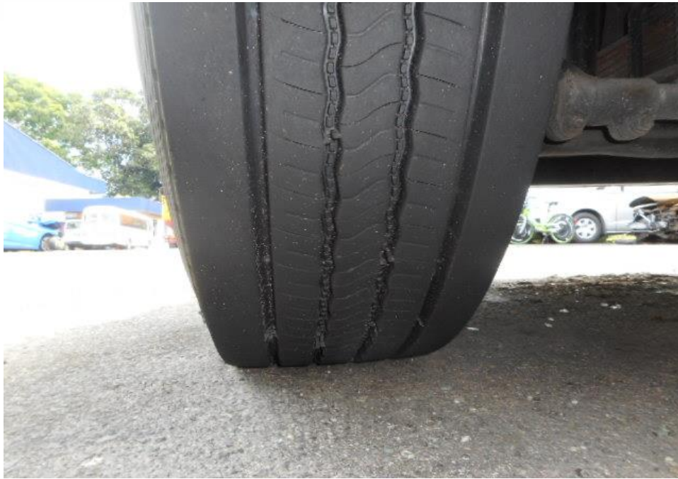
Photo 8 shows the condition of the front left tyres of the Lorry, which were observed to be in serviceable condition with remaining tread depth of approximately 12.7mm. There was also no tear, cut or burst mark(s) on the outer and the inner sidewalls as well as across the tread of the 12 tyres that were fitted on the Lorry.
