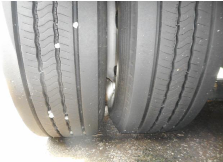
Photo 6 shows the condition of the rear right tyre of the Lorry, which was observed to be in serviceable condition with remaining tread depth of approximately 12.9mm. The tyre, which was wrapped around standard steel wheel rim, was also observed to be sufficiently inflated for vehicular operation.
