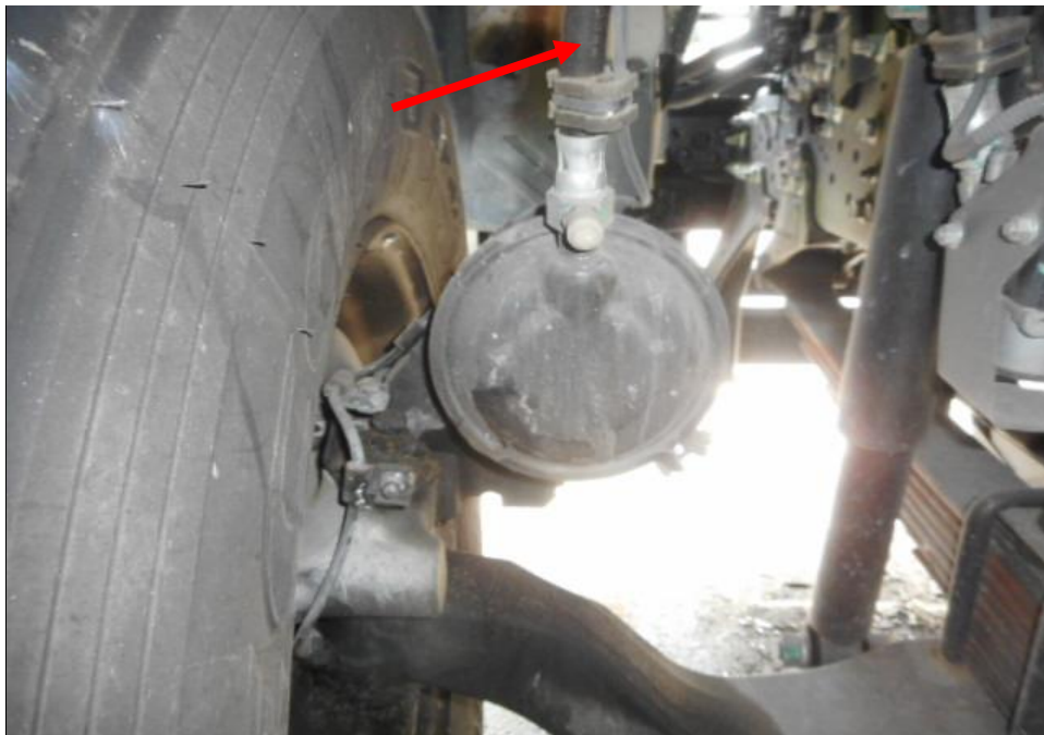
Photo 12 shows the brake pipe (arrowed) at the front left wheel of the Lorry. I did not observe any leakage of brake fluid at the time of my inspection of the Lorry. My visual examination of the various mechanical components in the braking system had indicated that there was no internal leakage of pressure/vacuum and there components were generally in good condition.
