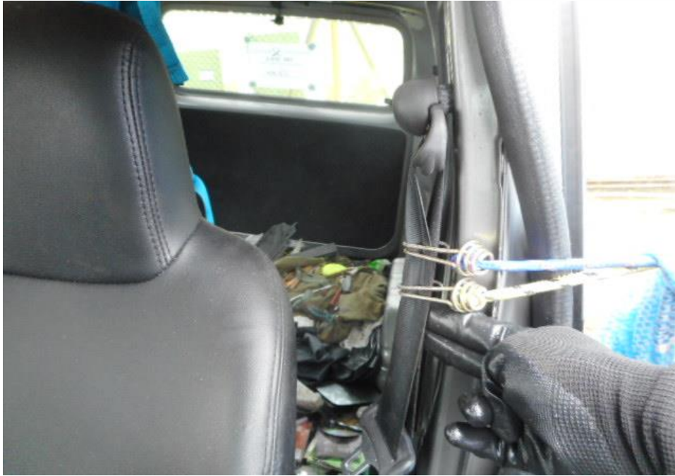
Photo 30 shows that the seat belt on the left seat was not worn at the material time of accident as the safety pre-tensioners was activated at the moment of impact and caused the seat belt to be locked into the last position.
