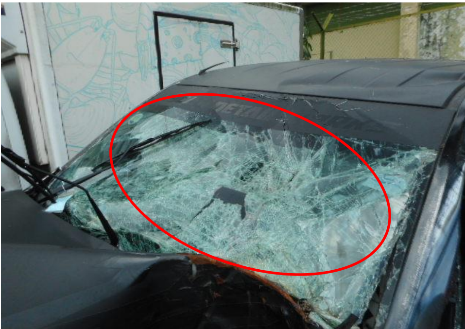
Photo 4 shows the close up view of the Motor Van's front body at the time of my inspection. The Motor Van was observed to have sustained damage at its front portion. Its front windscreen (circled) was damaged as a result of the accident.
