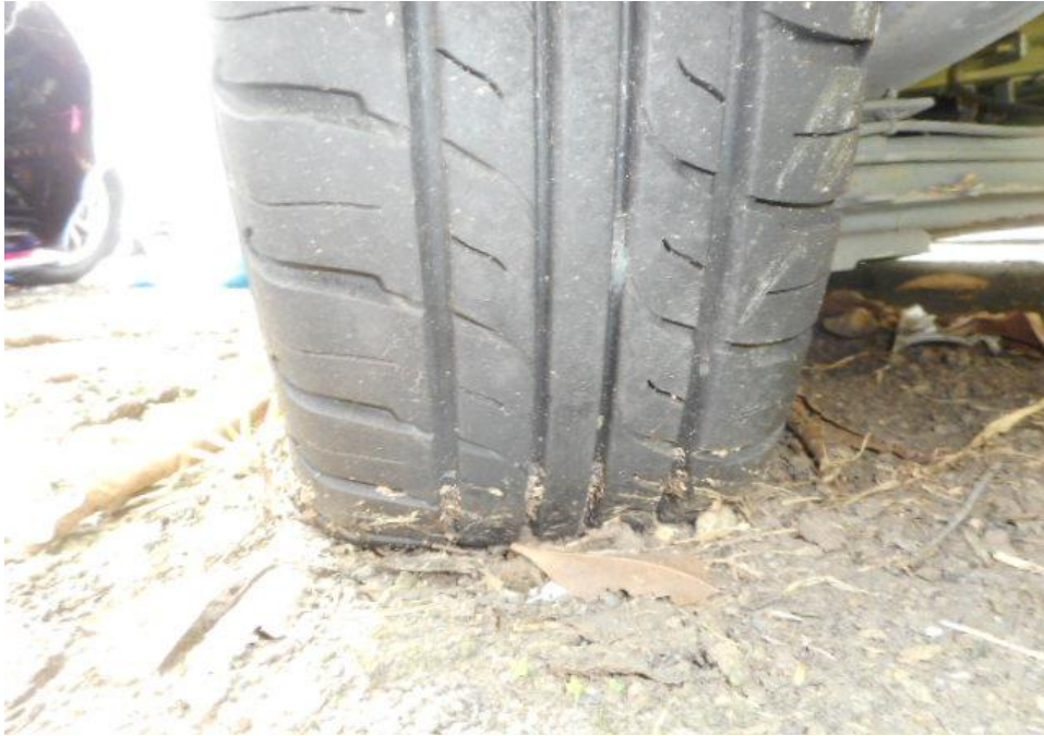
Photo 13 shows the condition of the rear left tyre of the Motor Van, which was observed to be in serviceable condition with remaining tread depth of approximately 6mm. The tyre was also observed to be sufficiently inflated for vehicular operation with no tear, cut or burst mark(s).
