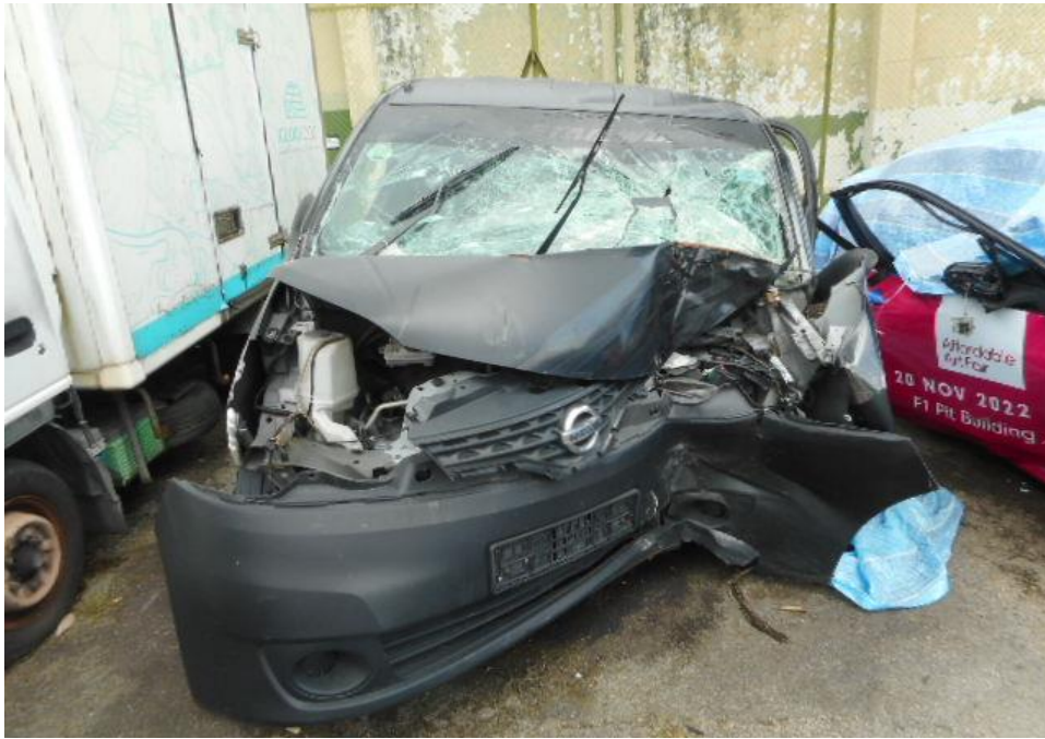
Photo 3 shows a general view of the Motor Van's front body at the time of my inspection. The Motor Van was observed to have sustained damage at its front and left portion. Its windscreen, front bonnet, front bumper, front left fender and left door was the body parts and various engine compartments were also damaged as a result of the accident. The Supplemental Restraint System (SRS) was activated as a result of the accident.
