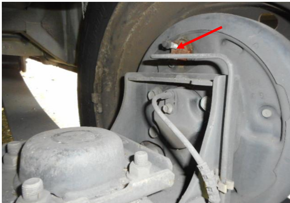
Photo 28 shows the brake hose/pipe (arrowed) at the rear right wheel of the Motor Van. No leakage of brake fluid was observed. Visual examination of the various components of the braking system like the drum brake etc. had revealed all to be intact and without visible damage.
