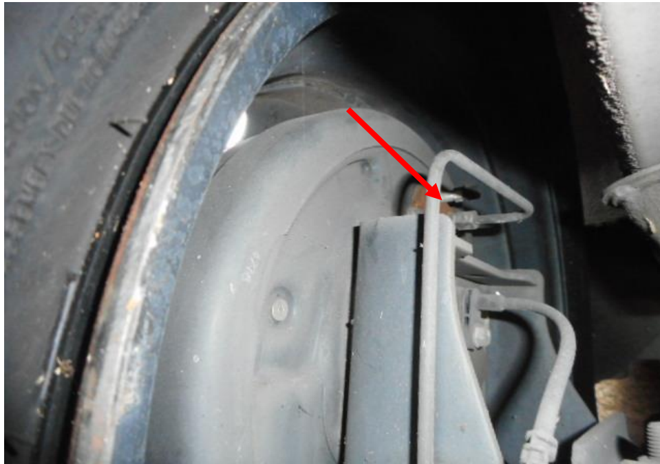
Photo 27 shows the brake hose/pipe (arrowed) at the rear left wheel of the Motor Van. No leakage of brake fluid was observed. Visual examination of the various components of the braking system like the drum brake etc. had revealed all to be intact and without visible damage.
