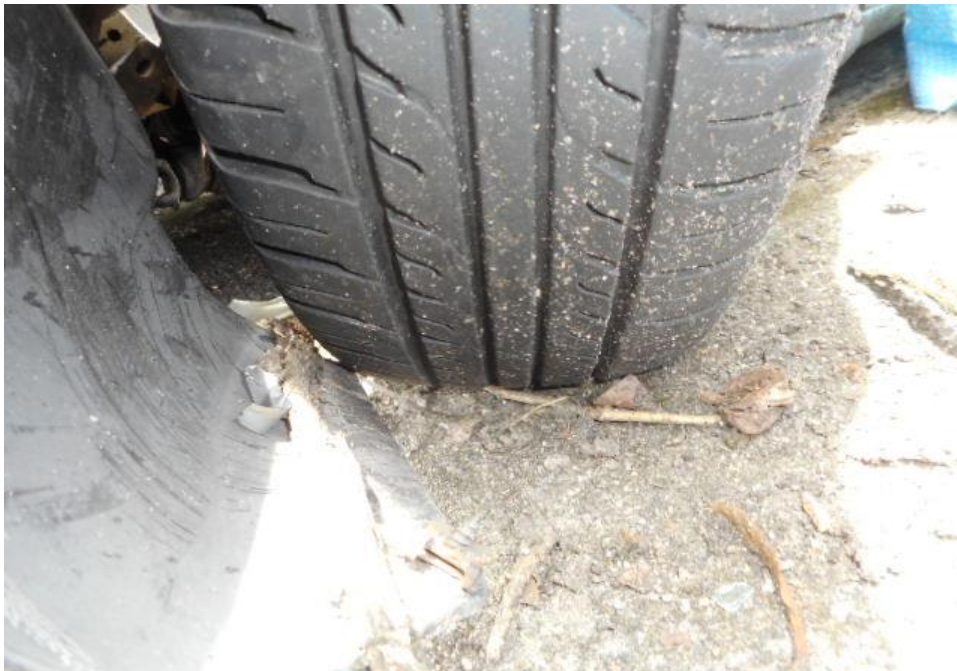
Photo 14 shows the condition of the front left tyre of the Motor Van, which was observed to be in serviceable condition with remaining tread depth of approximately 5.8mm. The tyre was also observed to be sufficiently inflated for vehicular operation with no tear, cut or burst mark(s).
