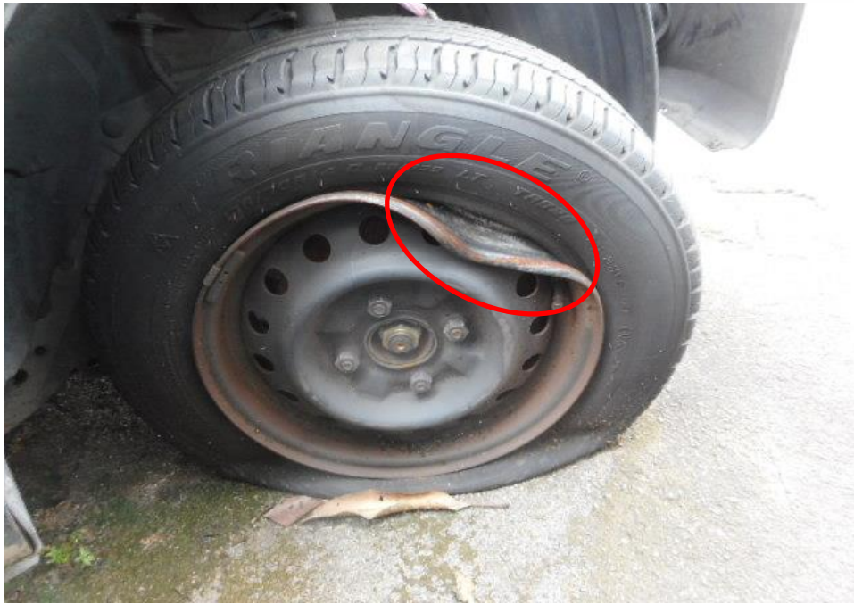
Photo 11 shows the close up condition of the front right tyre and wheel rim of the Motor Van, the wheel rim was dented and the tyre was observed to be and deflated (circled) as a result of the accident with remaining tread depth of approximately 5.9mm.
