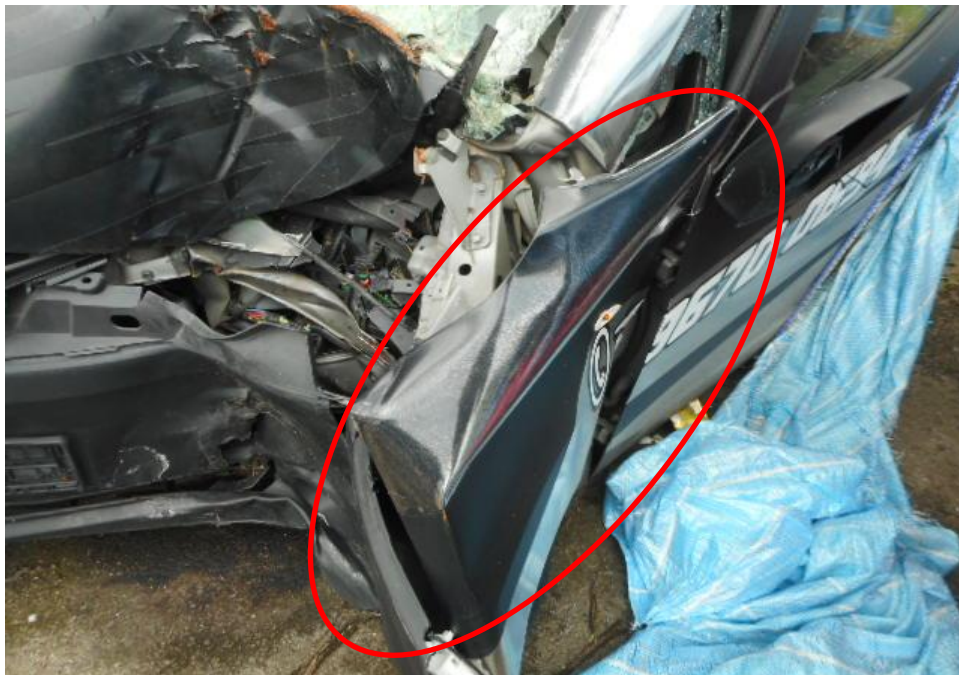
Photo 6 shows the close up view of the Motor Van's front body at the time of my inspection. The Motor Van was observed to have sustained damage at its front portion. Its front left fender (circled) was damaged as a result of the accident.
