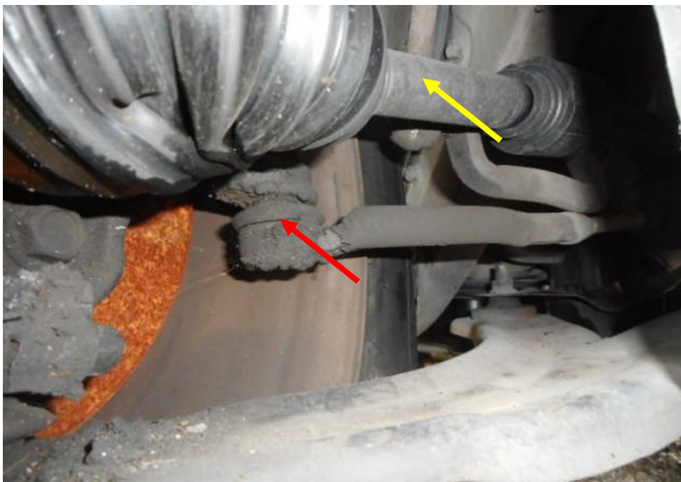
Photo 24 shows the various undercarriage components at the front right wheel of the Motor Van, in particular the steering tie rod (red arrow) and right driveshaft (yellow arrow) was observed to be intact.
