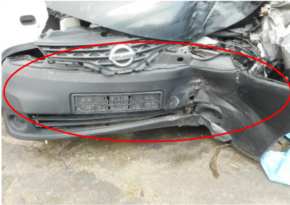
Photo 5 shows the close up view of the Motor Van's front body at the time of my inspection. The Motor Van was observed to have sustained damage at its front portion. Its front bumper (circled) was damaged as a result of the accident.
