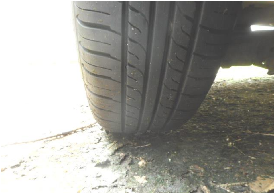
Photo 12 shows the general condition of the rear right tyre of the Motor Van, which was observed to be in serviceable condition with remaining tread depth of approximately 6m. The tyre was also observed to be sufficiently inflated for vehicular operation with no tear, cut or burst mark(s).
