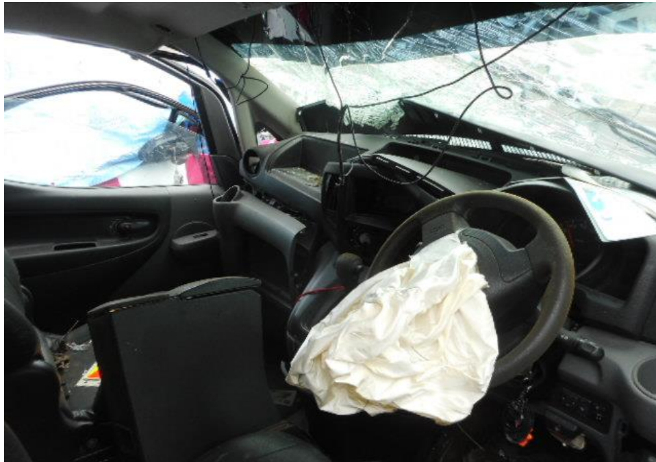
Photo 15 shows the deployment of the Supplemental Restraint System (SRS) airbag in the Motor Van as a result of the accident.
