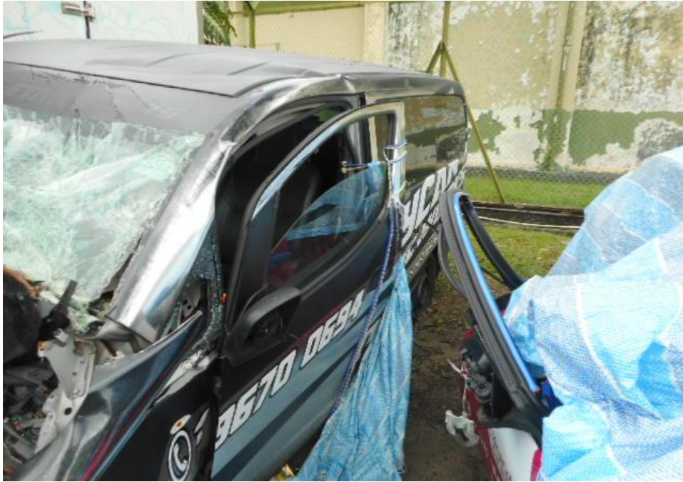
Photo 7 shows a general view of the Motor Van's left body at the time of my inspection. The Motor Van was observed to have sustained damage at its left portion. Its left door (circled) was damaged as a result of the accident.
