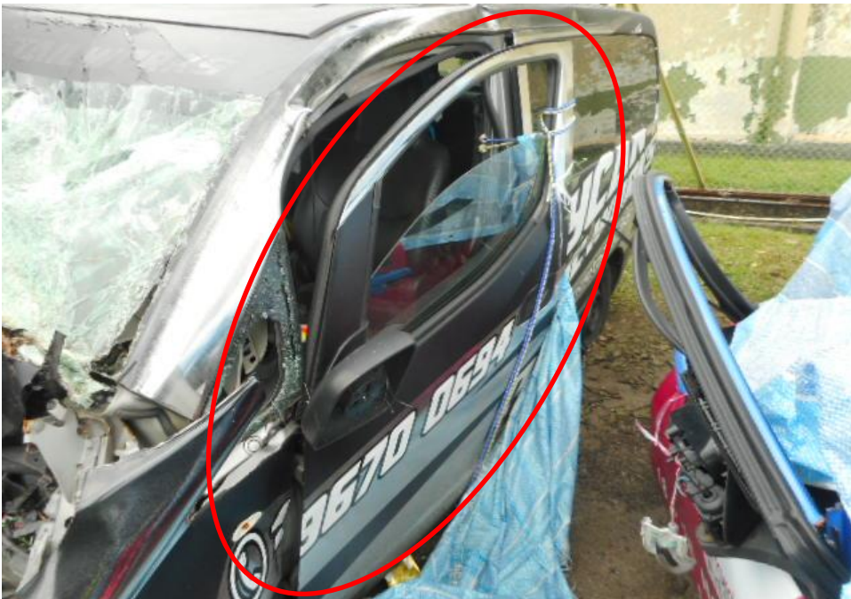
Photo 8 shows the close up view of the Motor Van's left body at the time of my inspection. The Motor Van was observed to have sustained damage at its left portion. Its left door (circled) was damaged as a result of the accident.
