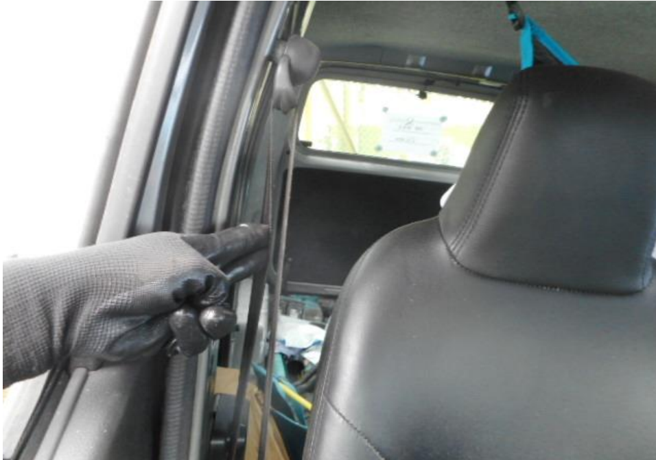
Photo 29 shows that the seat belt on the right seat was not worn at the material time of accident as the safety pre-tensioners was activated at the moment of impact and caused the seat belt to be locked into the last position.
