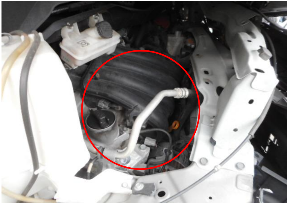
Photo 18 shows the close up view of the Motor Van's front body at the time of my inspection. The Motor Van was observed to have sustained damage at its front portion. Its engine (circled) was amongst the various components in the engine compartments were also damaged as a result of the accident.
