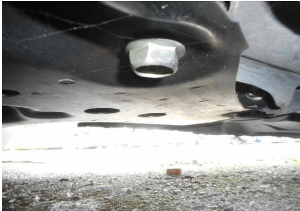
Photo 21 shows the undercarriage of the Motor Van, at the area where the engine housing and transmission housing are located. I did not find any sign(s) or indication(s) of fluid leak and/or fluid stain(s) on the underside of the Motor Van.
