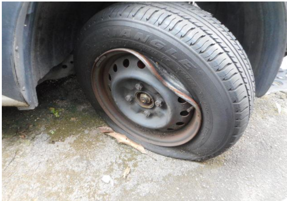
Photo 10 shows the general condition of the front right tyre and wheel rim of the Motor Van. The wheel rim was observed to be dented and its tyre was observed deflated as a result of the accident.
